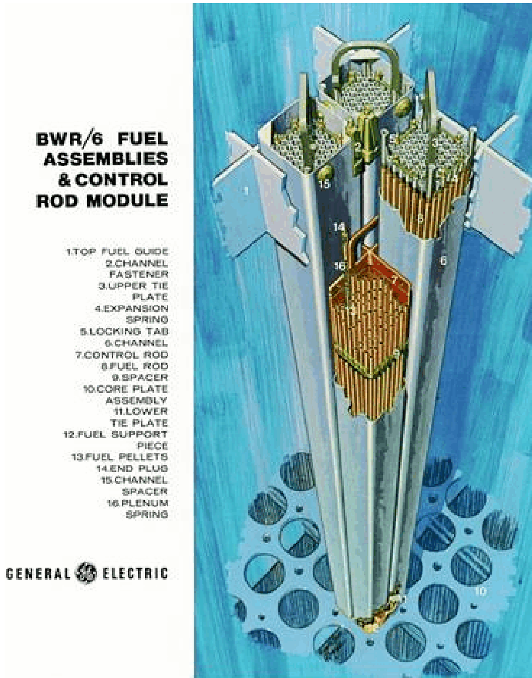
Fig. //2// BWR fuel assembly
