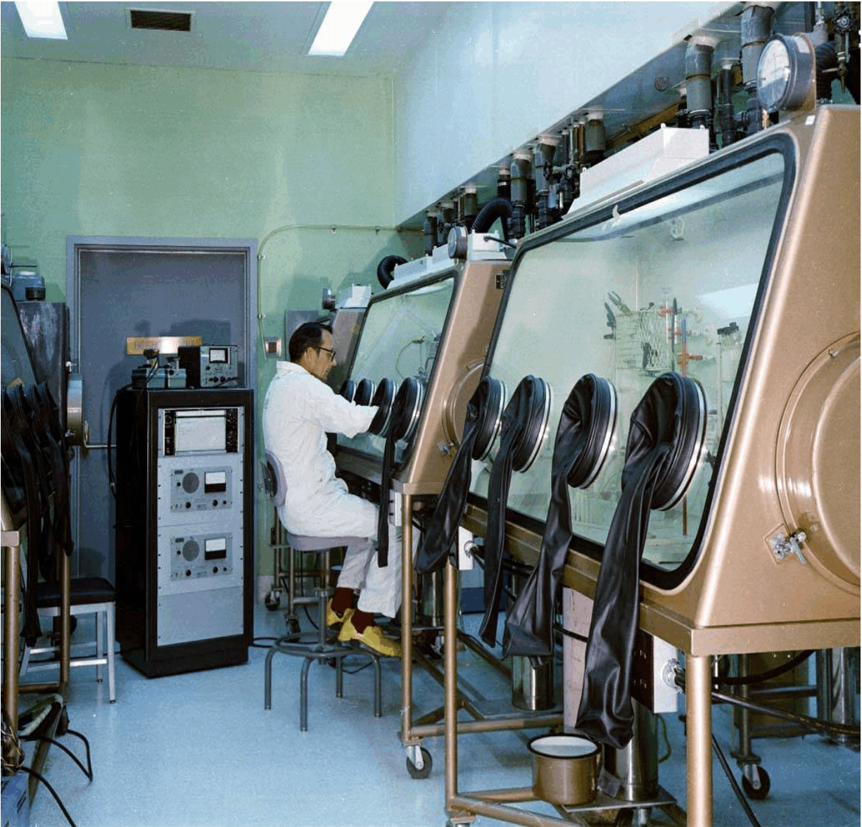
Fig. //10// Glove boxes used for handling nuclear materials having low levels of penetrating radiation
