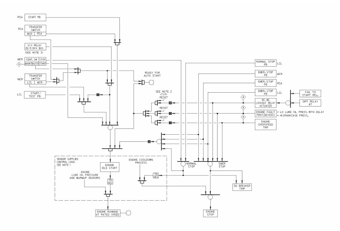
On-Site Standby Diesel Generator Initiating Circuit Logic Diagram
