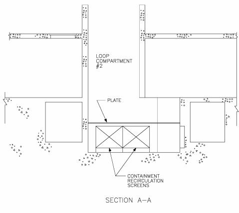
NOTE 1 - MINIMUM PLATE SIZE AND ELEVATION LIMITS ARE DEFINED IN SUBSECTION 6.3.2.2.7.1.
