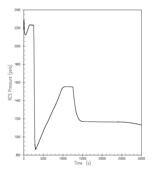
Figure 15.6.3-2 **Reactor Coolant System Pressure for SGTR**
