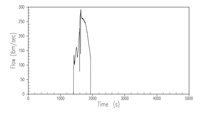
Figure 15.6.5.4B-24 **2-Inch Cold Leg Break – Accumulator-1 Injection Rate**
