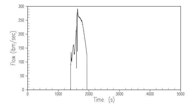
Figure 15.6.5.4B-25 **2-Inch Cold Leg Break – Accumulator-2 Injection Rate**
