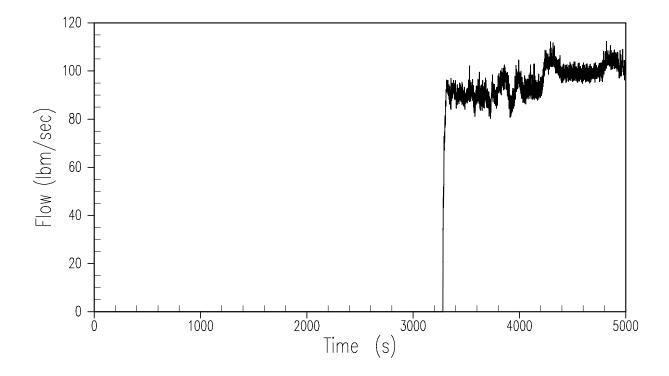
Figure 15.6.5.4B-26 **2-Inch Cold Leg Break – IRWST-1 Injection Rate**
