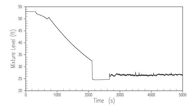
Figure 15.6.5.4B-7 **Inadvertent ADS – CMT-1 Mixture Level**
