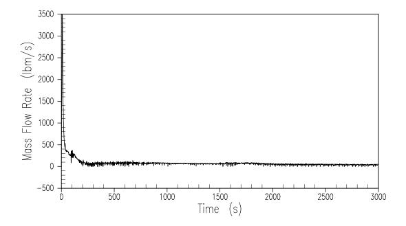
Figure 15.6.5.4B-72 **10-Inch Cold Leg Break – Core Exit Vapor Flow**
