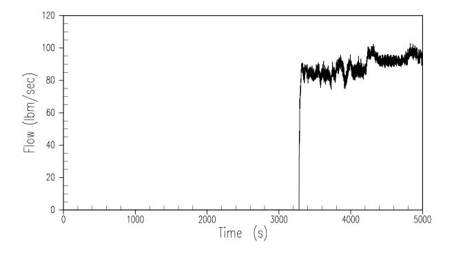
Figure 15.6.5.4B-27 **2-Inch Cold Leg Break – IRWST-2 Injection Rate**
