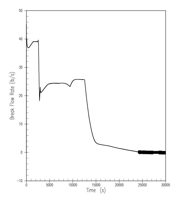
Figure 15.6.3-5 **Primary-to-Secondary Break Flow Rate for SGTR**
