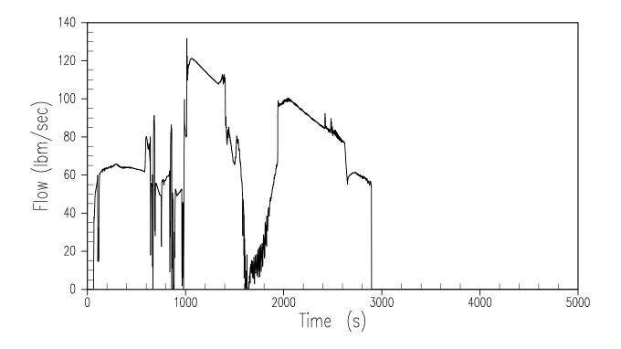
Figure 15.6.5.4B-22 **2-Inch Cold Leg Break – CMT-1 Injection Rate**
