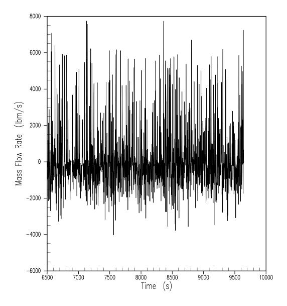
Figure 15.6.5.4C-7A Liquid Flow Rate out of the Core
