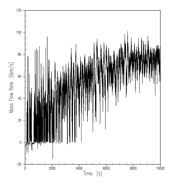
Figure 15.6.5.4C-14 **DVI–B Mixture Flow Rate**(**DEDVI Case**)
