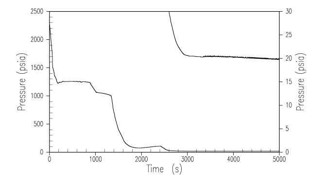
Figure 15.6.5.4B-17 **2-Inch Cold Leg Break – RCS Pressure**
