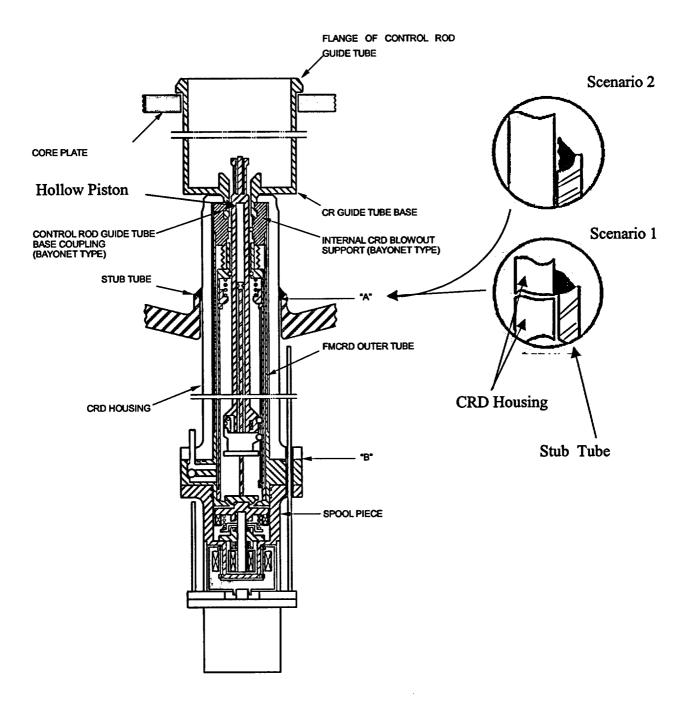
Figure 1: Internal CRD Blowout Support Schematic (from DCD Tier 2, figure 4.6-7 with additional information)
