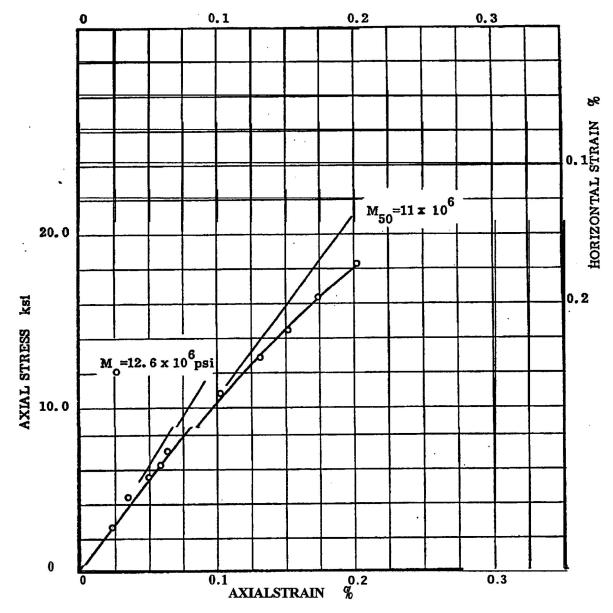
Diorite M = Modulus of Deformation Borehole E1-1 Depth 79.5 to 79.3 ft
