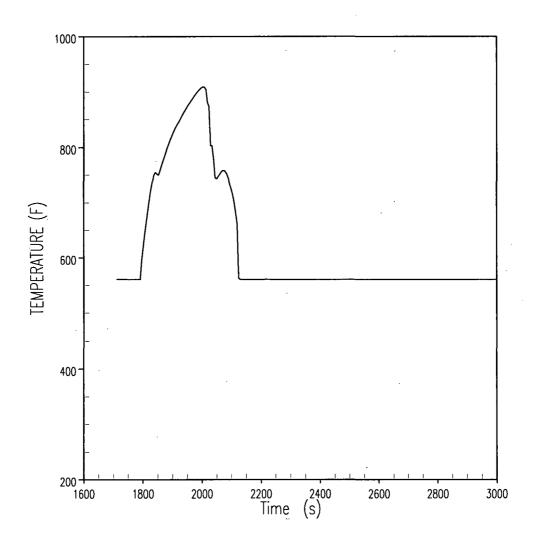
Figure 2-1: Salem Unit 2 RSG SBLOCA Analysis 2-inch PCT Results
