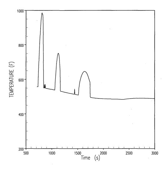
Figure 2-2: Salem Unit 2 RSG SBLOCA Analysis 3-inch PCT Results
