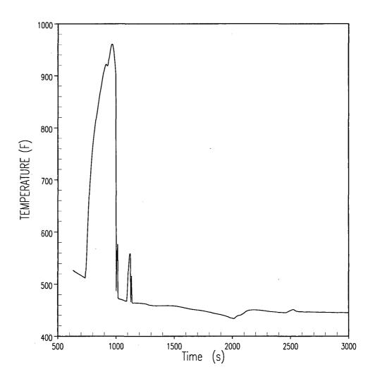
Figure 2-3: Salem Unit 2 RSG SBLOCA Analysis 4-inch PCT Results
