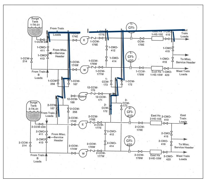
**CT:** Student correctly Highlightshighlights flowpath between 1E CCW and Unit 2 CCW system on Figure 4.
