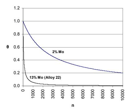
Figure 5. Current transient during crevice corrosion propagation of Alloy 22 in 5 M NaCl solutions at 95  $^{\circ}$ C [203  $^{\circ}$ F] (He and Dunn, 2005). [cm<sup>2</sup> = inch<sup>2</sup>/6.45]
