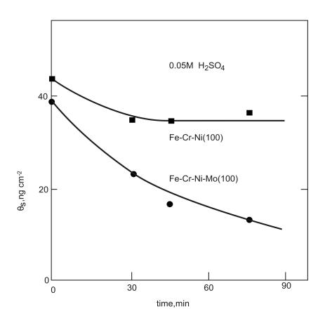
Figure 4. Calculated sulfur dissolution kinetics for 13 % Mo (Alloy 22 case) based on the model by Marcus and Moscatelli (1989). " $\theta$ " is fractional sulfur coverage; and "n" is atomic plane number under corrosion ~ 1-hour corrosion for 10,000. The upper curve is the model fitted to experimental data of Ni-2Mo (a/o), from Marcus and Moscatelli (1989)
