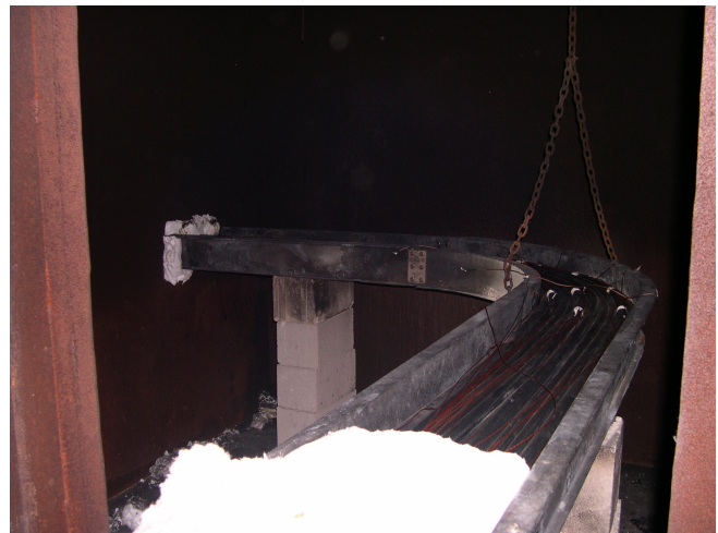
Figure 3.6 – Photo of Test Assembly Positioned in Test Chamber
