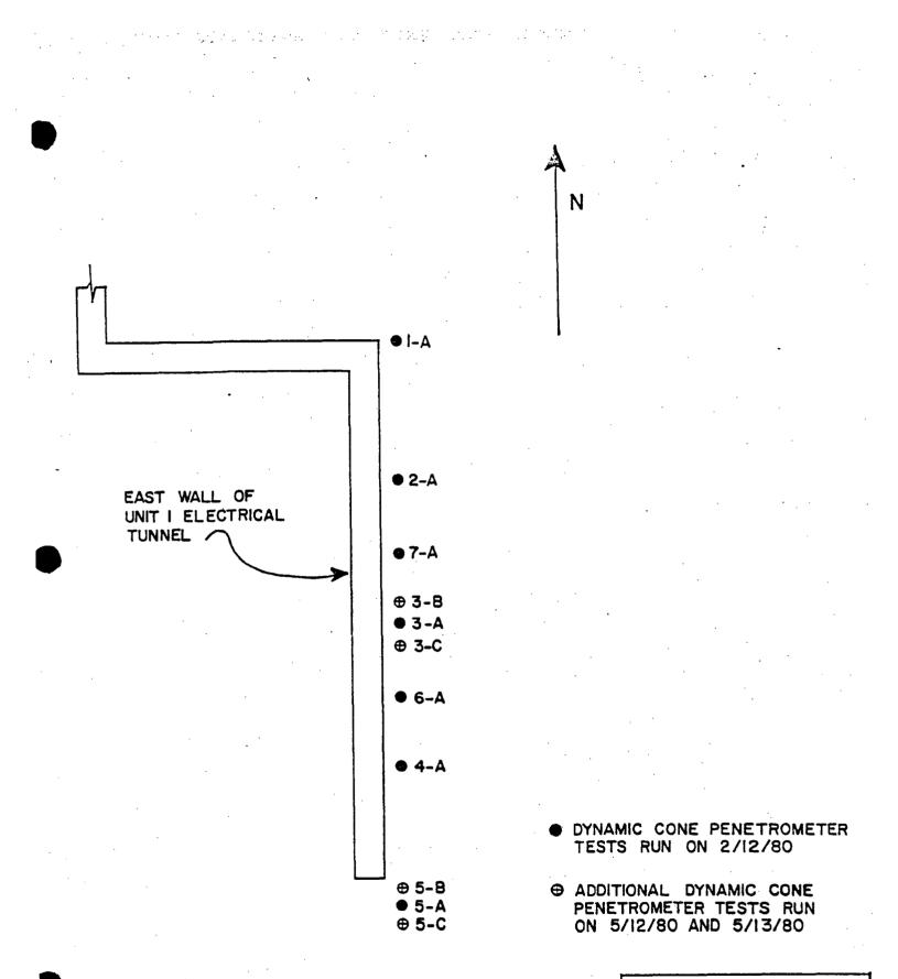
PLAN SHOWING LOCATIONS OF DYNAMIC CONE PENETROMETER TESTS ADJACENT TO ELECTRICAL TUNNEL EAST WALL.
