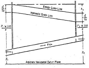
Figure 1-4 Energy Balance for Two Paints in a Fluid
