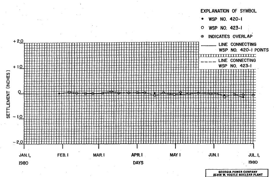
SETTLEMENT VERSUS TIME FOR ELECTRICAL TUNNEL UNIT I SCALE: DRAWING NO. REV. JOB NO. 9510 FIGURE 16-4A
