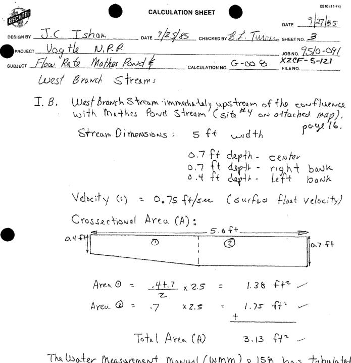
The Water Measurement Manual (WMM) p 158 has tabulated a series of correction coefficients which relates the surface velocity to average stream velocity. These coefficients are based on the roughness of the channel & tho depth of the channel.
