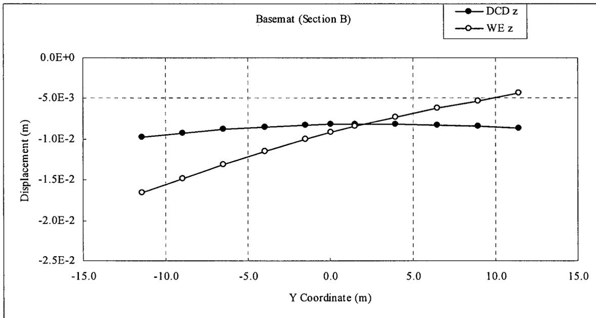
Figure 3.8-93 (11)-b Comparison of Settlement (CB, W -E direction)
