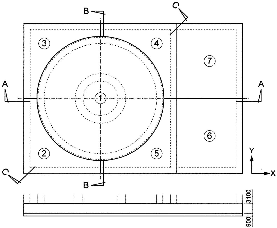
Figure 3.8-93(25) Zone of Basemat for Concrete Pour
