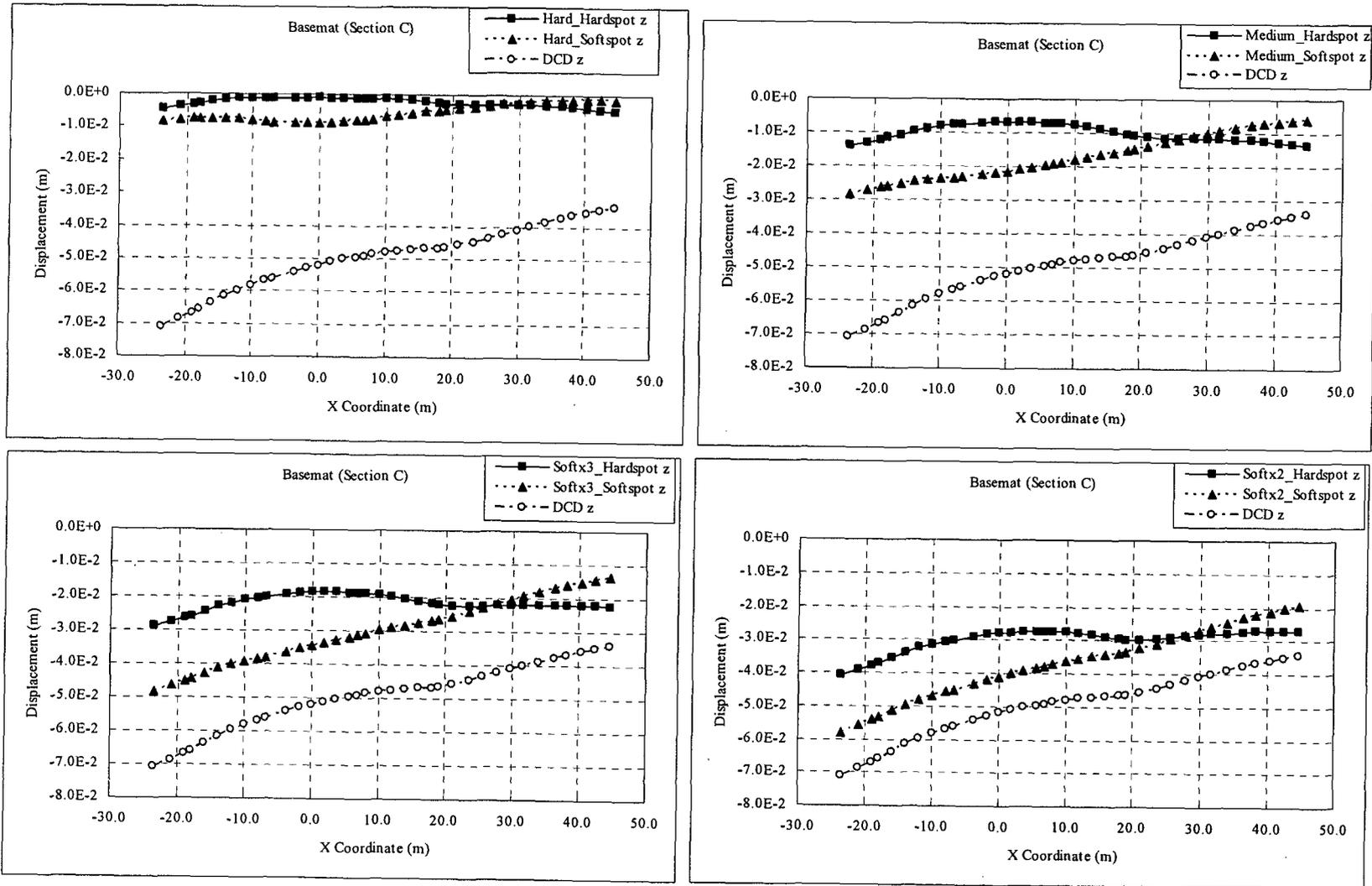
Figure 3.8-93 (15)-b Comparison of Basemat Deformation N-S Section)
