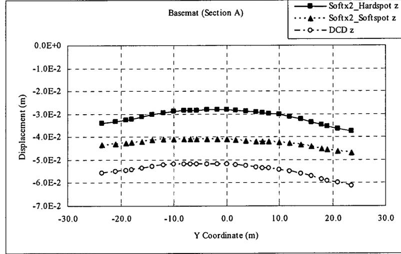
Figure 3.8-93 (15) -a Comparison of Basemat Deformation (E-W Section)
