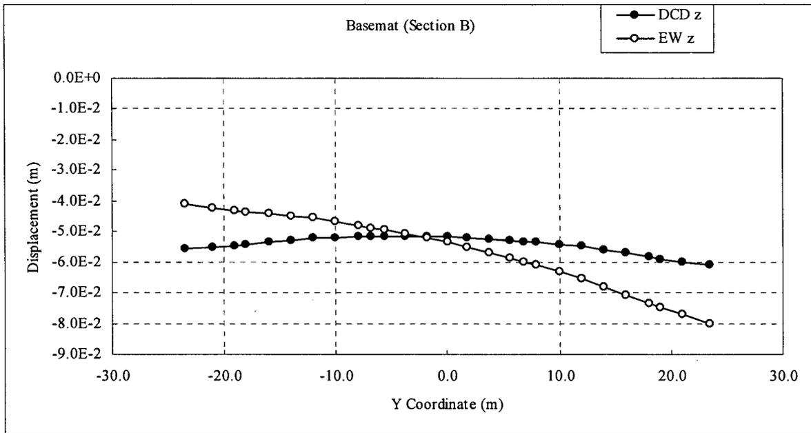
**Figure 3.8-93 (10)-a Comparison of Settlement (RBF, E-W direction)**
