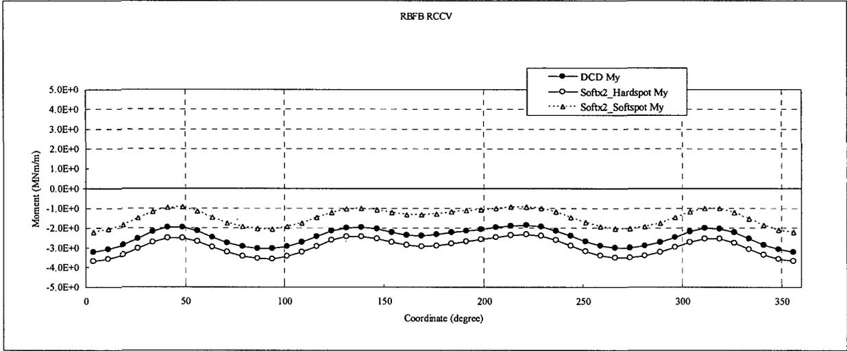
Figure 3.8-93 (18)-d Comparison of Sectional Moments (RCCV bottom, Soft x2)
