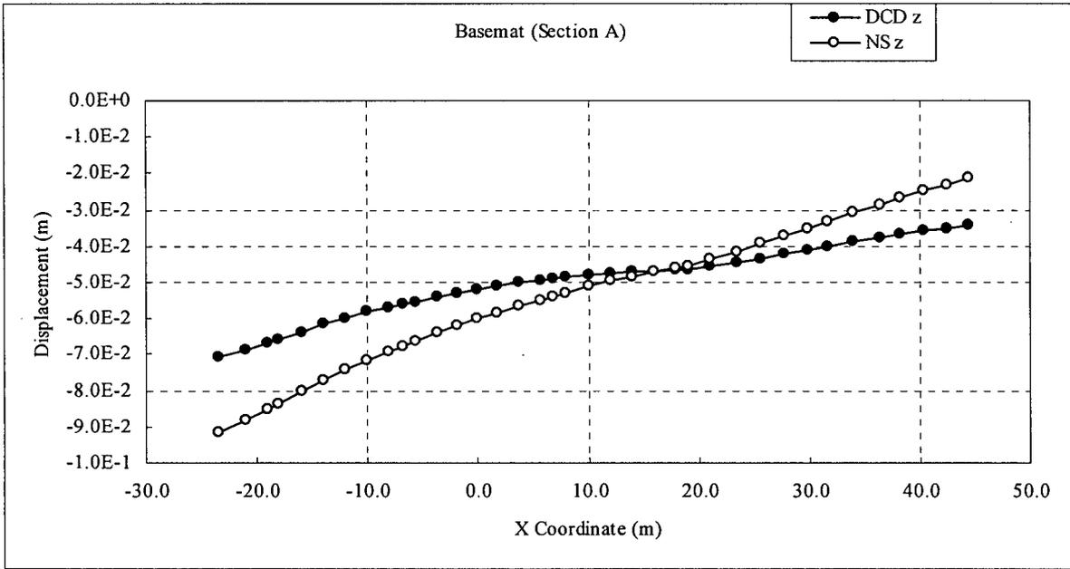
Figure 3.8-93 (10)-c Comparison of Settlement (RBF, N-S direction)
