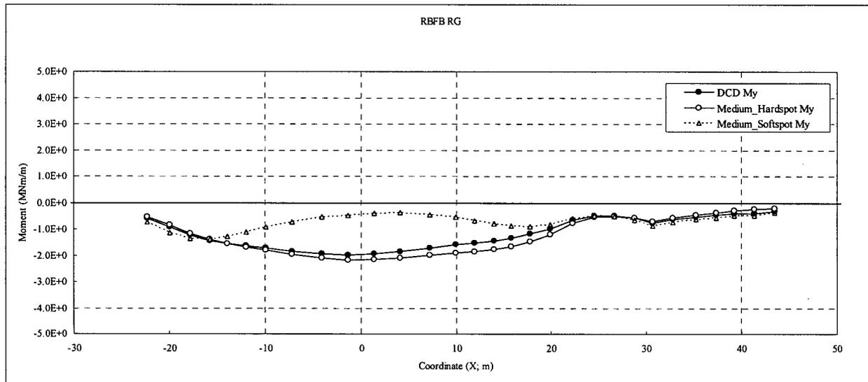
Figure 3.8-93 (23)-b Comparison of Sectional Moments (RG, Medium)
