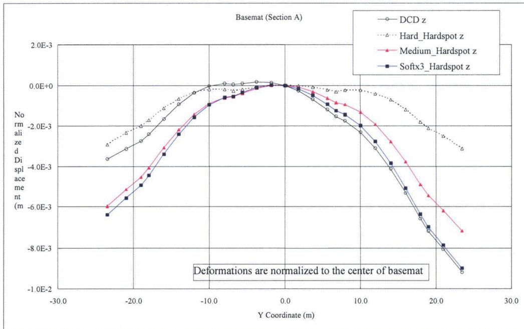
Figure 3.8-93 (24)-a Comparison of Normalized Basemat Displacement (E-W Section)
