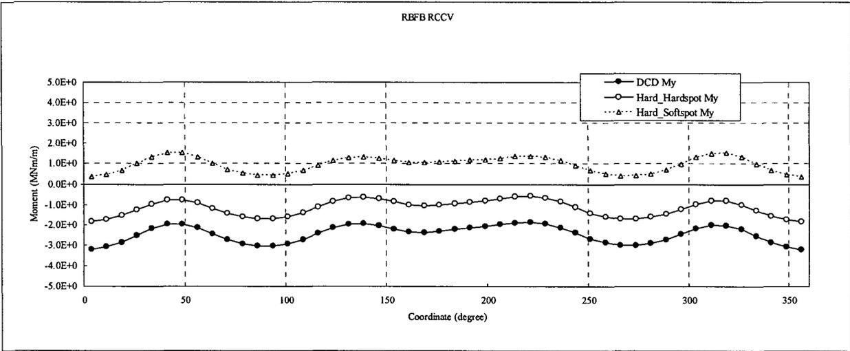
Figure 3.8-93 (18)-a Comparison of Sectional Moments (RCCV bottom, Hard)
