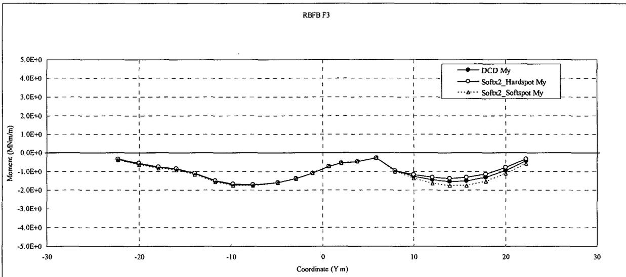
Figure 3.8-93 (21)-d Comparison of Sectional Moments (F3, Soft x2)
