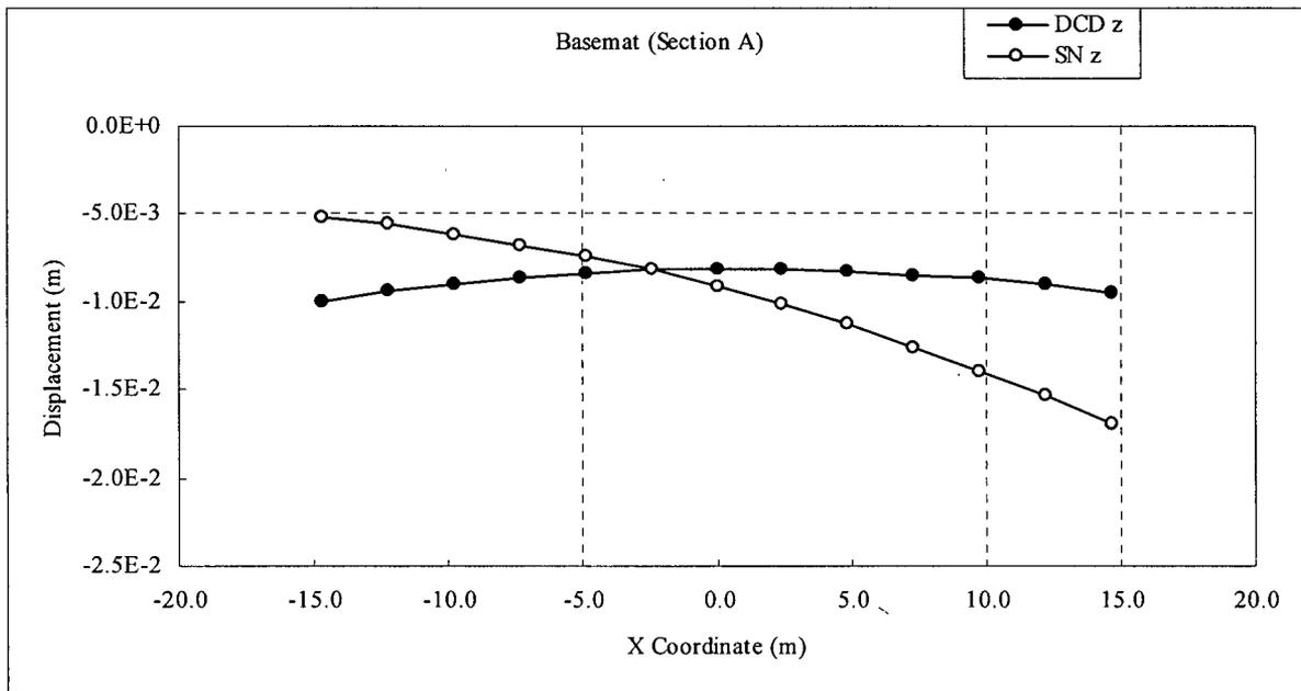
Figure 3.8-93 (11)-d Comparison of Settlement (CB, S-N direction)
