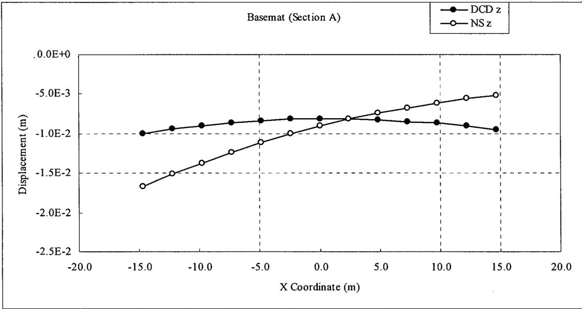
Figure 3.8-93 (11)-c Comparison of Settlement (CB, N-S direction)
