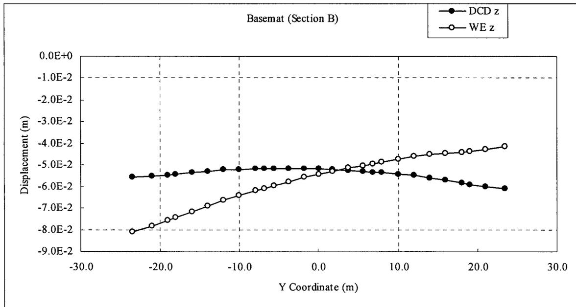
**Figure 3.8-93 (10)-b Comparison of Settlement (RBF, W-E direction)**
