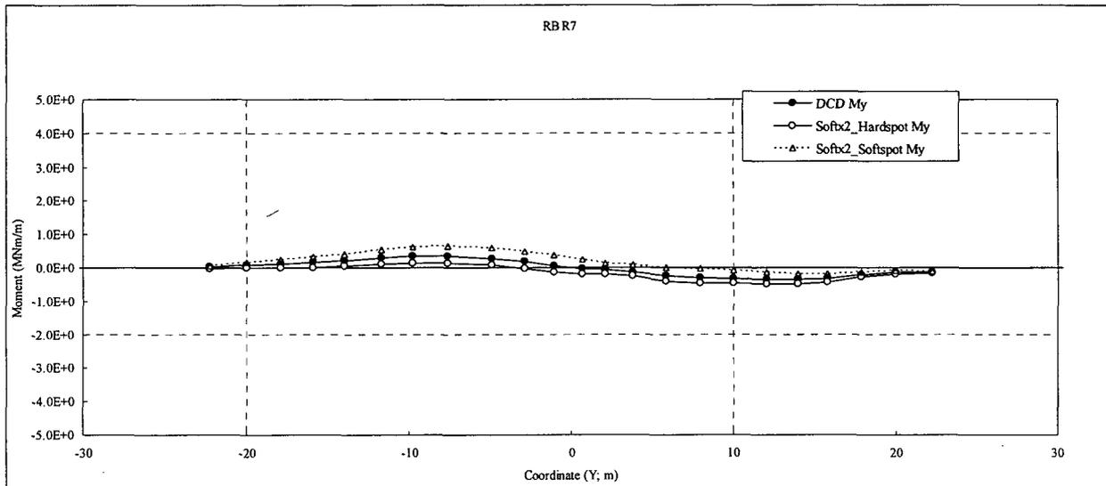
Figure 3.8-93 (20)-d Comparison of Sectional Moments (R7, Soft x2)
