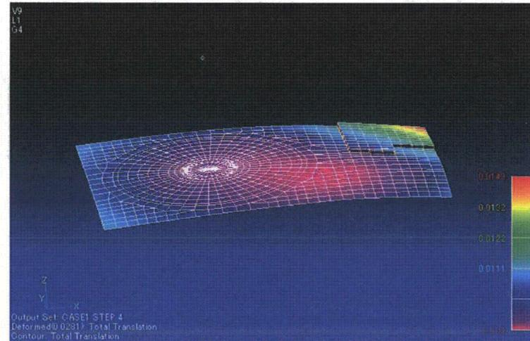
Figure 3.8-93(5) -c Deformation of basemat (CaseA - Step 3) Figure 3.8-93(5) -d Deformation of basemat (CaseA - Step 4)
