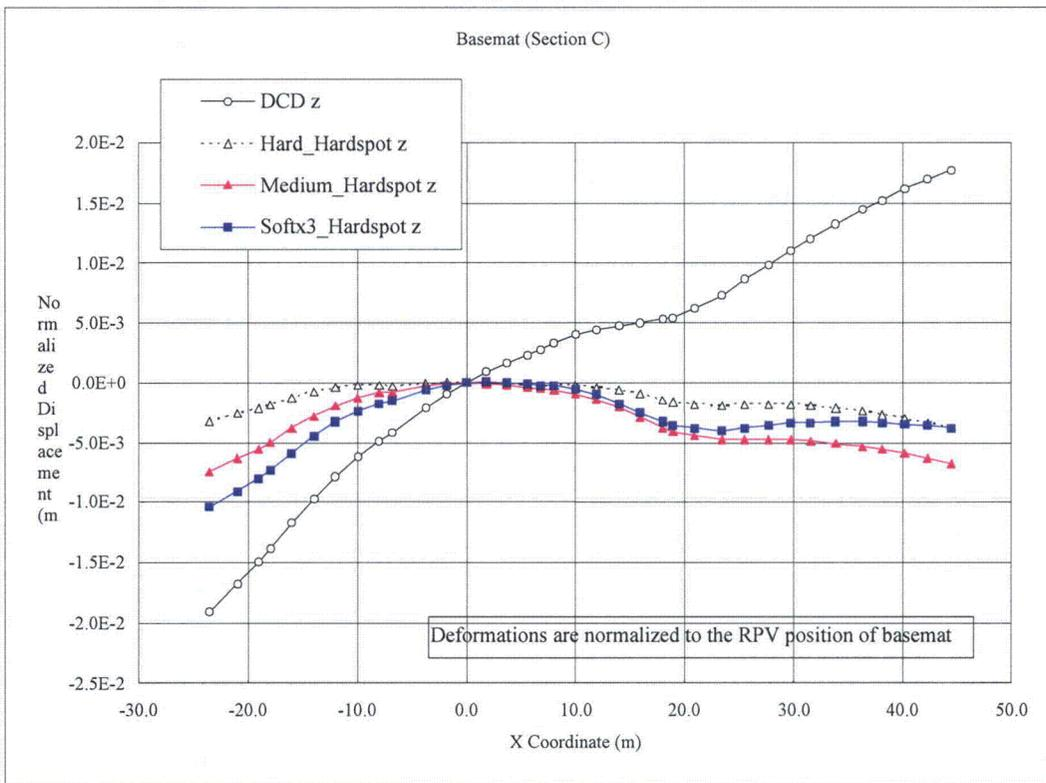
Figure 3.8-93 (24)-b Comparison of Normalized Basemat Displacement (N-S Section)
