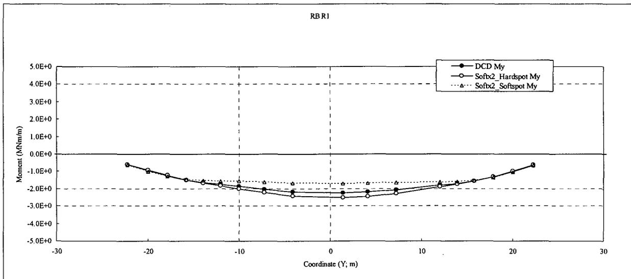
Figure 3.8-93 (19)-d Comparison of Sectional Moments (R1, Soft x2)
