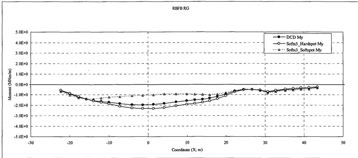
Figure 3.8-93 (23)-c Comparison of Sectional Moments (RG, Soft x3)
