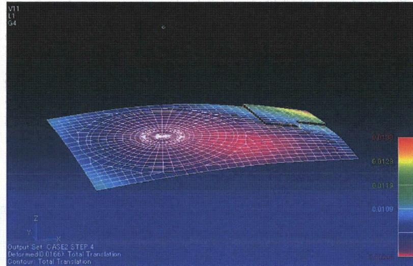
**Figure 3.8-93(6) -c Deformation of basemat (CaseB - Step 3) Figure 3.8-93(6) -d Deformation of basemat (CaseB - Step 4)**
