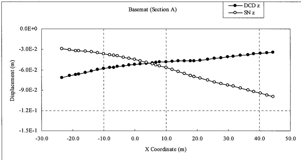
Figure 3.8-93 (10)-d Comparison of Settlement (RBF, S-N direction)
