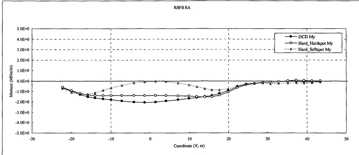
Figure 3.8-93 (22)-a Comparison of Sectional Moments (RA, Hard)
