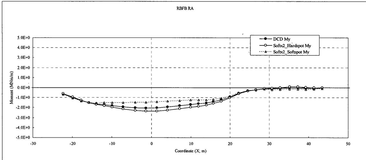
Figure 3.8-93 (22)-d Comparison of Sectional Moments (RA, Soft x2)
