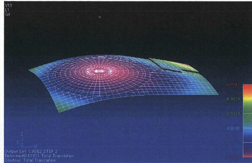
**Figure 3.8-93(6) -a Deformation of basemat (CaseB - Step 1) Figure 3.8-93(6) -b Deformation of basemat (CaseB - Step 2)**
