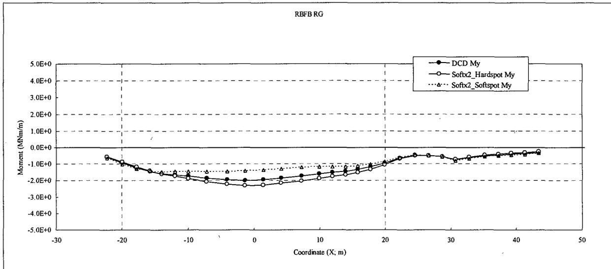
Figure 3.8-93 (23)-d Comparison of Sectional Moments (RG, Soft x2)
