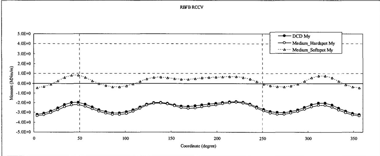
Figure 3.8-93 (18)-b Comparison of Sectional Moments (RCCV bottom, Medium)
