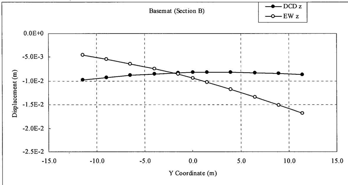
Figure 3.8-93 (11)-a Comparison of Settlement (CB, E-W direction)
