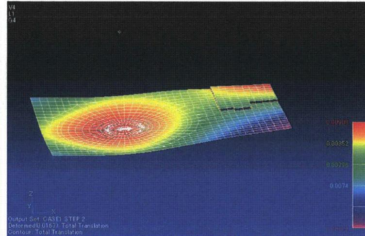
Figure 3.8-93(5) -a Deformation of basemat (CaseA - Step 1) Figure 3.8-93(5) -b Deformation of basemat (CaseA - Step 2)
