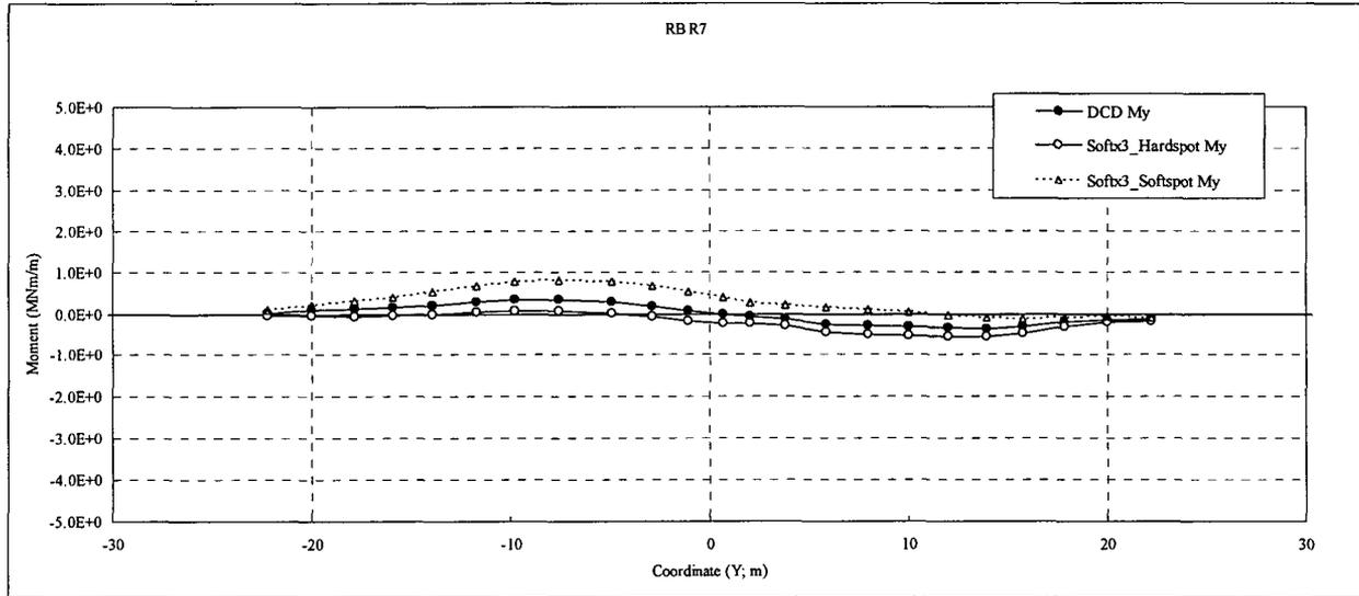
Figure 3.8-93 (20)-c Comparison of Sectional Moments (R7, Soft x3)
