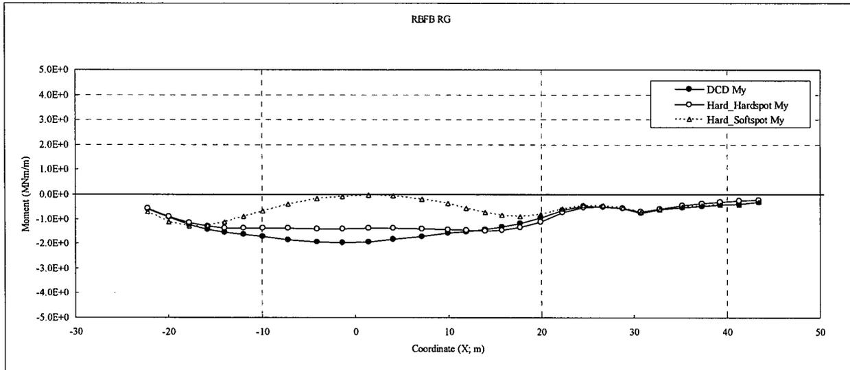
Figure 3.8-93 (23)-a Comparison of Sectional Moments (RG, Hard)
