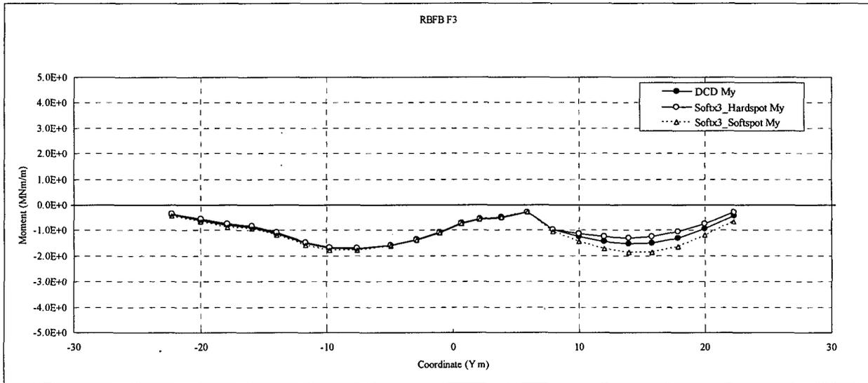
Figure 3.8-93 (21)-c Comparison of Sectional Moments (F3, Soft x3)
