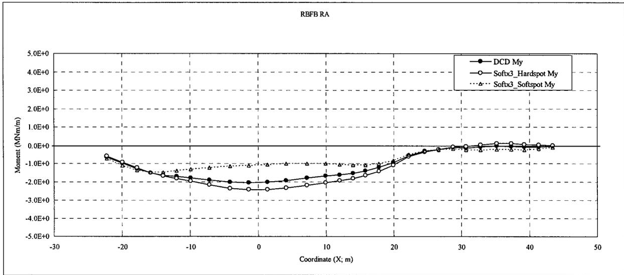
Figure 3.8-93 (22)-c Comparison of Sectional Moments (RA, Soft x3)
