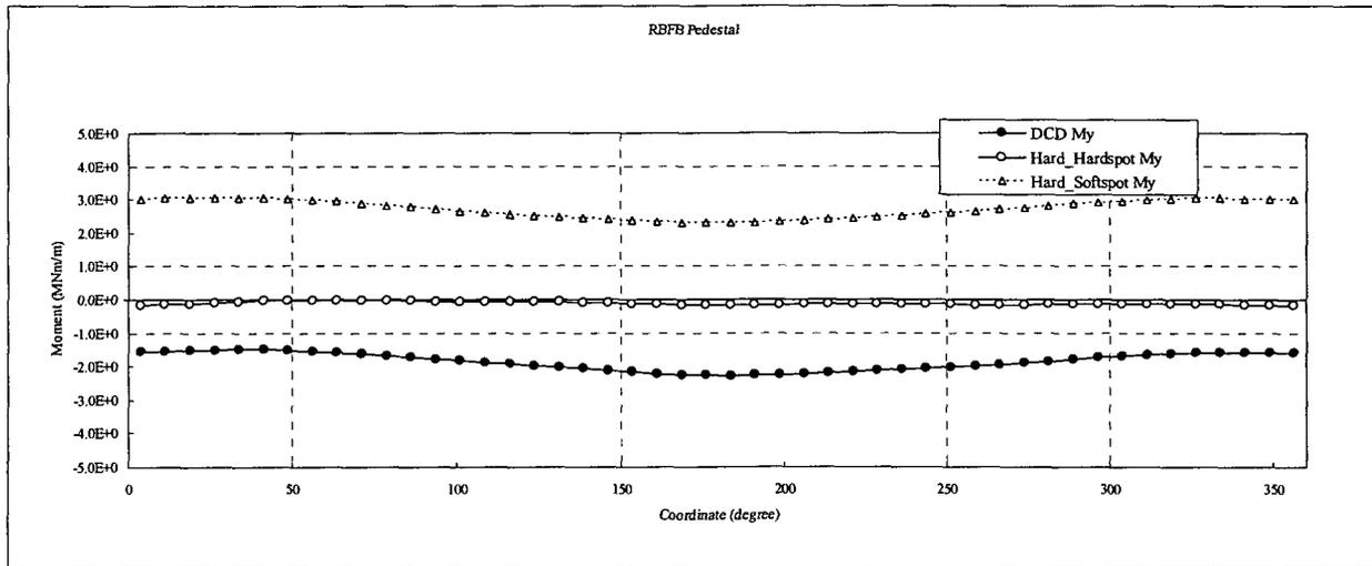
Figure 3.8-93 (17)-a Comparison of Sectional Moments (Pedestal, Hard)
