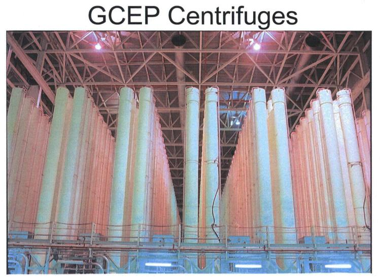
USEC's American Centrifuge is based on the U.S. Department of Energy's original centrifuges (pictured here), which operated in the 1980s at the Piketon facility.
