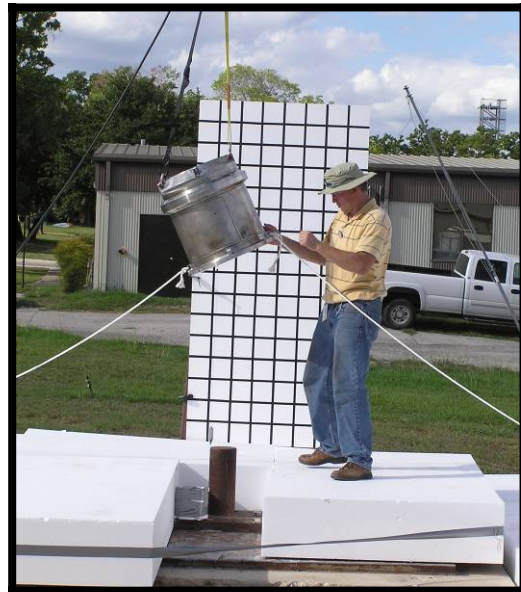
Photograph 4 – Test 1D HAC Bottom End Oblique Puncture Drop Set-up
