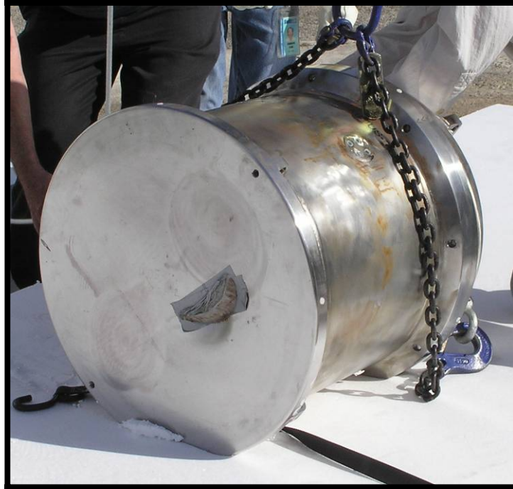
Photograph 17 – Test 1D Overpack Post-Drop Condition (View 1)
