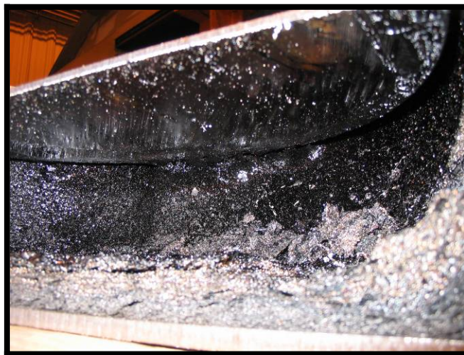
Photograph 45 – Test 2C Post-Test Overpack Lid Foam Condition (View 3)
