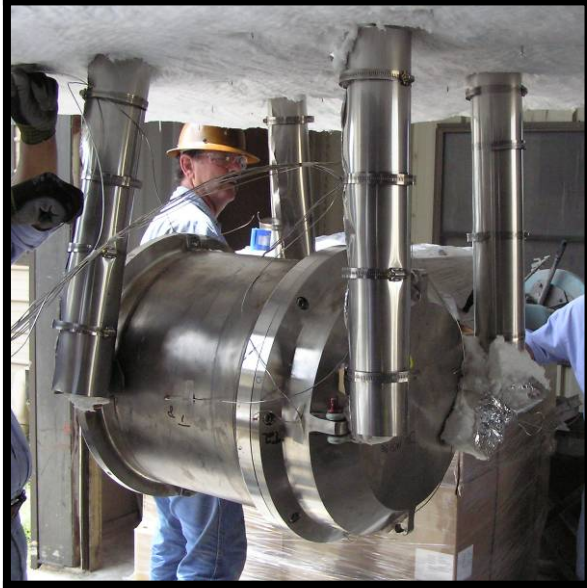
Photograph 7 – Test 2C HAC Thermal Set-up Outside Furnace
