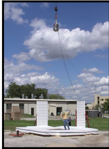
Photograph 2 – Test 1B HAC Top End Drop Set-up
