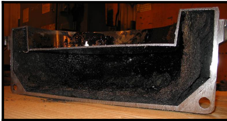
Photograph 44 – Test 2C Post-Test Overpack Lid Foam Condition (View 2)
