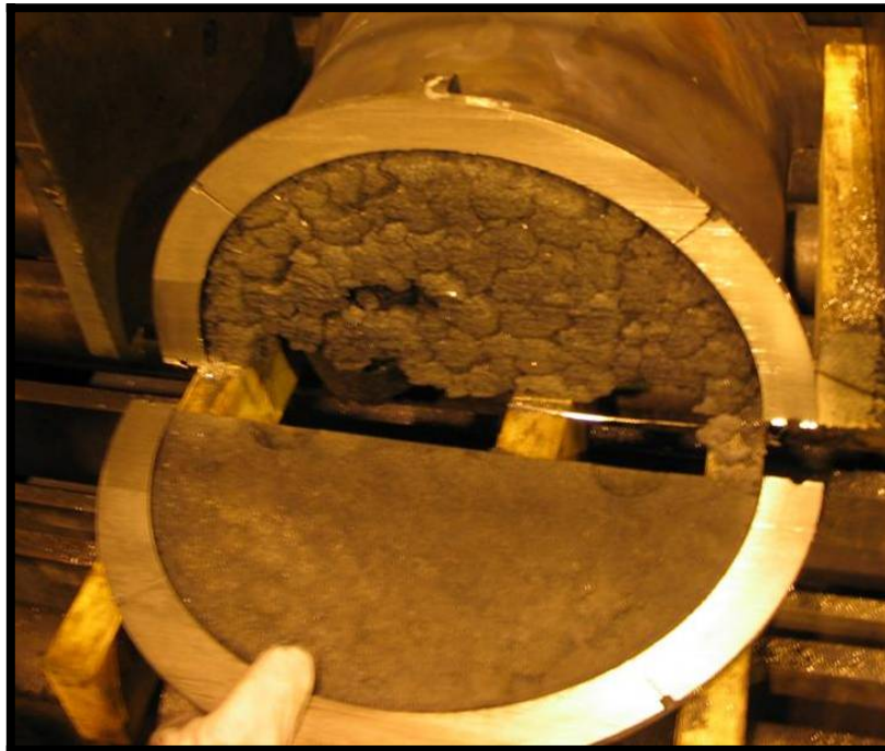
Photograph 40 – Test 2C Post-Test Overpack Base Foam Condition (View 2)
