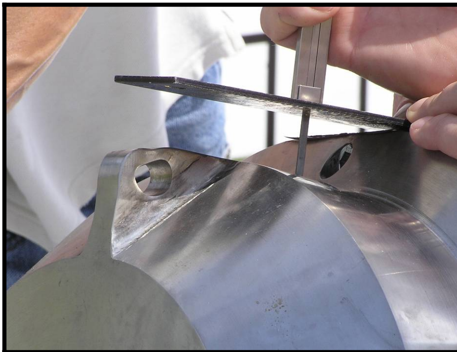
Photograph 20 – Test 2A Post-Drop Condition (View 2)
