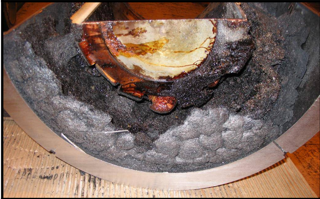
Photograph 41 – Test 2C Post-Test Overpack Base Foam Condition (View 3)
