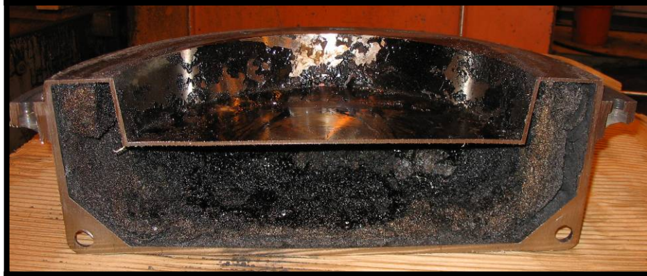
Photograph 43 – Test 2C Post-Test Overpack Lid Foam Condition (View 1)
