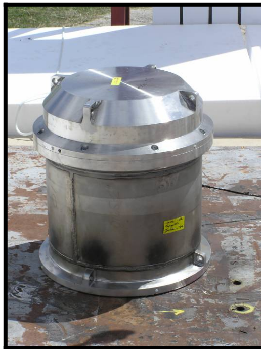
Photograph 12 – Test 1A Post-Drop Condition (View 2)
