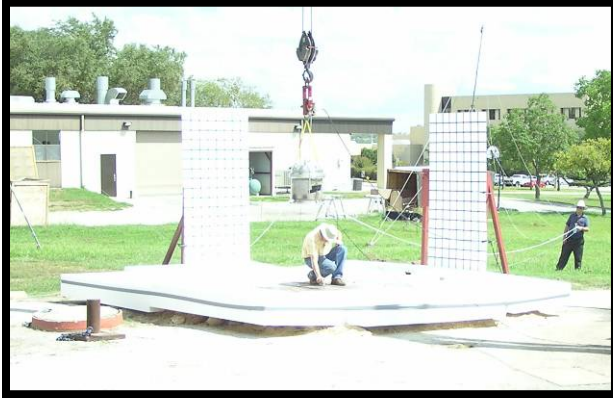
Photograph 1 – Test 1A NCT Bottom End Drop Set-up
