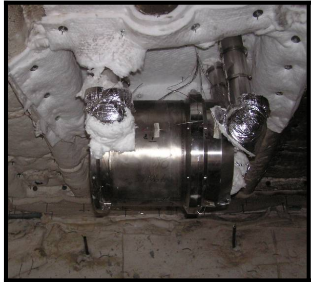
Photograph 8 – Test 2C HAC Thermal Set-up Inside Furnace
