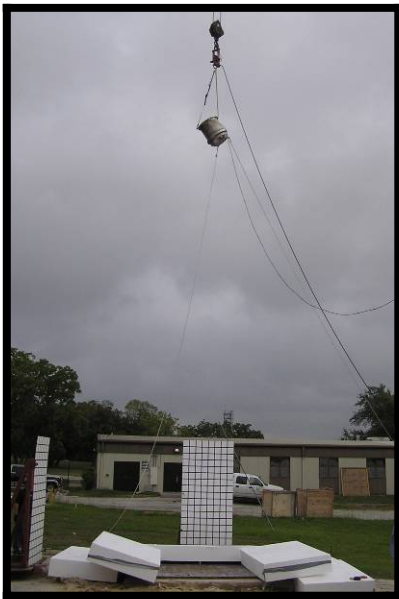
Photograph 3 – Test 1C HAC CG-Over-Top Corner Drop Set-up
