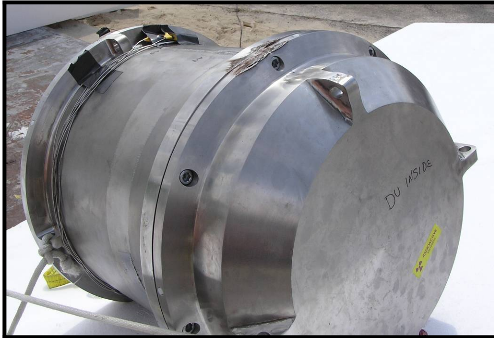
Photograph 19 – Test 2A Post-Drop Condition (View 1)
