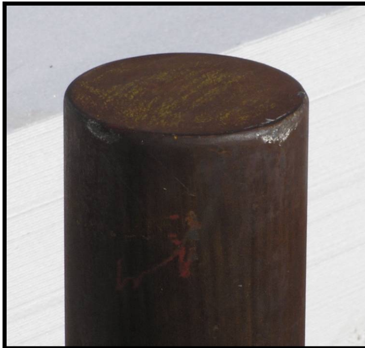
Photograph 18 – Test 1D Puncture Pin Post-Drop Condition (View 2)
