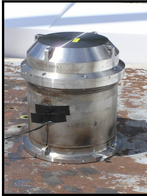
Photograph 11 – Test 1A Post-Drop Condition (View 1)
