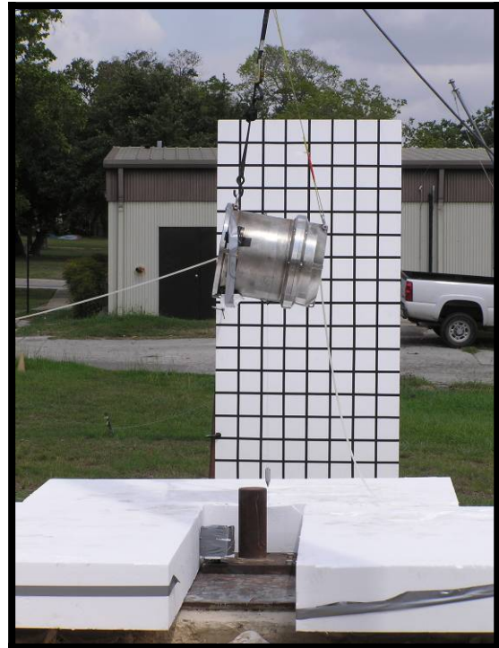
Photograph 6 – Test 2B HAC Side Puncture Drop Set-up
