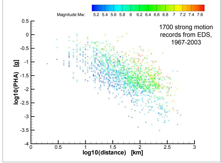
Peak Horizontal Acceleration (PHA) is measured in multiples of "g"
