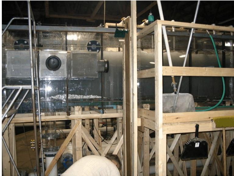
**Figure 5** RMI Debris Accumulation Underneath the Strainer Module
