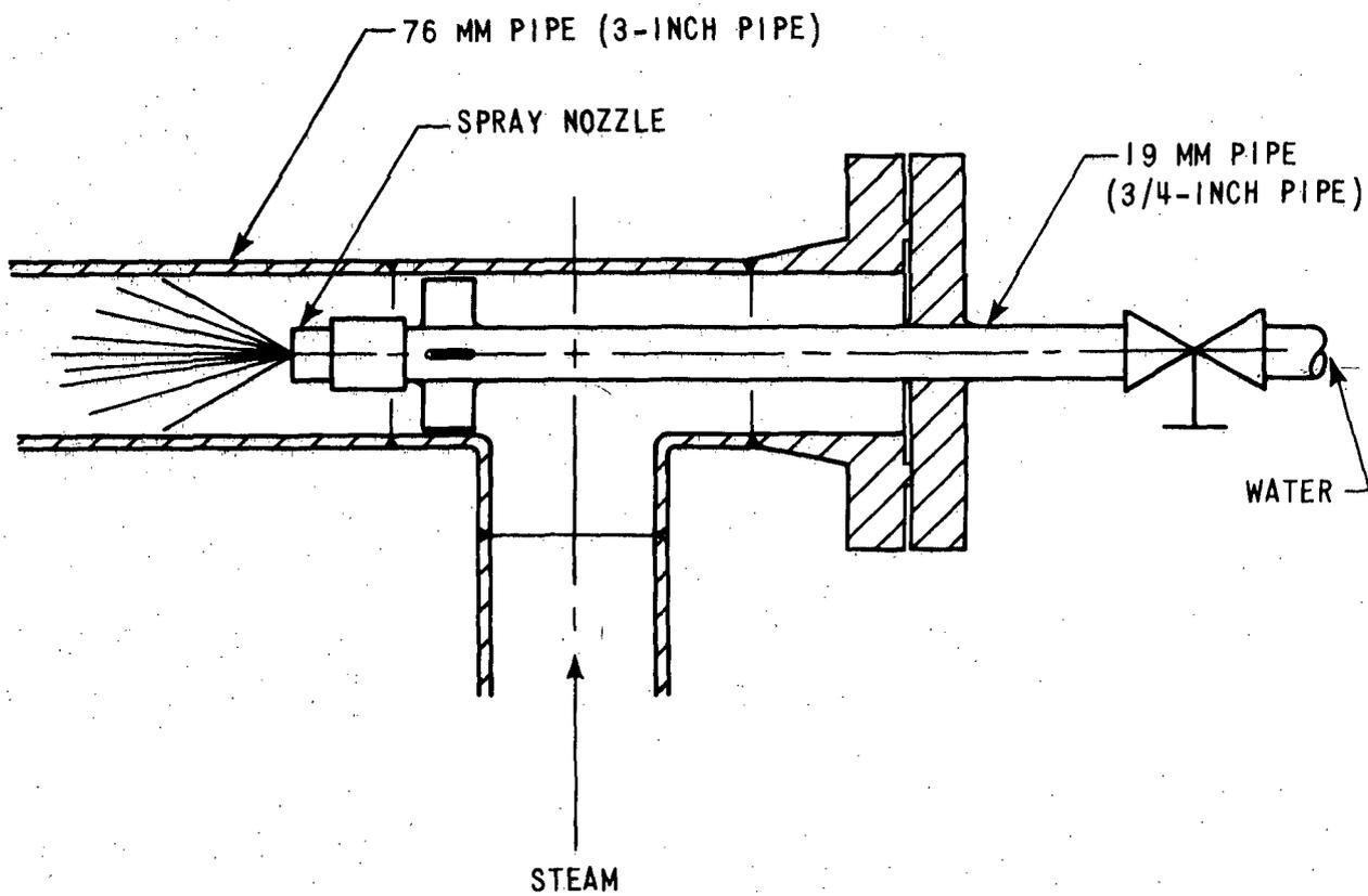
Figure 5-2. Diagram of the Steam-Water Mixer Section
