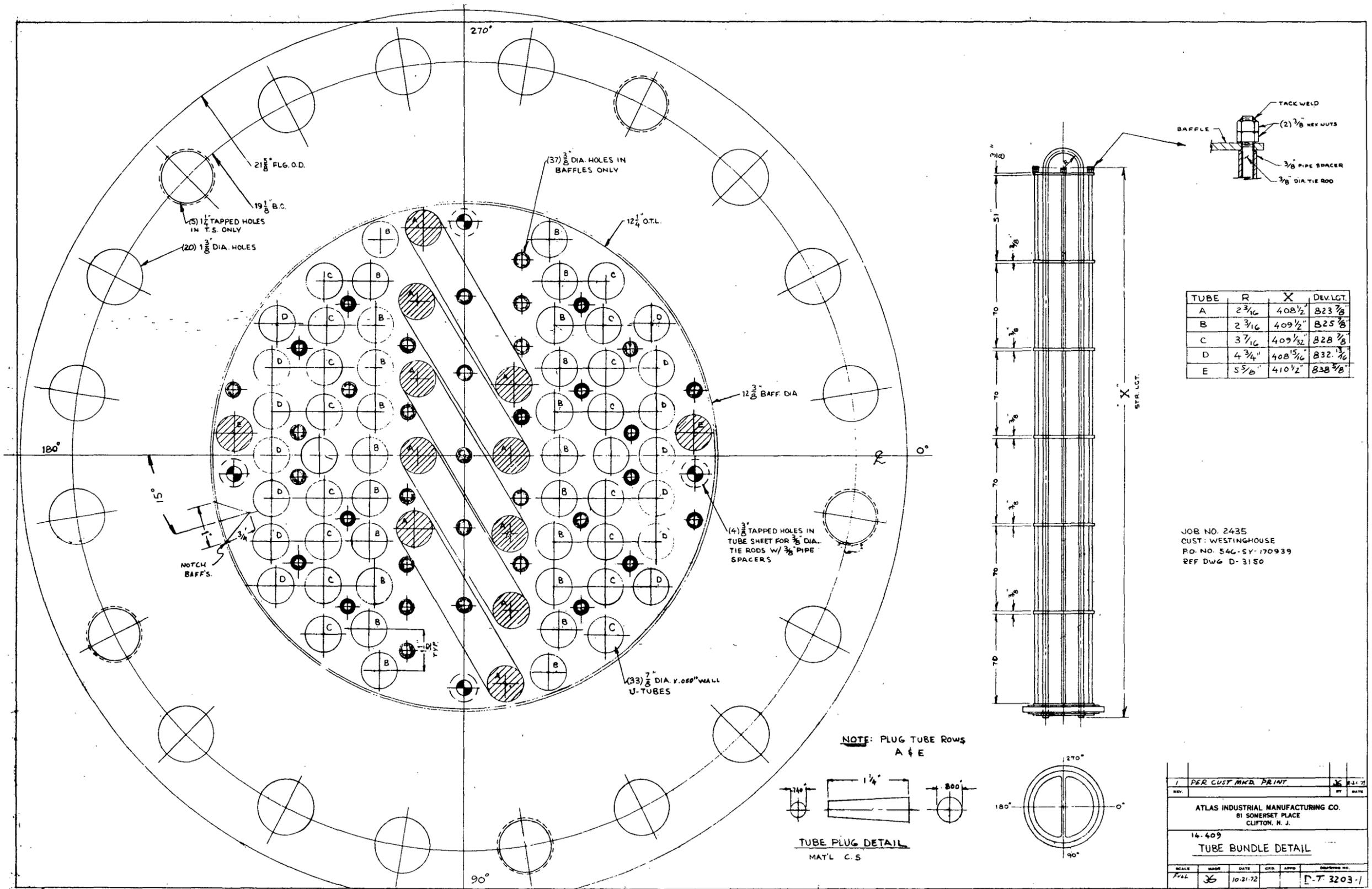
Figure 5-3. Details of the Construction of Separate Effects Test Steam Generator (Sheet 1 of 2)
