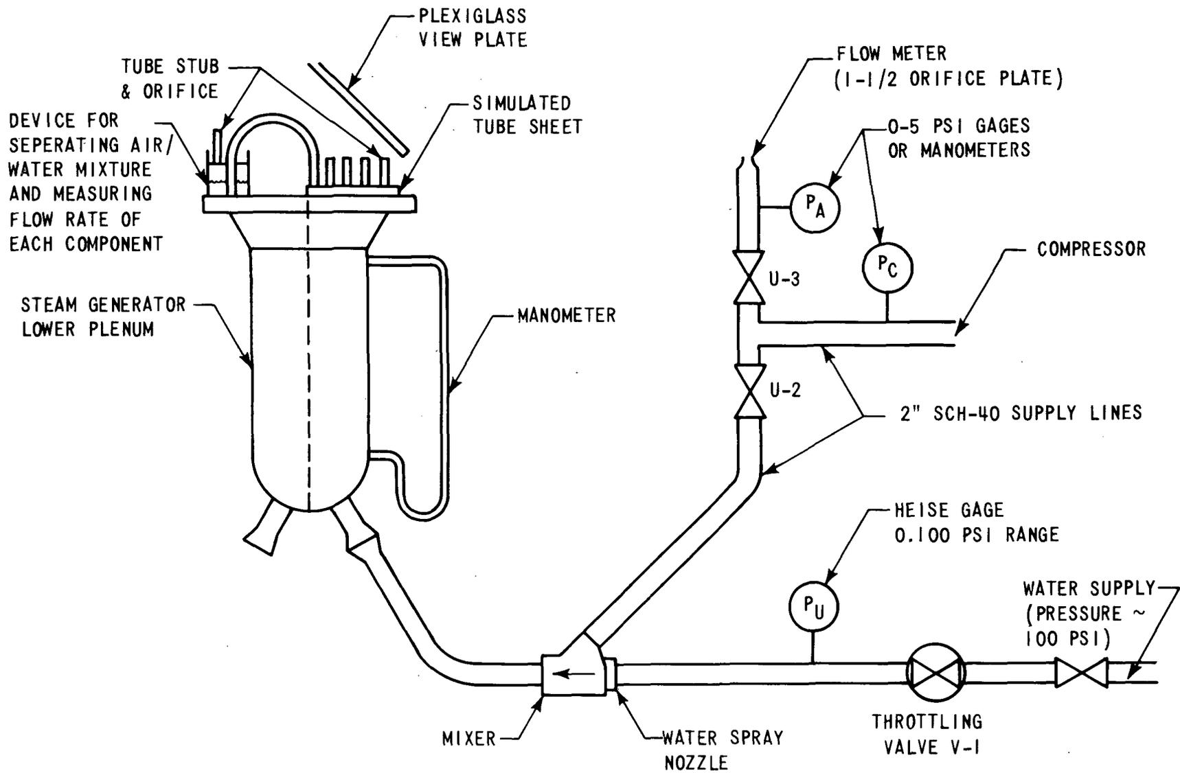
Figure C-2. Loop Schematic Diagram for the Plenum Air/Water Test
