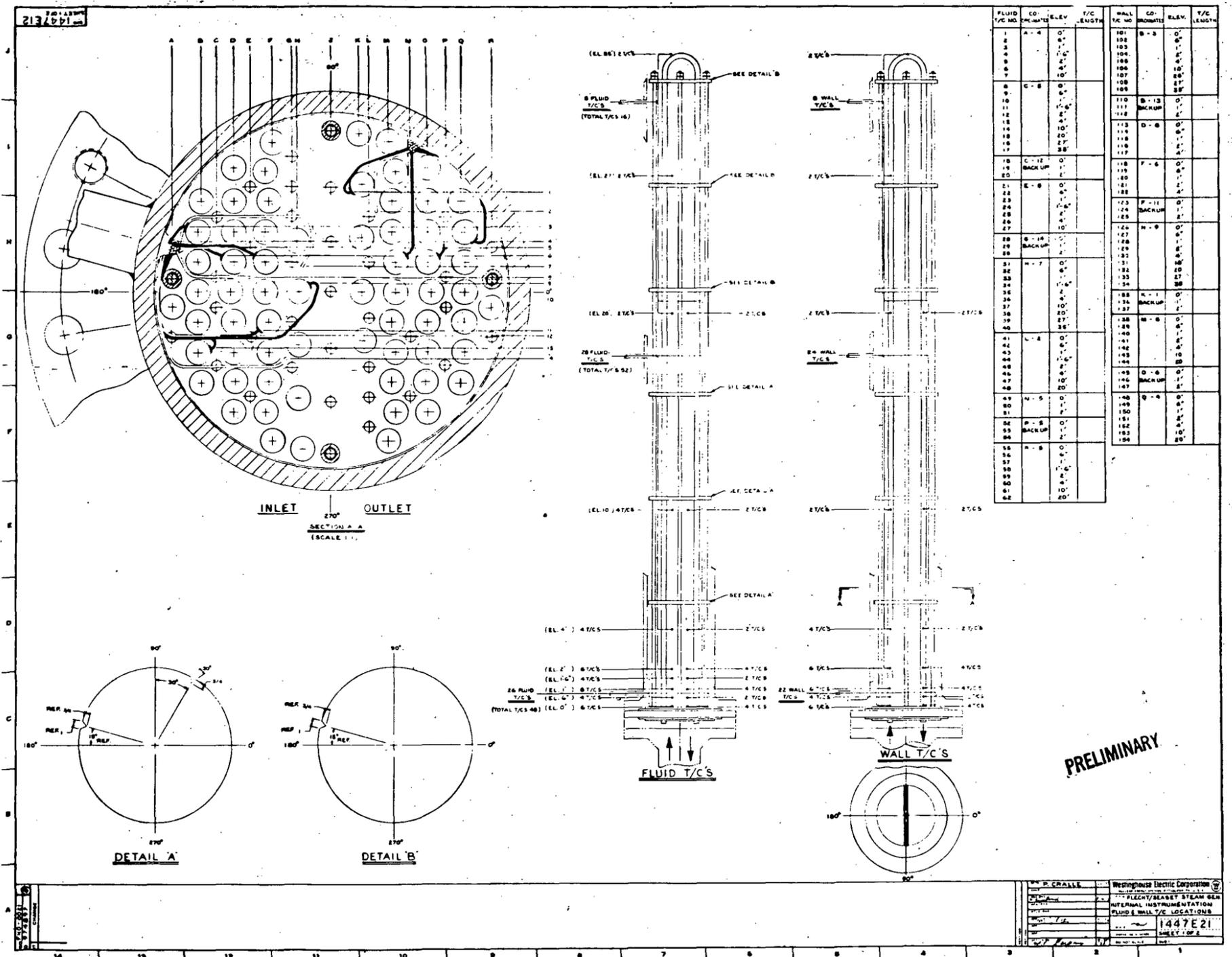
Figure 6-2. FLECHT SEASET Steam Generator Separate Effects Test Instrumentation Locations (Sheet 1 of 2)
