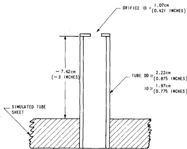
Figure C-1. Orifice Simulation of Steam Generator Tube Friction
