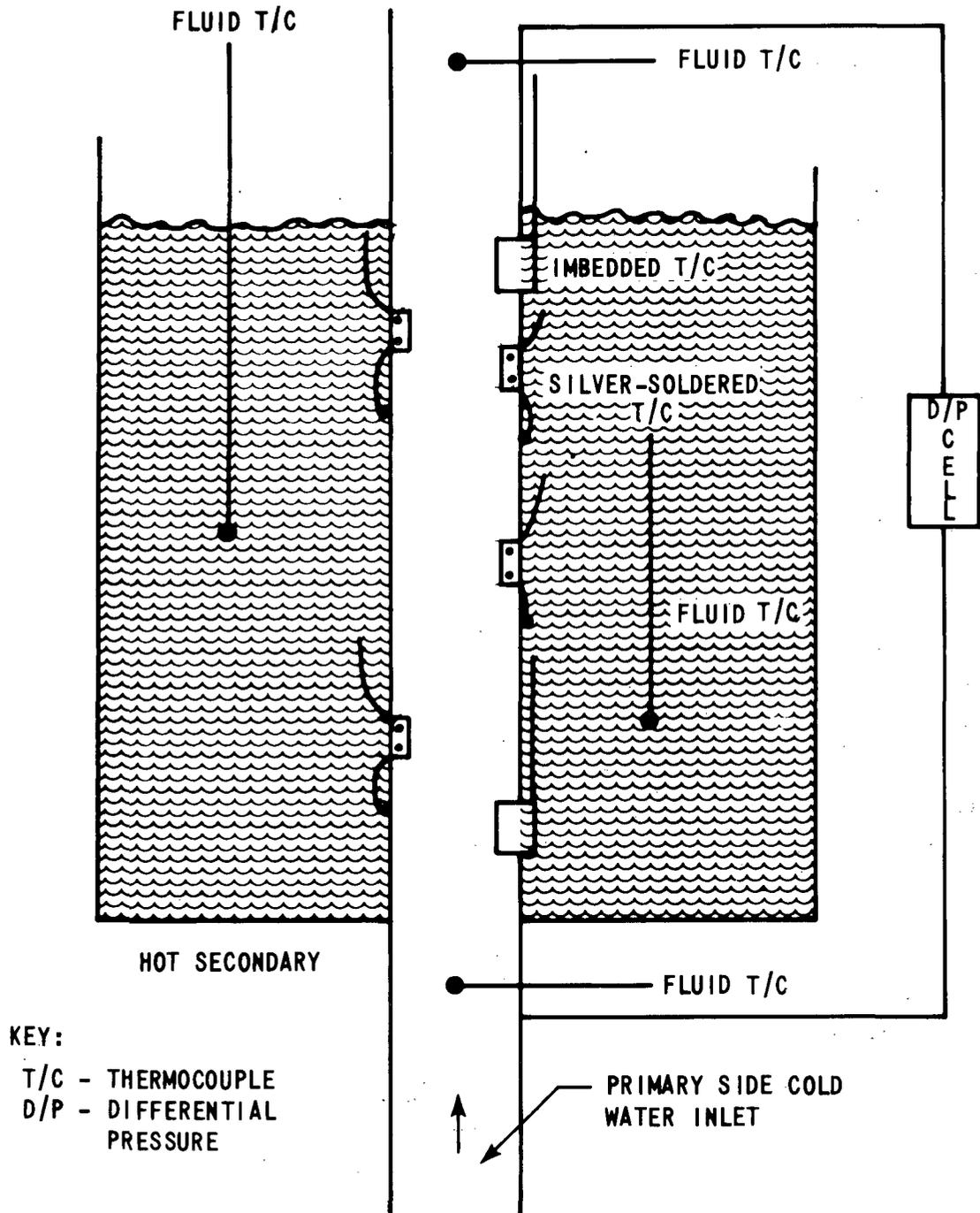
Figure 6-5. Schematic Diagram of the Thermocouple Bench Test
