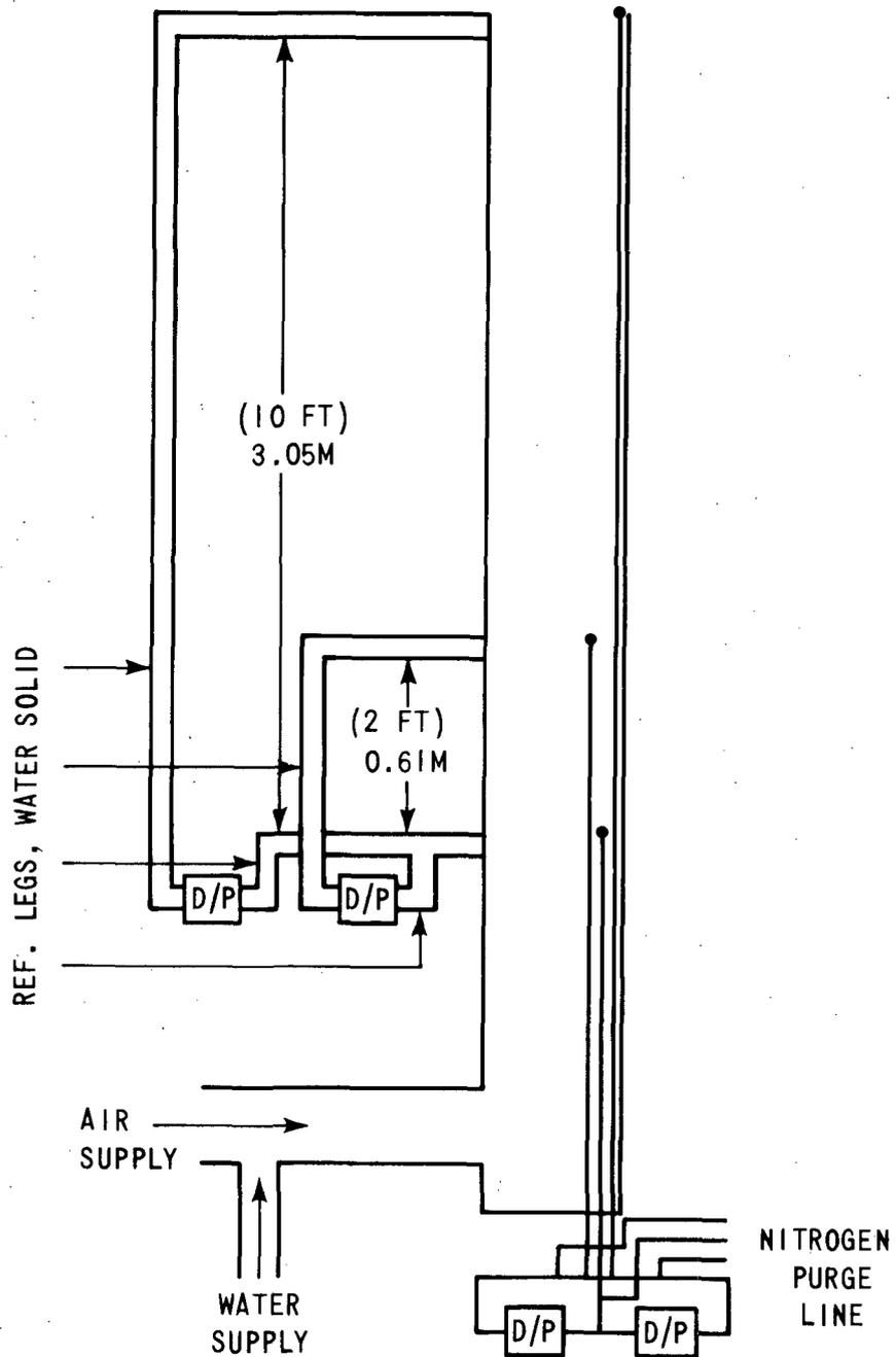
Figure 6-6. FLECHT SEASET Steam Generator Tube Pressure Probe Bench Test With Transparent Tube
