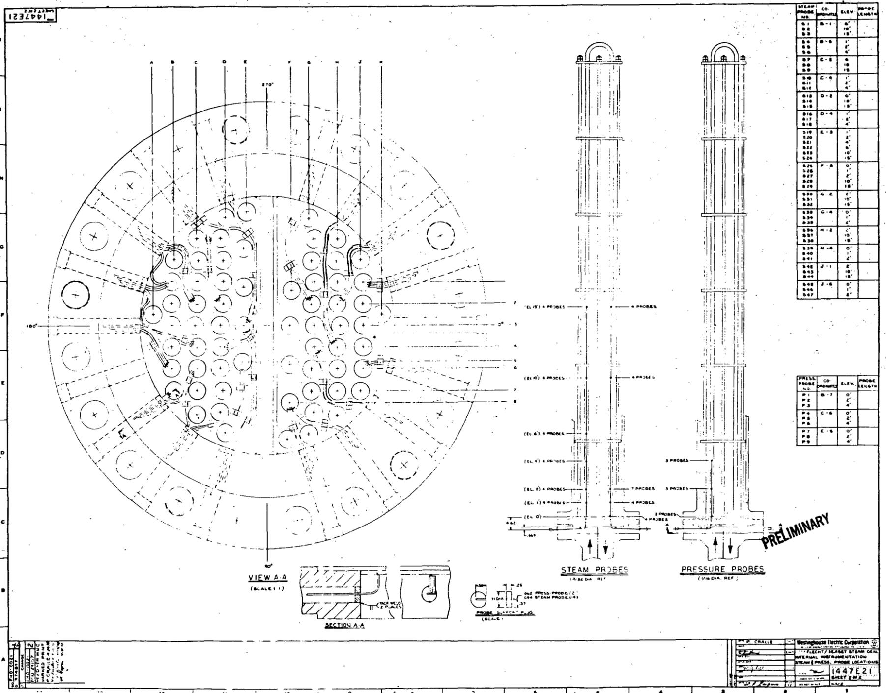
Figure 6-3. FLECHT SEASET Steam Generator Separate Effects Test Instrumentation Locations (Sheet 2 of 2)
