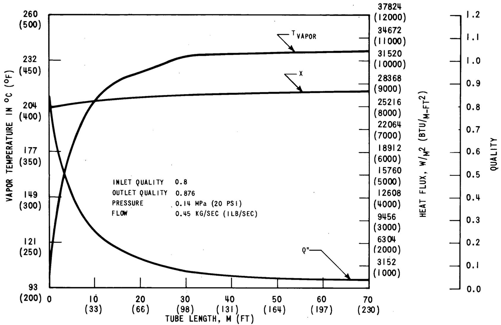
Figure 6-4. Primary Side Tube Steam Temperature, Quality, and Heat Flux Versus Tube Length
