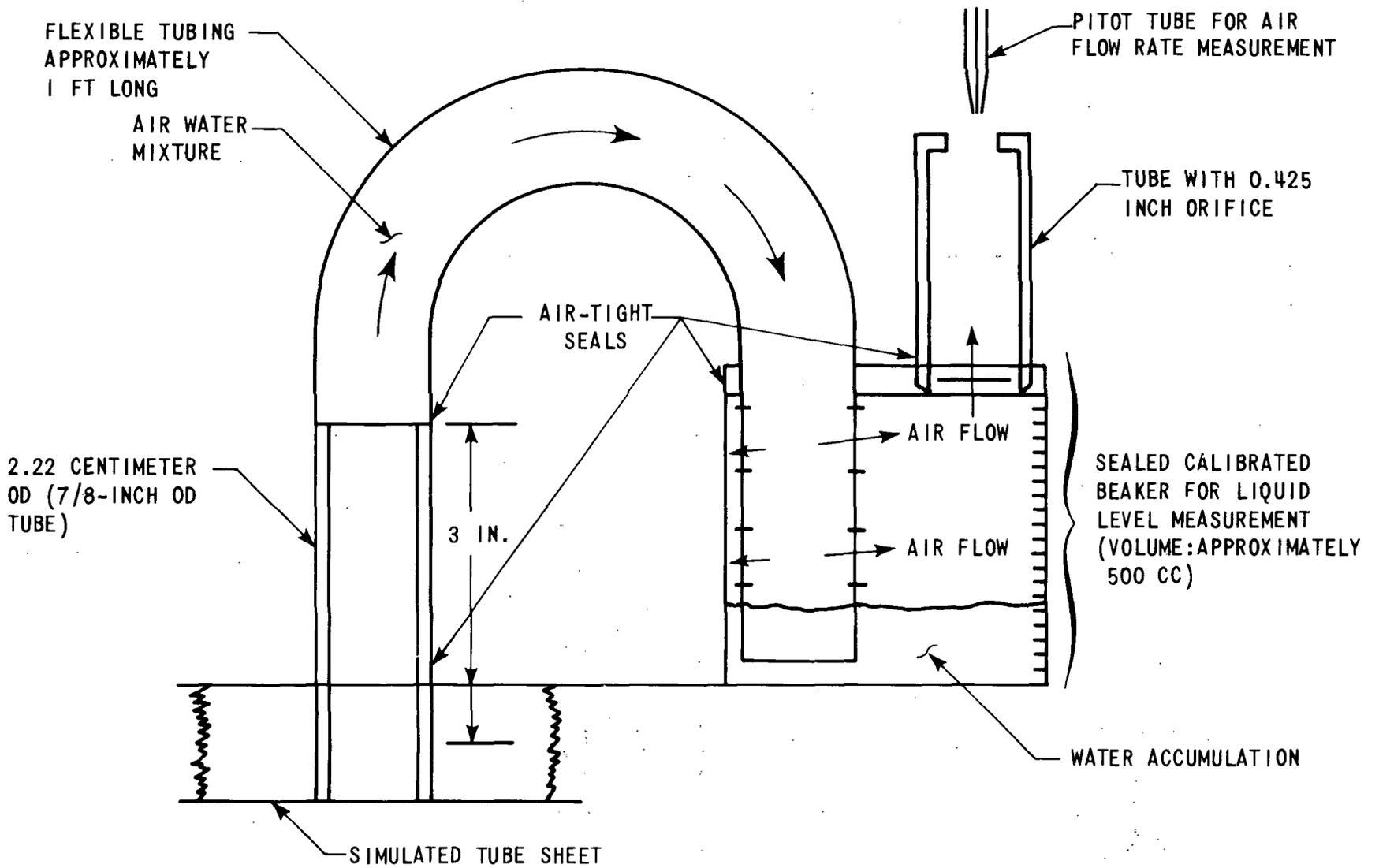
Figure C-3. Steam Generator Tube Air and Water Flow Rate Measurement
