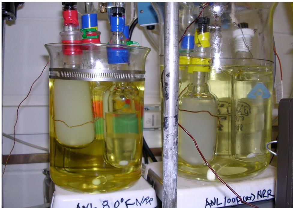
Figure 7. Small-scale test system configuration for tests conducted at 80 F (left) and 100 F (right).
