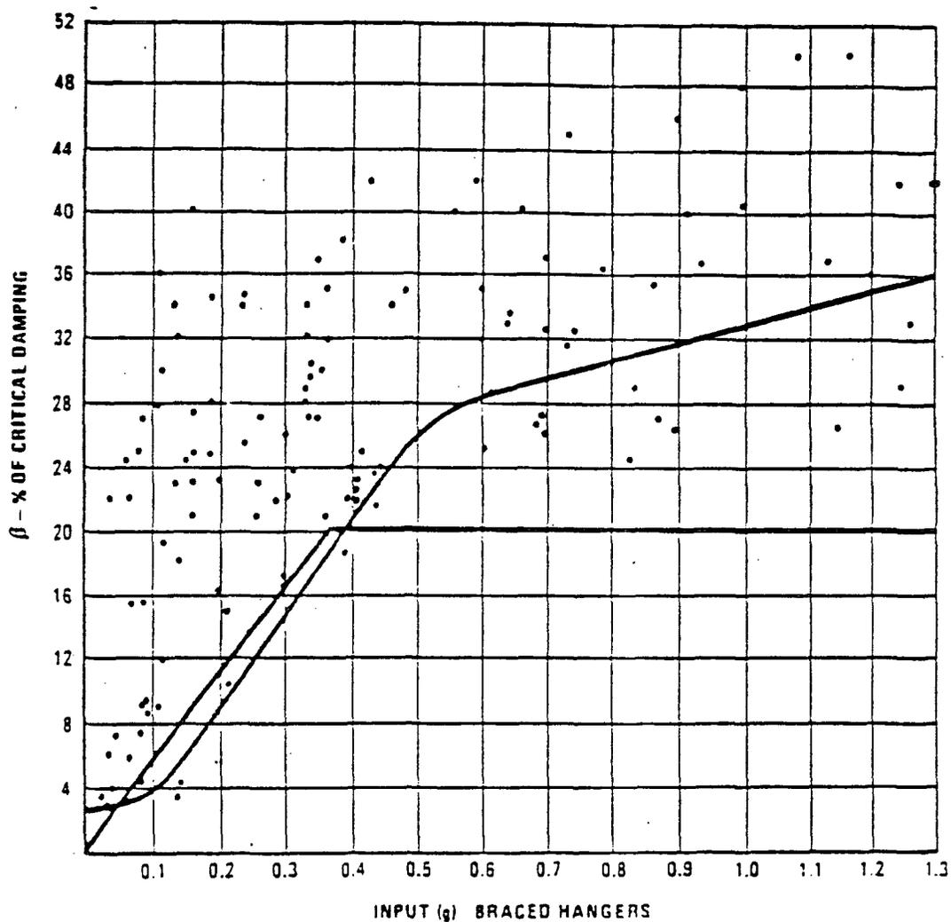
Figure 8. Damping vs. Input Level for Braced Hanger Systems<sup>4</sup>
