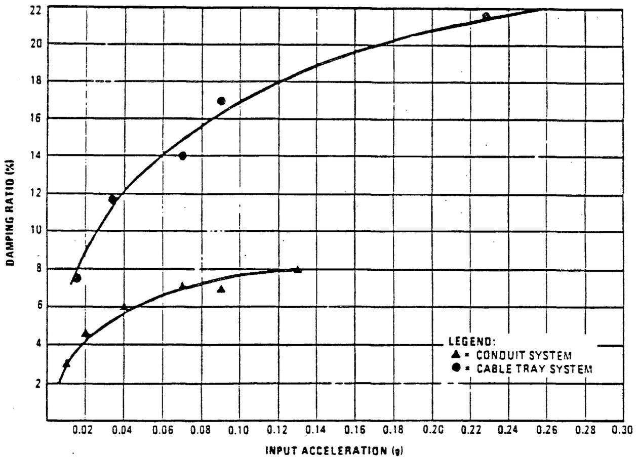
Figure 7. Typical Conduit and Tray Test Results<sup>4</sup>
