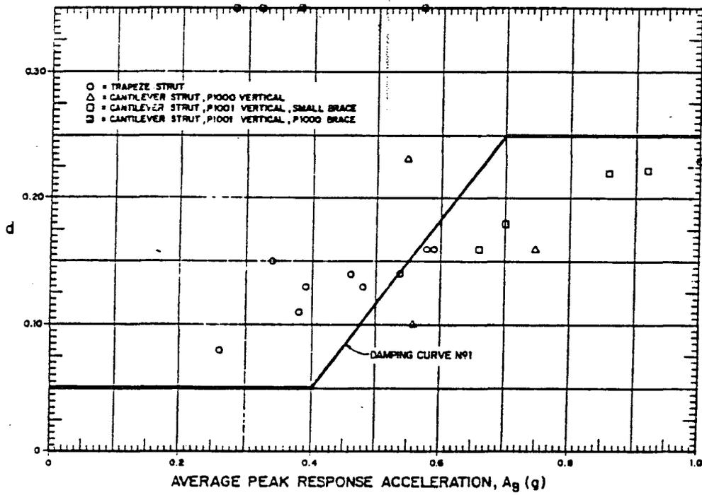
Figure 12. Damping Values for Strut-Supported Systems. 15
