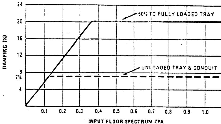
Figure 9. Recommended Damping for the Design of Raceway Systems<sup>4</sup>
