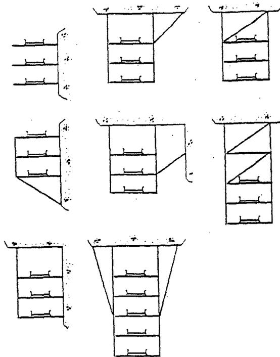
Figure 3. Cable Tray Support Systems<sup>2</sup>
