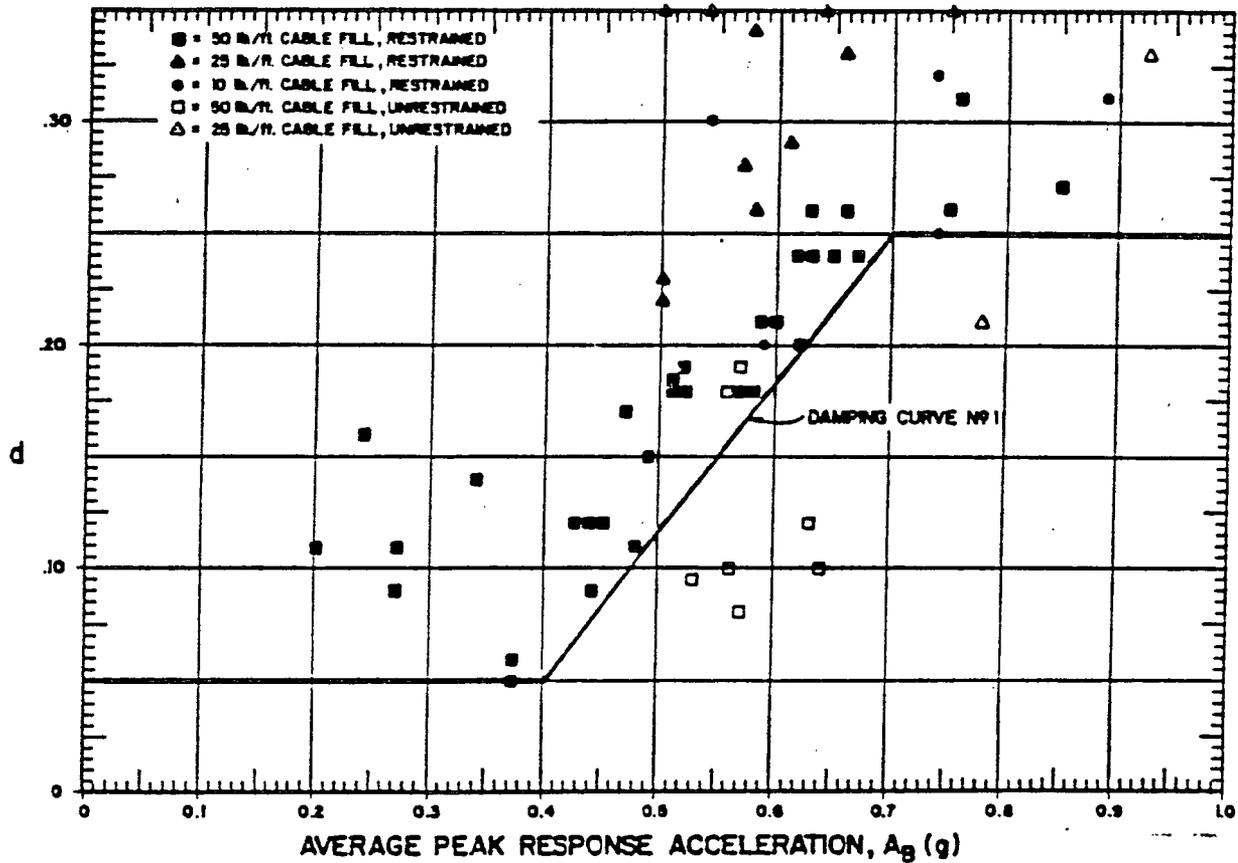
Figure 10. Damping values for Rod-Supported Cable Tray Systems<sup>15</sup>
