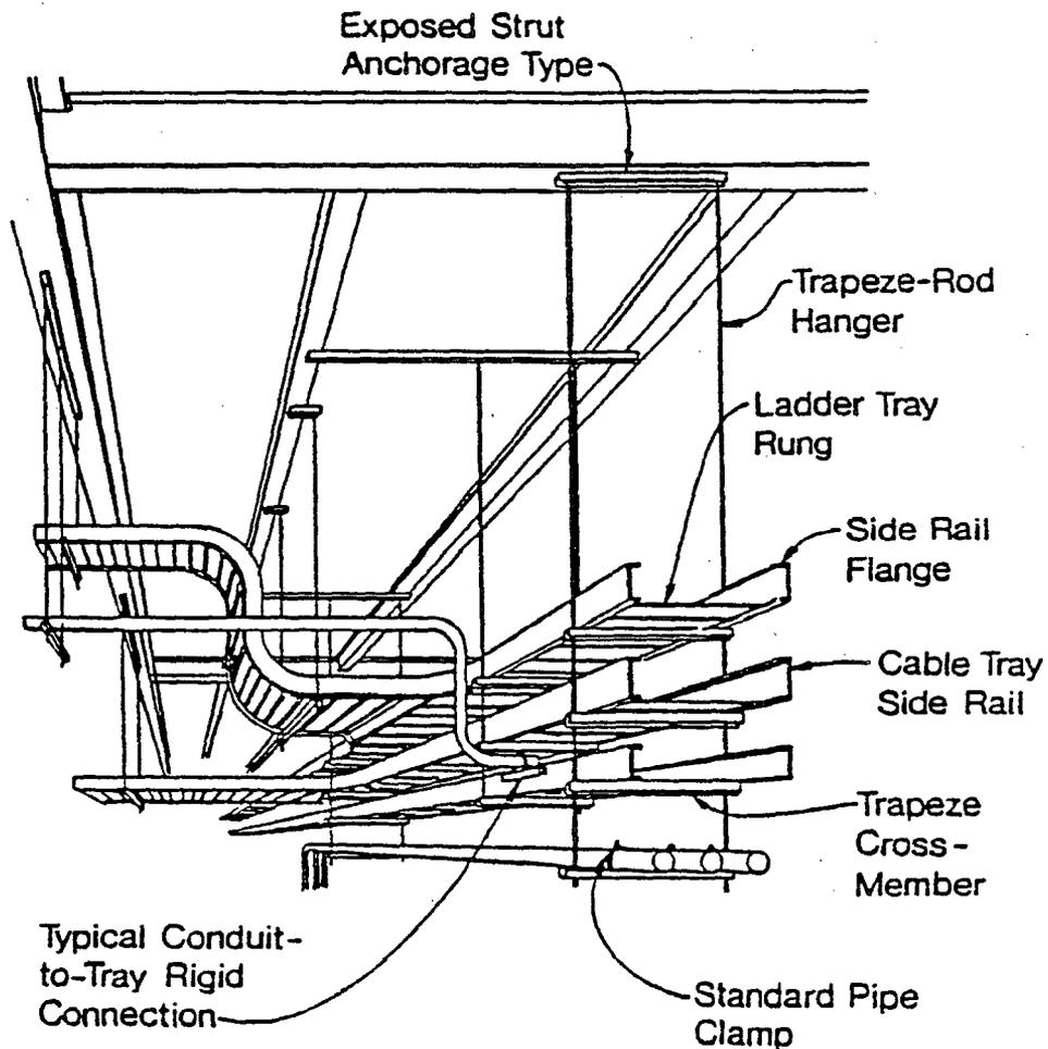
Figure 1. Cable Tray System<sup>1</sup>
