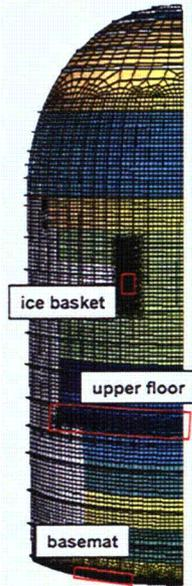
Figure 5.9: Locations of Corrosion Postulated for the PWR
