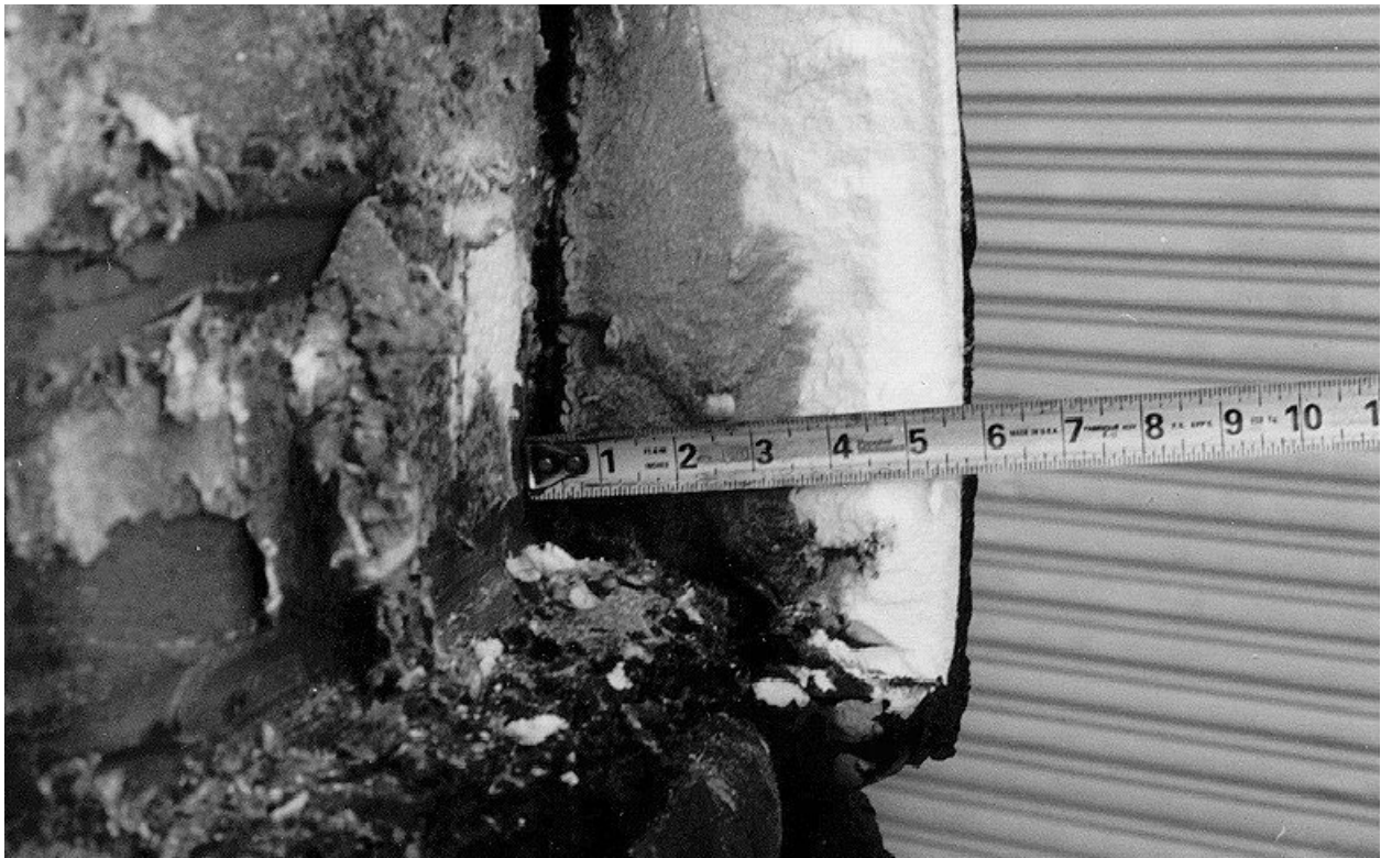
Figure 2.10.3-83 – CTU; Residual Foam in OCA Lid Side; Remote from Test Damage
