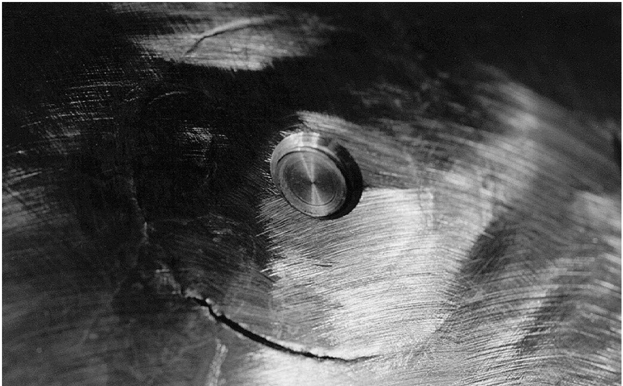
Figure 2.10.3-95 – CTU; Close-up View of Cracked OCV Vent Port Coupling Inner Weld
