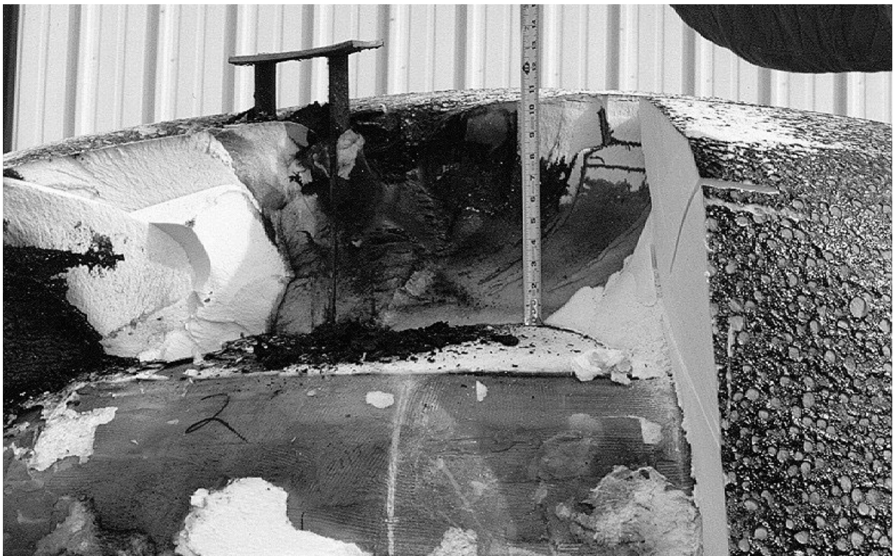
Figure 2.10.3-44 – ETU; Residual Foam in OCA Lid Top (~11")
