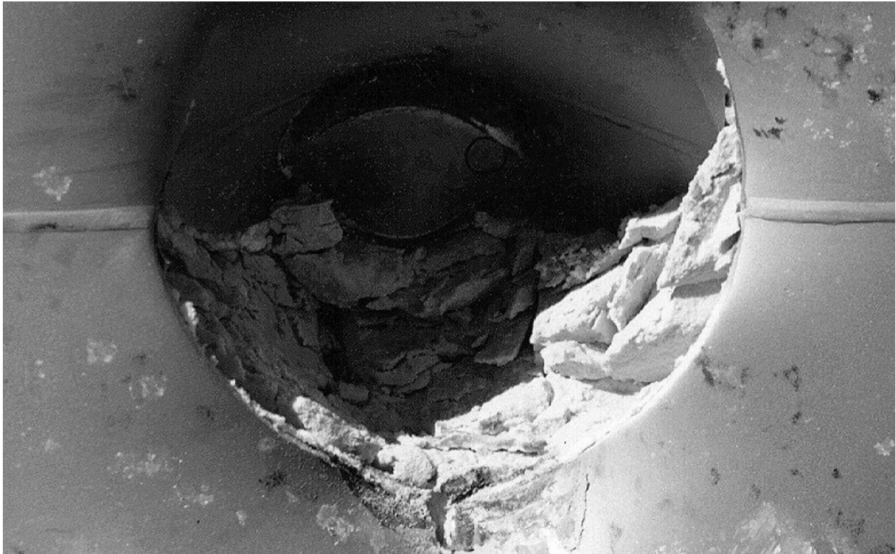
Figure 2.10.3-24 – ETU Puncture Drop Test 7; ~10½" High × ~11½" Wide Hole
