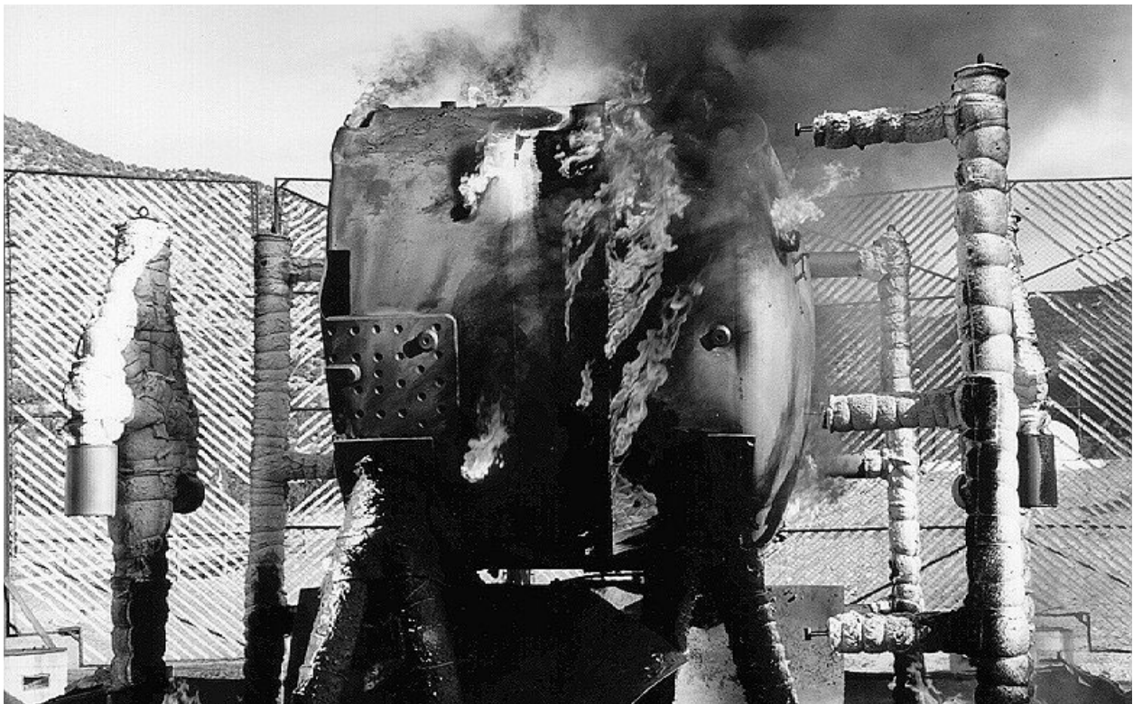
Figure 2.10.3-38 – ETU Fire Test 11; View ~17 Minutes after End of Fire
