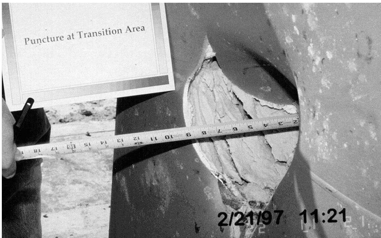
Figure 2.10.3-25 – ETU Puncture Drop Test 7; Radial Penetration ~8" Deep
