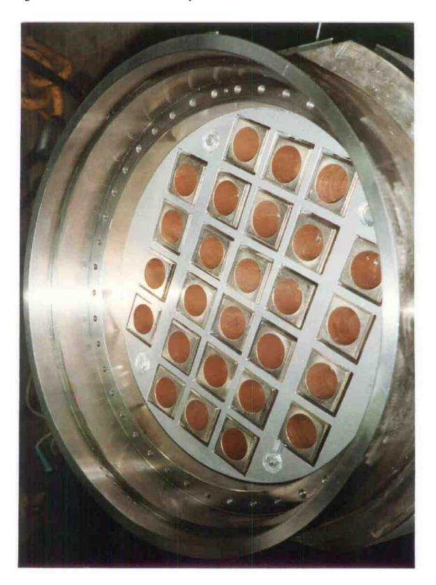
Figure 2.10.6-4 Top End Drop - Cask Penetration into Impact Limiter
