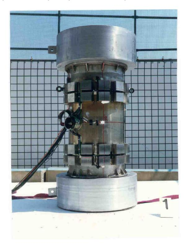
Figure 2.10.6-5 Side Drop - Detail of Shield Block Impact Near Bottom End
