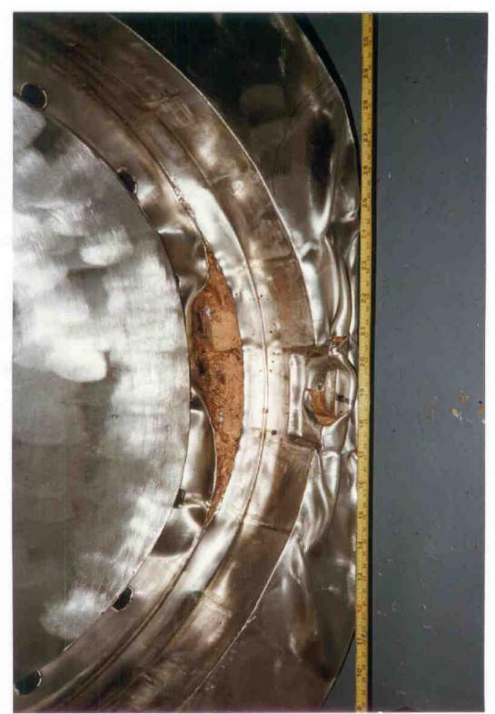
Figure 2.10.6-28 Bottom Oblique Drop Test (Test No. 1 of Phase 4) - Impact Limiter Deformations
