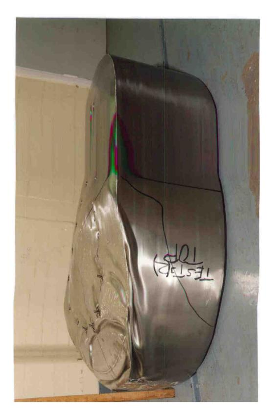
Figure 2.10.6-10 Cask Midpoint Pin Puncture - Outer Shell Deformation
