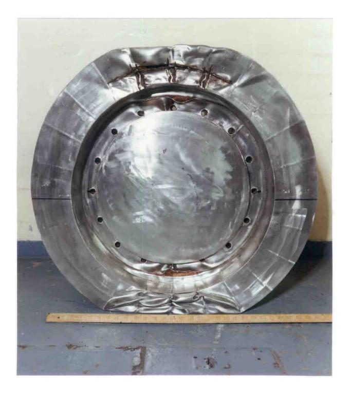
Figure 2.10.6-36 Side Drop Test (Test No. 2 of Phase 4) - Impact Limiter Deformations
