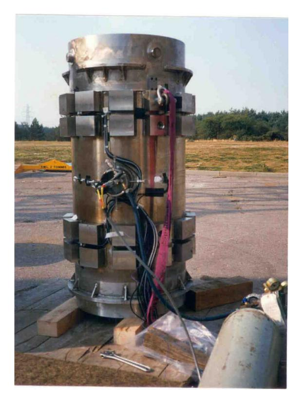
Figure 2.10.6-2 Assembly of Cask - Inner Lid Fitted
