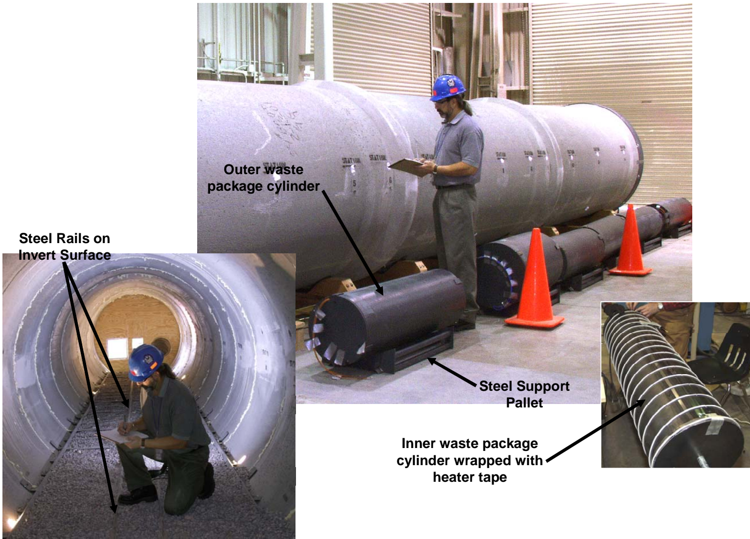
Figure 7.4.1-3. Photographs of the 25% Scale Test Components
