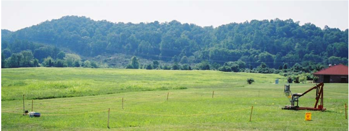
Figure 4 . An ISFSI Background Radiation Emulator is placed 40 feet from ISOCS detector to increase the local background by a factor of two.
