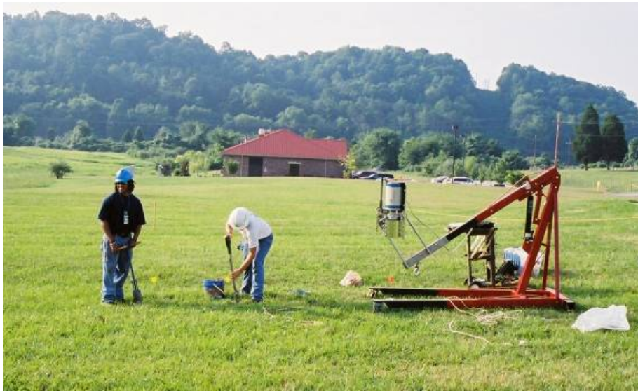
Figure 3. Engineers prepare the site for measurement. The ISOCS detector is mounted at 1 meter from the surface of the ground. Soil is exhumed for the placement of test sources.
