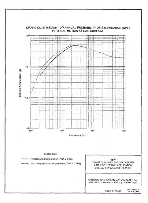
Figure 2-Horizontal and vertical response spectra for the Safe Shutdown Earthquake at the ESP site
