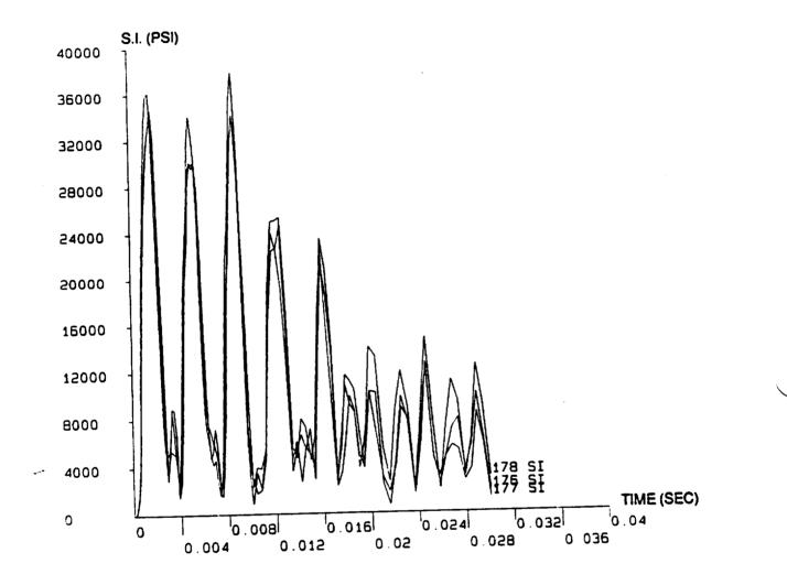
Spacer Disk 0° Orientation Side Drop Maximum Membrane S.I. vs. Time
