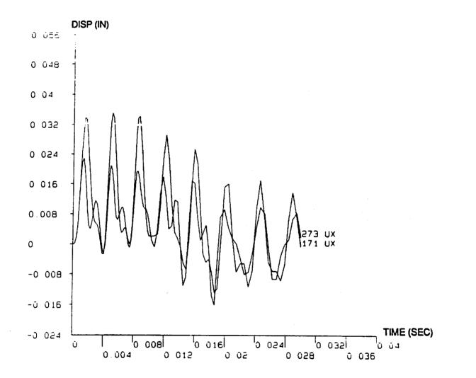
Spacer Disk 0° Orientation Side Drop Maximum Displacements vs. Time
