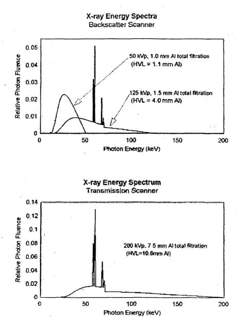
**Fig. 3.3.** Approximate photon energy spectra of the x-ray beams from two backscatter systems (top) and from a transmission system (bottom).
