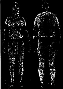
Fig. 3.1. Rapiscan's Secure 1000<sup>™</sup> backscatter system and sample images. Photographs courtesy of Rapiscan Security Products, Inc., Hawthorne, California.
