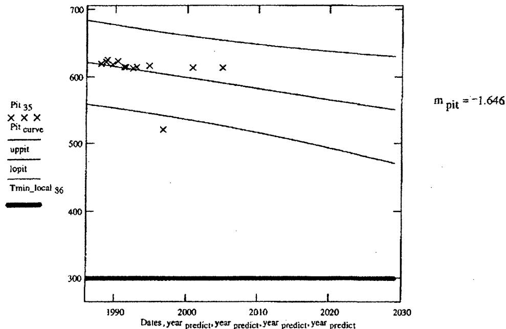
Therefore based on regression model the above curve shows that this pit will not corrode to below minimum required thickness by the plant end of life.
