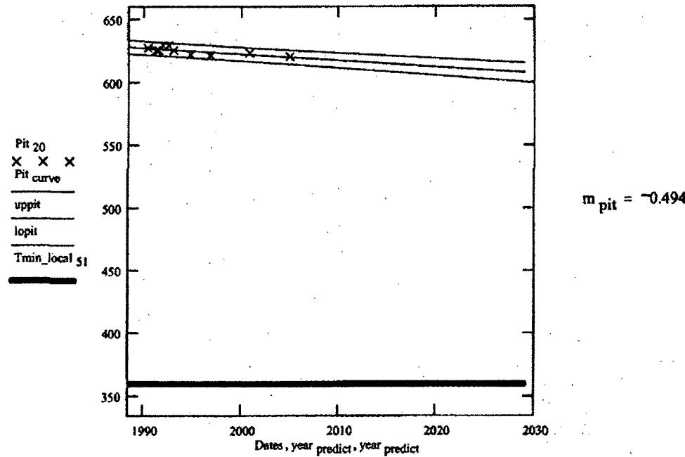
Therefore based on regression model the above curve shows that this pit will not corrode to below minimum required thickness by the plant end of life.
