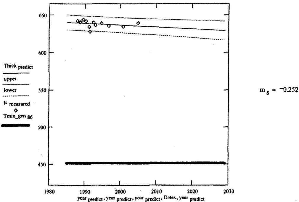
Therefore even though the regression model does not apply it still shows that the lower 95% confidence band will not corrode to below Drywell Vessel Minimum required thickness by the plant end of life.
