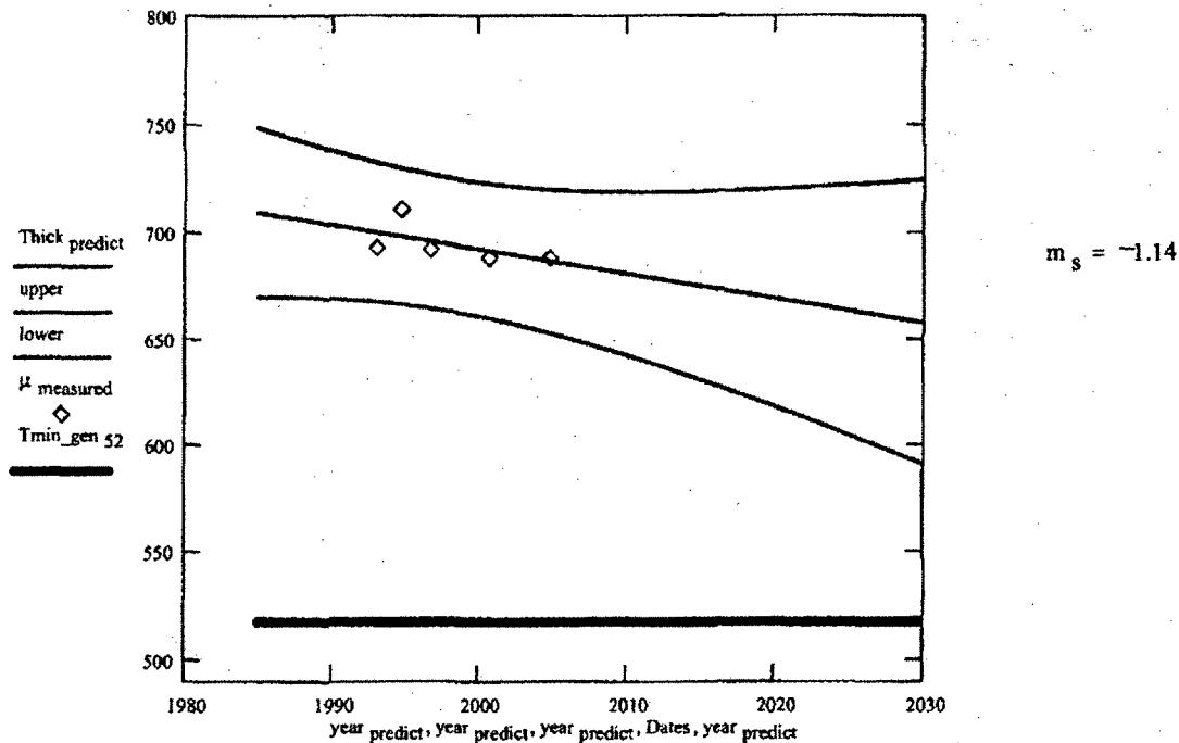
Therefore even though F-ratio does not support the regression model the above curve shows that even at the lower 95% confidence band this location will not corrode to below Drywell Vessel Minimum required thickness by the plant end of life.
