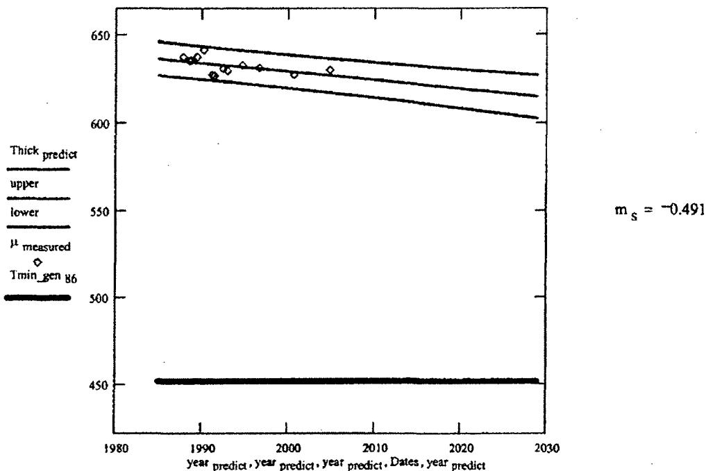
Therefore the regression model shows that even at the lower 95% confidence band this location will not corrode to below Drywell Vessel Minimum required thickness by the plant end of life.
