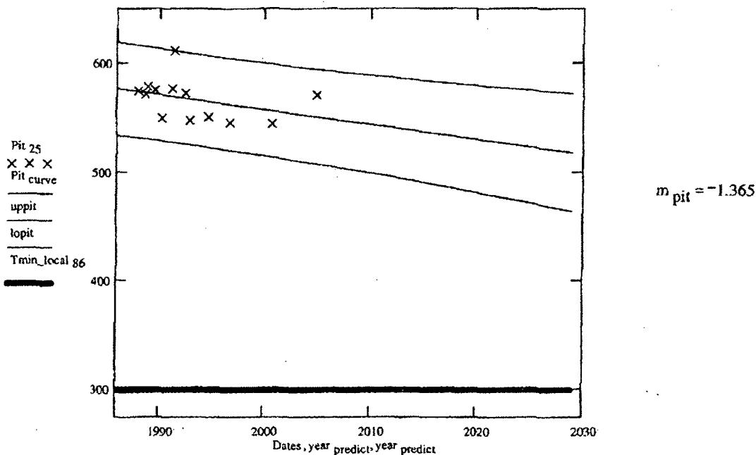
Therefore even though the regression model does not apply, it shows that this pit will not corrode to below minimum required thickness by the plant end of life.
