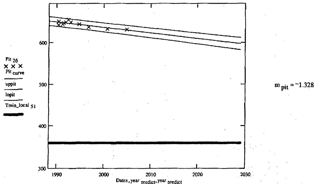
Therefore based on regression model the above curve shows that this pit will not corrode to below minimum required thickness by the plant end of life or life extension.
