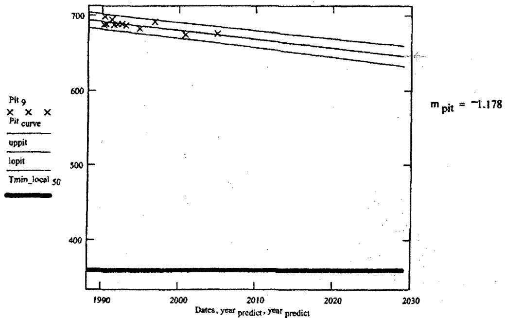
Therefore based on the regression model the above curve shows that this pit will not corrode to below minimum required thickness by the plant end of life or past plant life extension.
