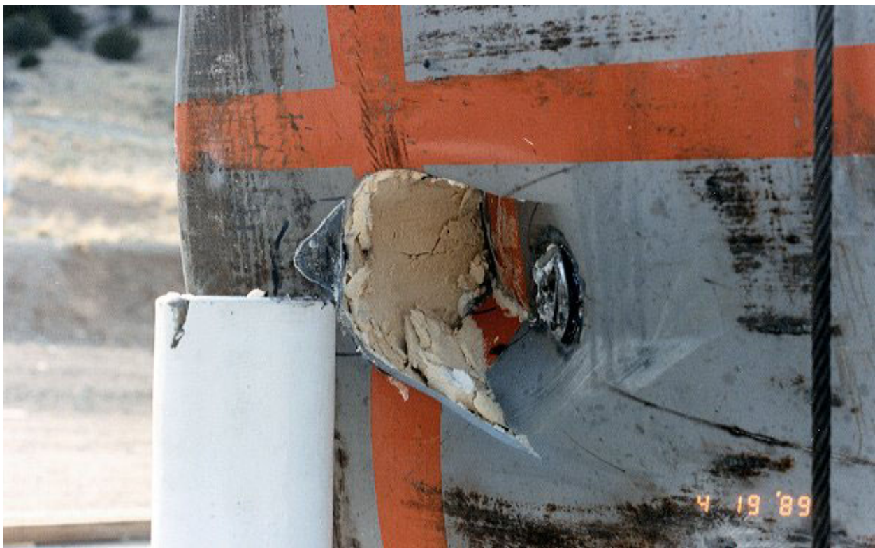
Figure 2.10.3-87 – CTU-3 Puncture Drop 4; Post-Drop Damage
