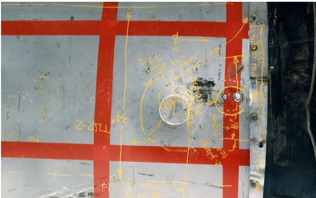
Figure 2.10.3-39 – CTU-1 Puncture Drop No. 6; Post-Drop Damage
