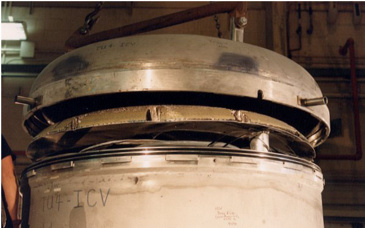
Figure 2.10.3-98 – CTU-3 Disassembly; ICV Lid Removal
