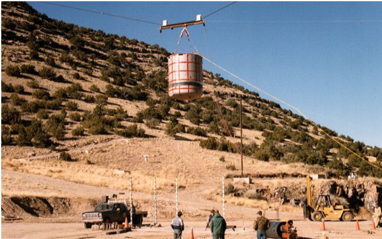
Figure 2.10.3-34 – CTU-1 Free Drop No. 4; Pre-Drop Positioning
