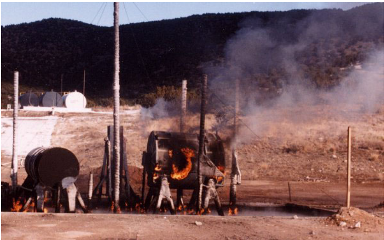
Figure 2.10.3-77 – CTU-2 Fire No. 9; Post-Fire Cool-Down
