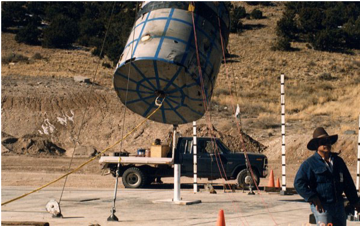
Figure 2.10.3-66 – CTU-2 Puncture Drop No. 5; Pre-Drop Positioning
