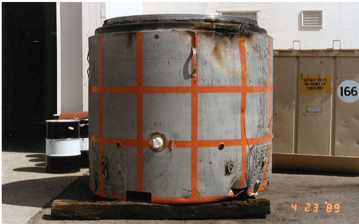
Figure 2.10.3-97 – CTU-3 Disassembly; OCA Body
