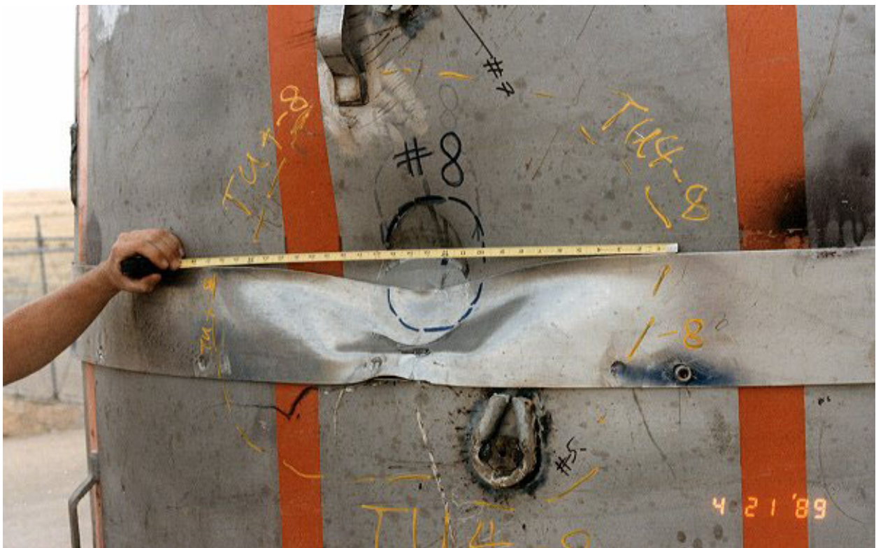
Figure 2.10.3-95 – CTU-3 Puncture Drop 8; Post-Drop Damage
