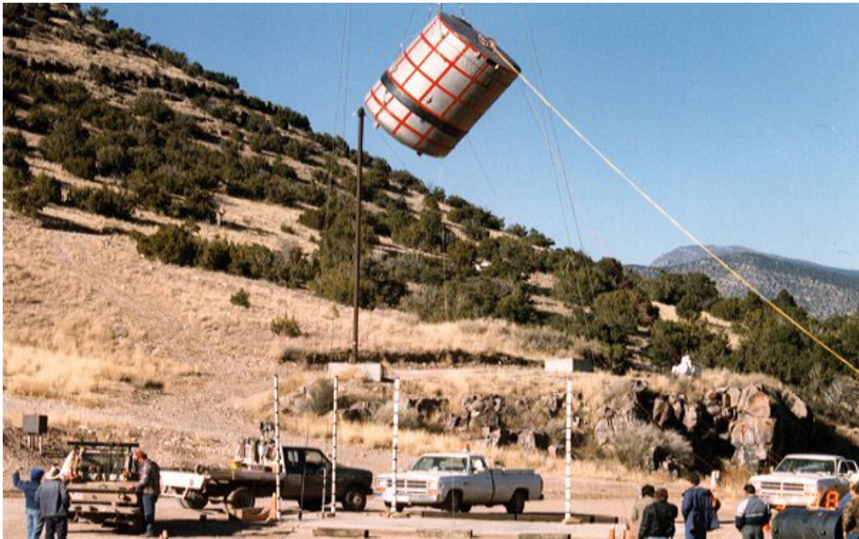
Figure 2.10.3-32 – CTU-1 Free Drop No. 3; Pre-Drop Positioning
