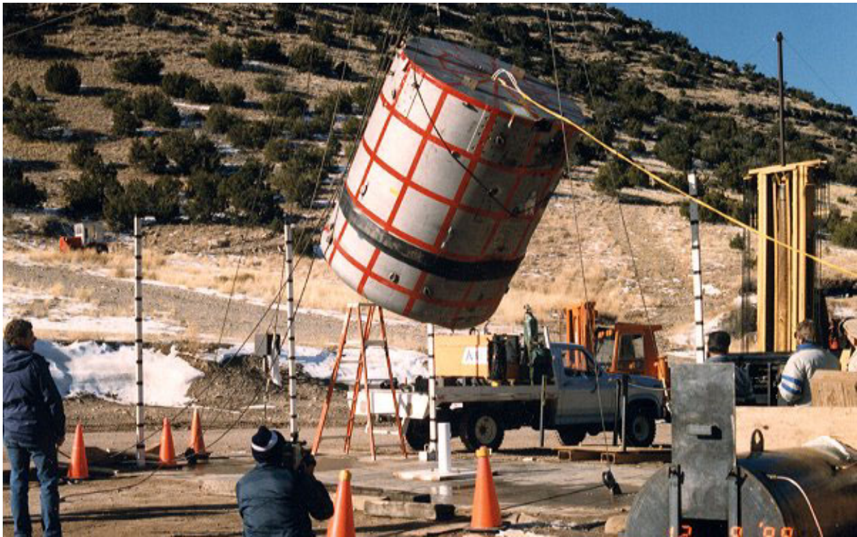
Figure 2.10.3-42 – CTU-1 Puncture Drop No. 8; Pre-Drop Positioning
