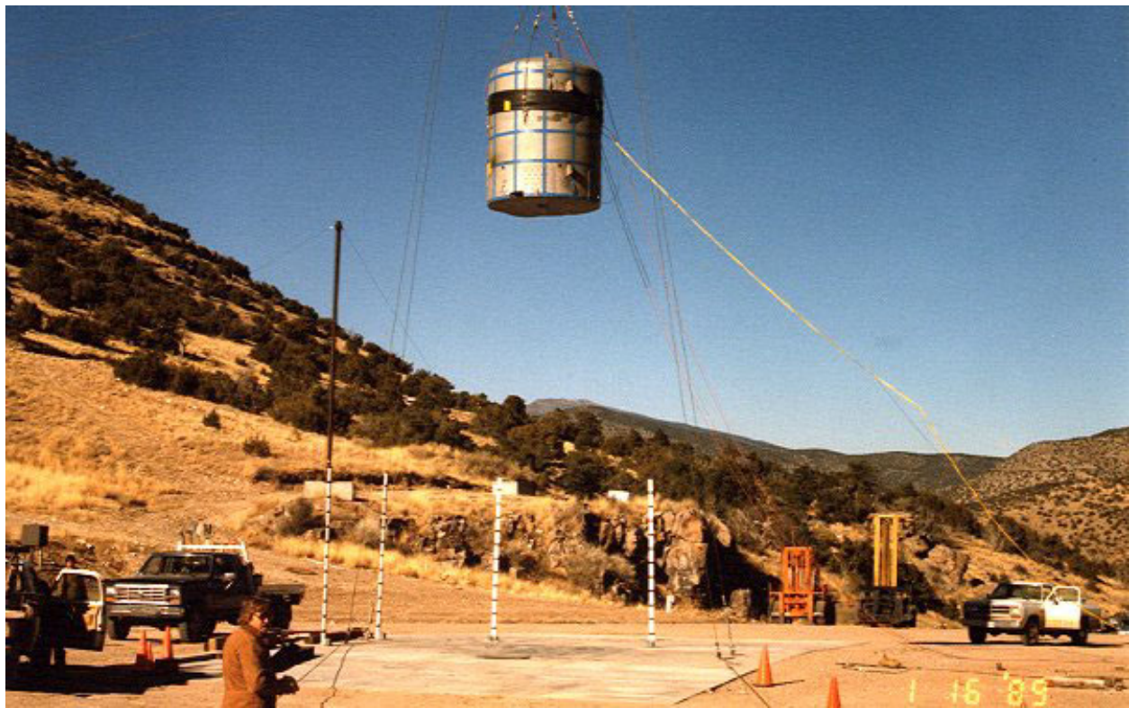
Figure 2.10.3-58 – CTU-2 Free Drop No. 2; Pre-Drop Positioning
