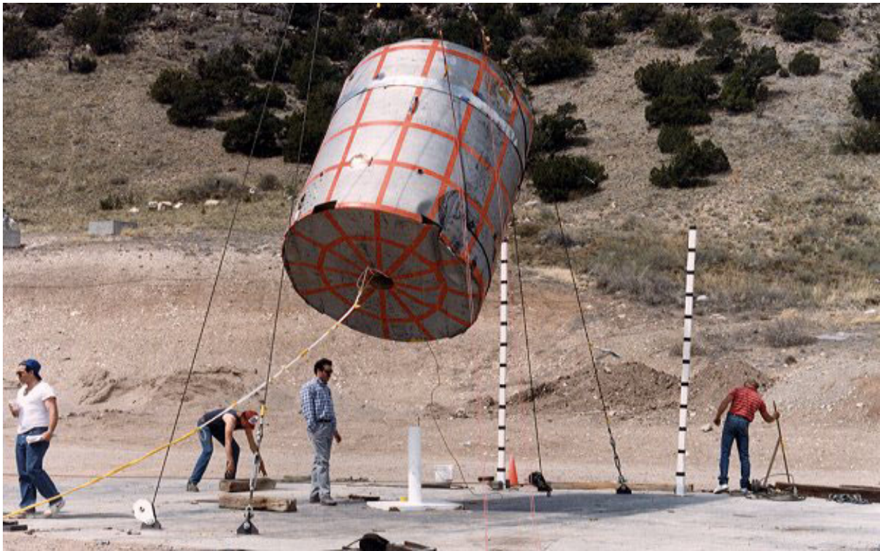
Figure 2.10.3-88 – CTU-3 Puncture Drop No. 5; Pre-Drop Positioning
