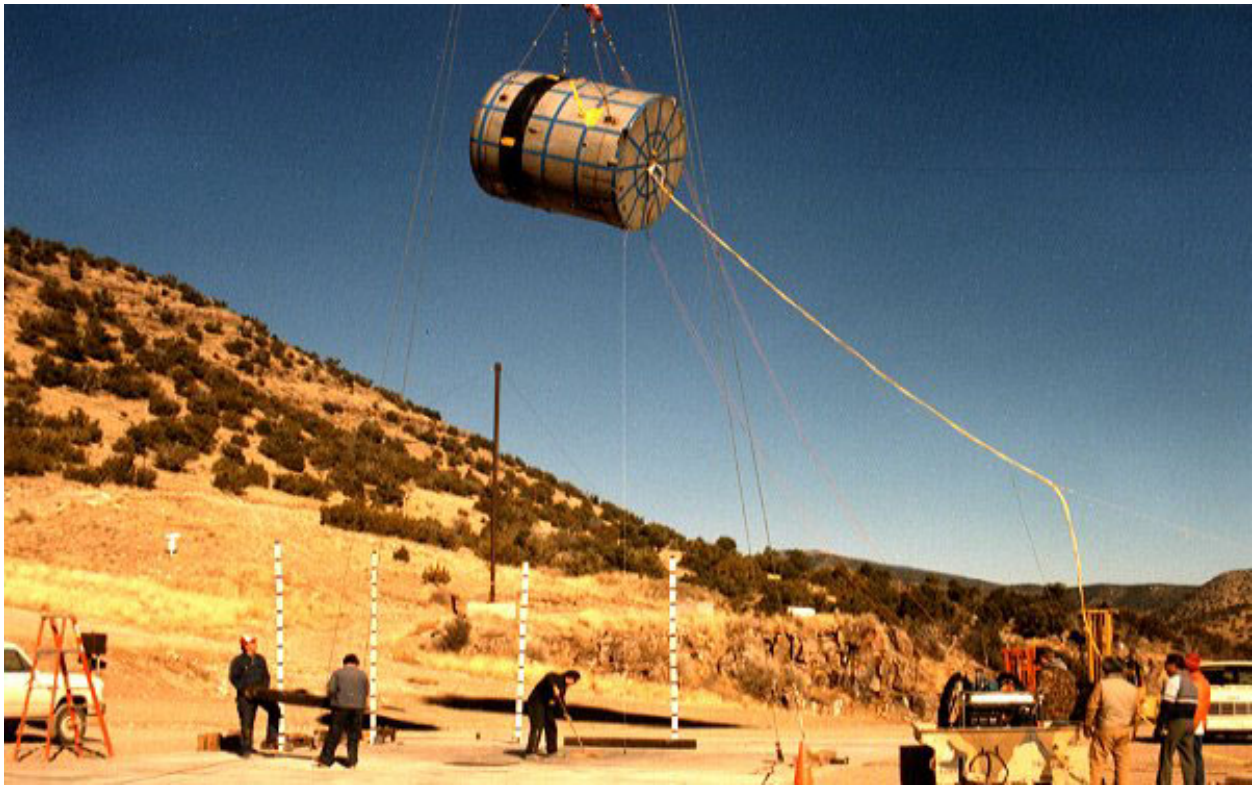
Figure 2.10.3-60 – CTU-2 Free Drop No. 3; Pre-Drop Positioning
