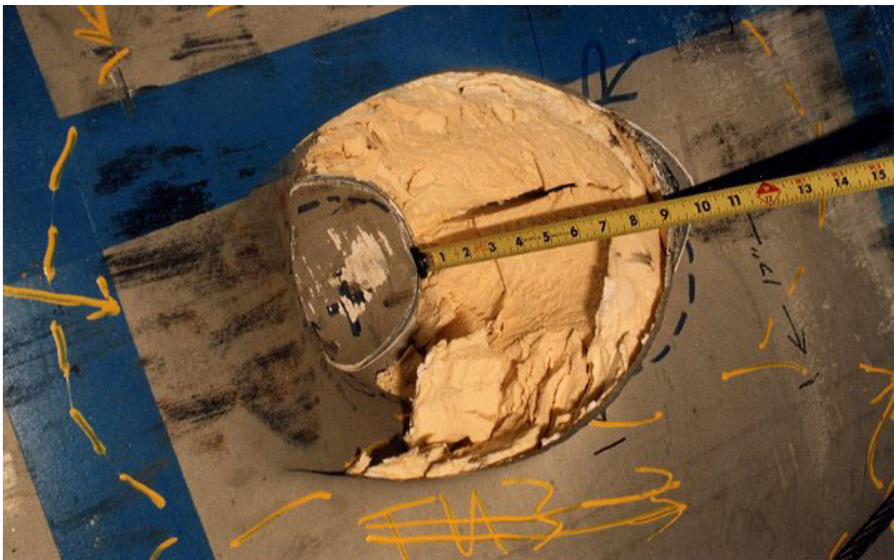
Figure 2.10.3-63 – CTU-2 Puncture Drop R; Post-Drop Damage
