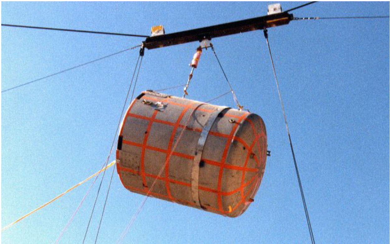
Figure 2.10.3-80 – CTU-3 Free Drop No. 1; Pre-Drop Positioning
