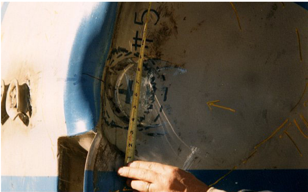
Figure 2.10.3-67 – CTU-2 Puncture Drop 5; Post-Drop Damage
