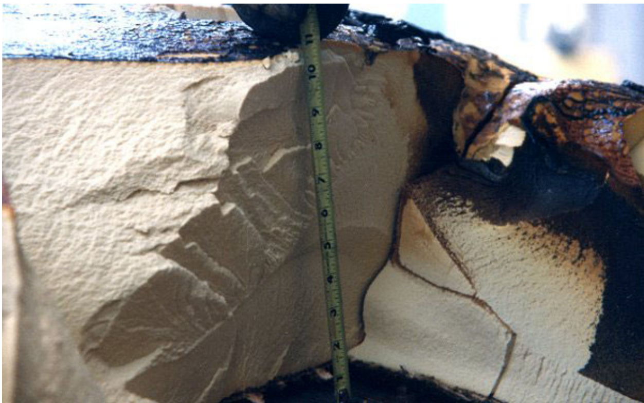
Figure 2.10.3-51 – CTU-1 Disassembly; OCA Lid Unburned Foam Thickness
