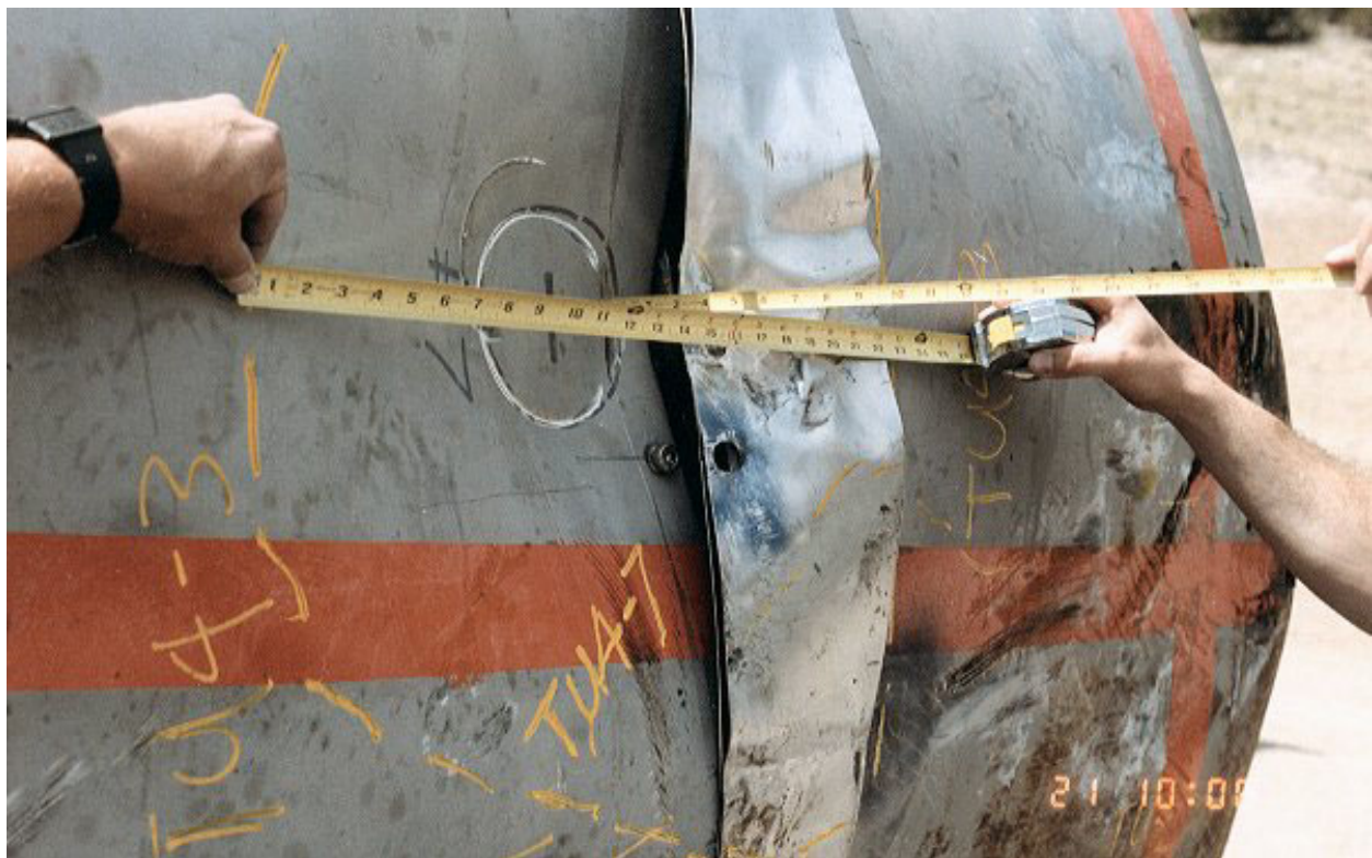
Figure 2.10.3-93 – CTU-3 Puncture Drop 7; Post-Drop Damage
