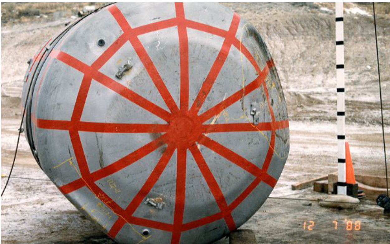
Figure 2.10.3-35 – CTU-1 Free Drop No. 4; Post-Drop Damage
