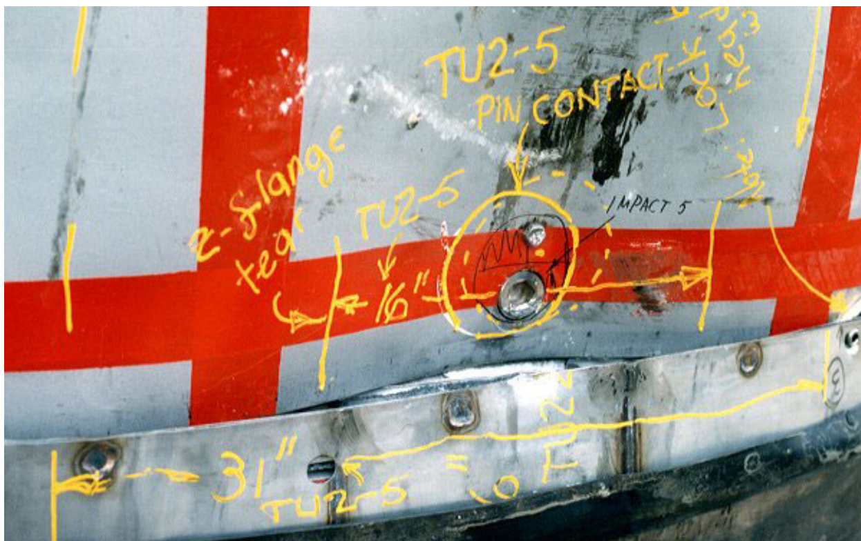
Figure 2.10.3-37 – CTU-1 Puncture Drop No. 5; Post-Drop Damage
