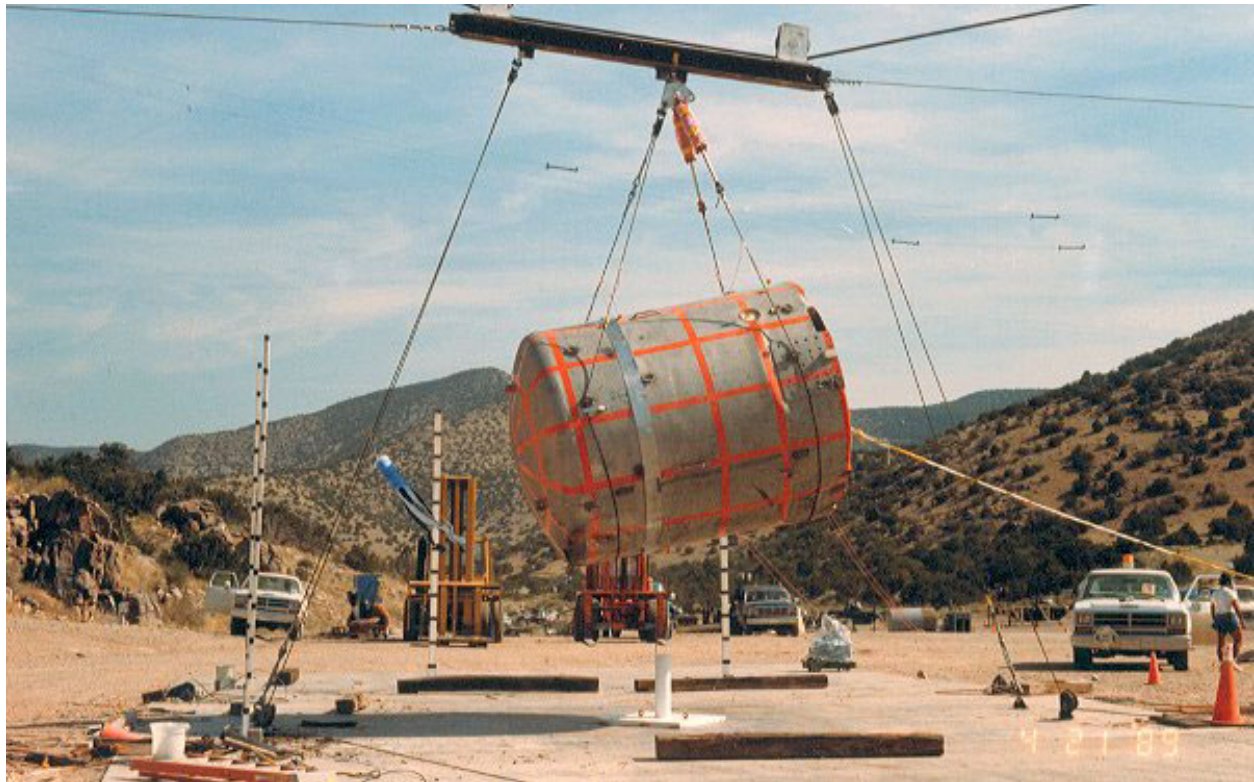
Figure 2.10.3-92 – CTU-3 Puncture Drop No. 7; Pre-Drop Positioning
