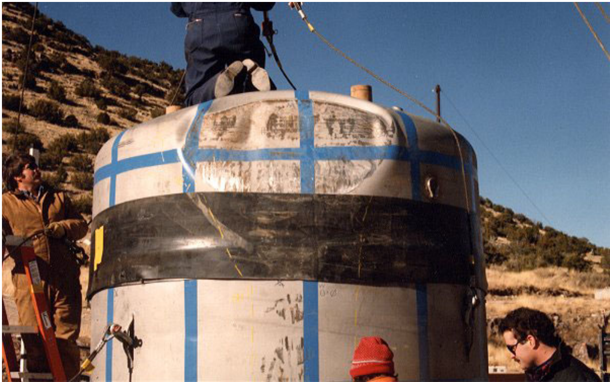
Figure 2.10.3-56 – CTU-2 Free Drop No. 1; Post-Drop Damage
