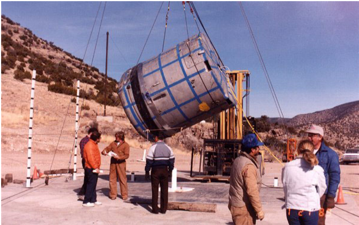
Figure 2.10.3-72 – CTU-2 Puncture Drop No. 8; Pre-Drop Positioning
