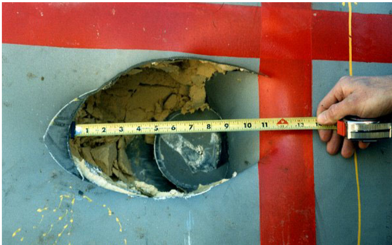
Figure 2.10.3-41 – CTU-1 Puncture Drop No. 7; Post-Drop Damage
