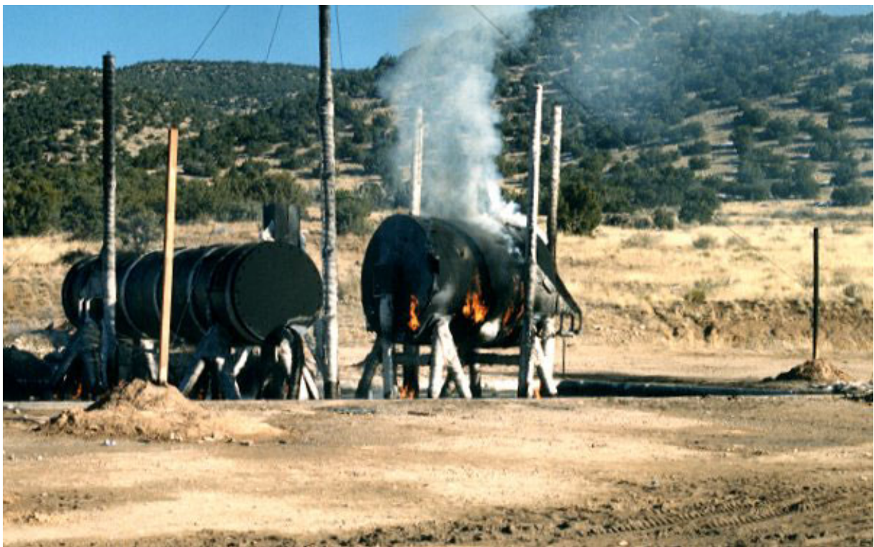
Figure 2.10.3-49 – CTU-1 Fire No. 10; Post-Fire Cool-Down
