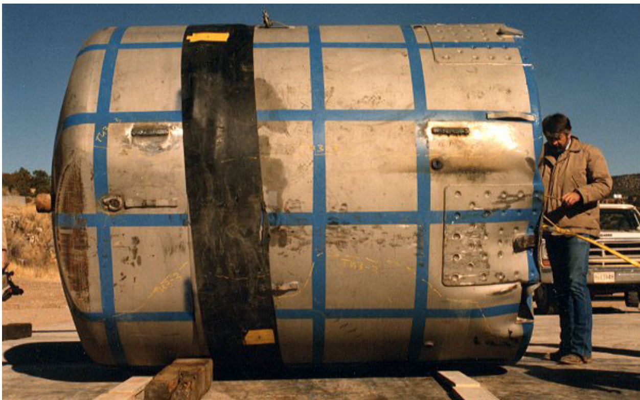
Figure 2.10.3-61 – CTU-2 Free Drop No. 3; Post-Drop Damage
