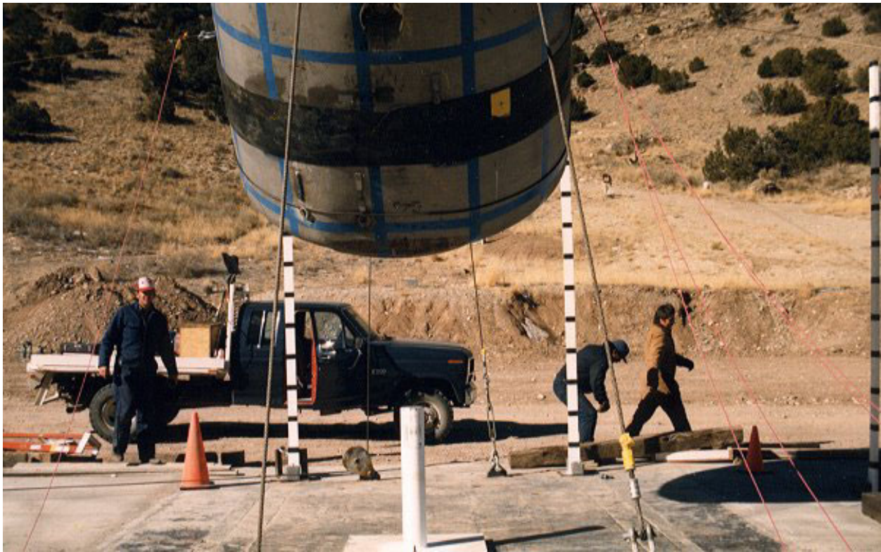
Figure 2.10.3-64 – CTU-2 Puncture Drop No. 4; Pre-Drop Positioning
