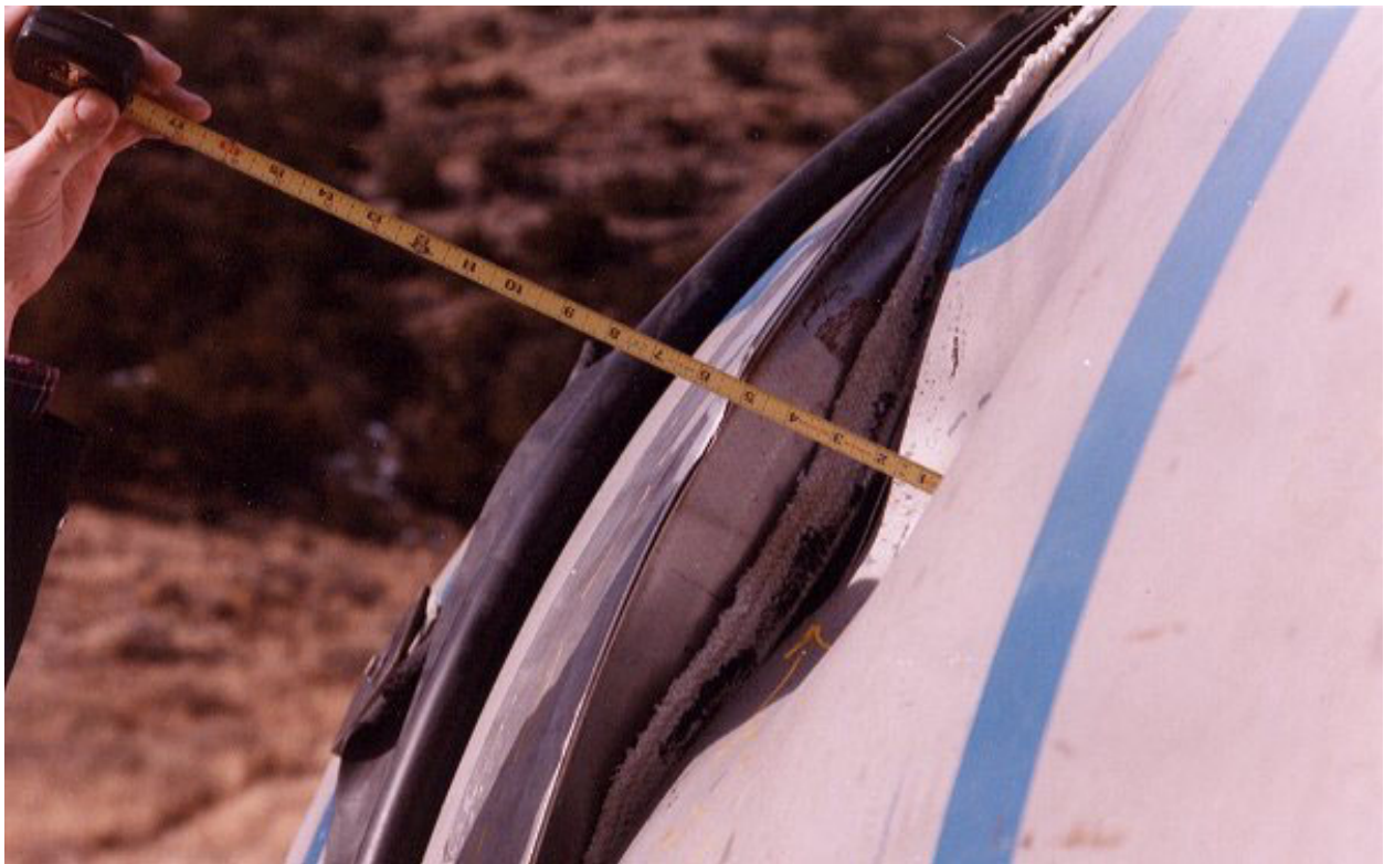
Figure 2.10.3-71 – CTU-2 Puncture Drop 7; Post-Drop Damage
