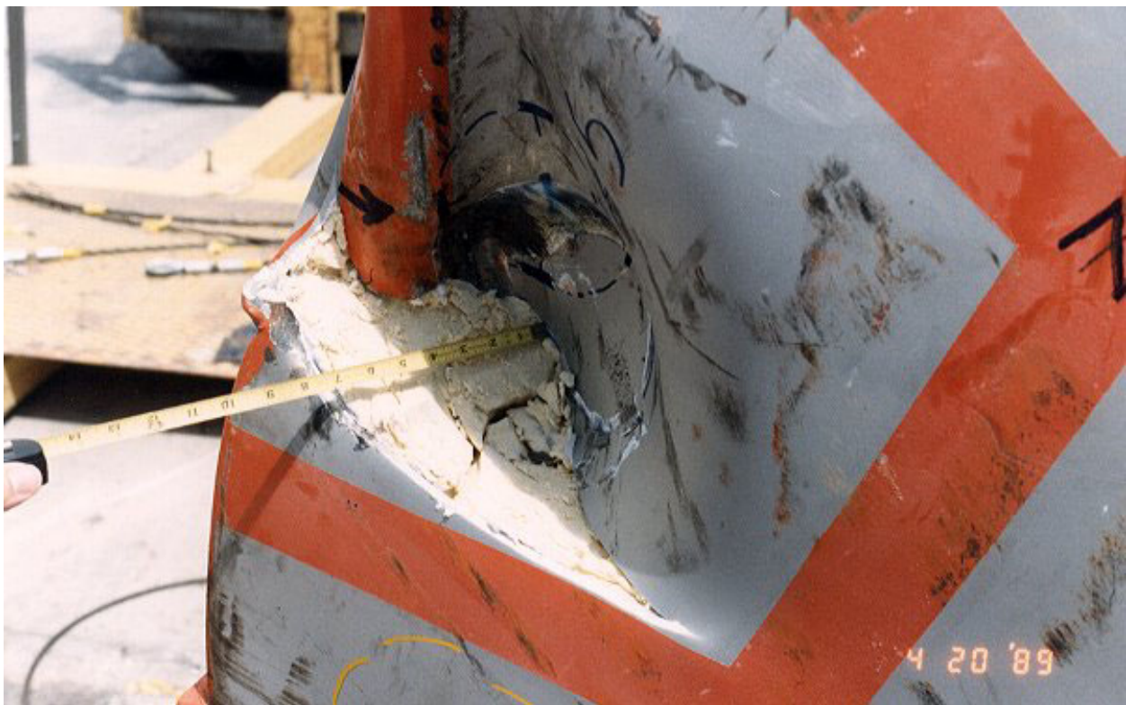
Figure 2.10.3-89 – CTU-3 Puncture Drop 5; Post-Drop Damage
