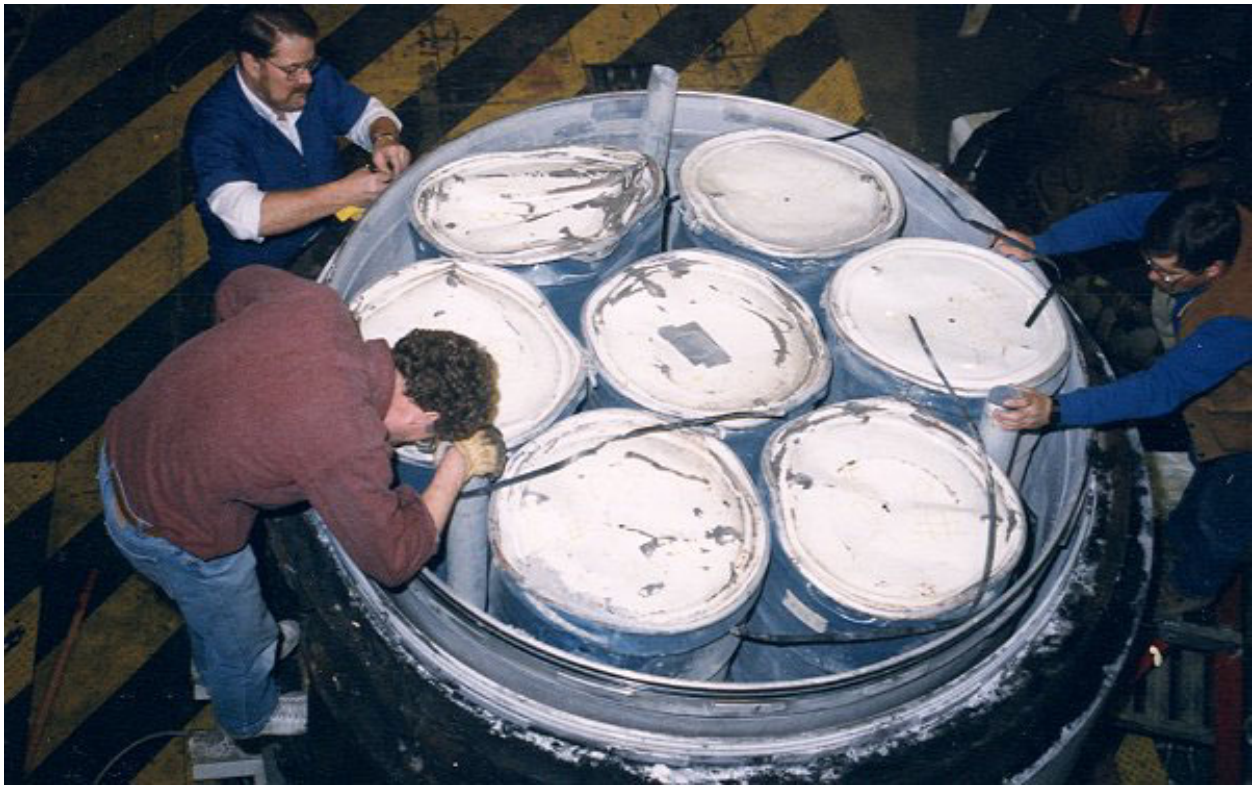
Figure 2.10.3-52 – CTU-1 Disassembly; Payload Drum Removal
