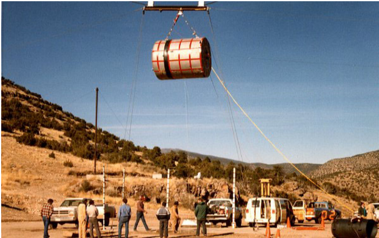
Figure 2.10.3-30 – CTU-1 Free Drop No. 2; Pre-Drop Positioning
