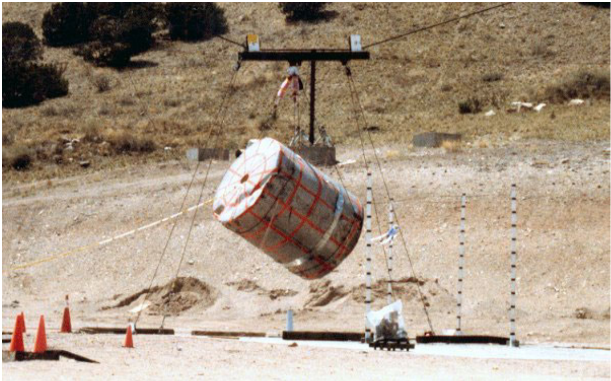
Figure 2.10.3-94 – CTU-3 Puncture Drop No. 8; Pre-Drop Positioning
