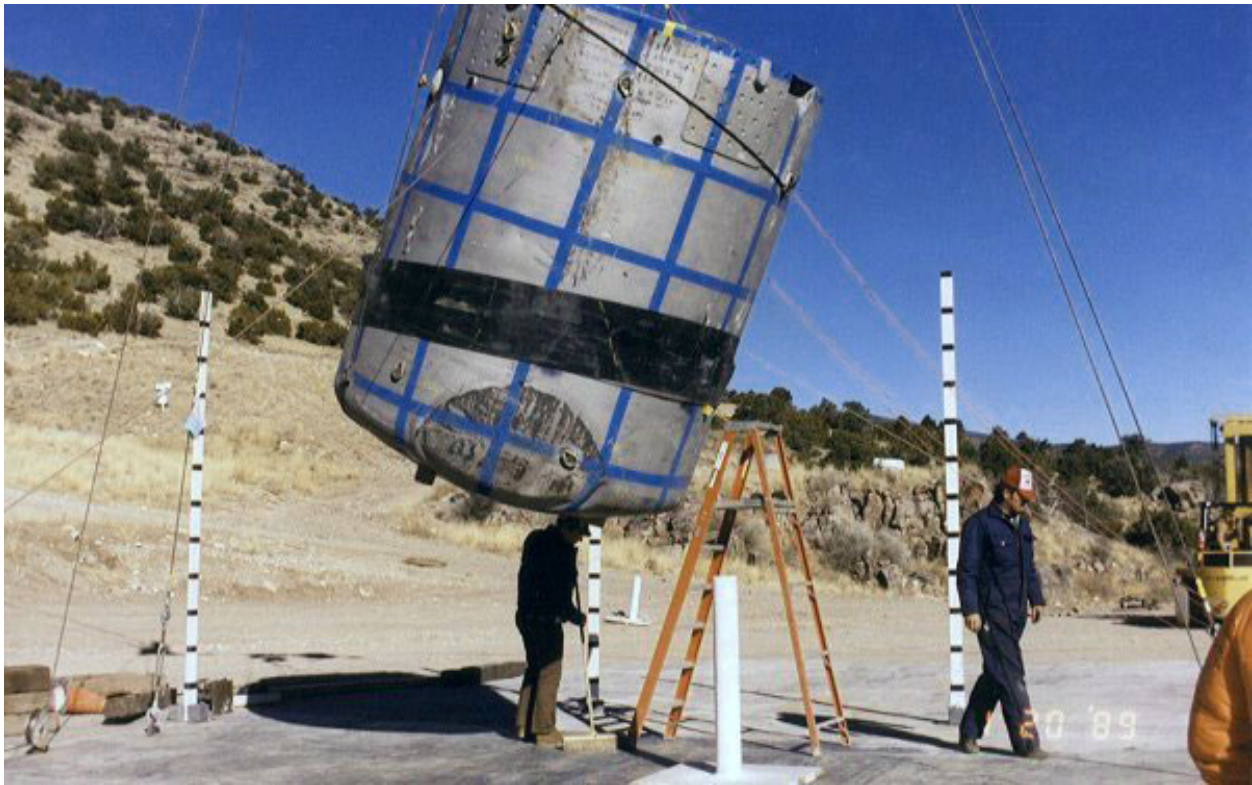
Figure 2.10.3-68 – CTU-2 Puncture Drop No. 6; Pre-Drop Positioning
