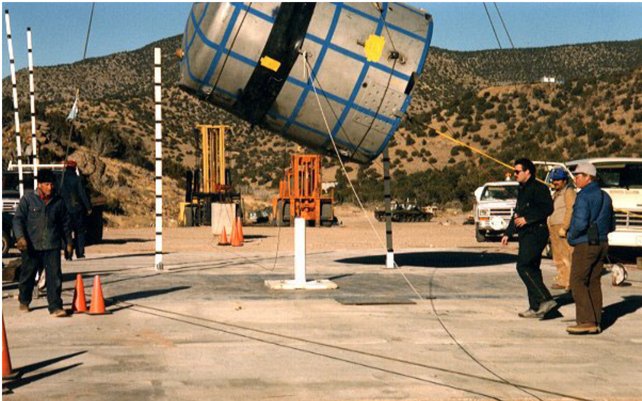
Figure 2.10.3-62 – CTU-2 Puncture Drop No. R; Pre-Drop Positioning
