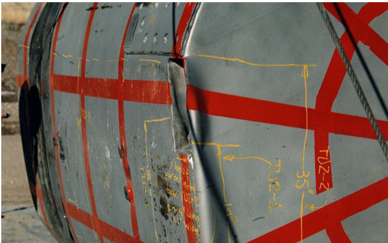
Figure 2.10.3-31 – CTU-1 Free Drop No. 2; Post-Drop Damage
