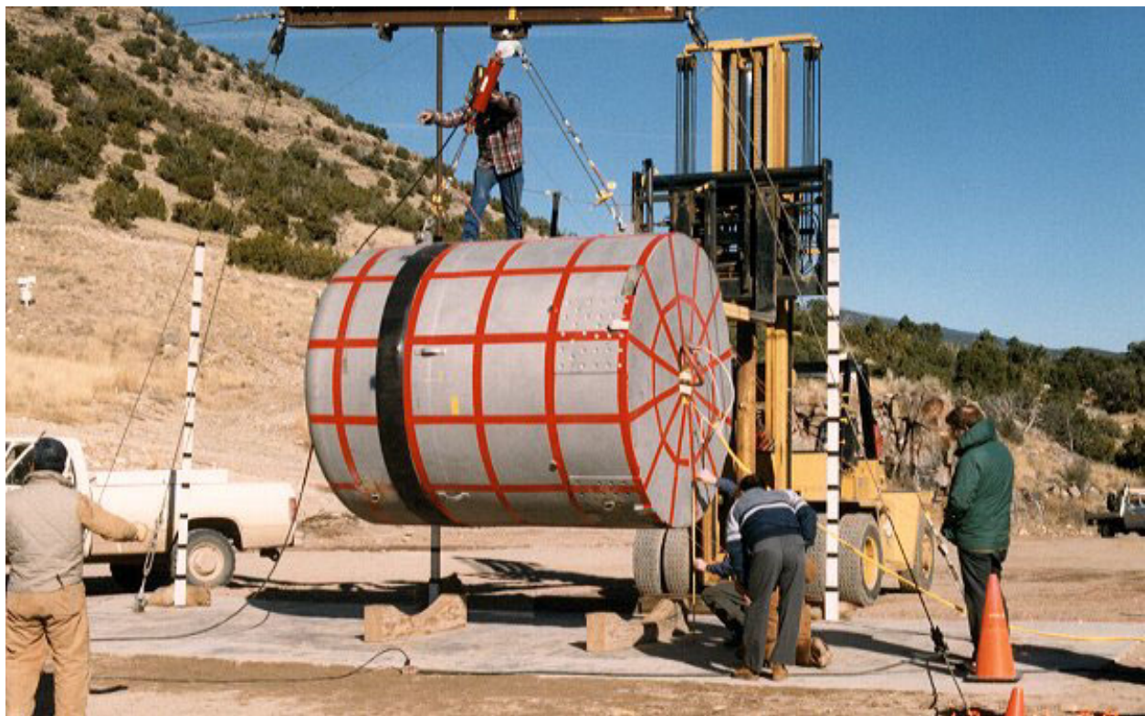
Figure 2.10.3-27 – CTU-1 Free Drop No. 1; Pre-Drop Positioning
