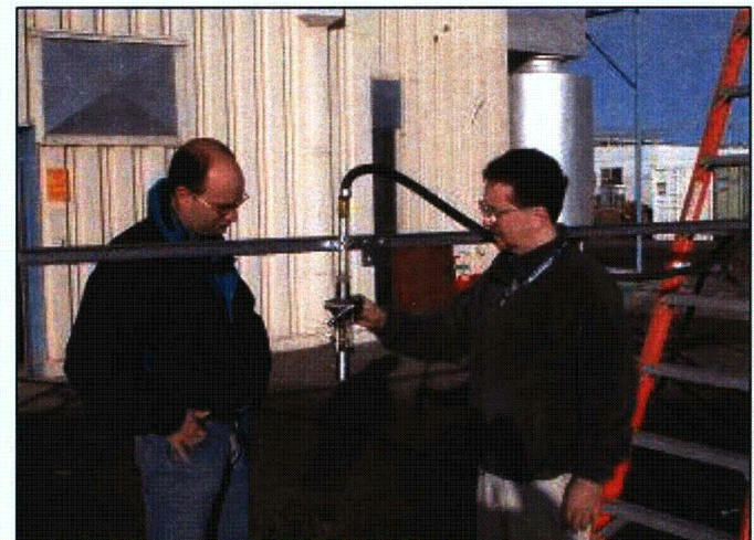
Testing Saltcake Dissolution Nozzles
