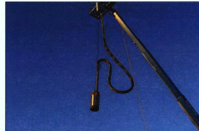
Adjustable Height Retrieval Pump
