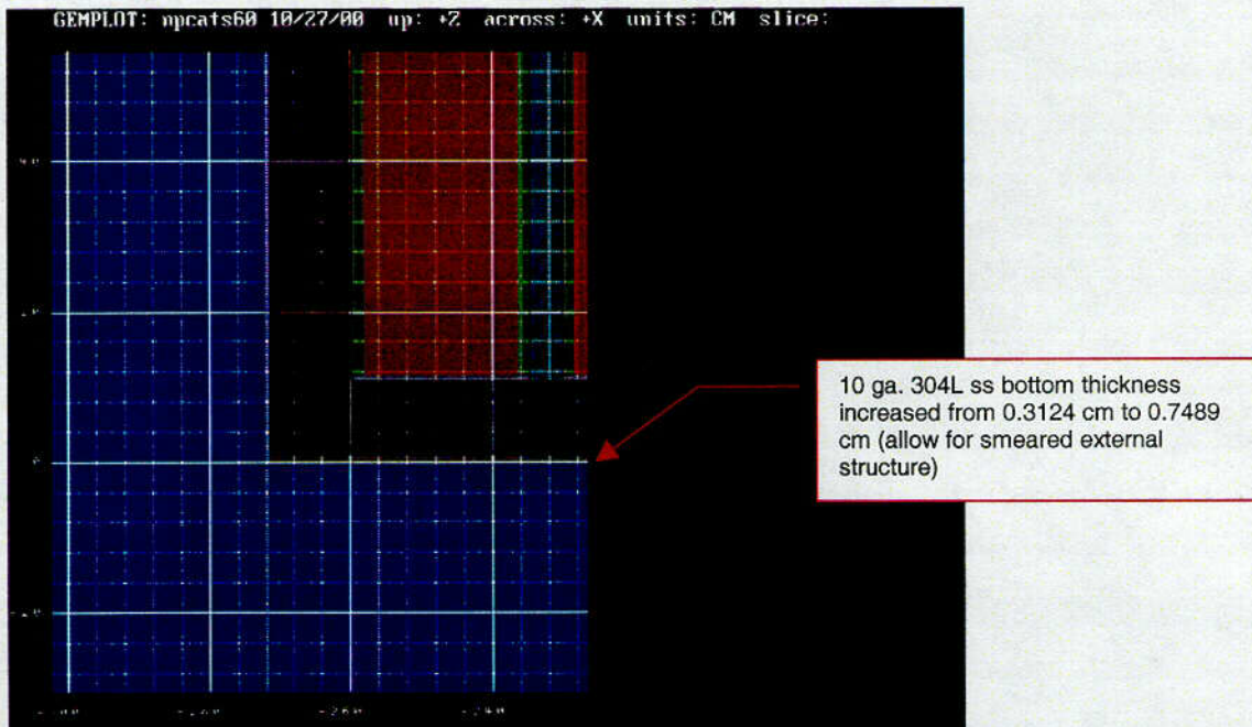
Figure 6.7h – Fully reflected damaged 5 \times 5 \times 6 package array: 60 kgs \text{UO}_2 + \text{H}_2\text{O} mixture, maximum burn, external structure add-on to bottom of OCA body (vertical zoom, lower left array corner)
