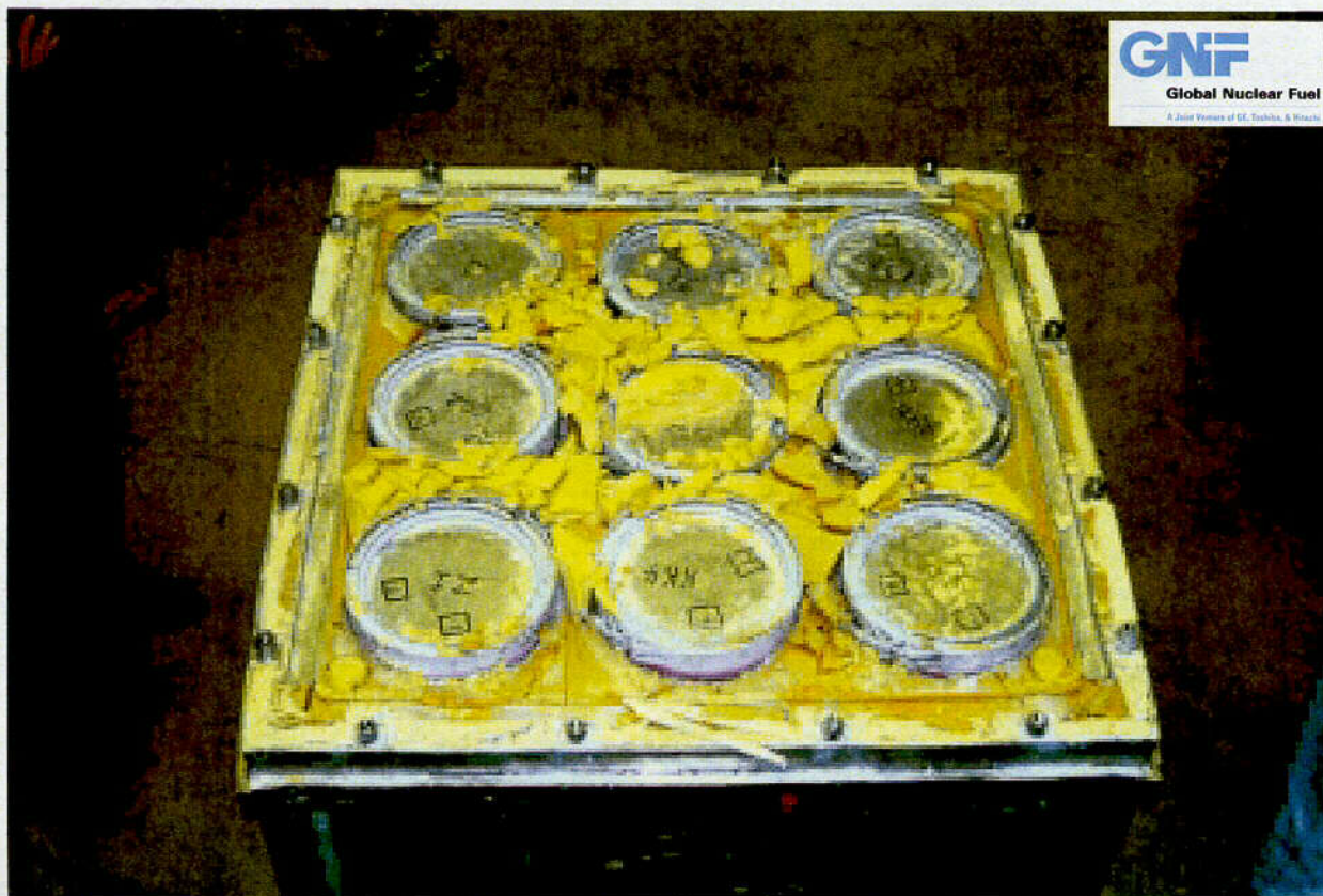
Figure 2.10.1-95 – CTU-4 Post-Test Disassembly; View of OCA Lid Foam Debris
