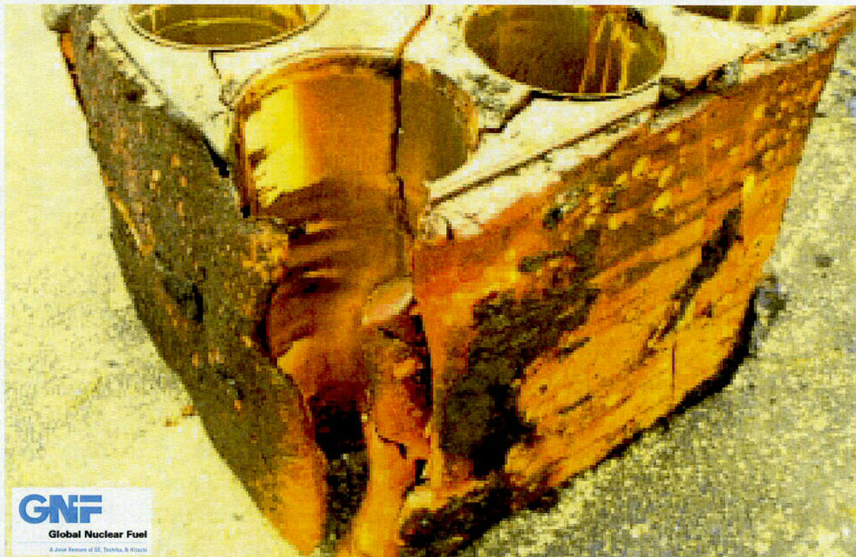
Figure 2.10.1-56 – CTU-2 Post-Test Disassembly; View of Damage to OCA Foam Block
