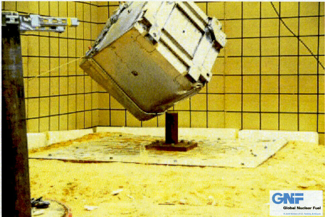
Figure 2.10.1-39 – CTU-2 Puncture Drop Test No. 9A, Immediately After Impact
