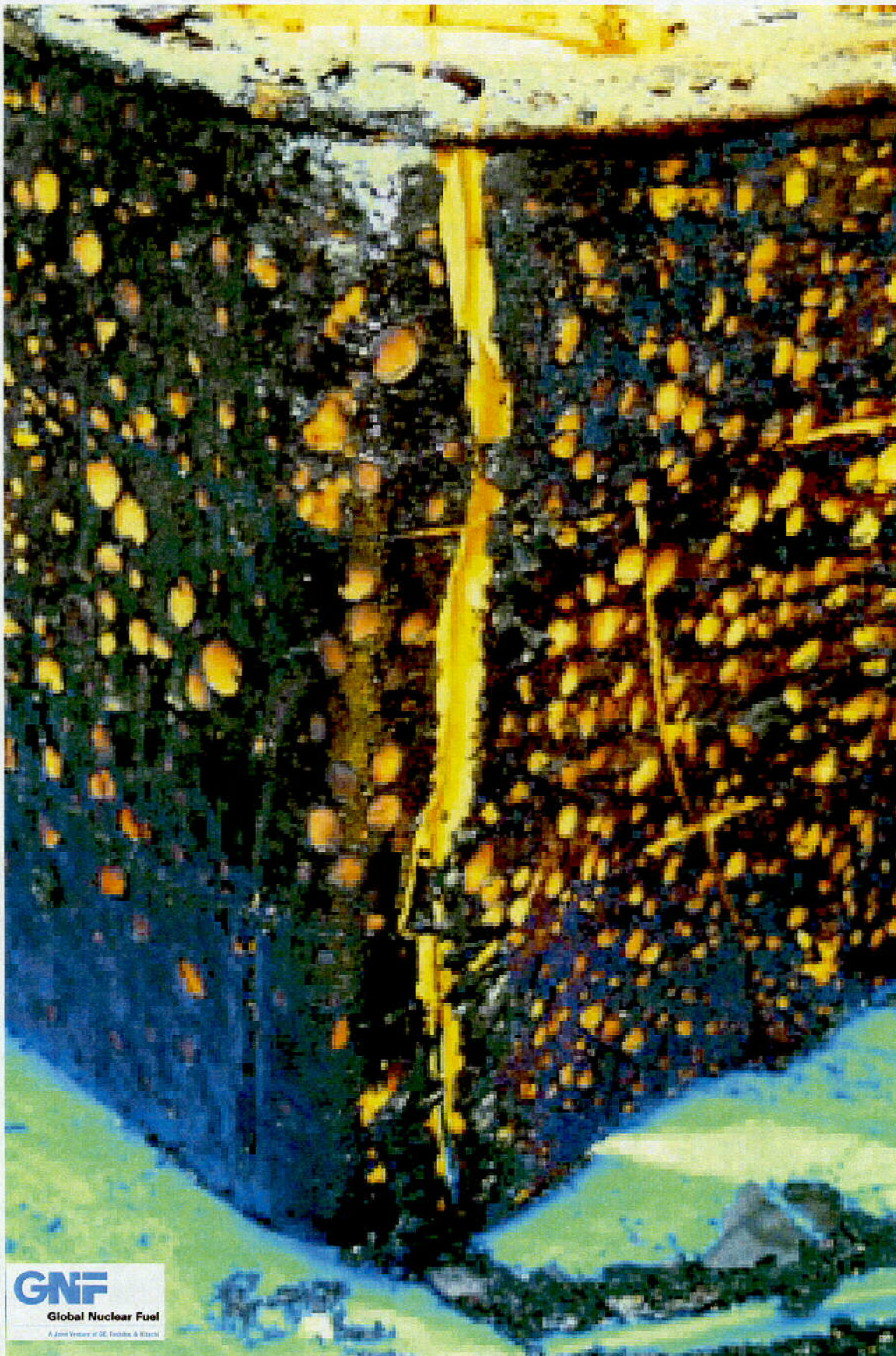
Figure 2.10.1-28 – CTU-1 Post-Test Disassembly; View of Foam Crack Near Impact Corner
