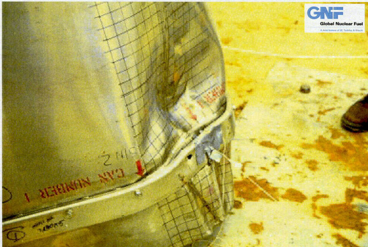
Figure 2.10.1-41 – CTU-2 Puncture Drop Test No. 9B; View of Damage
