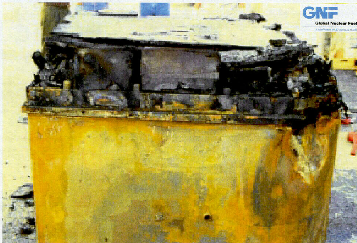
Figure 2.10.1-48 – CTU-2 Post-Test Disassembly; View of OCA Body w/ OCA Lid Removed
