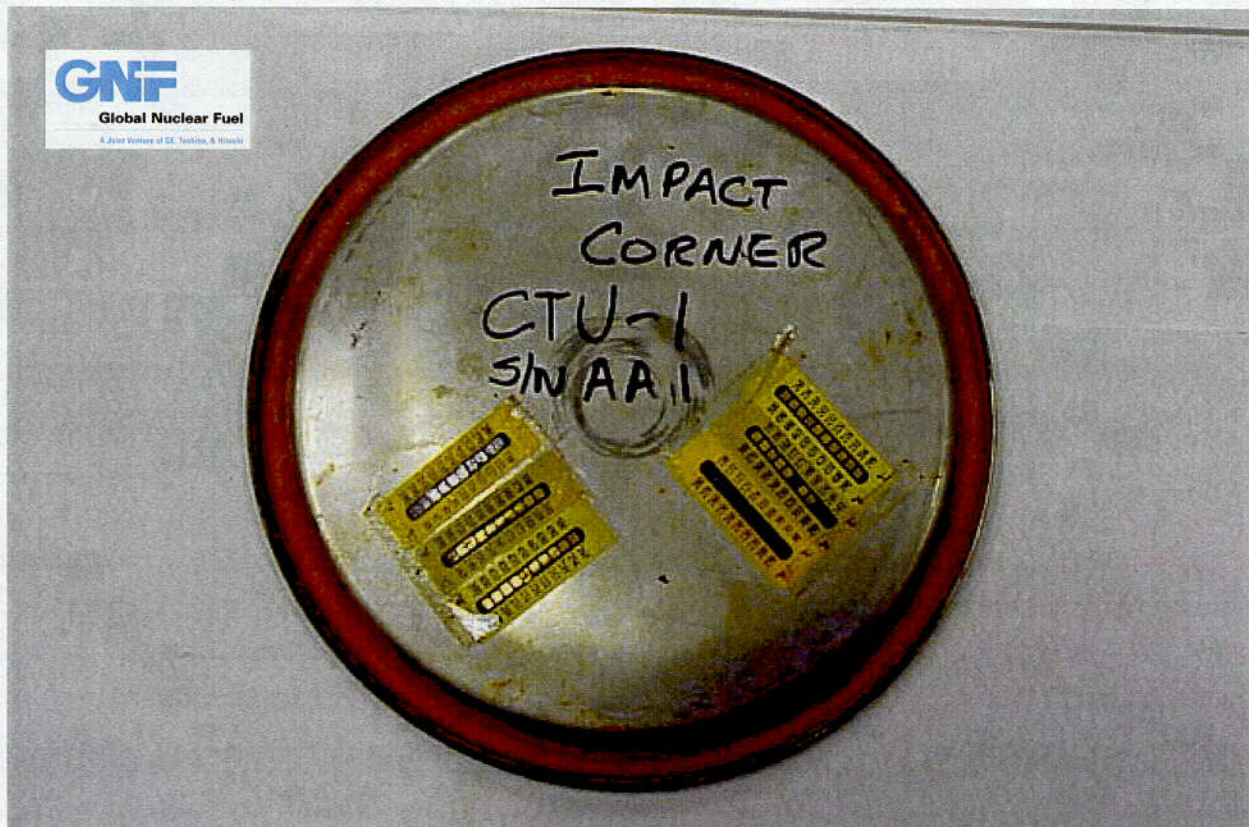
Figure 2.10.1-31 – CTU-1 Post-Test Disassembly; View of ICCA Closure Lid
