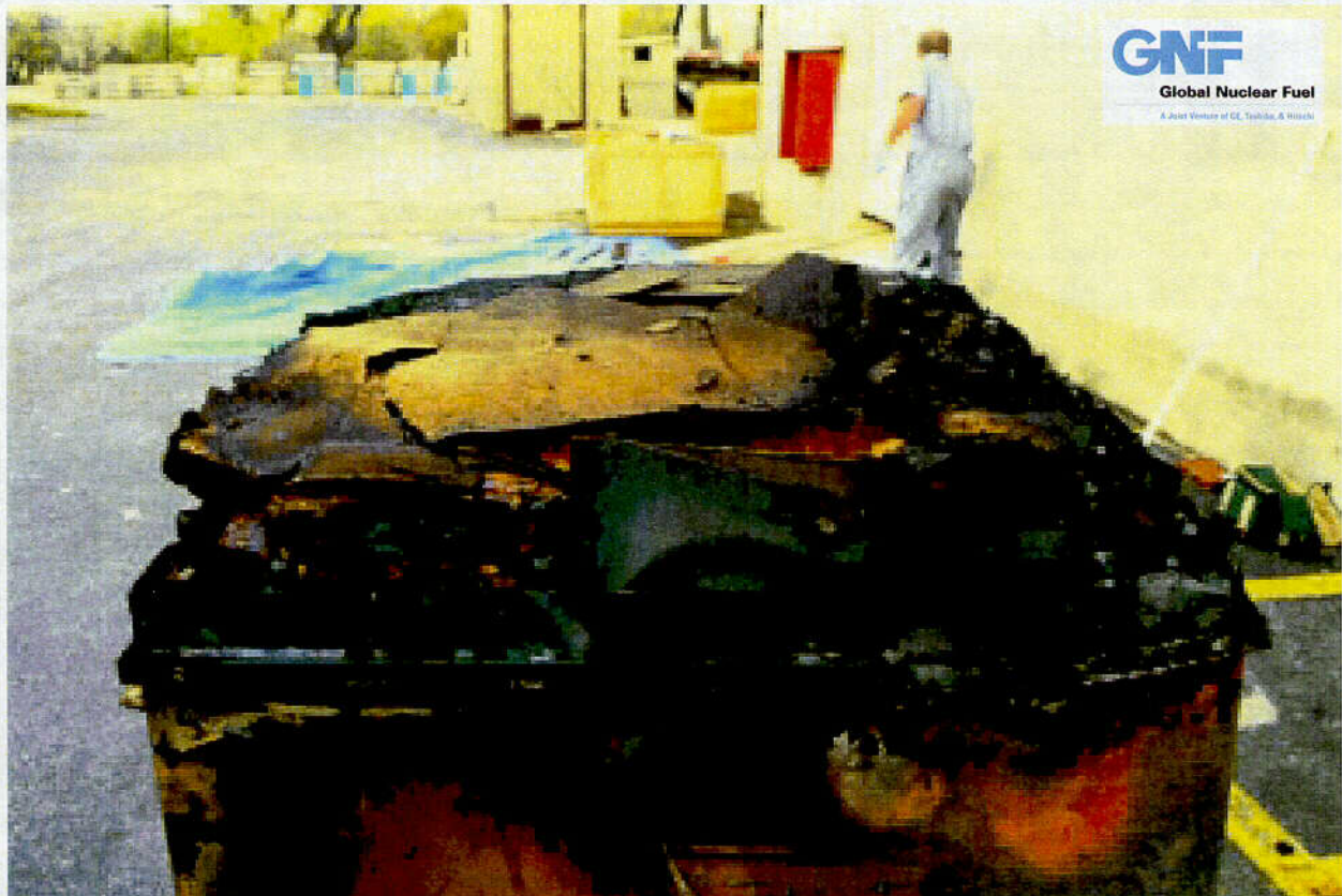
Figure 2.10.1-24 – CTU-1 Post-Test Disassembly; View of OCA Body with OCA Lid Removed
