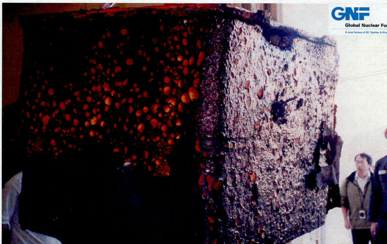
Figure 2.10.1-76 – CTU-3 Post-Test Disassembly; View of Residual OCA Foam Block
