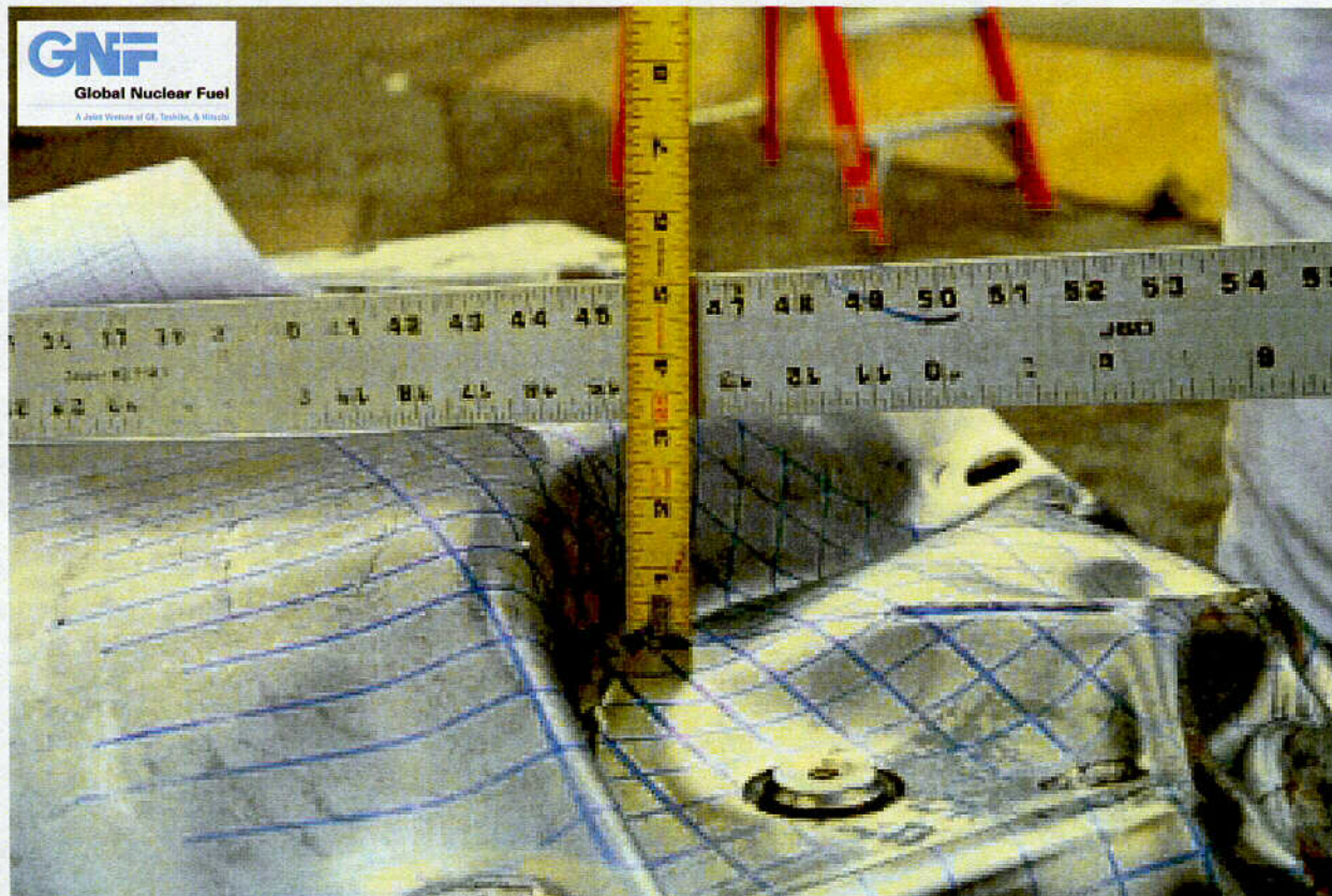
Figure 2.10.1-13 – CTU-1 Free Drop Test No. 2; Height of Buckle of OCA Lid Corner
