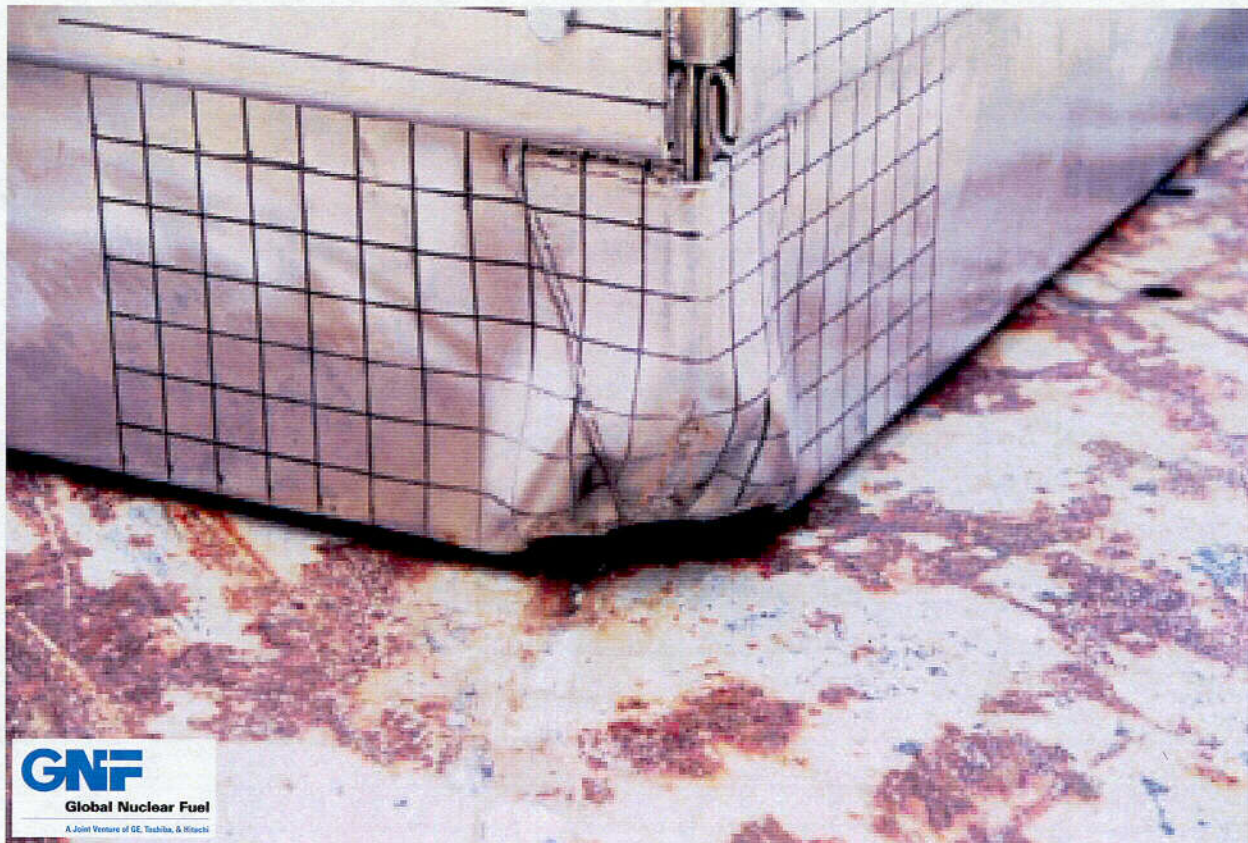
Figure 2.10.1-58 – CTU-3 Free Drop Test No. 1; OCA Lid Corner Damage; ~5" Wide
