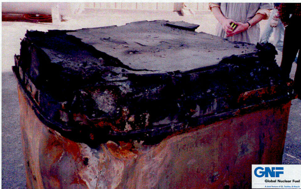
Figure 2.10.1-71 – CTU-3 Post-Test Disassembly; View with OCA Lid Removed
