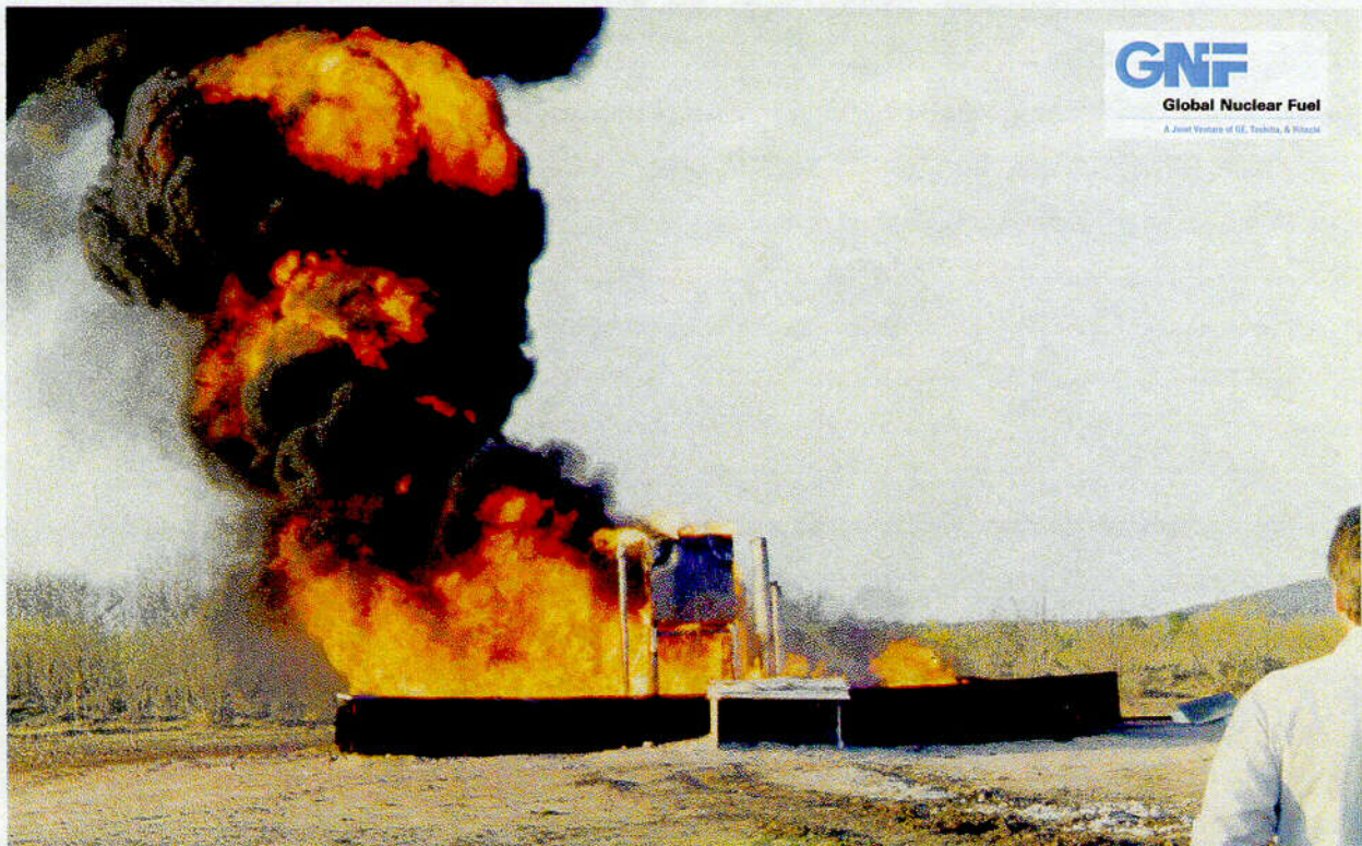
Figure 2.10.1-19 - CTU-1 Fire Test No. 15; Overall View ~32 Minutes after Start
