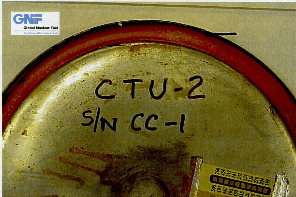
Figure 2.10.1-53 – CTU-2 Post-Test Disassembly; View of ICCA Gasket
