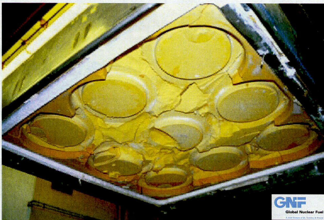
Figure 2.10.1-94 – CTU-4 Post-Test Disassembly; View of Underside of OCA Lid
