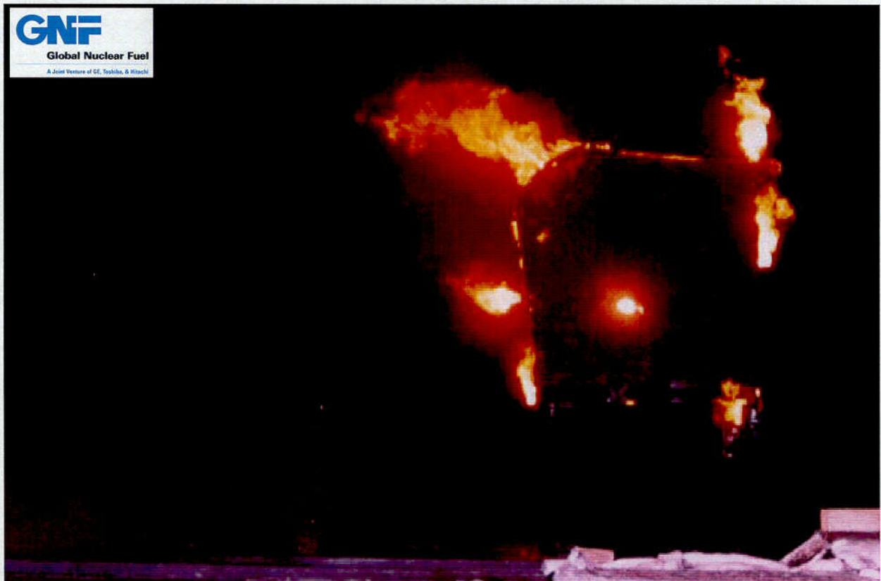
Figure 2.10.1-67 – CTU-3 Fire Test 15; View ~15 Minutes after End of Fire (Note Flares)
