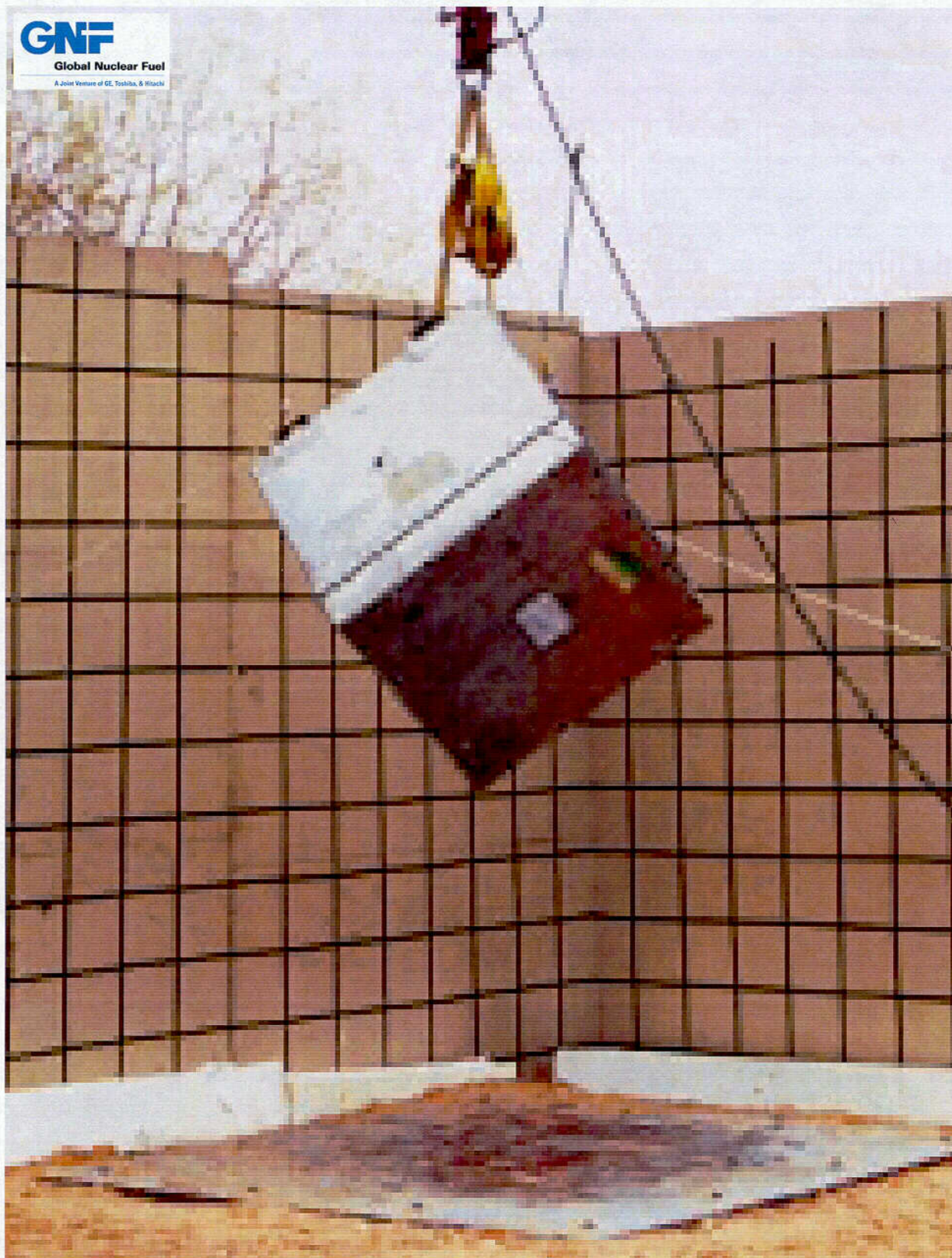
Figure 2.10.1-57 – CTU-3 Free Drop Test No. 1; NCT Drop onto OCA Lid Corner
