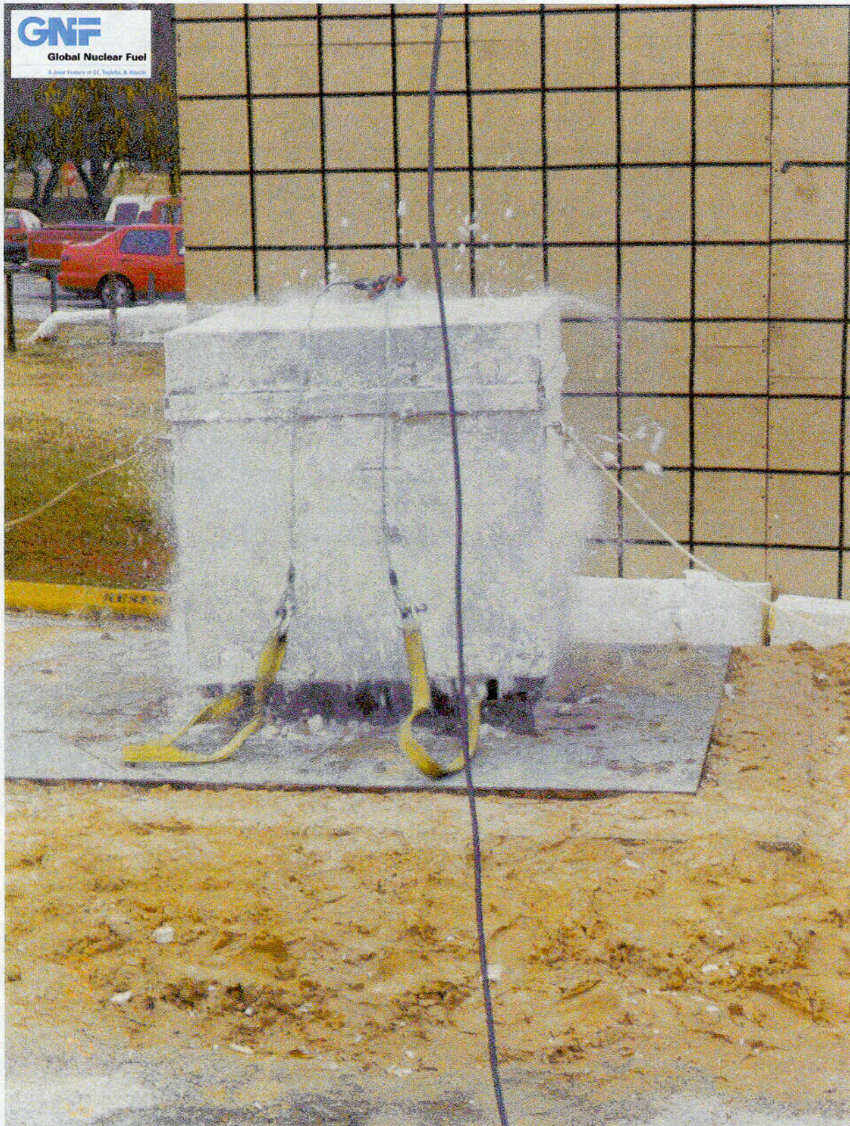
Figure 2.10.1-82 – CTU-4 Free Drop Test No. 7; NCT Drop at Impact
