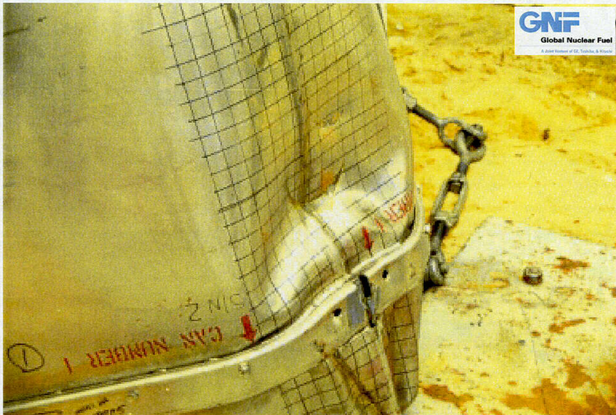
Figure 2.10.1-40 – CTU-2 Puncture Drop Test No. 9A; Close-up View of Damage
