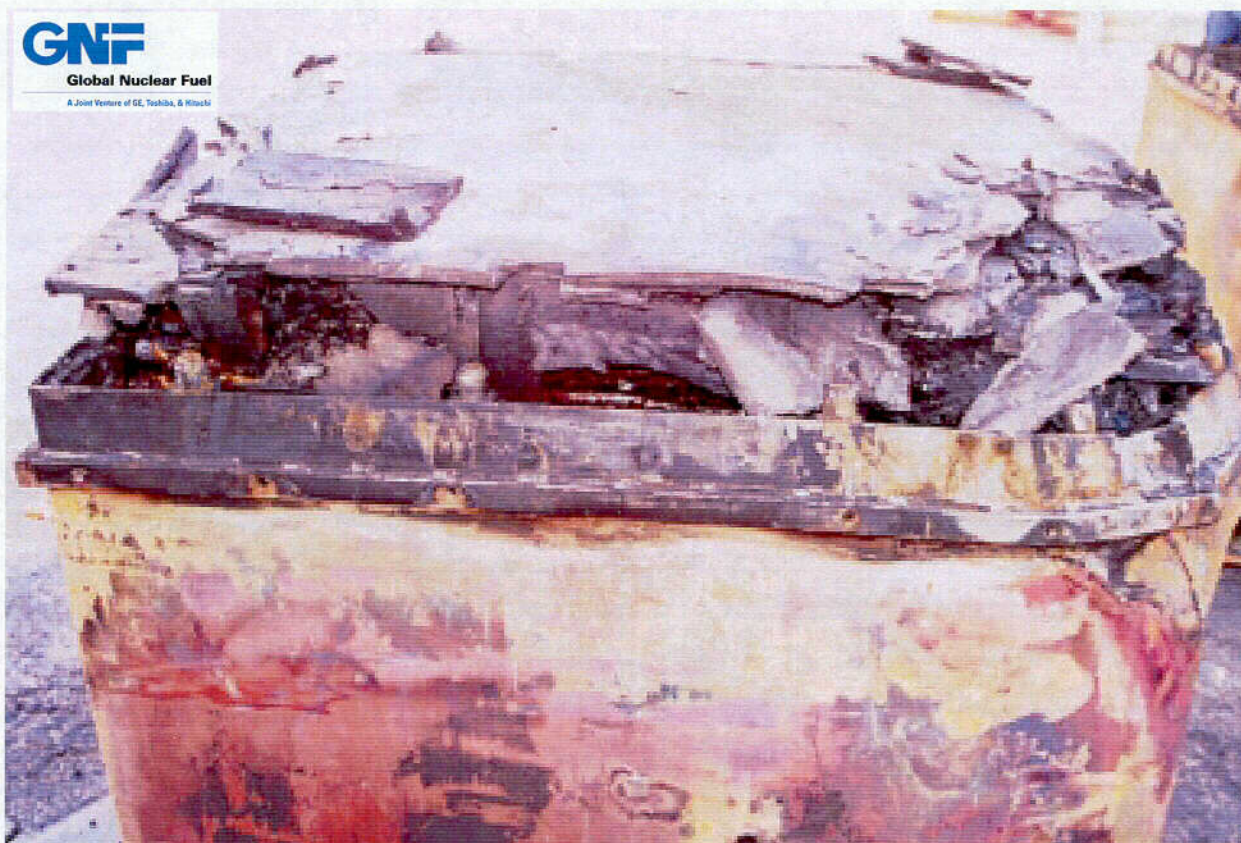
Figure 2.10.1-72 – CTU-3 Post-Test Disassembly; View with OCA Lid Removed
