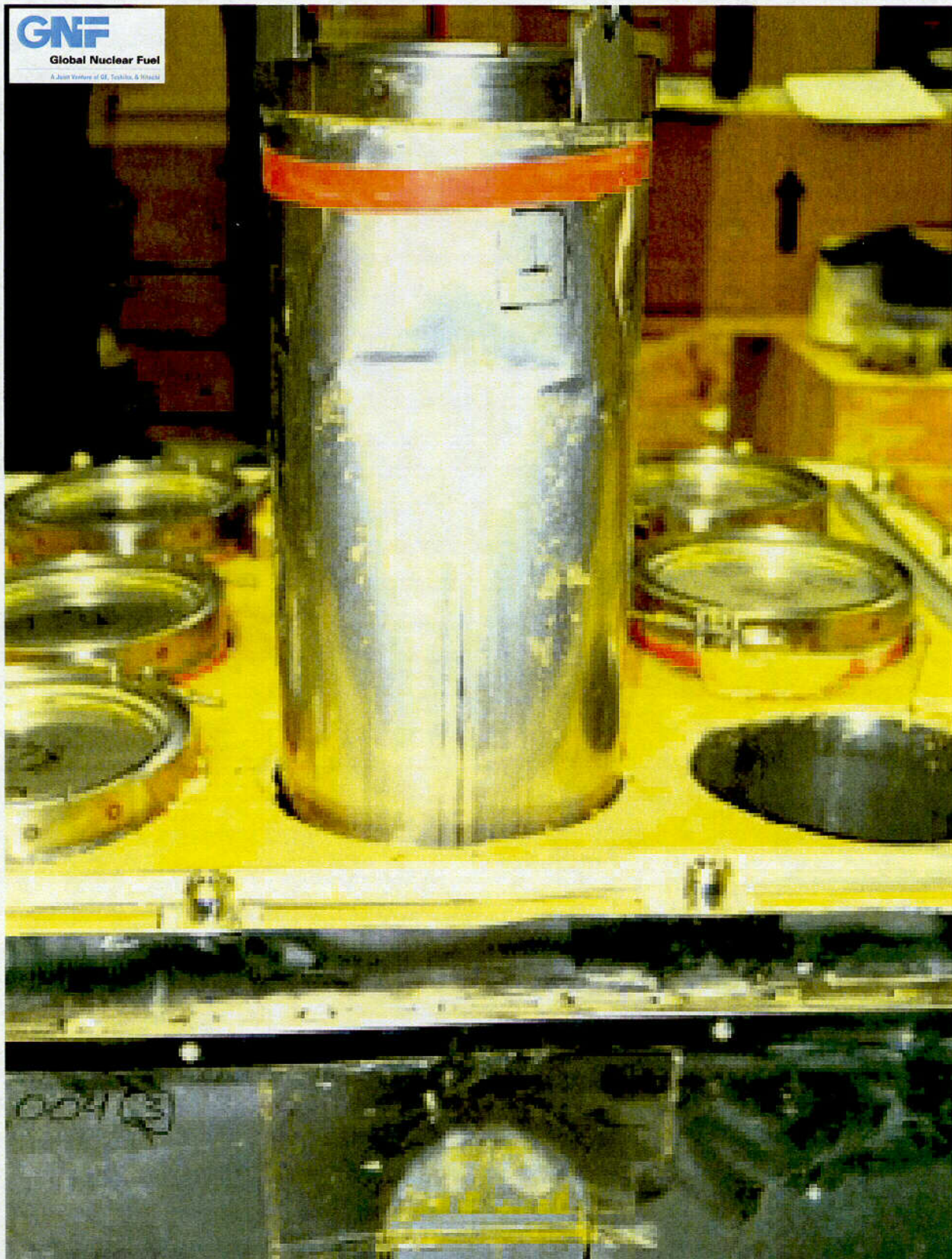
Figure 2.10.1-98 – CTU-4 Post-Test Disassembly; Close-up View of Damaged ICCA
