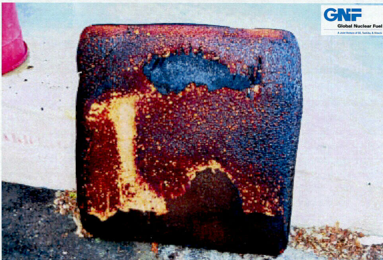
Figure 2.10.1-77 – CTU-3 Post-Test Disassembly; View of Residual OCA Bottom Foam
