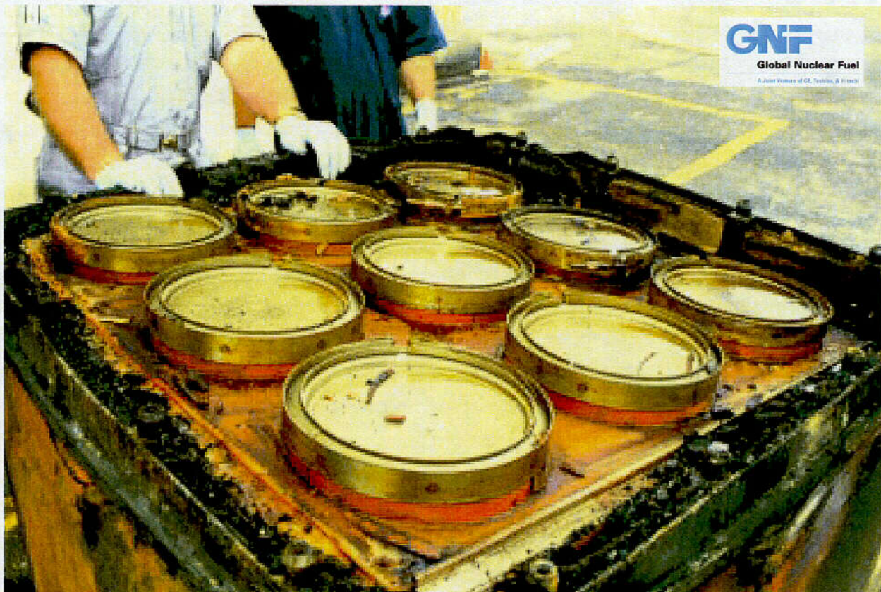
Figure 2.10.1-26 – CTU-1 Post-Test Disassembly; View of ICCAs/Foam Block Structure
