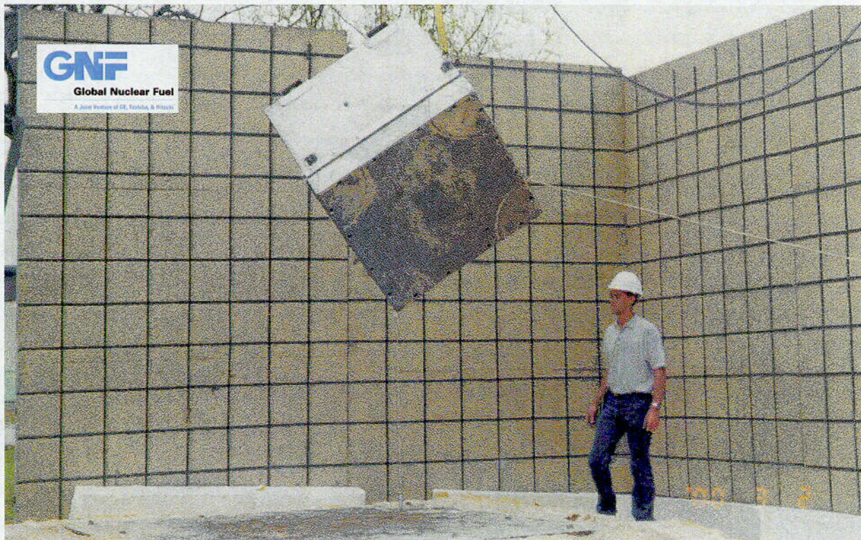
Figure 2.10.1-9 - CTU-1 Free Drop Test No. 1; NCT Drop onto OCA Lid Corner
