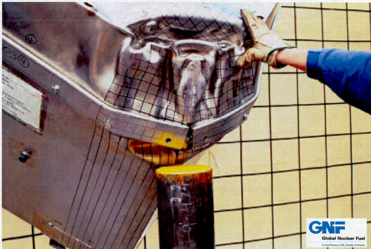
Figure 2.10.1-61 - CTU-3 Puncture Drop Test No. 11; Orientation of CTU Prior to Test
