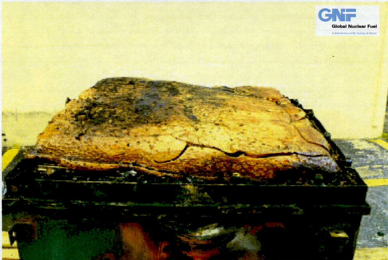
Figure 2.10.1-25 – CTU-1 Post-Test Disassembly; View of Residual Foam w/ Foam Char Removed
