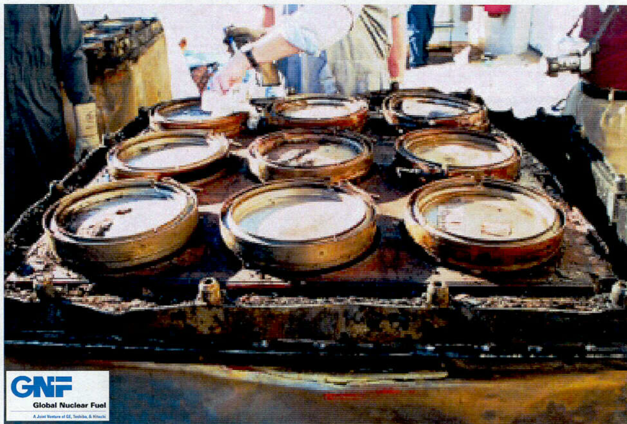
Figure 2.10.1-73 – CTU-3 Post-Test Disassembly; View of ICCAs/Foam Block Structure
