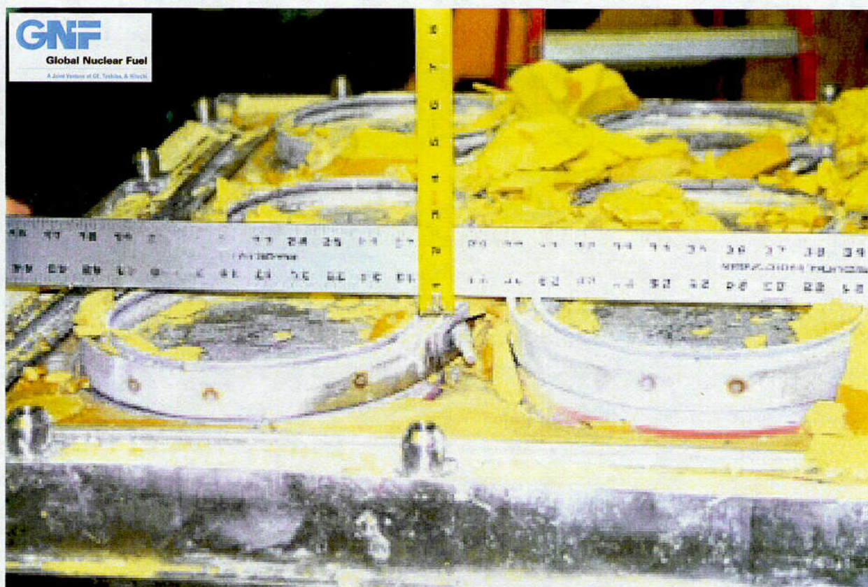
Figure 2.10.1-96 – CTU-4 Post-Test Disassembly; View of Vertical Position of ICCAs
