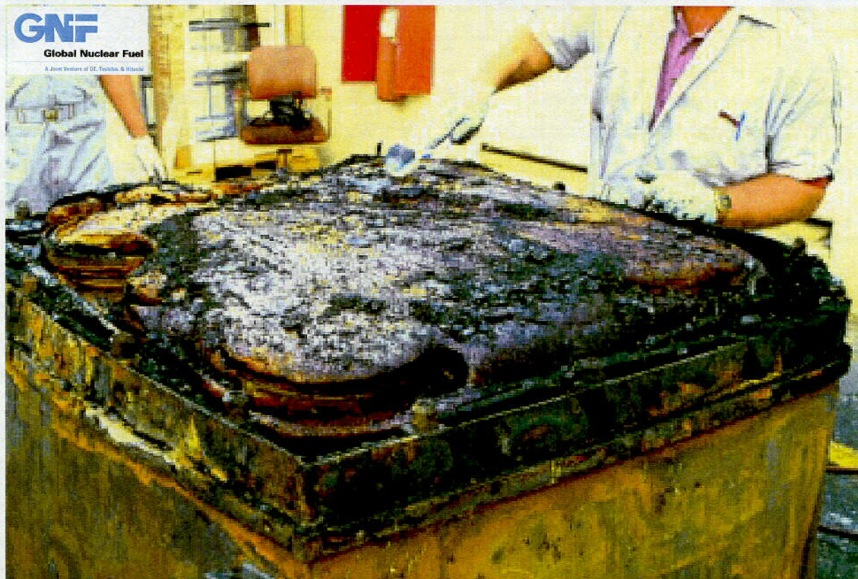
Figure 2.10.1-49 – CTU-2 Post-Test Disassembly; Residual Foam with Foam Char Removed
