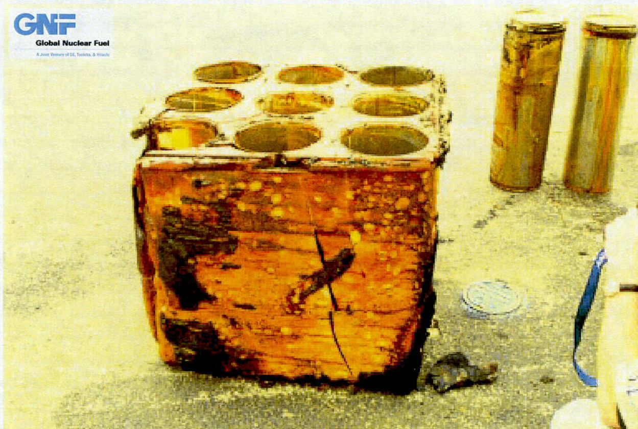
Figure 2.10.1-55 – CTU-2 Post-Test Disassembly; View of OCA Residual Foam Block
