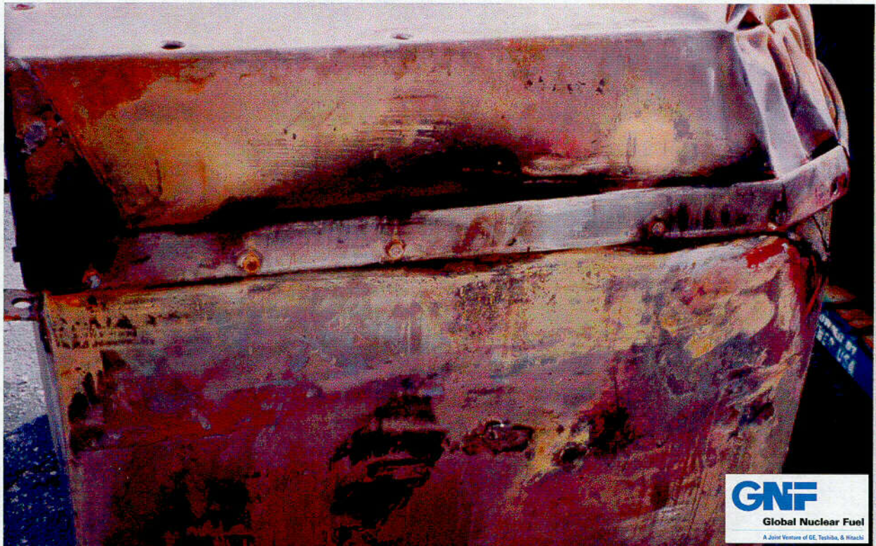
Figure 2.10.1-68 – CTU-3 Post-Test Disassembly; Overall View of Test Unit
