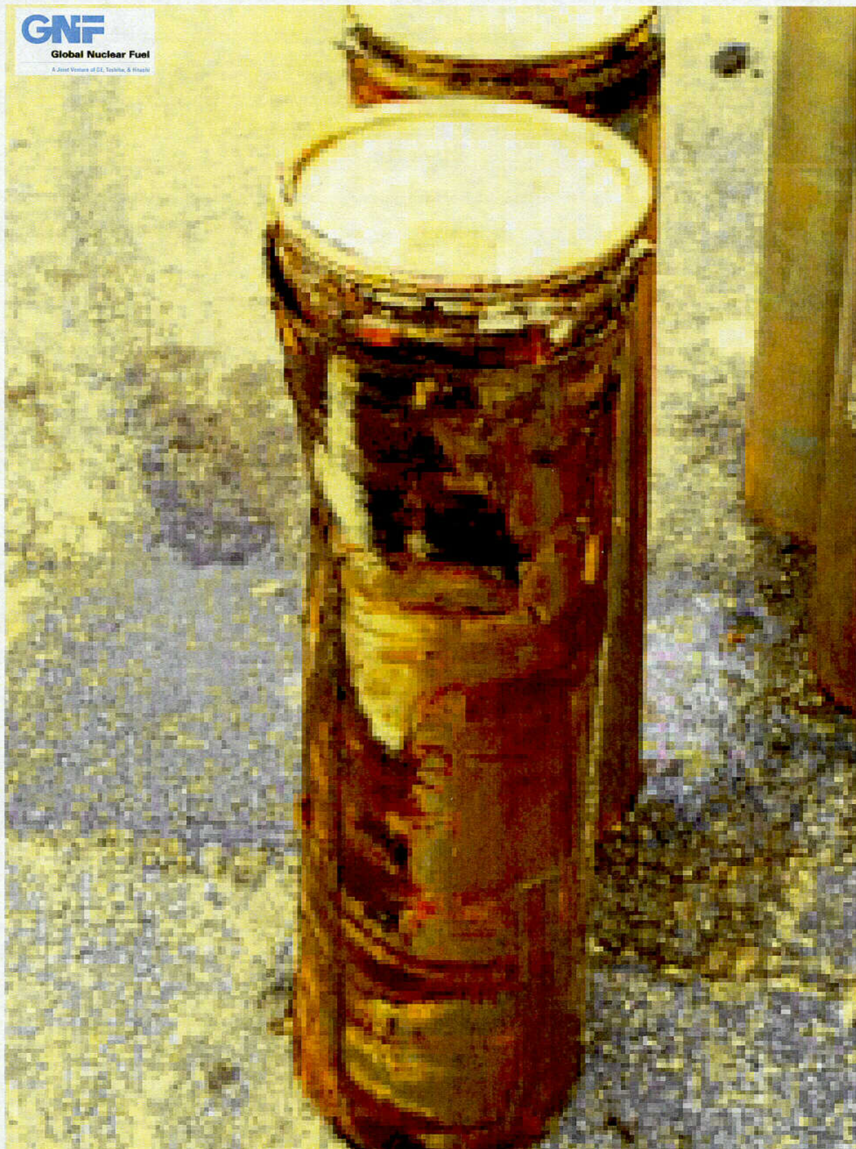
Figure 2.10.1-51 – CTU-2 Post-Test Disassembly; View of Damage to ICCA Closest to Impact
