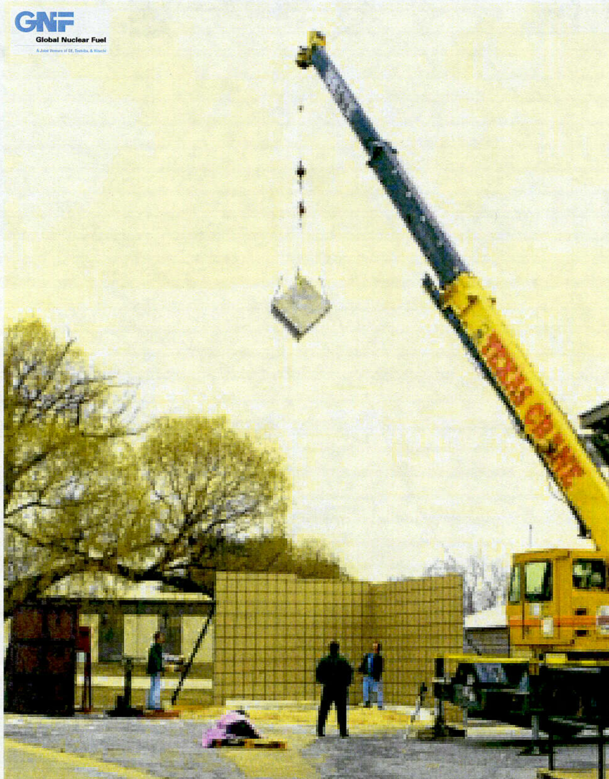
Figure 2.10.1-35 - CTU-2 Free Drop Test No. 4; HAC Drop on Side Edge
