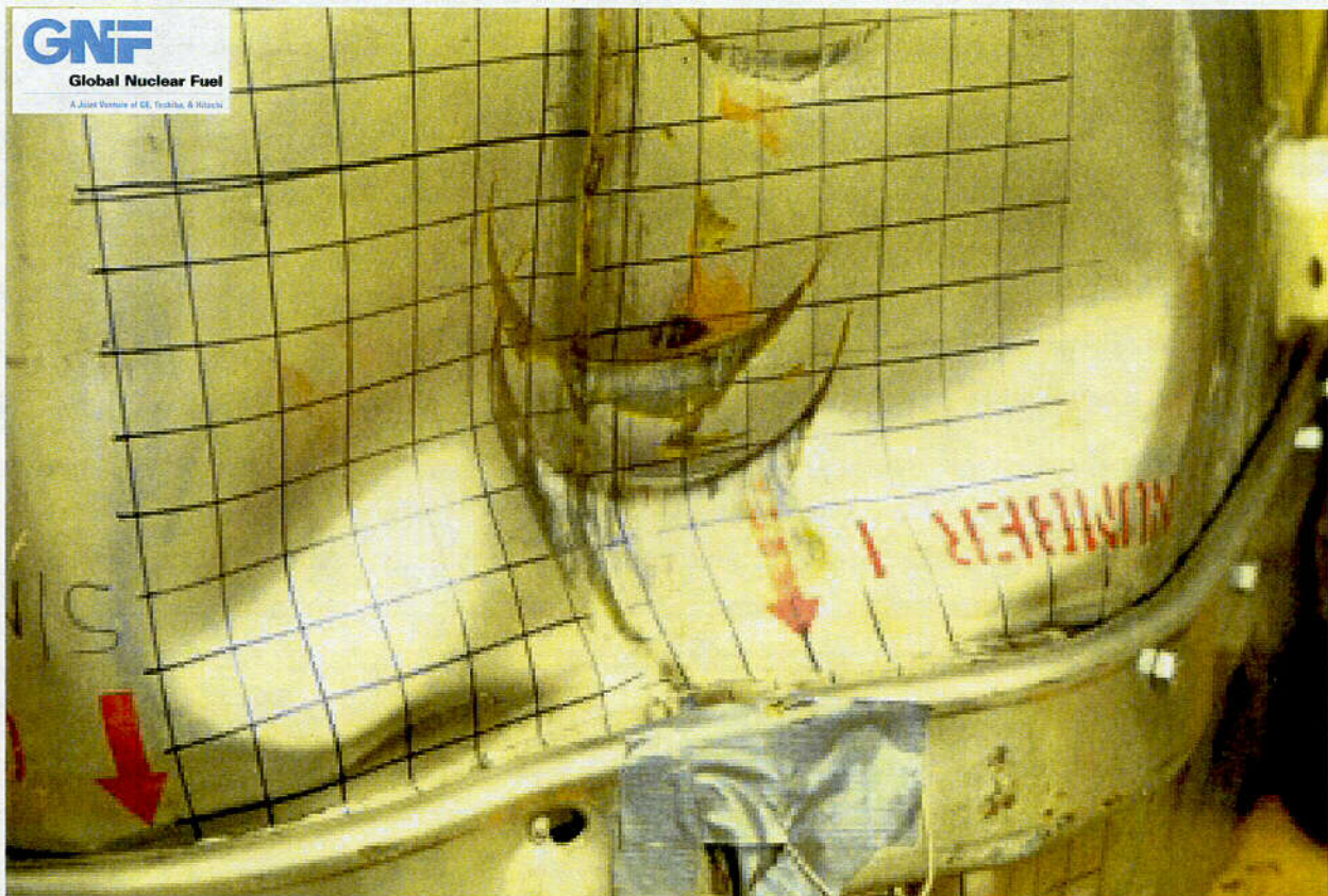
Figure 2.10.1-42 – CTU-2 Puncture Drop Test No. 9B; Close-up View of Damage
