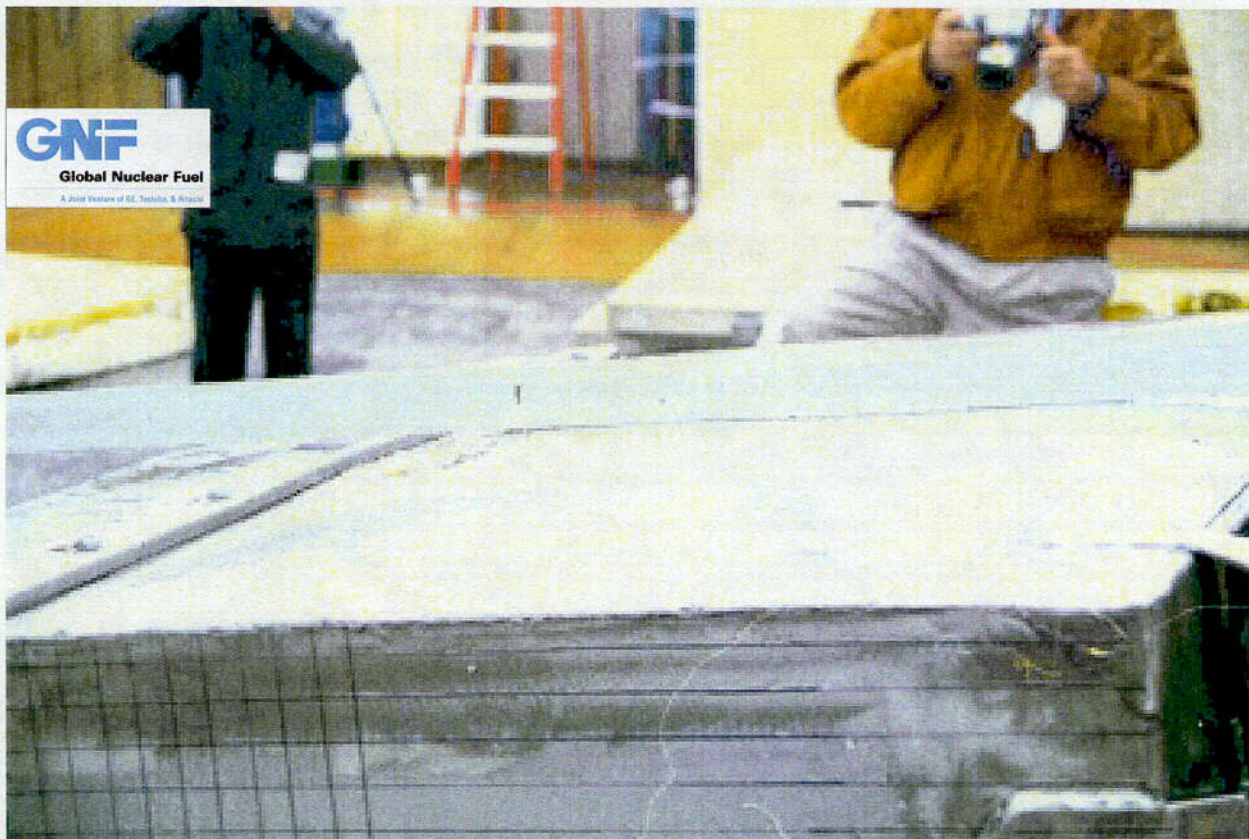
Figure 2.10.1-79 – CTU-4 Free Drop Test No. 6; View of Damage
