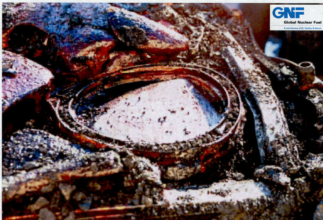
Figure 2.10.1-74 – CTU-3 Post-Test Disassembly; Close-up View of Damaged ICCA Closure Lid
