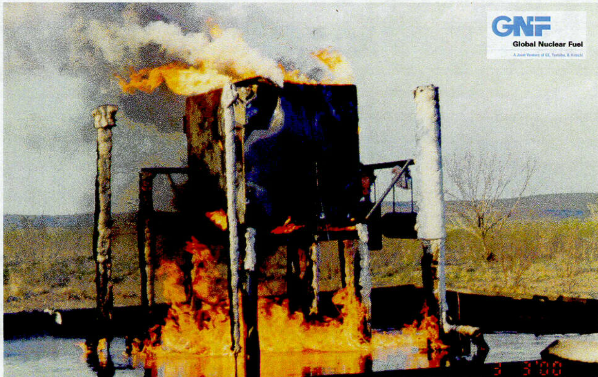
Figure 2.10.1-20 - CTU-1 Fire Test No. 15; View ~35 Minutes after Start
