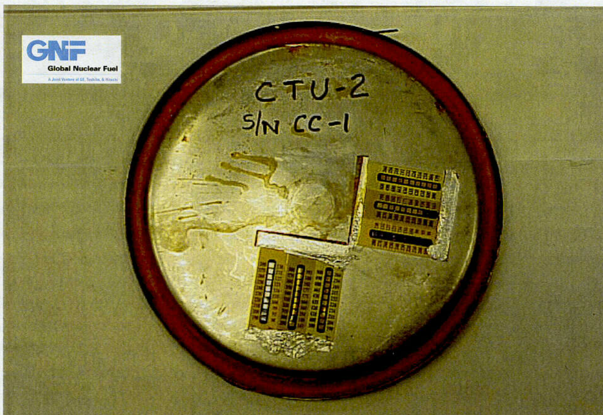
Figure 2.10.1-52 – CTU-2 Post-Test Disassembly; View of ICCA Closure Lid
