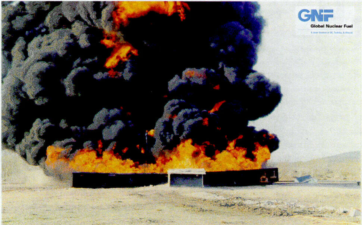
Figure 2.10.1-18 – CTU-1 Fire Test No. 15; Overall View ~3 Minutes after Start
