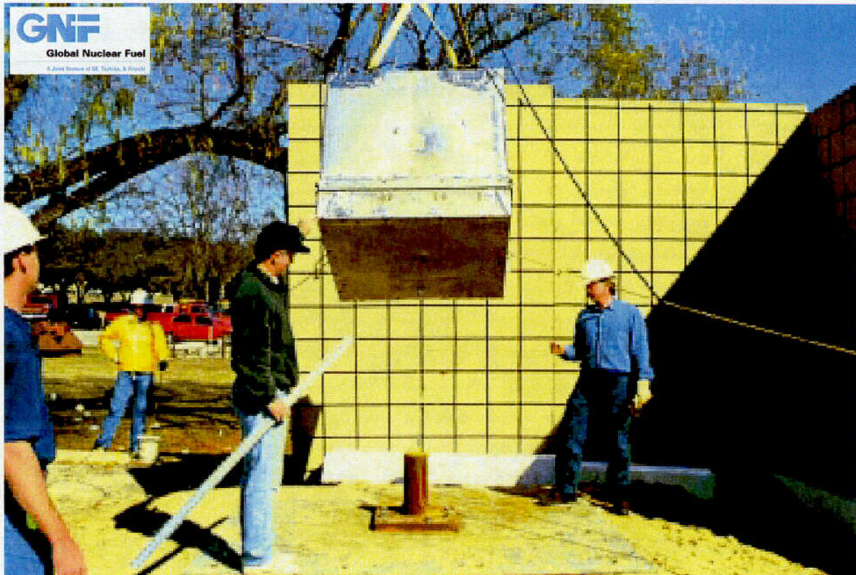
Figure 2.10.1-92 – CTU-4 Puncture Drop Test No. 14; HAC Oblique Puncture on OCA Lid
