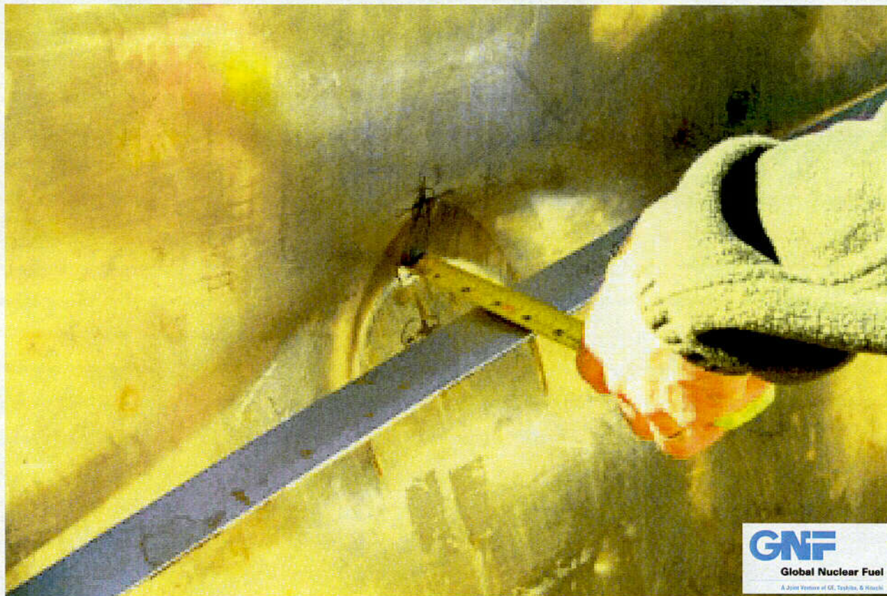
Figure 2.10.1-93 – CTU-4 Puncture Drop Test No. 14; Close-up of Damage; ~2½" Deep
