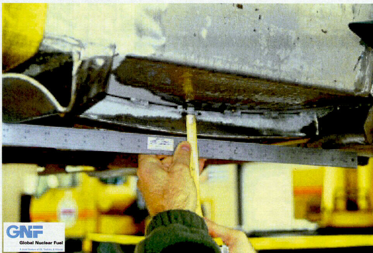
Figure 2.10.1-86 – CTU-4 Free Drop Test No. 8; Close-up View of Damage; ~1½" Deep
