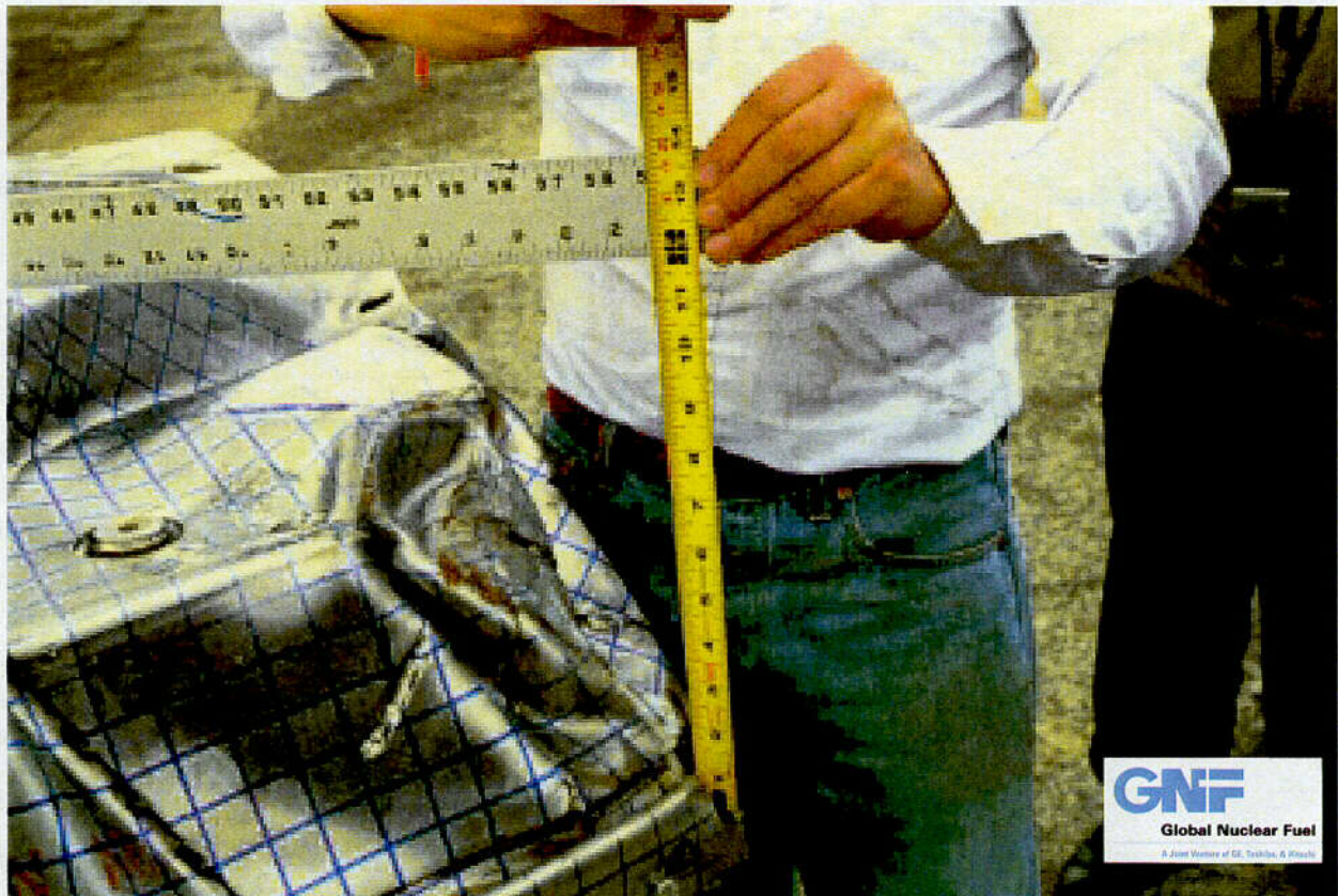
Figure 2.10.1-14 - CTU-1 Free Drop Test No. 2; Overall Vertical Deformation of OCA Lid Corner
