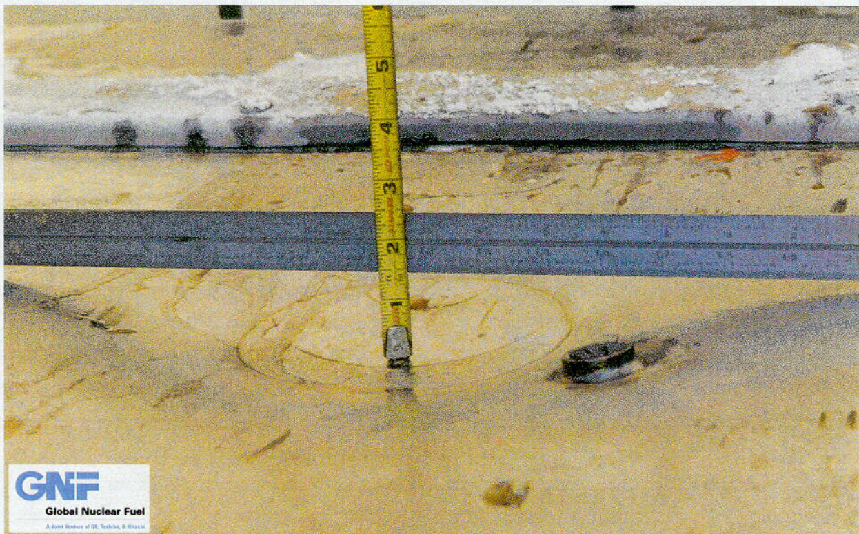
Figure 2.10.1-88 – CTU-4 Puncture Drop Test No. 12; Close-up View of Damage; ~1½" Deep
