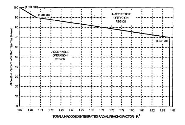
Note: The  $F_r^T$  limit should be reduced for reactor coolant flow rates  $\ge$  349,200 gpm and < 360,000 gpm (see Section 2.6).
