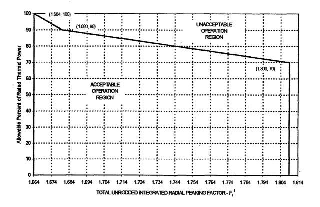
FIGURE 2.6-2 TOTAL UNRODDED INTEGRATED RADIAL PEAKING FACTOR vs. Allowable Rated Thermal Power For Reactor Coolant Flow Rates < 360,000 gpm and ≥ 354,600 gpm
