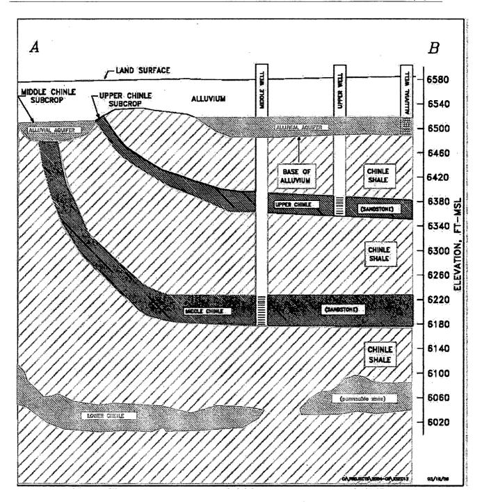
Figure 3 Typical Geologic Cross Section (Reproduced from Hydro-Engineering 2006)
