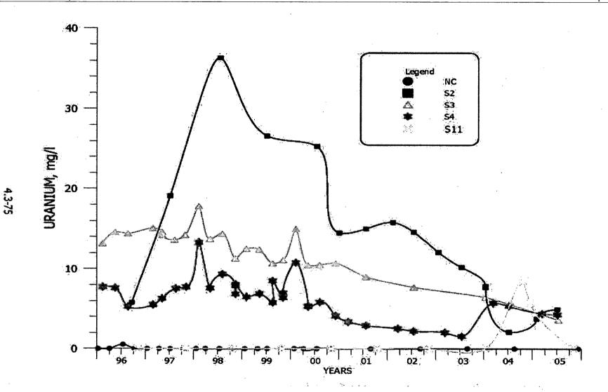
Figure 11 Uranium Concentration for POC Well S4 (Reproduced from Hydro-Engineering 2006)
