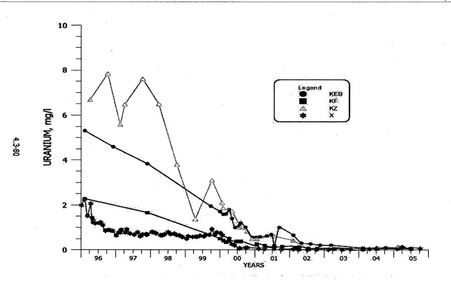
Figure 13 Uranium Concentration for POC Well X (Reproduced from Hydro-Engineering 2006)
