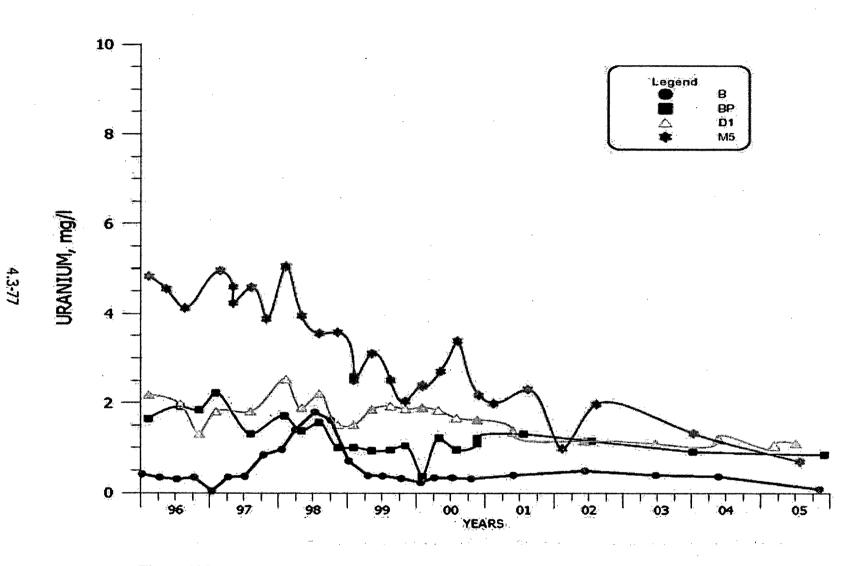
Figure 12 Uranium Concentration for POC Well D1 (Reproduced from Hydro-Engineering 2006)
