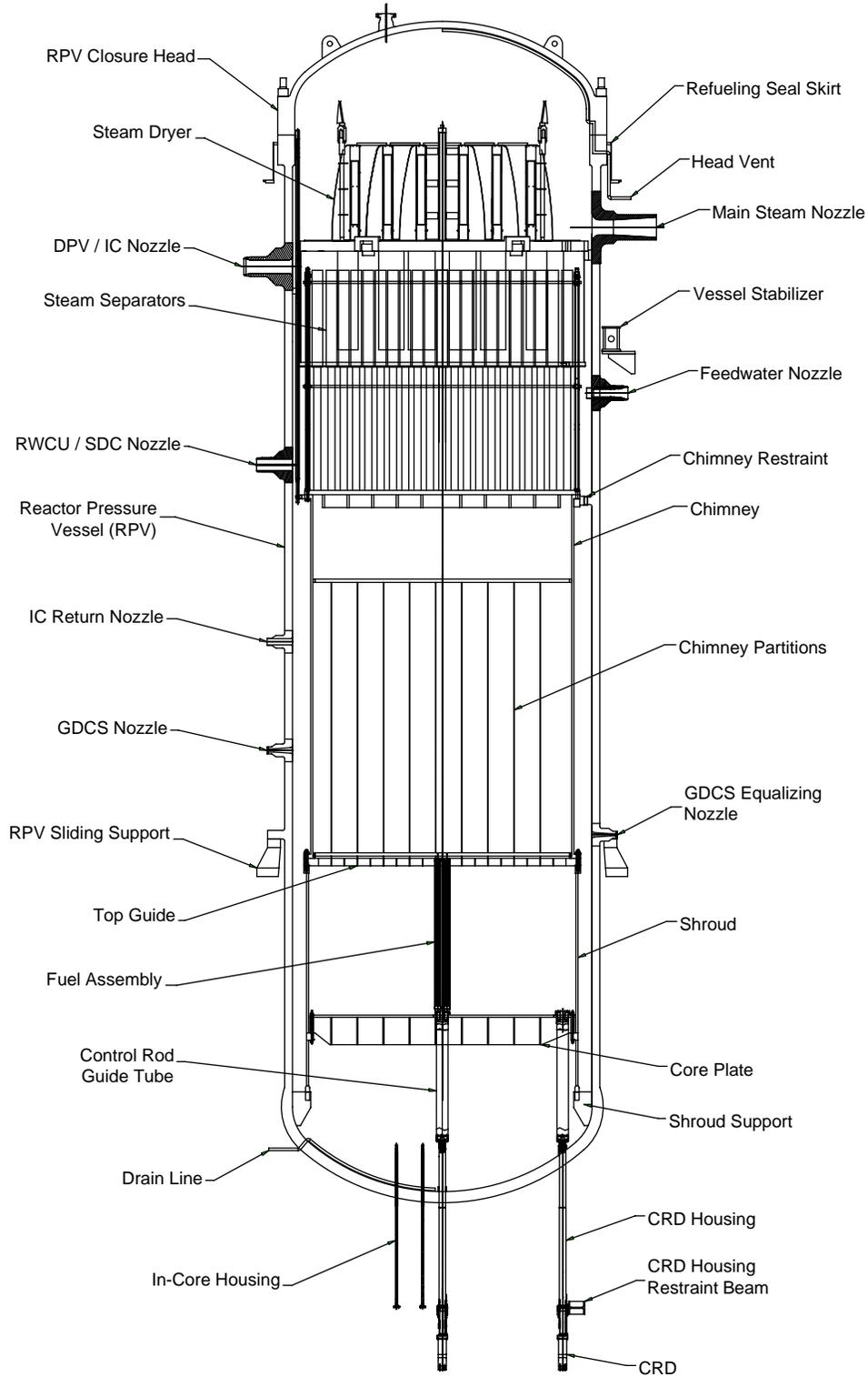
Figure 5.3-3. Reactor Pressure Vessel System Key Features
