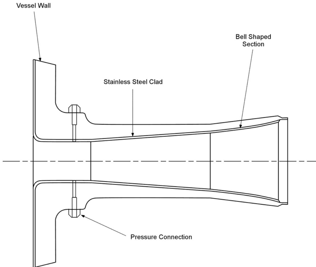
Figure 5.4-1. Main Steamline Nozzle and Flow Restrictor
