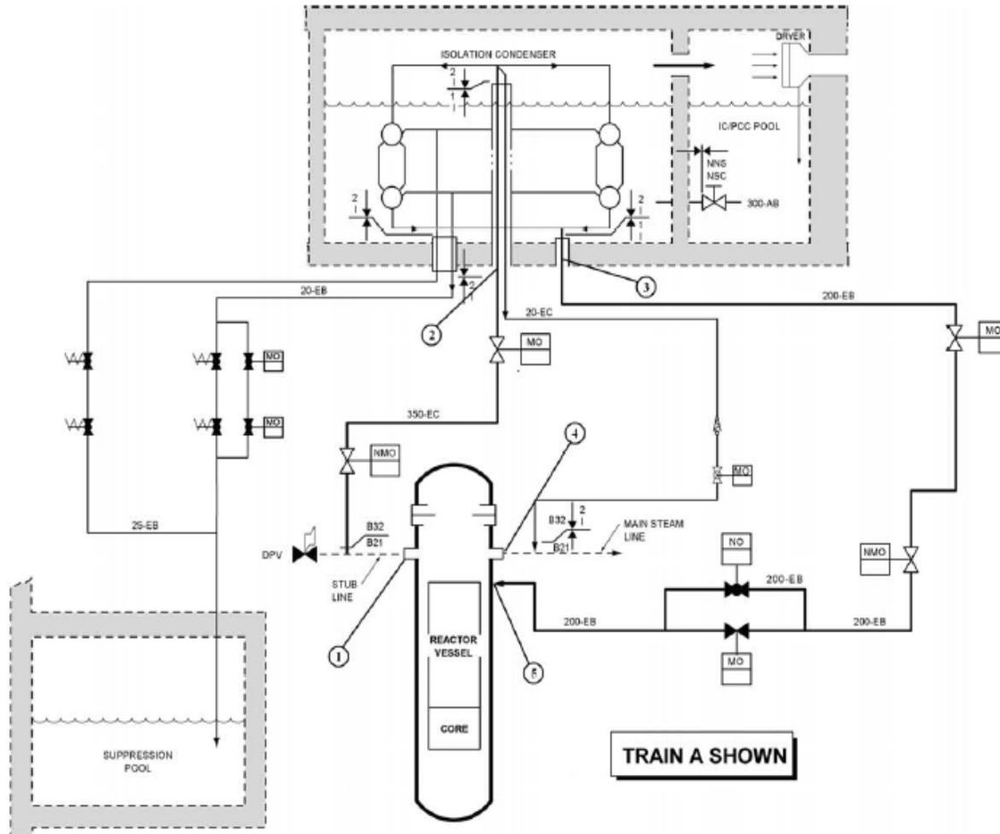
Figure 5.4-4. Isolation Condenser System Simplified Process Diagram
