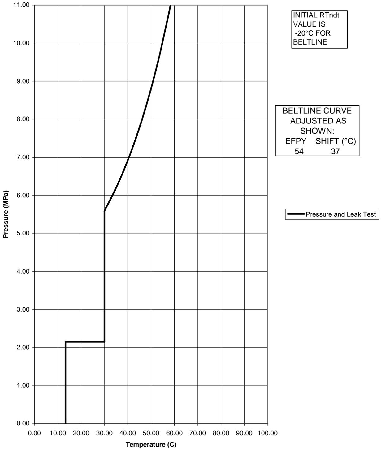
Figure 5.3-1. Minimum Temperatures Required Versus Reactor Pressure for Hydrotest — Core Not Critical (Representative curve for the ESBWR)
