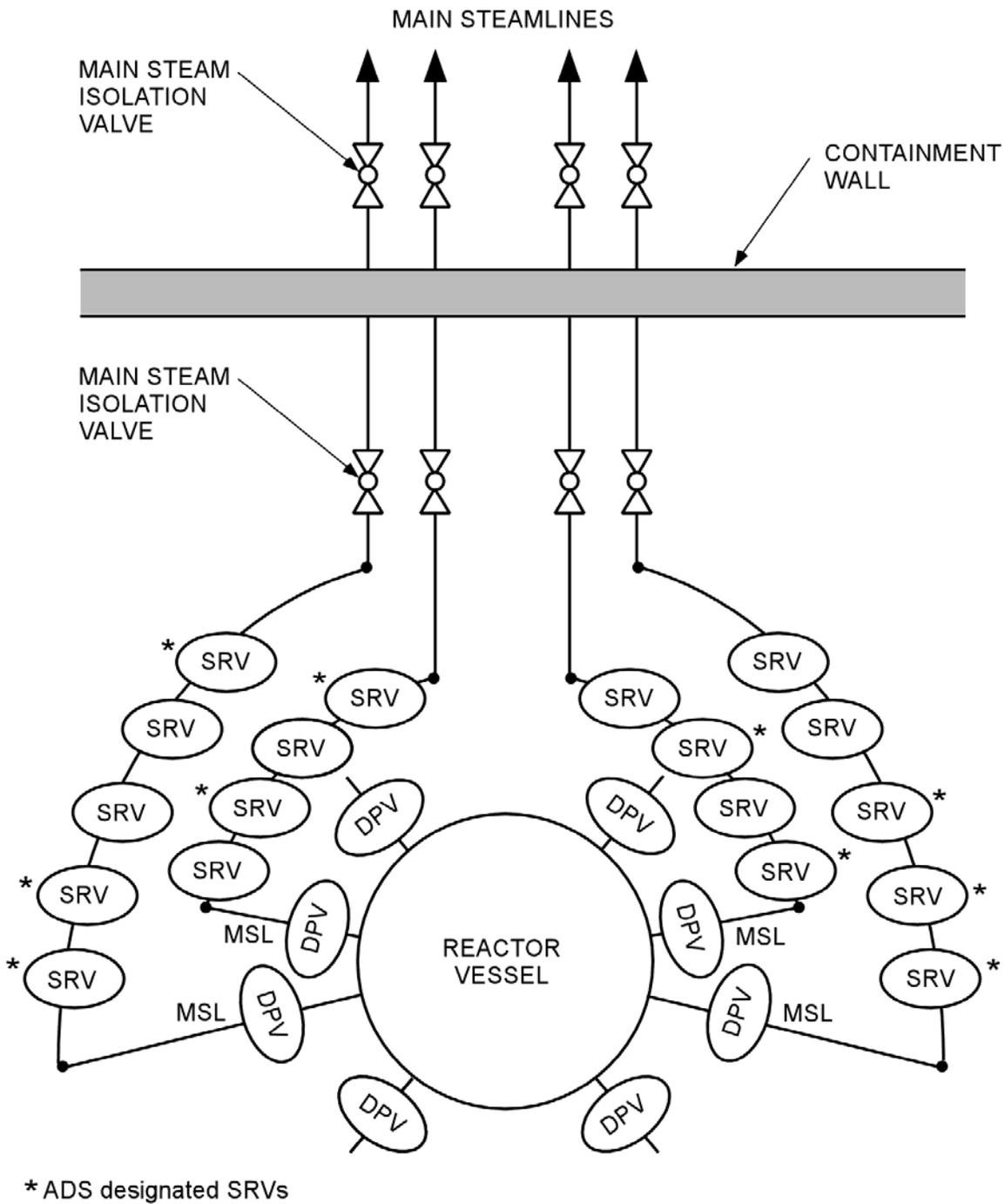
Figure 5.2-2. Safety-Relief Valves, Depressurization Valves and Steamline Diagram
