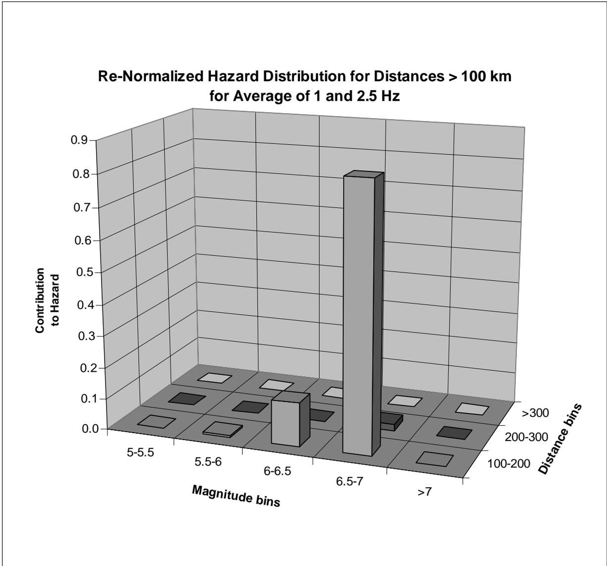
**Figure D.5. Renormalized Hazard Distribution for Distances > 100 km for Average of 1 and 2.5 Hz**
