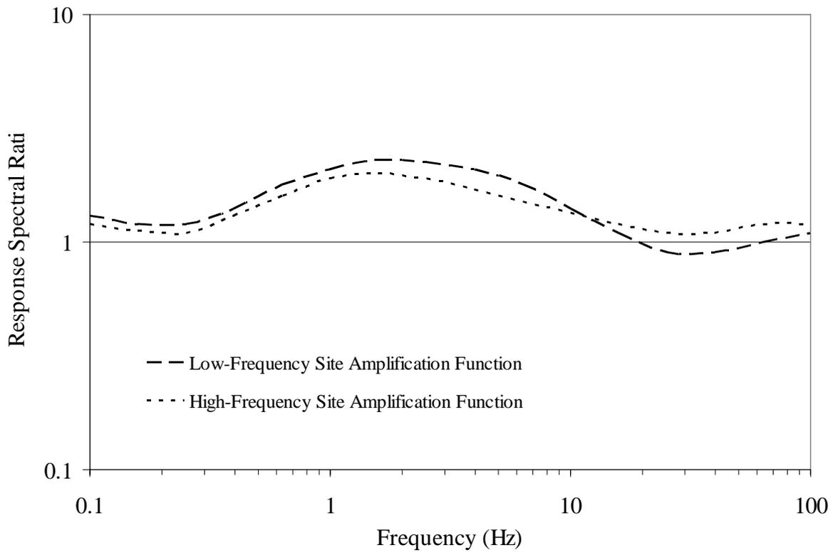
**Figure E.2. Mean Site Amplification Functions for Low- and High-Frequency Characteristic Earthquakes for 1 E-05 Annual Probability Level**
