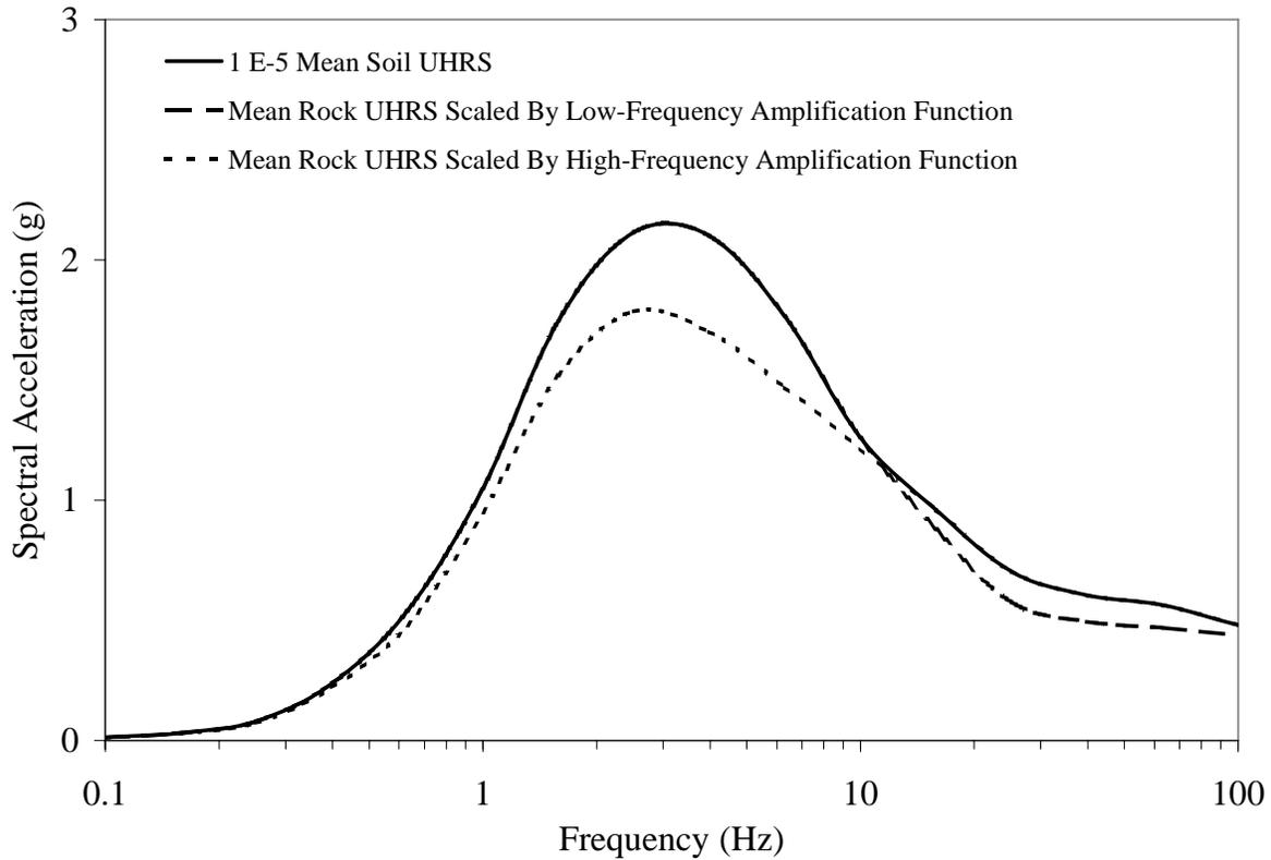
**Figure E.3. Free-Surface Soil Uniform Hazard Response Spectra Compared to Spectra Resulting from Scaling of Mean Rock UHRS by Low- and High-Frequency Amplification Functions**
