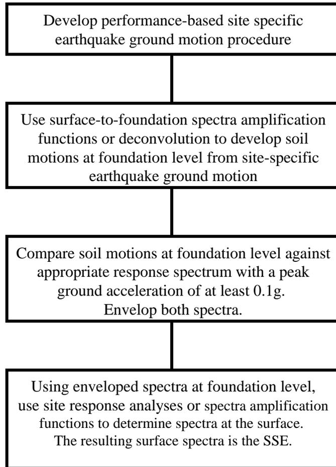
**Figure 3. Possible Development Methodology of Safe Shutdown Earthquake**
