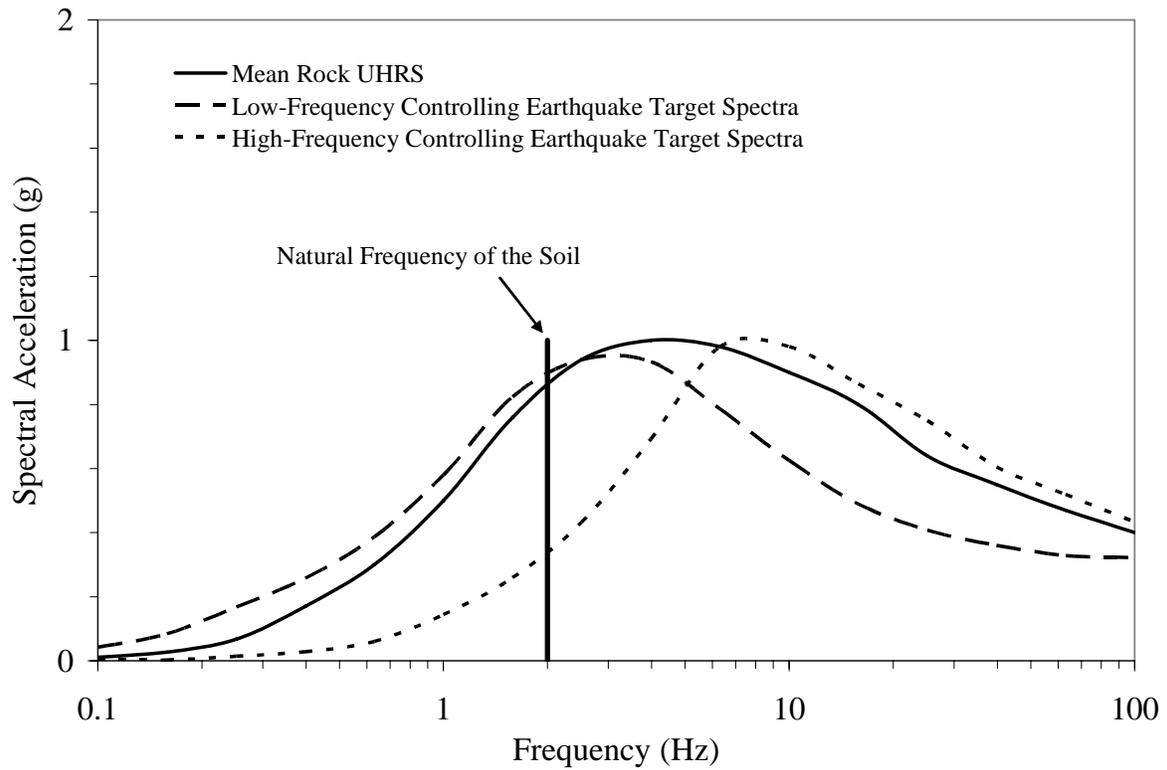
**Figure E.1. Comparison of the 1 E-05 Rock UHRS, the Target Spectra for the High- and Low-Frequency Controlling Earthquakes, and the Natural Frequency of the Soil Column**
