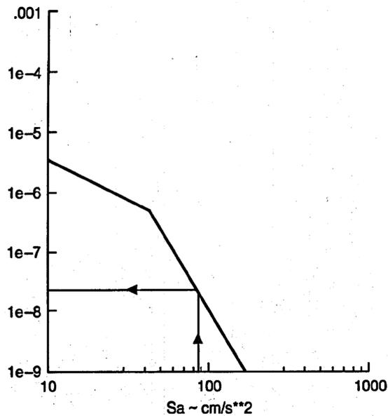
**Figure D.2. 1 Hz Mean Hazard Curve for Distance Bin 25 - 50 km & Magnitude Bin 6 - 6.5**
