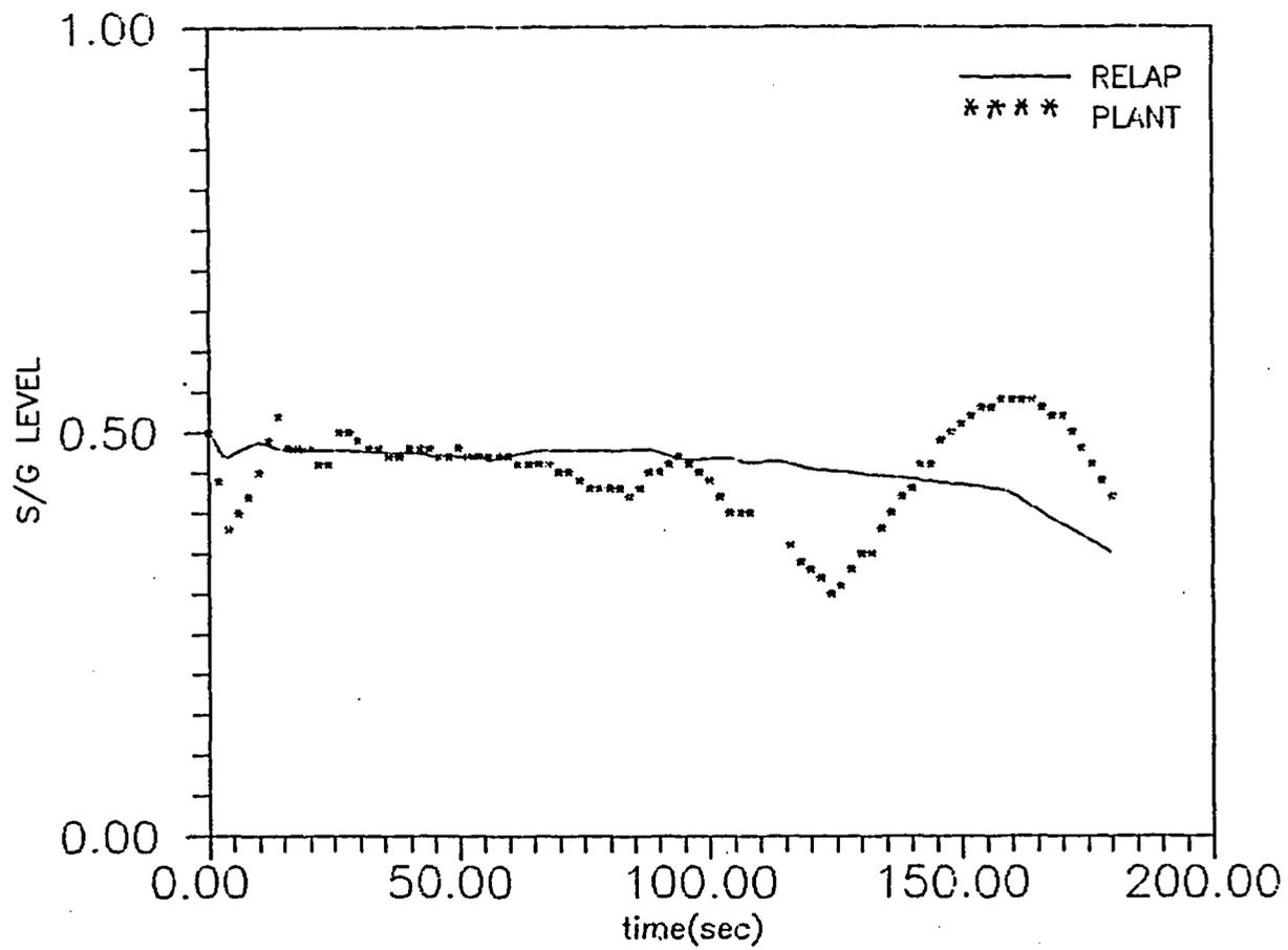
Figure 5.8 STEAM GENERATOR LEVEL
