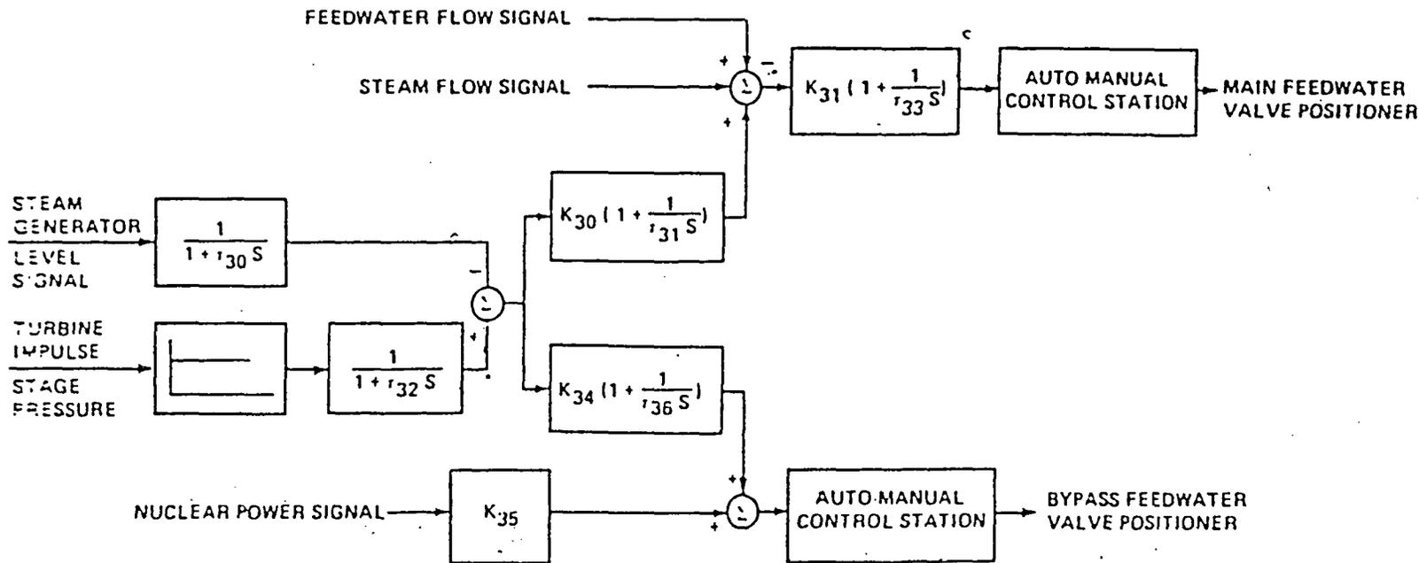
Figure 2-5 Functional Block Diagram of the Steam Generator Level Control System
