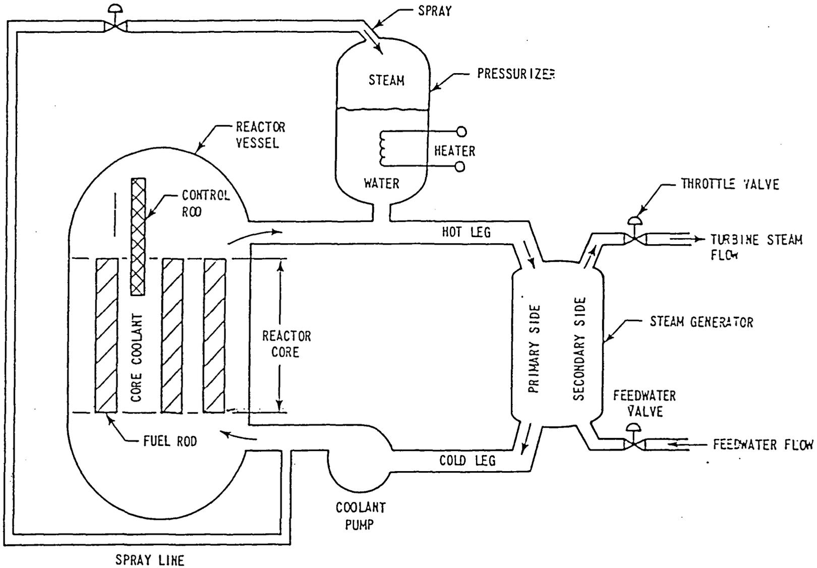
Figure 2-1. Pressurized Water Reactor Schematic Diagram
