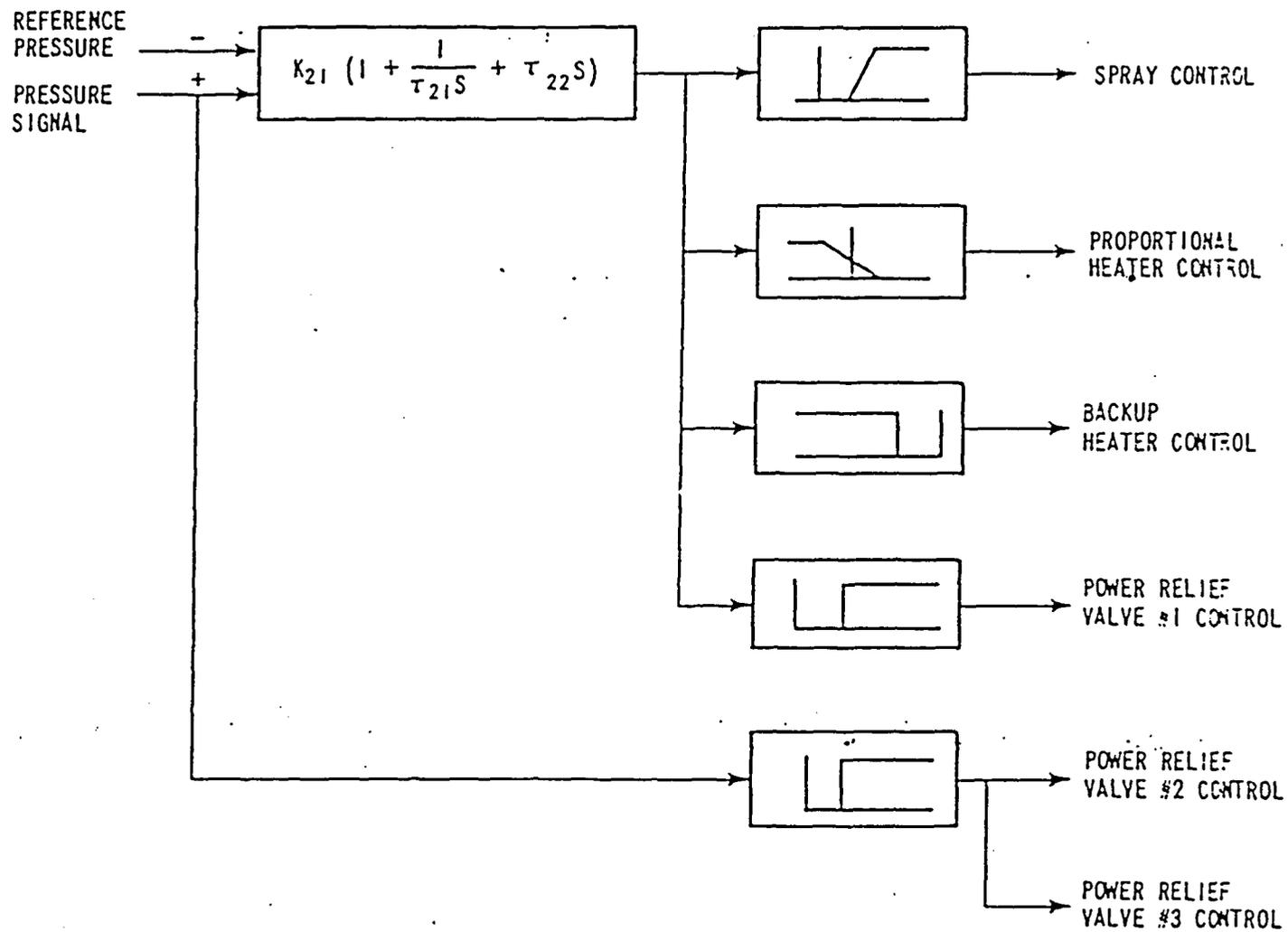
Figure 2-3 . Functional Block Diagram of the Pressurizer Pressure Control System
