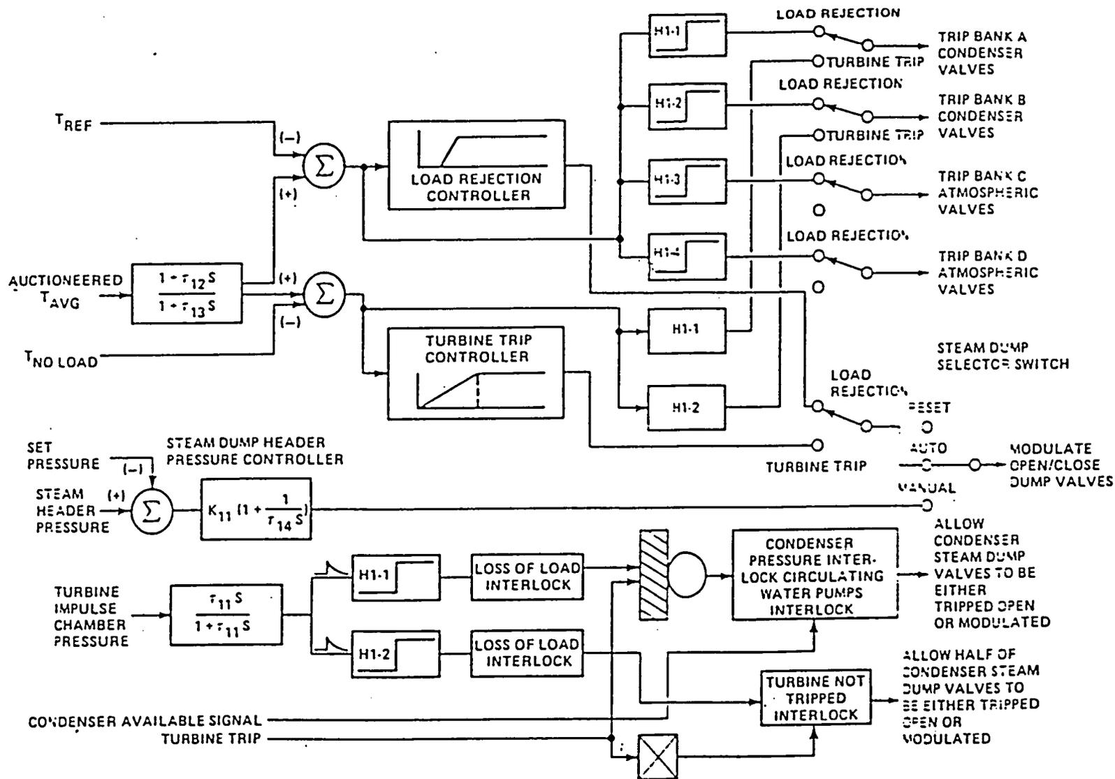
Figure 2.7 Functional Block Diagram of the Steam Dump Control System
