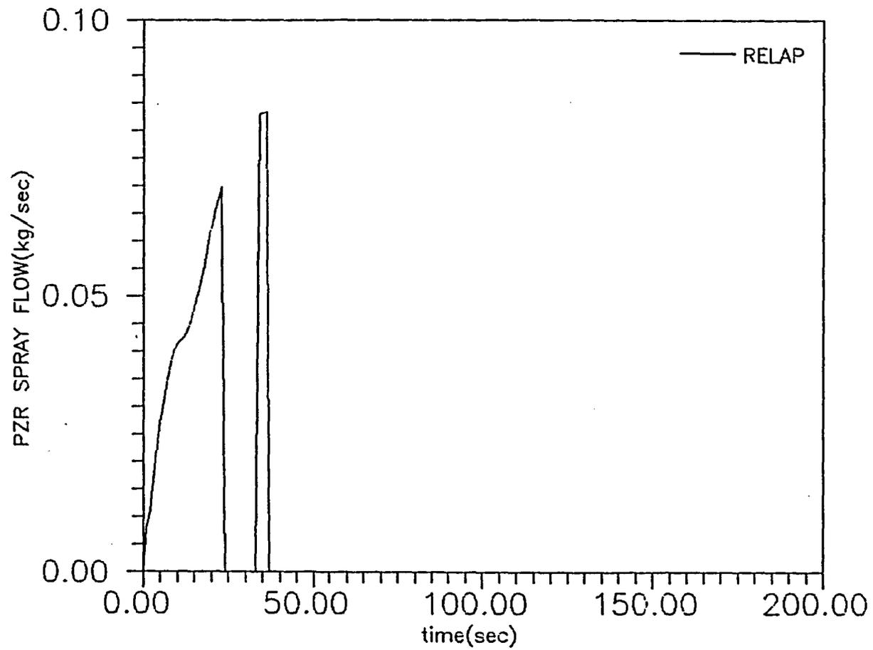
Figure 5.6 PRESSURIZER SPRAY FLOW (kg/sec)
