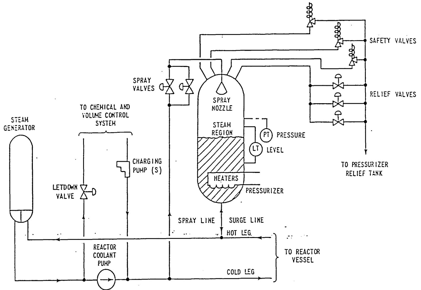
Figure 2-2. Pressurizer Pressure and Level Associated Equipment Arrangement
