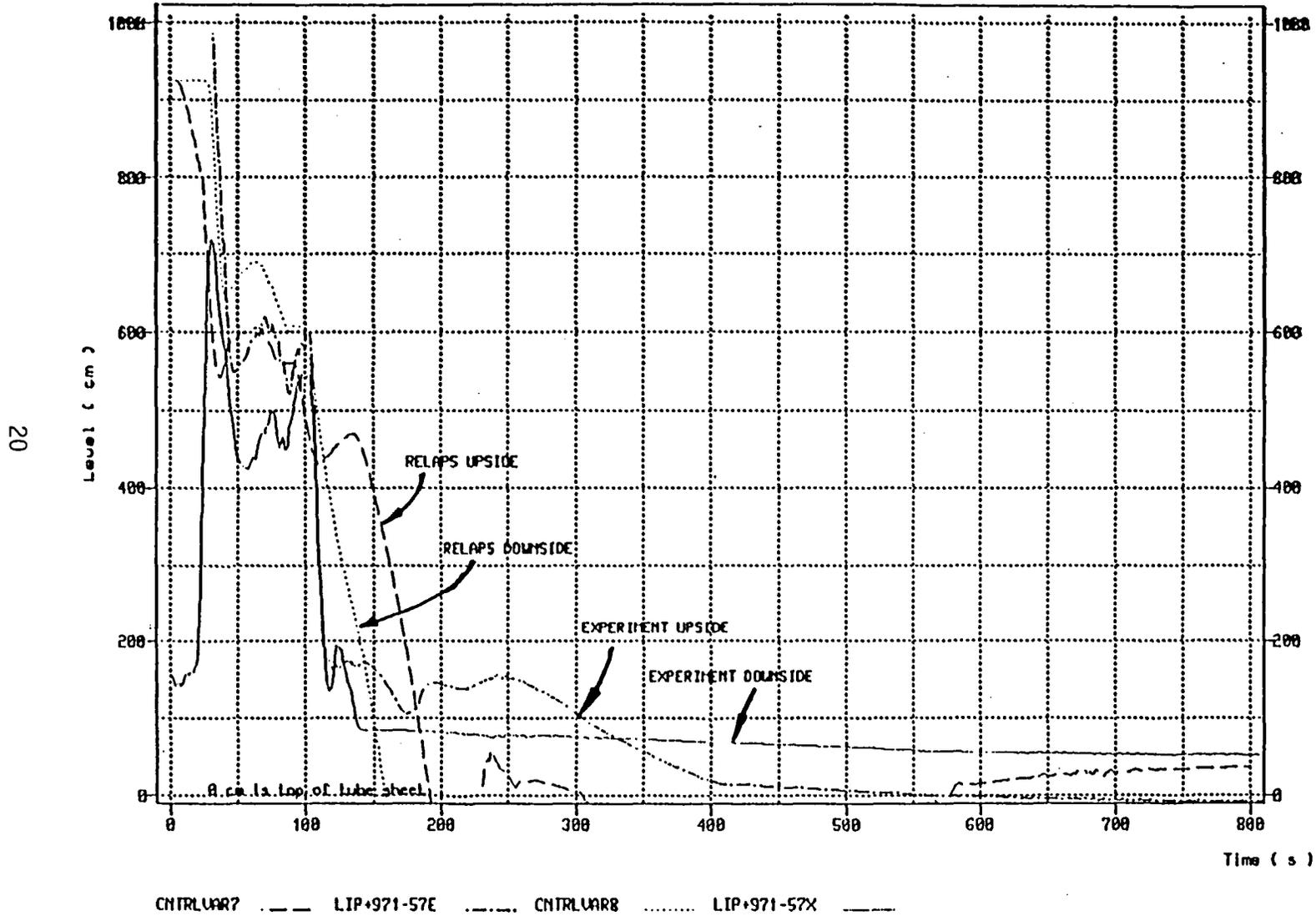
Figure 8. Collapsed Liquid Levels in Intact Loop U-tubes
