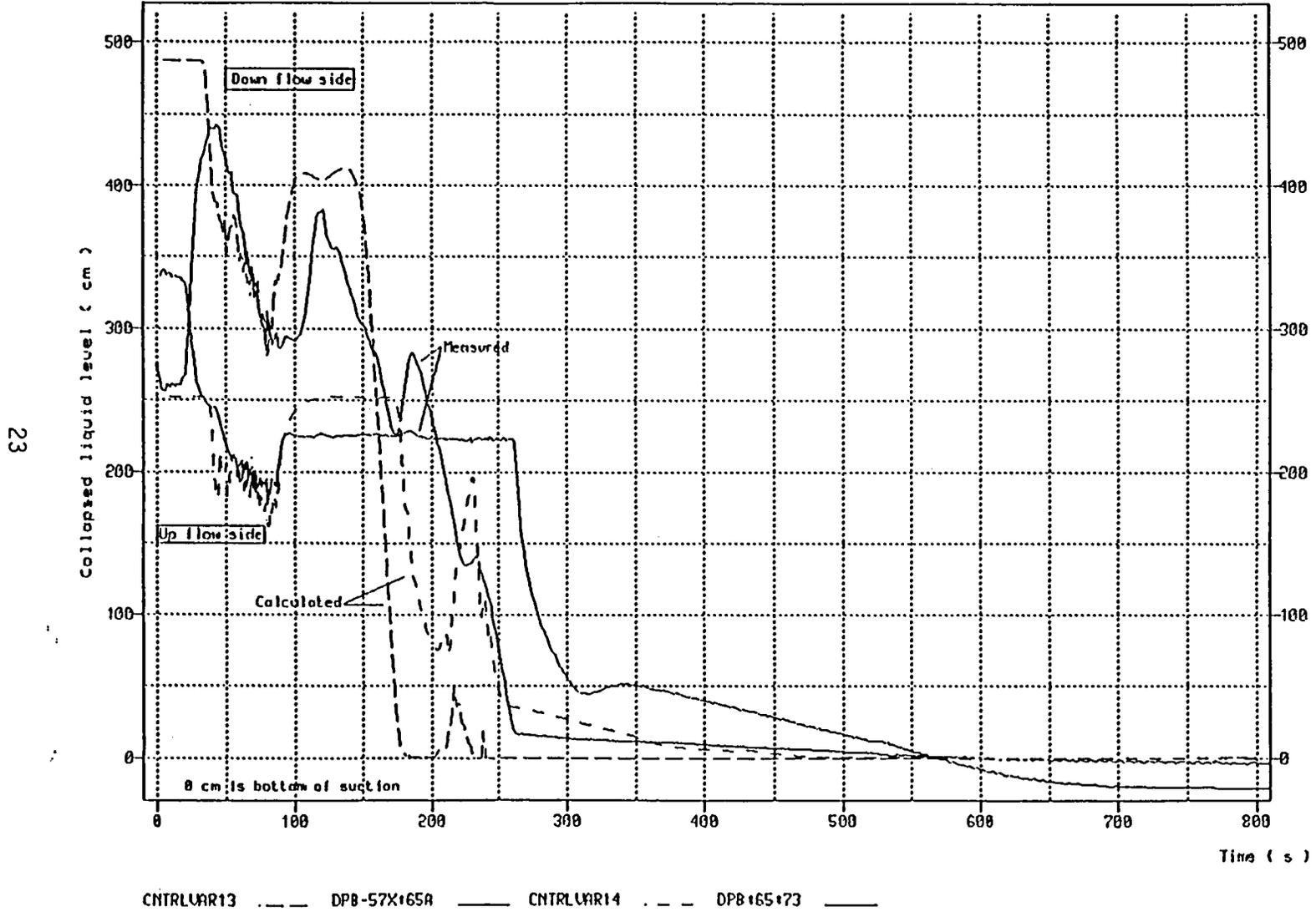
Figure 11: Measured and calculated BL pump suction collapsed liquid level
