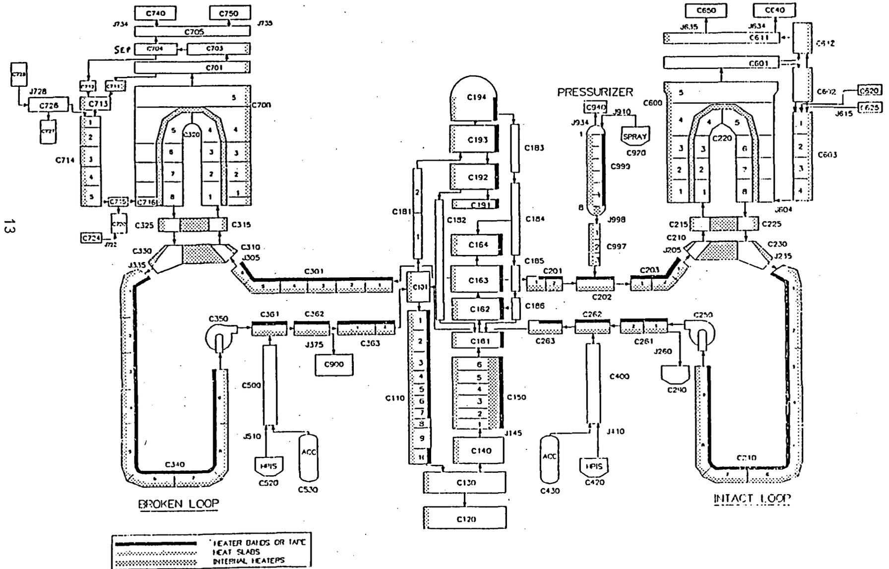
Figure 1: RELAP5 noding diagram for Semiscale S-LH-1 Calculation ( Base case )
