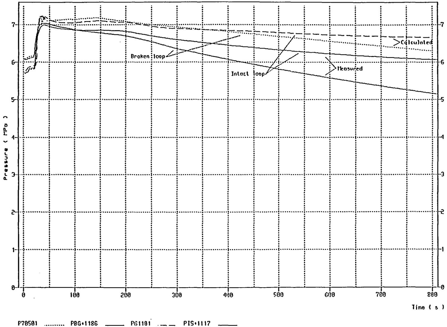
Figure 6 : Measured and calculated secondary pressures ( Base case )
