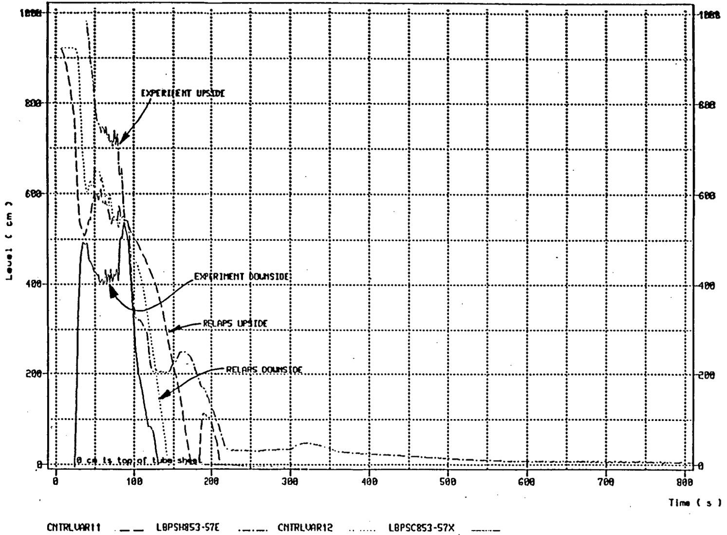
Figure 9. Collapsed Liquid Levels in Broken Loop U-tube
