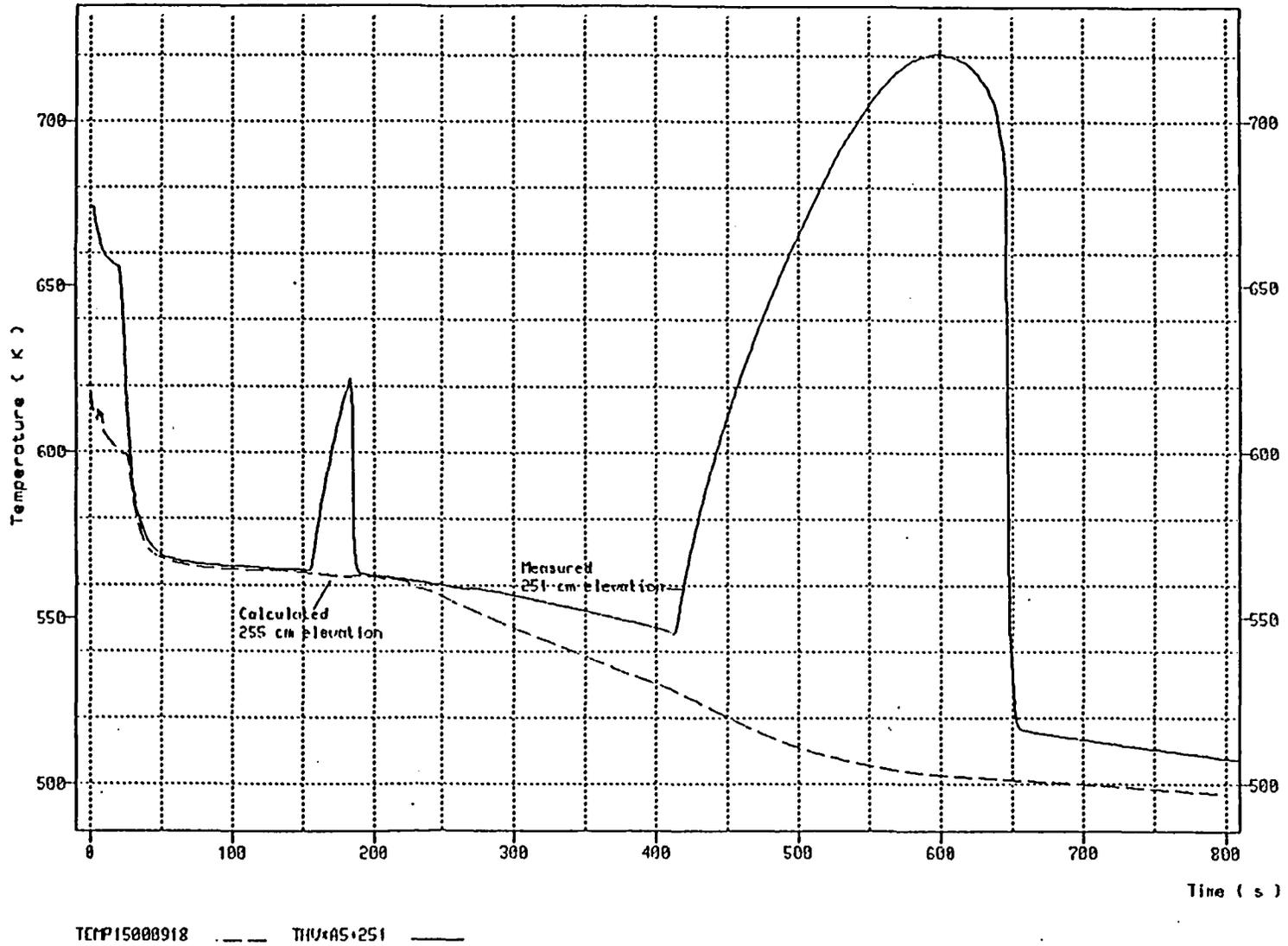
Figure 15 : Measured and calculated heater rod temperatures ( Base case )
