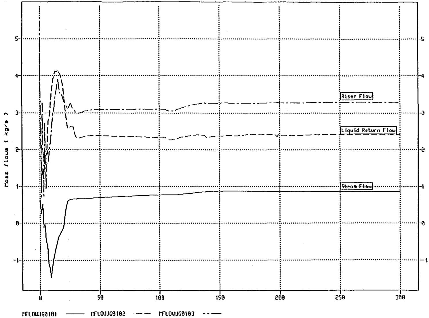
Figure 3 : Intact loop steam generator separator mass flow rates
