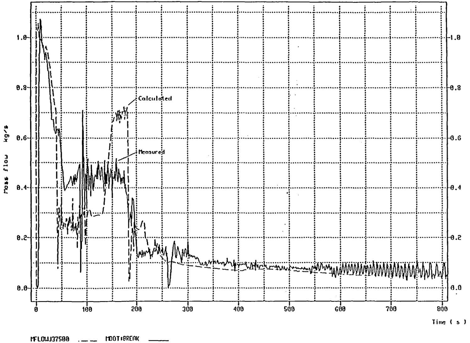
Figure 7 : Measured and calculated break flow ( Base case )
