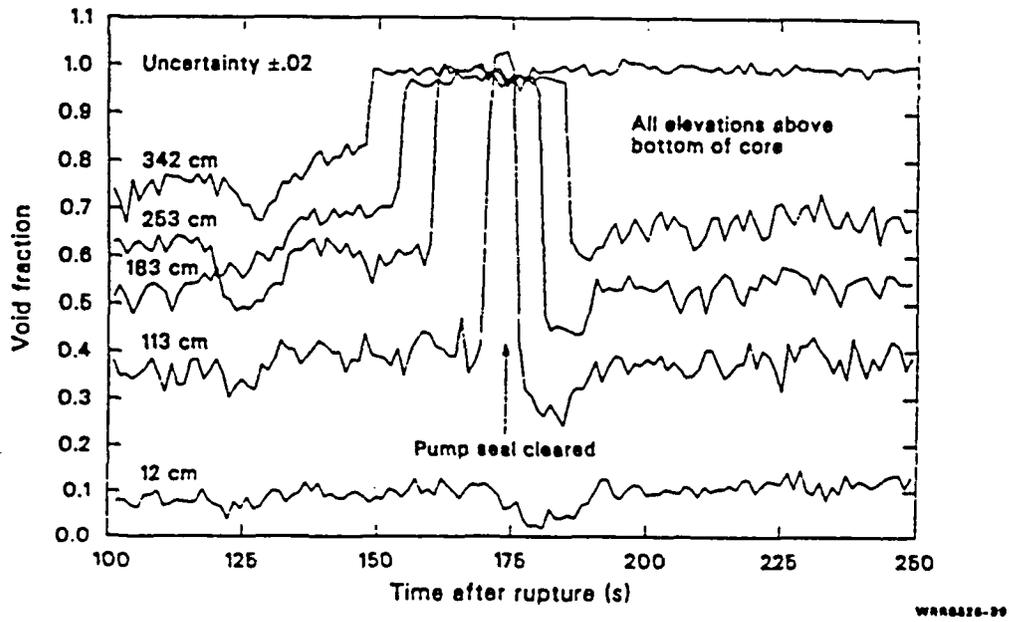
Figure 13a : Measured vessel axial void fraction distribution during the manometric depression
