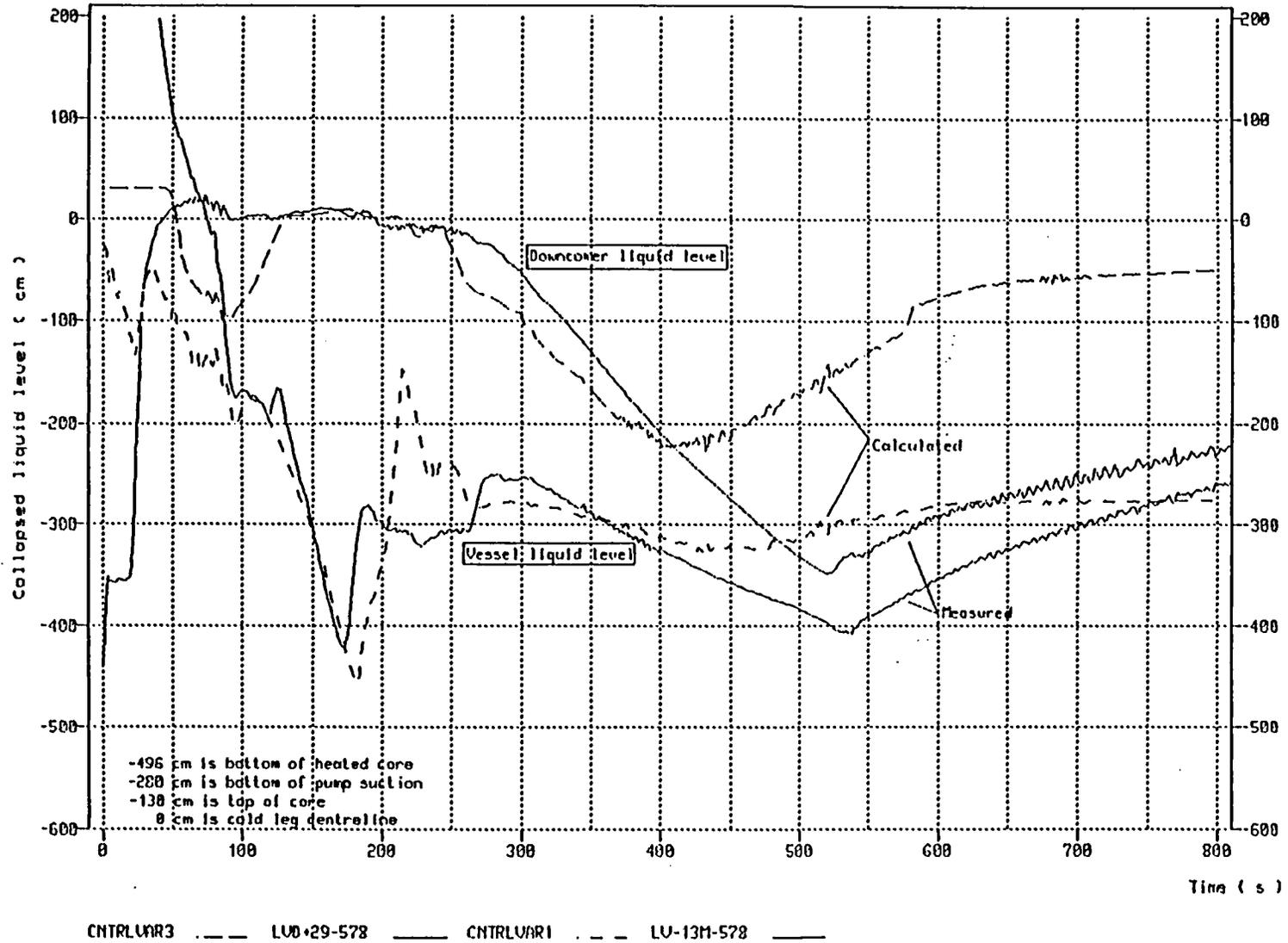
Figure 12 : Vessel and downcomer collapsed liquid levels ( Base case )
