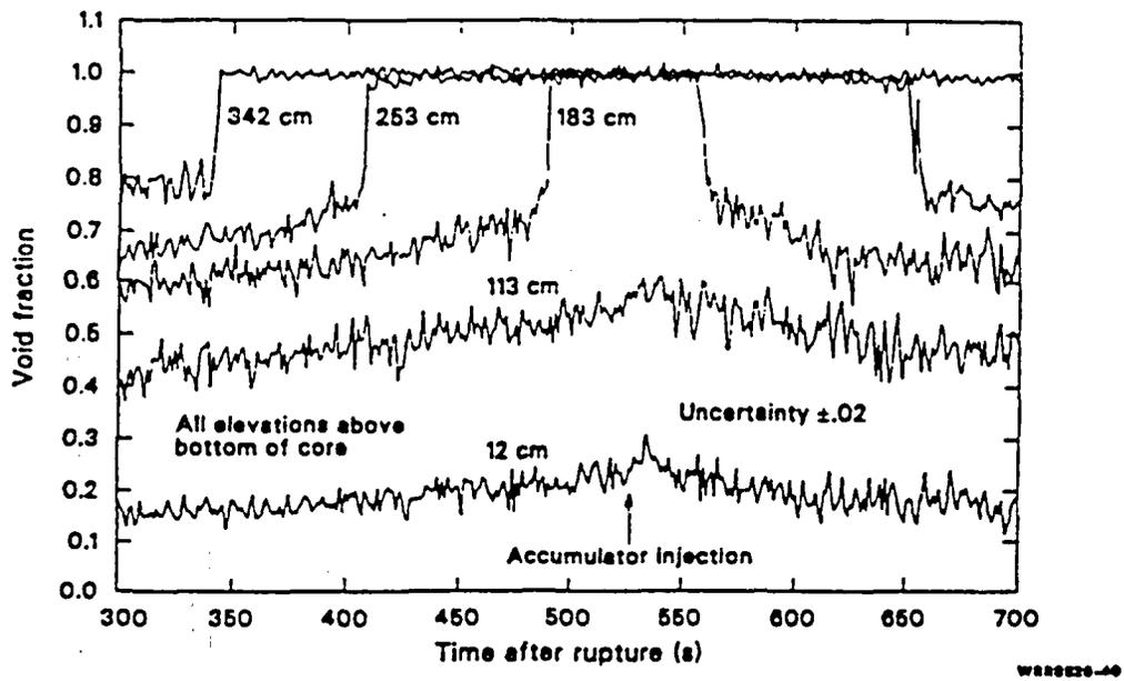
Figure 13b : Measured vessel axial void fraction distribution during core boildown
