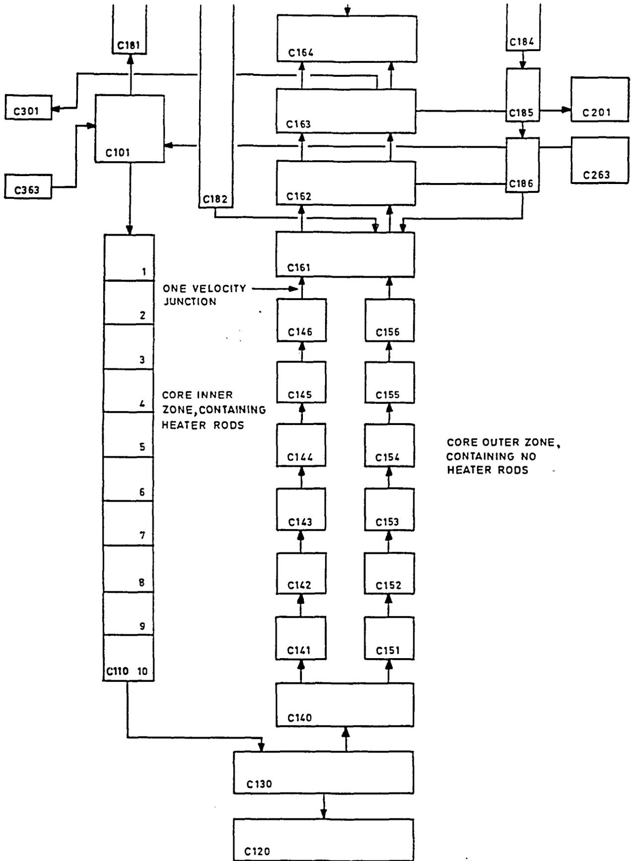
FIG.16 RENODALISATION OF THE CORE
