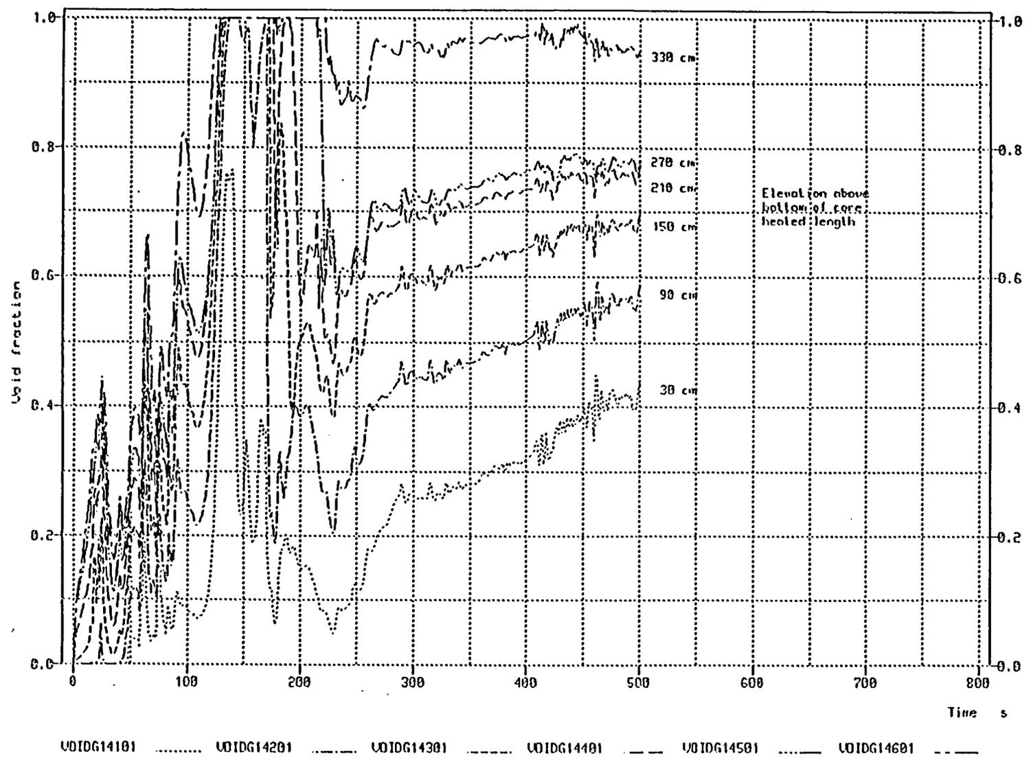
Figure 18 : Calculated core void fraction ( Sensitivity study )
