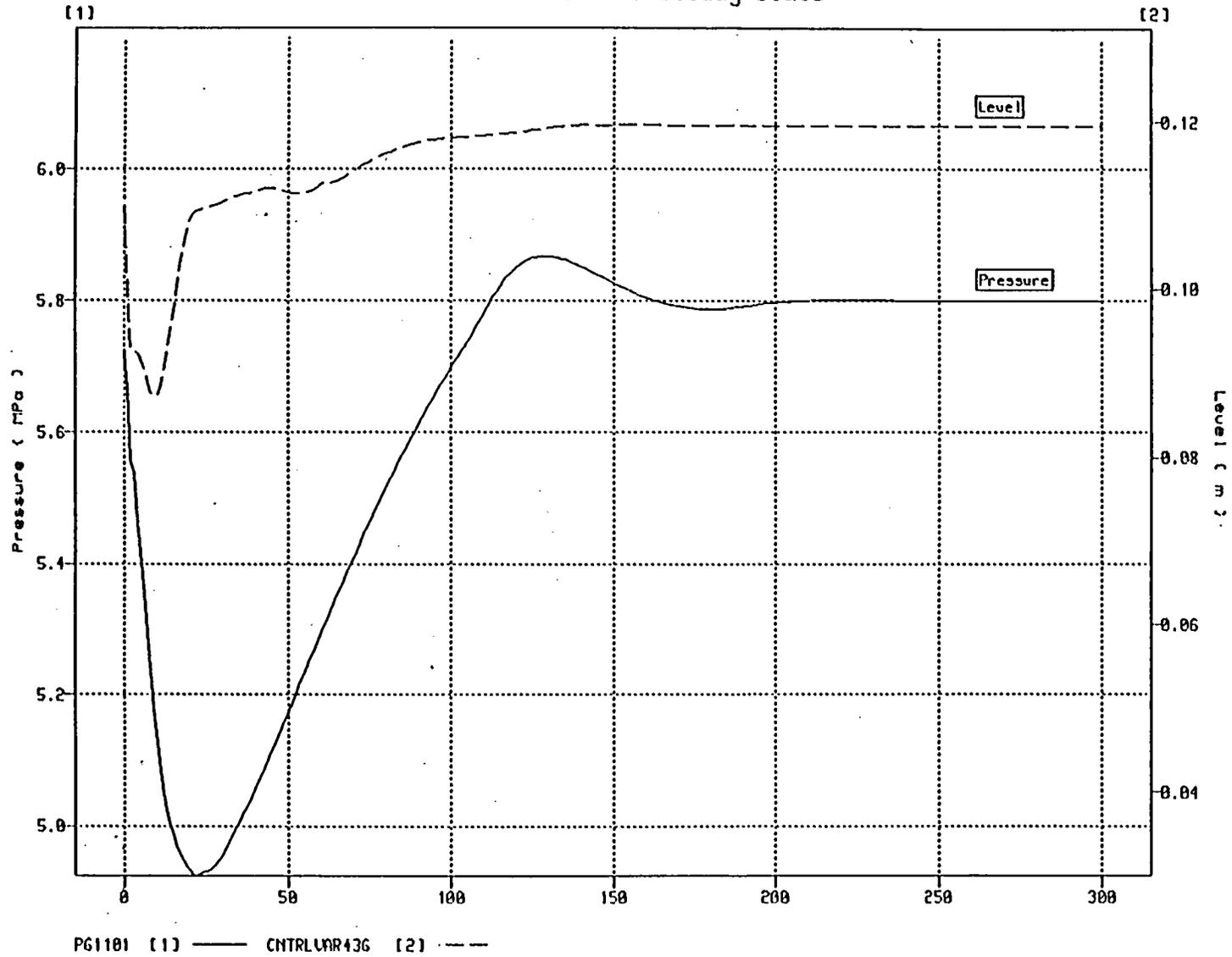
Figure 4 : Intact loop steam generator pressure and collapsed liquid level
