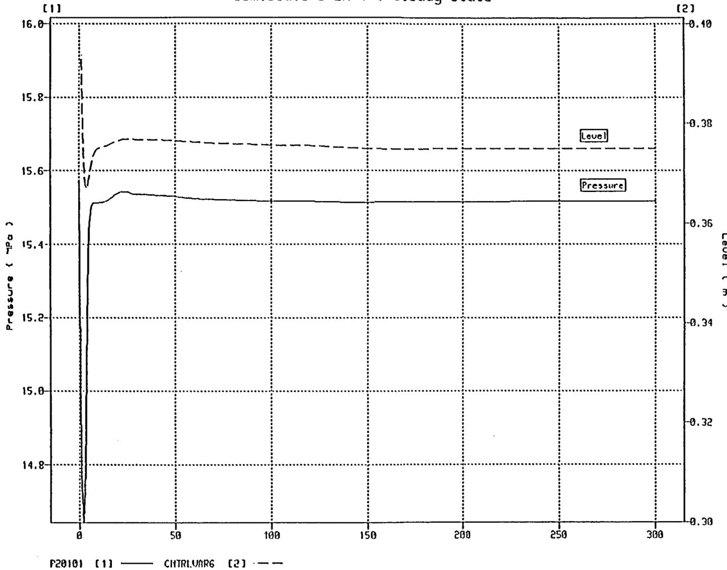
Figure 2 : Hot leg pressure and pressurizer level
