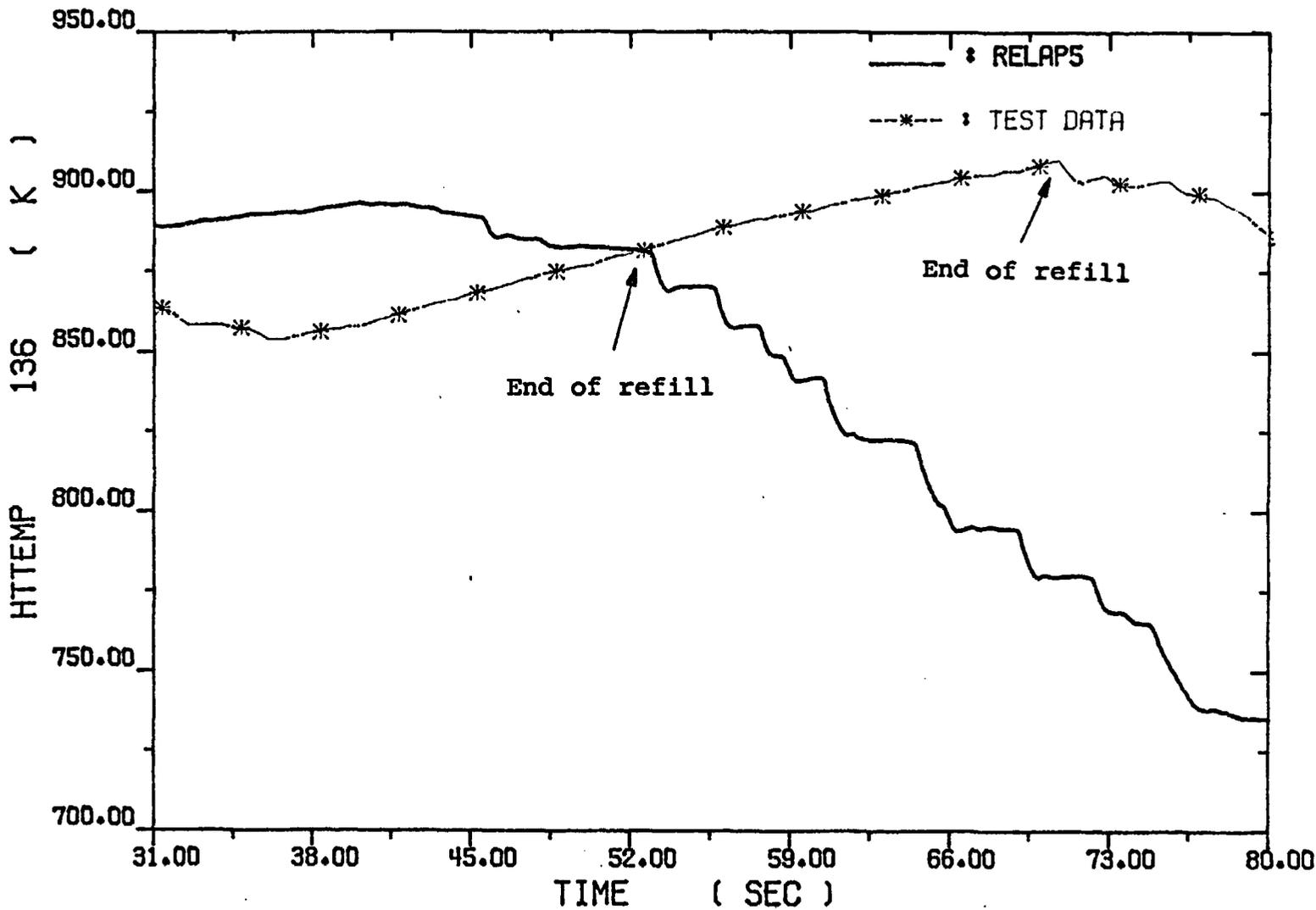
Fig. 4-22. Low Power Rod Hot Spot Cladding Temperatures
