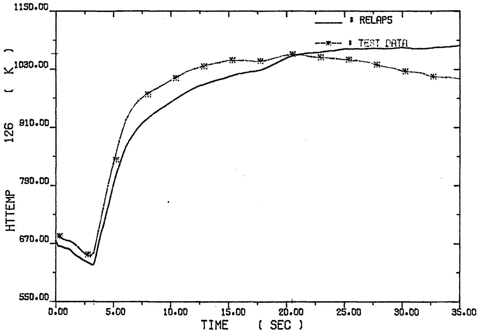
Fig. 4-13. High Power Rod Hot Spot Cladding Temperatures
