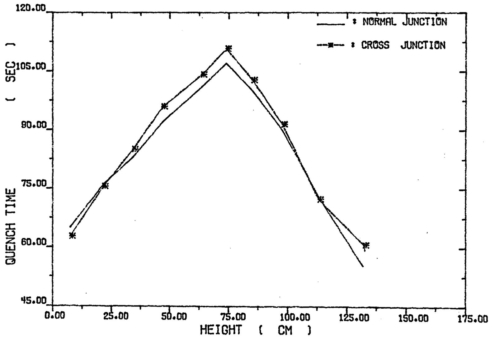
Fig. 4-69. High Power Rod Quench Time versus Elevation
