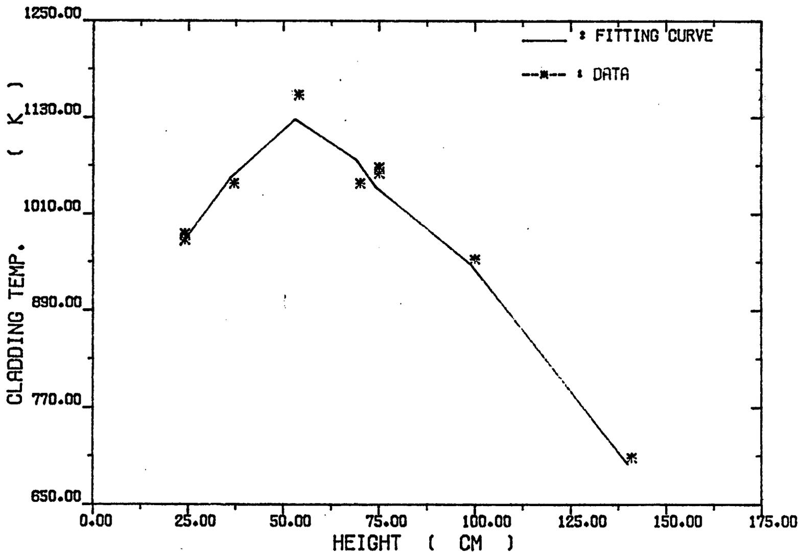
Fig. 4-33. Curve Fitting of The High Power Rod Peak Cladding Temperature versus Elevation
