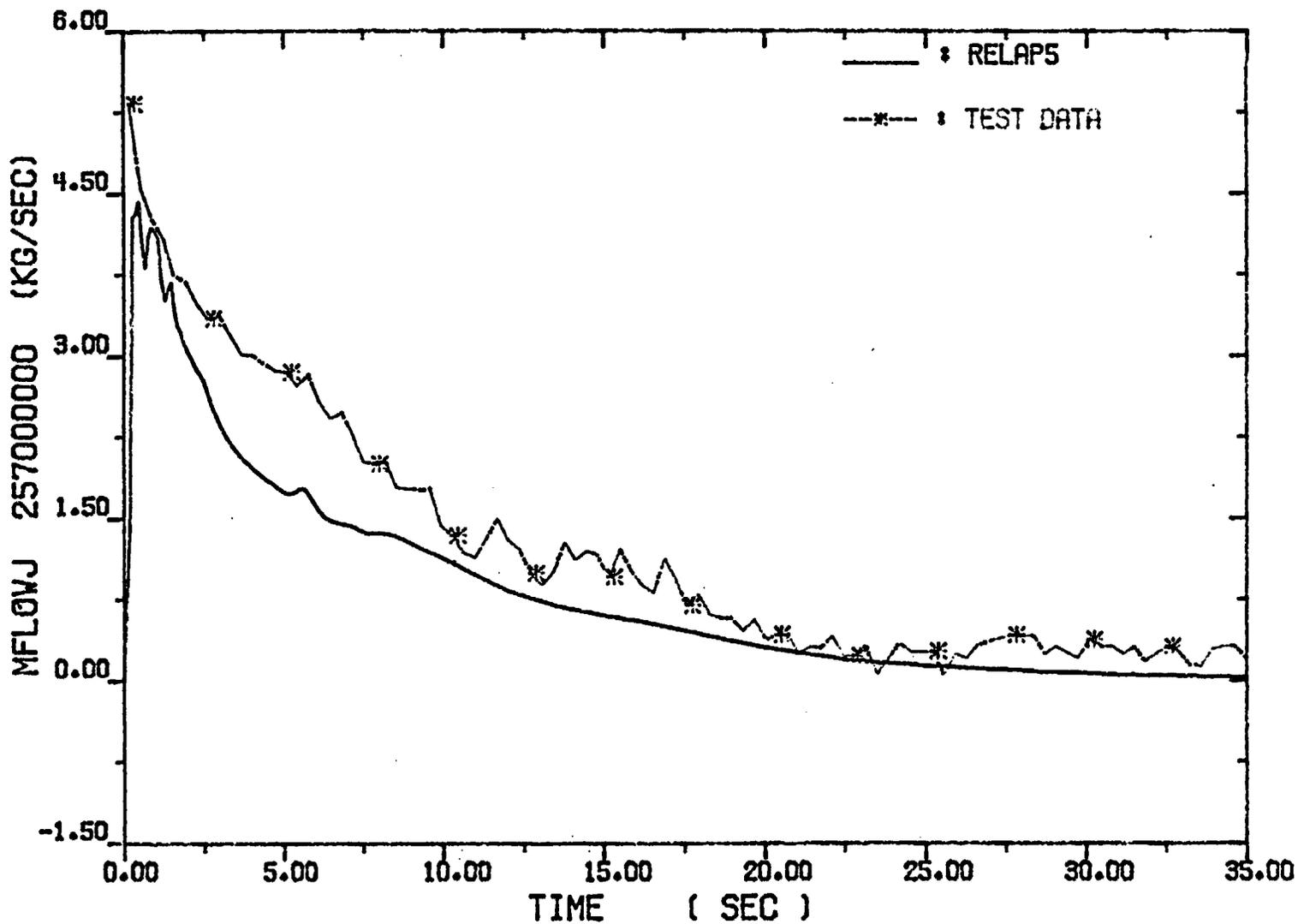
Fig. 4-1. Break Flow Rates near Pump Side
