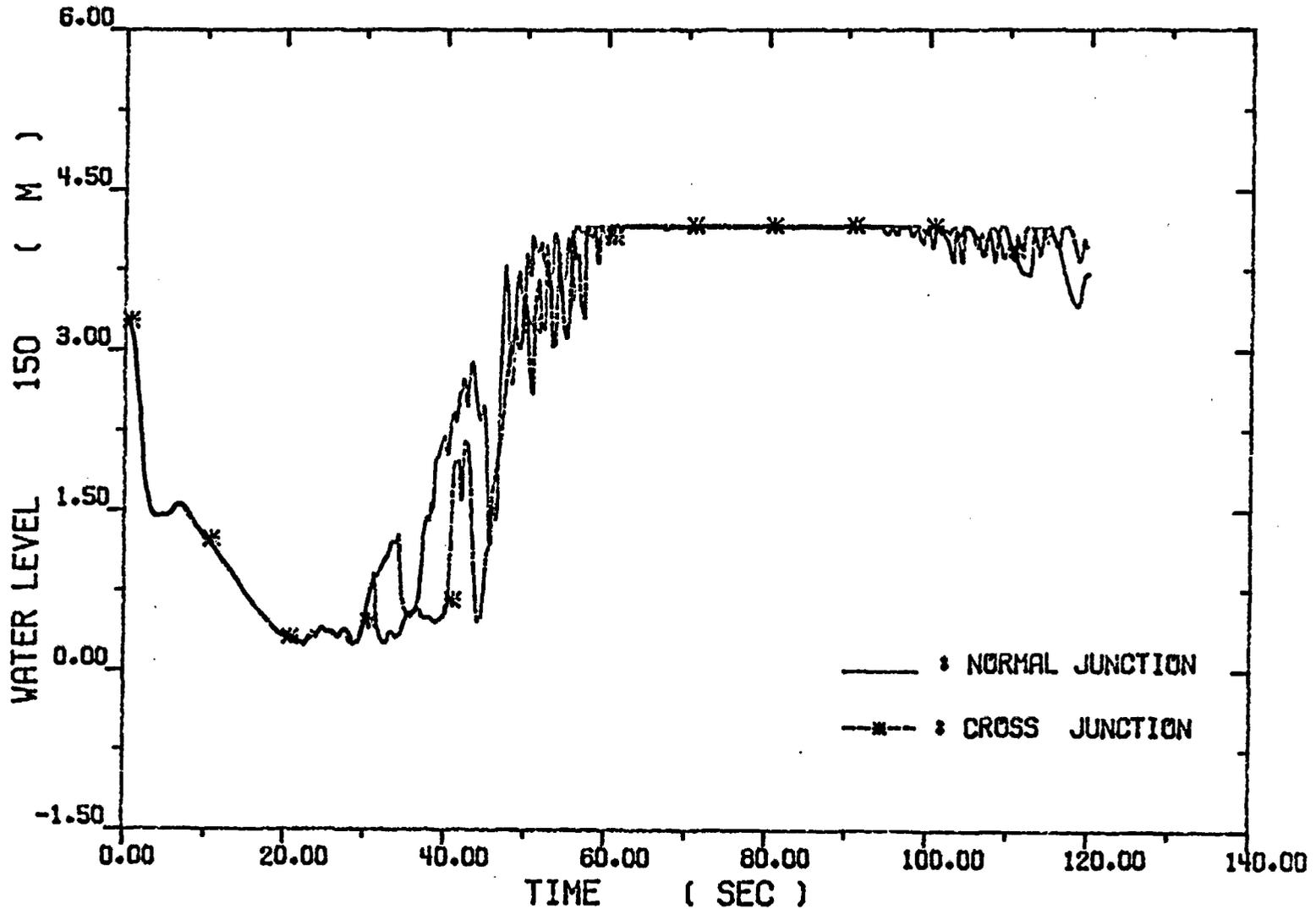
Fig. 4-66. Collapsed Water Levels across The Downcomer
