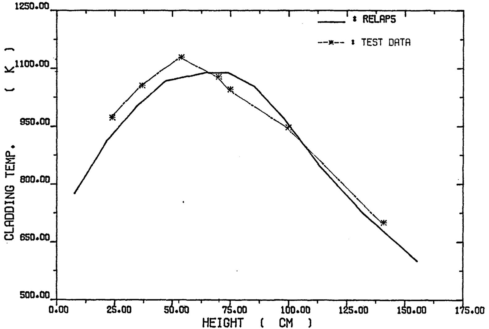
Fig. 4-35. High Power Rod Peak Cladding Temperatures Versus Elevation
