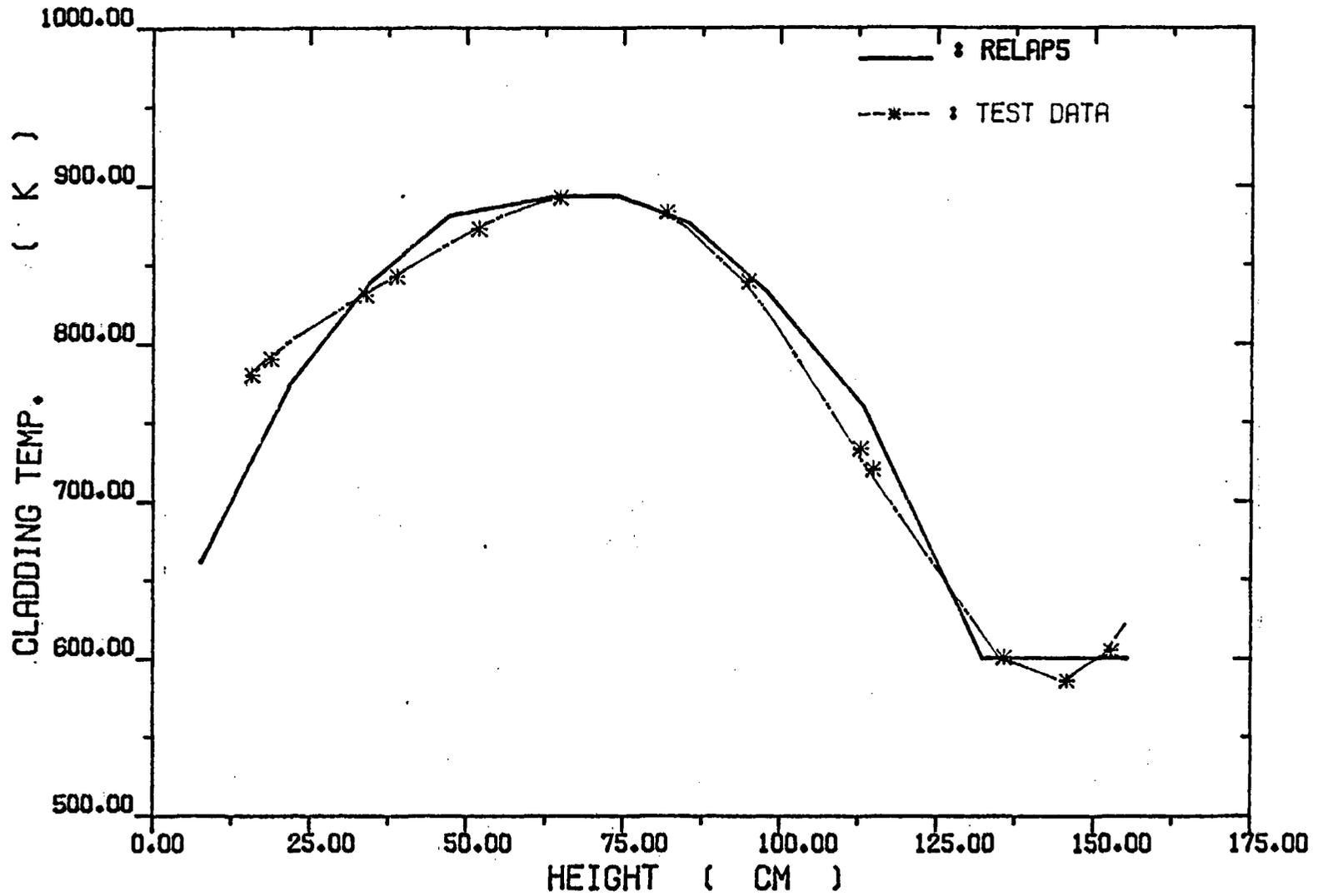
Fig. 4-34. Low Power Rod Peak Cladding Temperatures Versus Elevation
