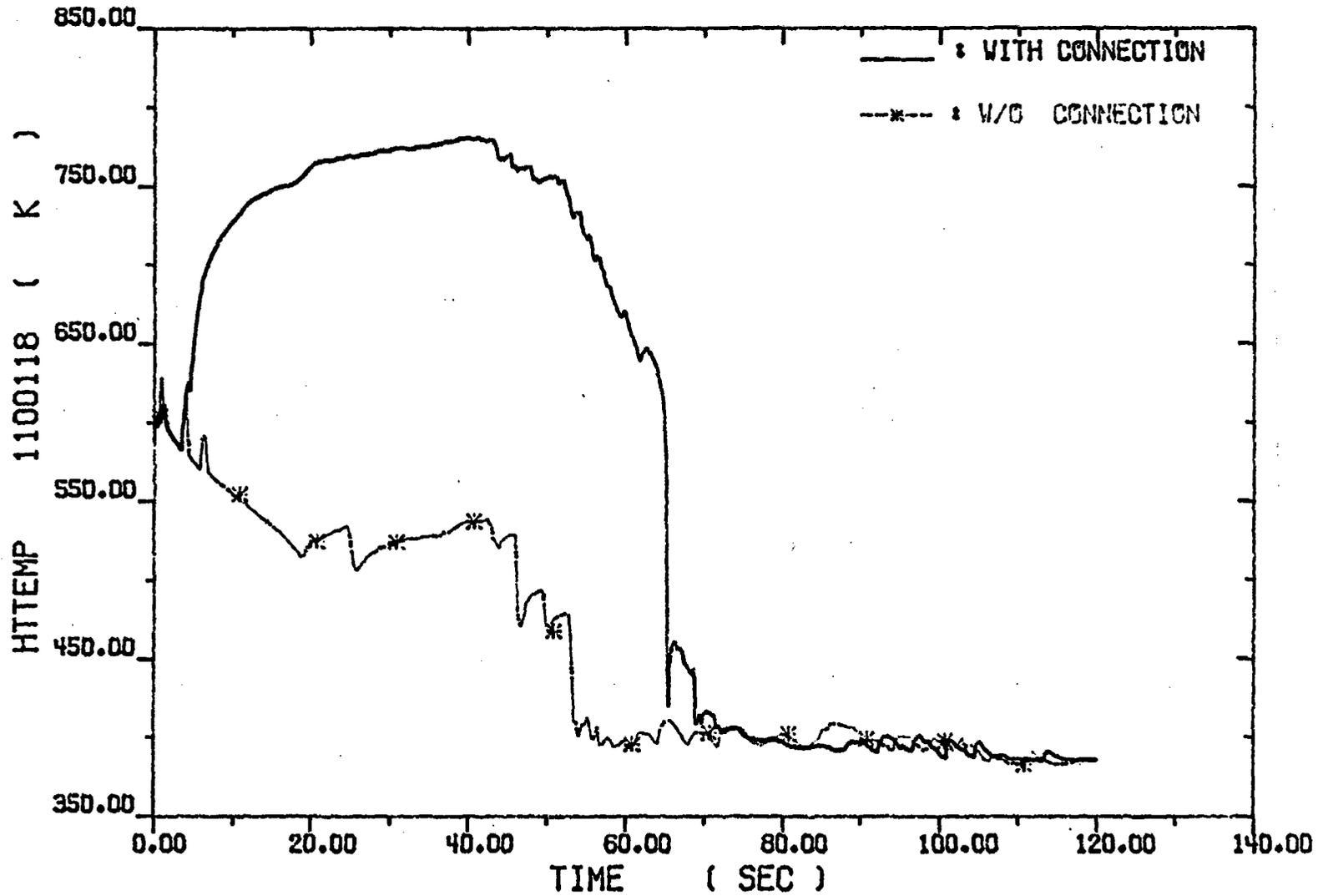
Fig. 4-44. High Power Rod Bottom Section Cladding Temperatures
