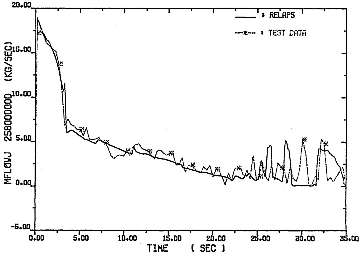
Fig. 4-2. Break Flow Rates near Vessel Side
