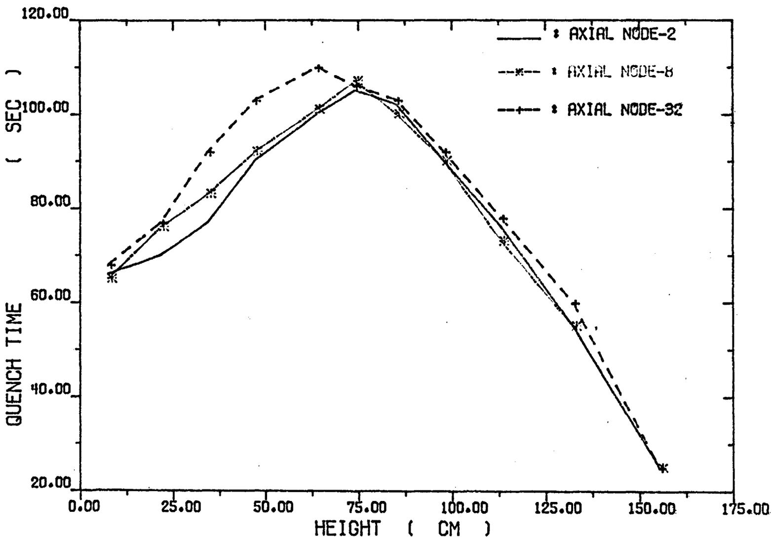
Fig. 4-53. High Power Rod Quench Time versus Elevation
