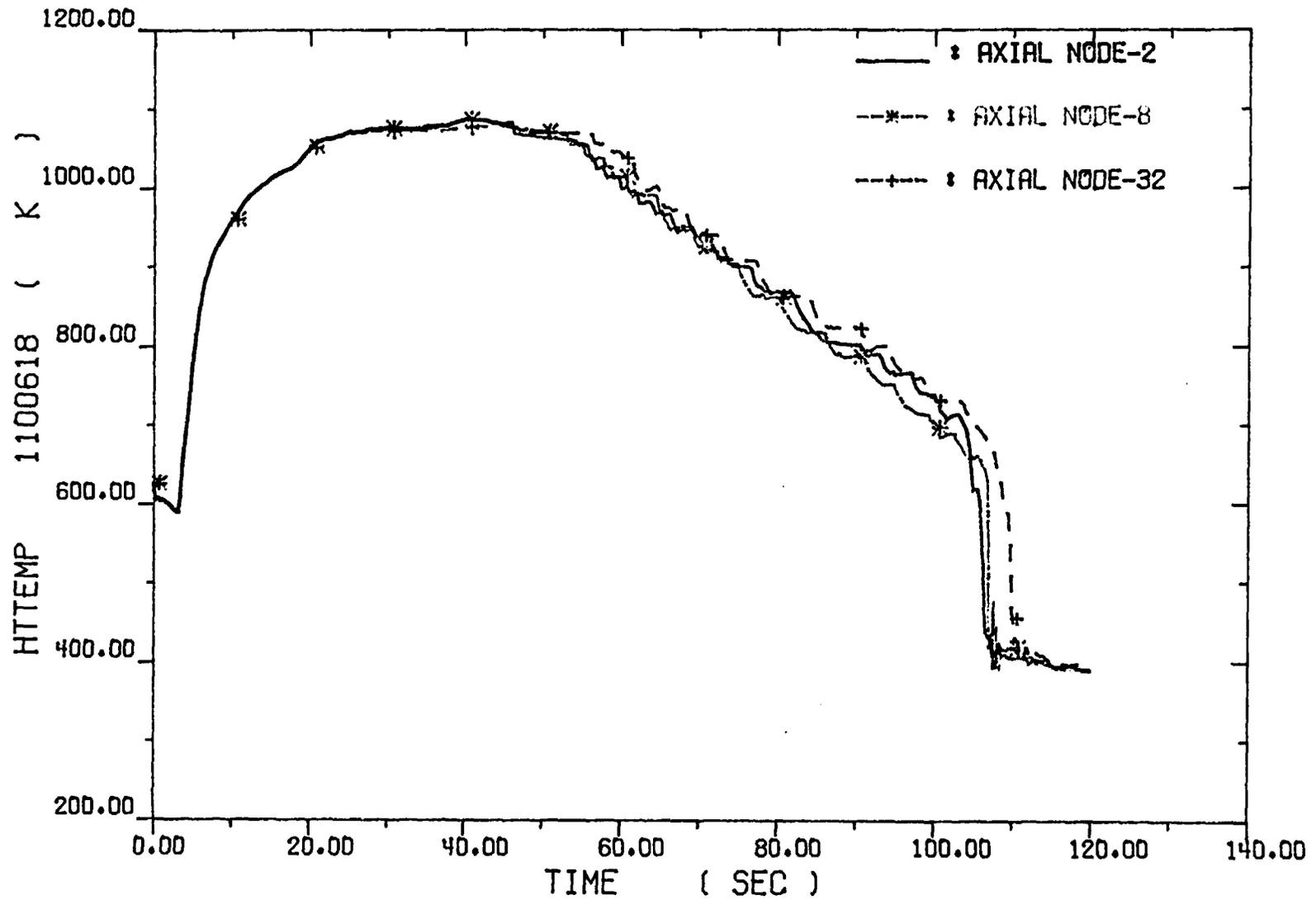
Fig. 4-55. High Power Rod Hot Spot Cladding Temperatures
