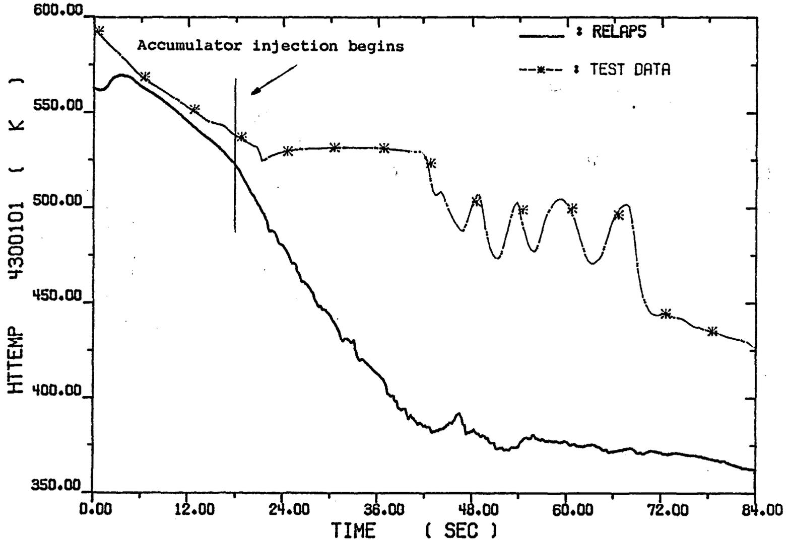
Fig. 4-19. Core Barrel Wall Temperatures
