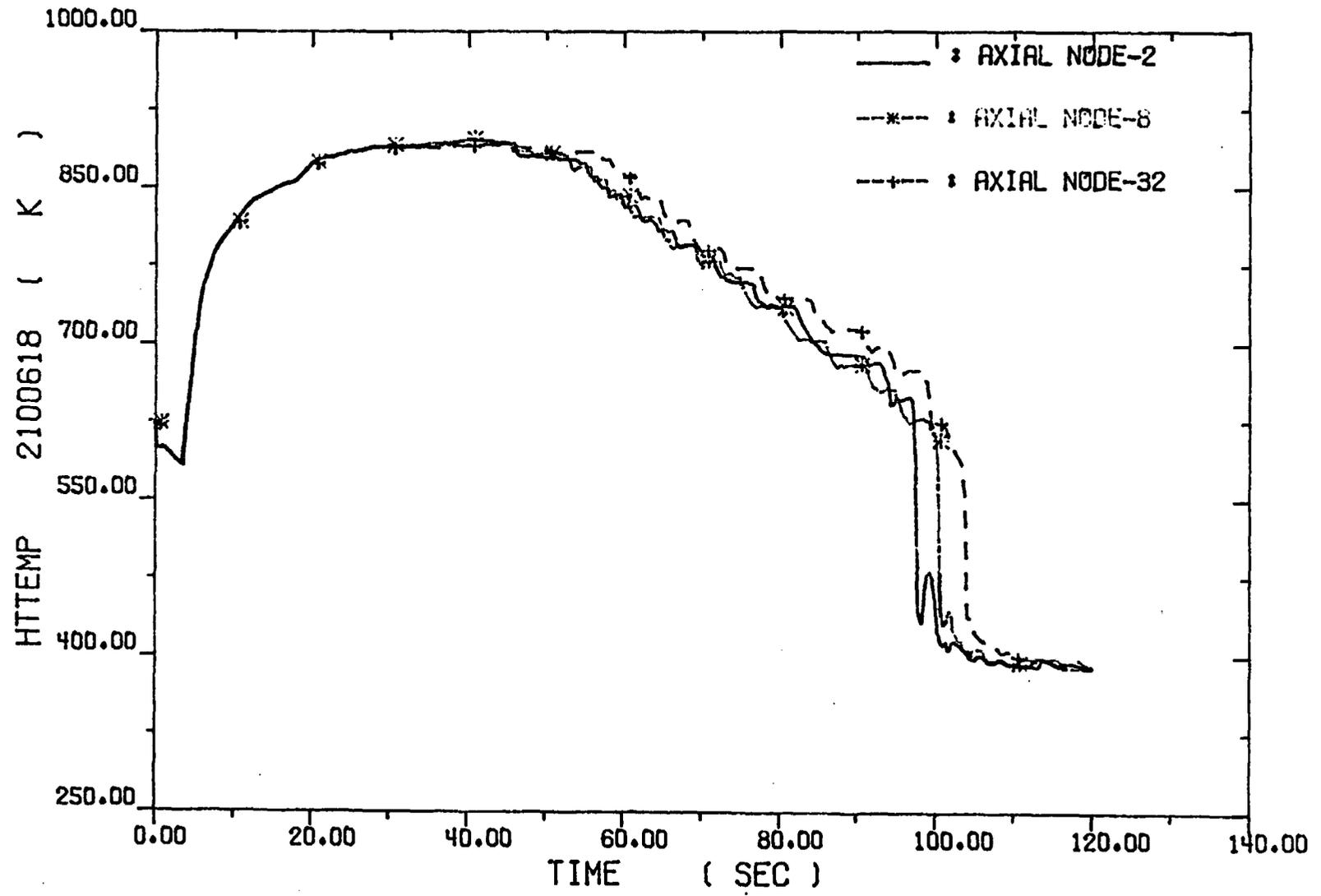
Fig. 4-56. Low Power Rod Hot Spot Cladding Temperatures
