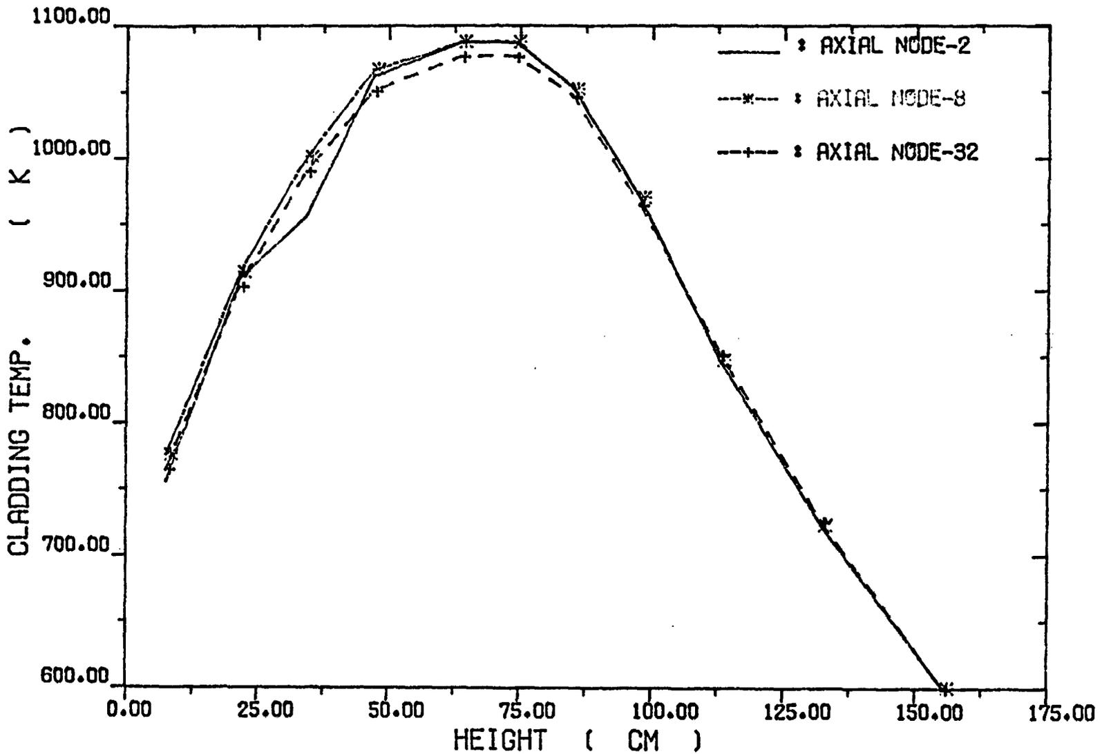
Fig. 4-51. High Power Rod Peak Cladding Temperatures versus Elevation
