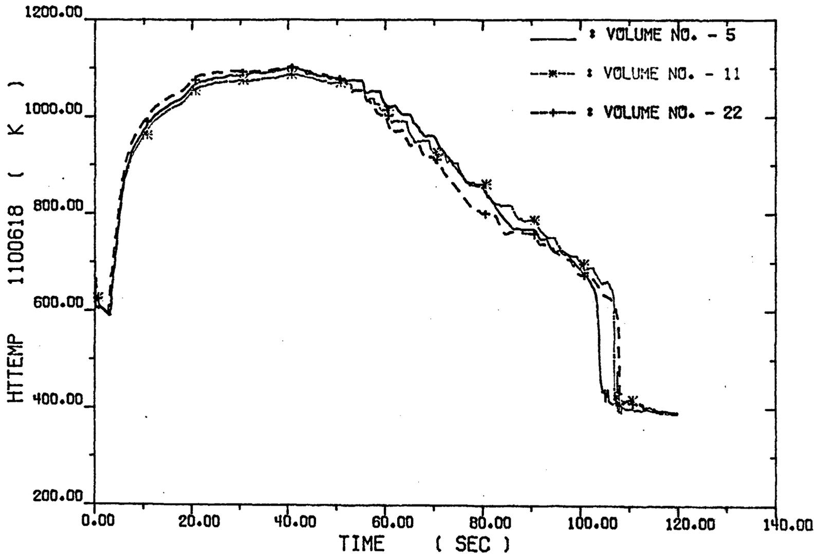
Fig. 4-61. High Power Rod Cladding Temperatures
