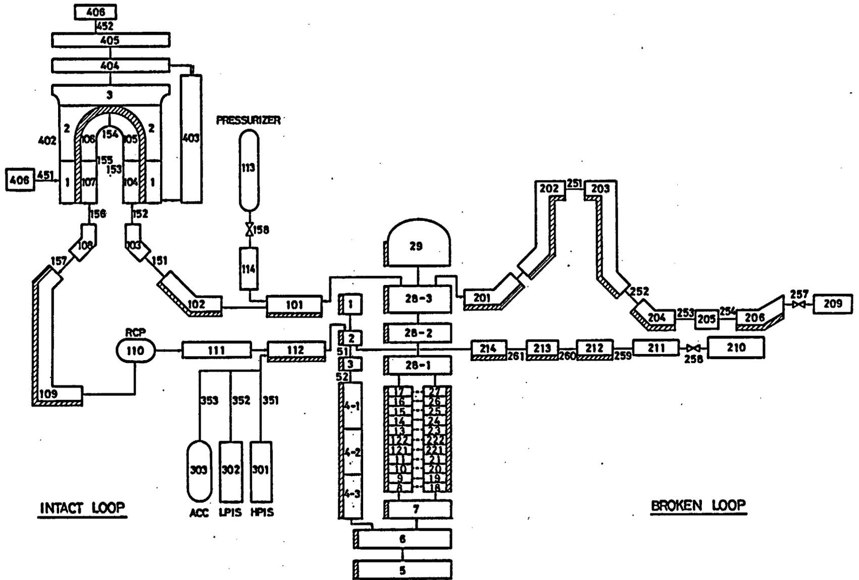
Fig. 3-1. Semiscale Mod-1 System Noding Diagram
