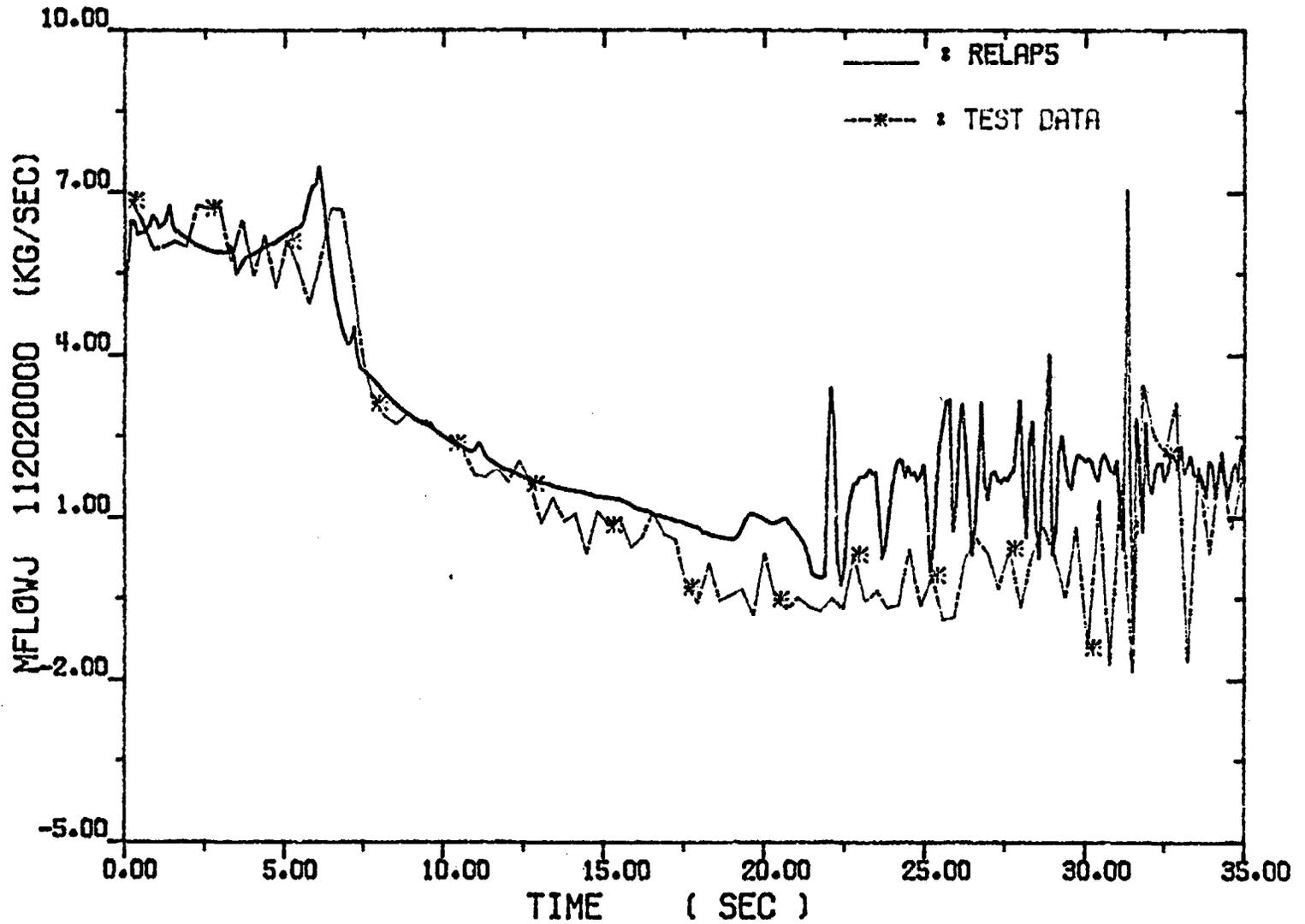
Fig. 4-5. Intact Loop Cold Leg Flow Rates
