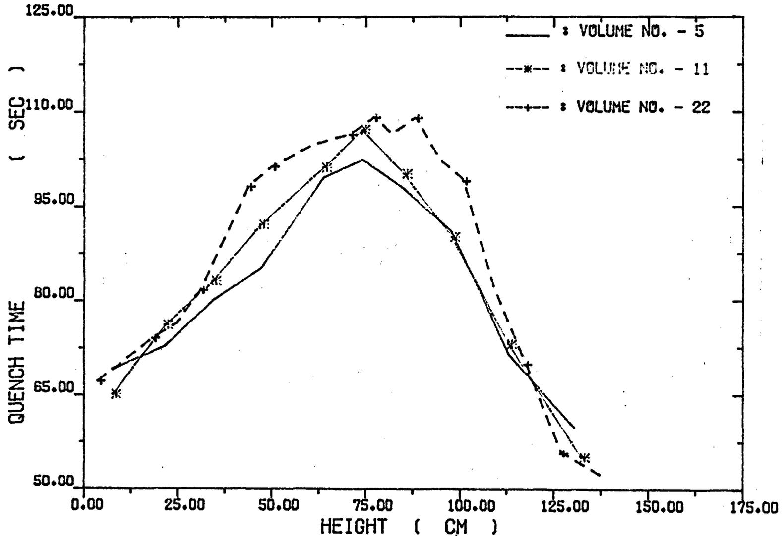
Fig. 4-60. High Power Rod Quench Time versus Elevation
