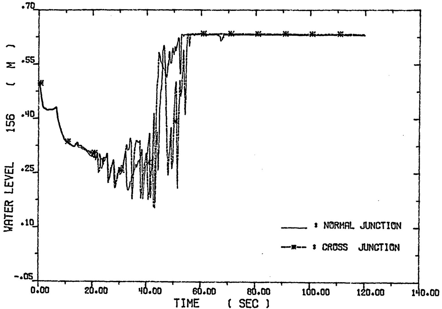
Fig. 4-67. Collapsed Water Levels across The Lower Plenum
