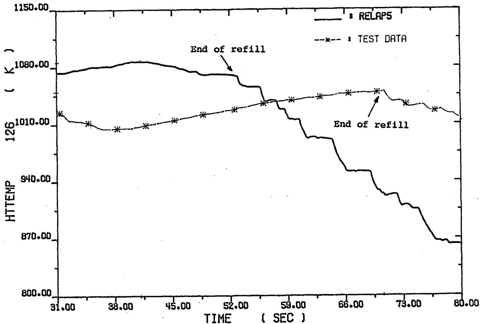
Fig. 4-23. High Power Rod Hot Spot Cladding Temperatures
