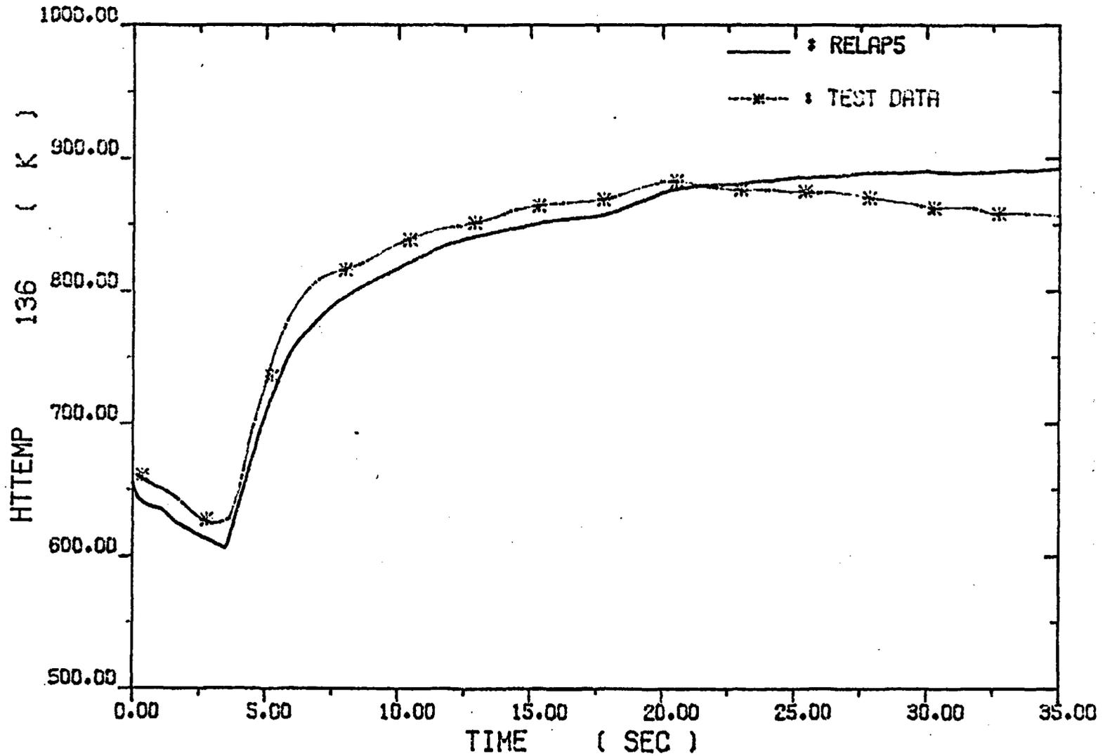
Fig. 4-14. Low Power Rod Hot Spot Cladding Temperatures
