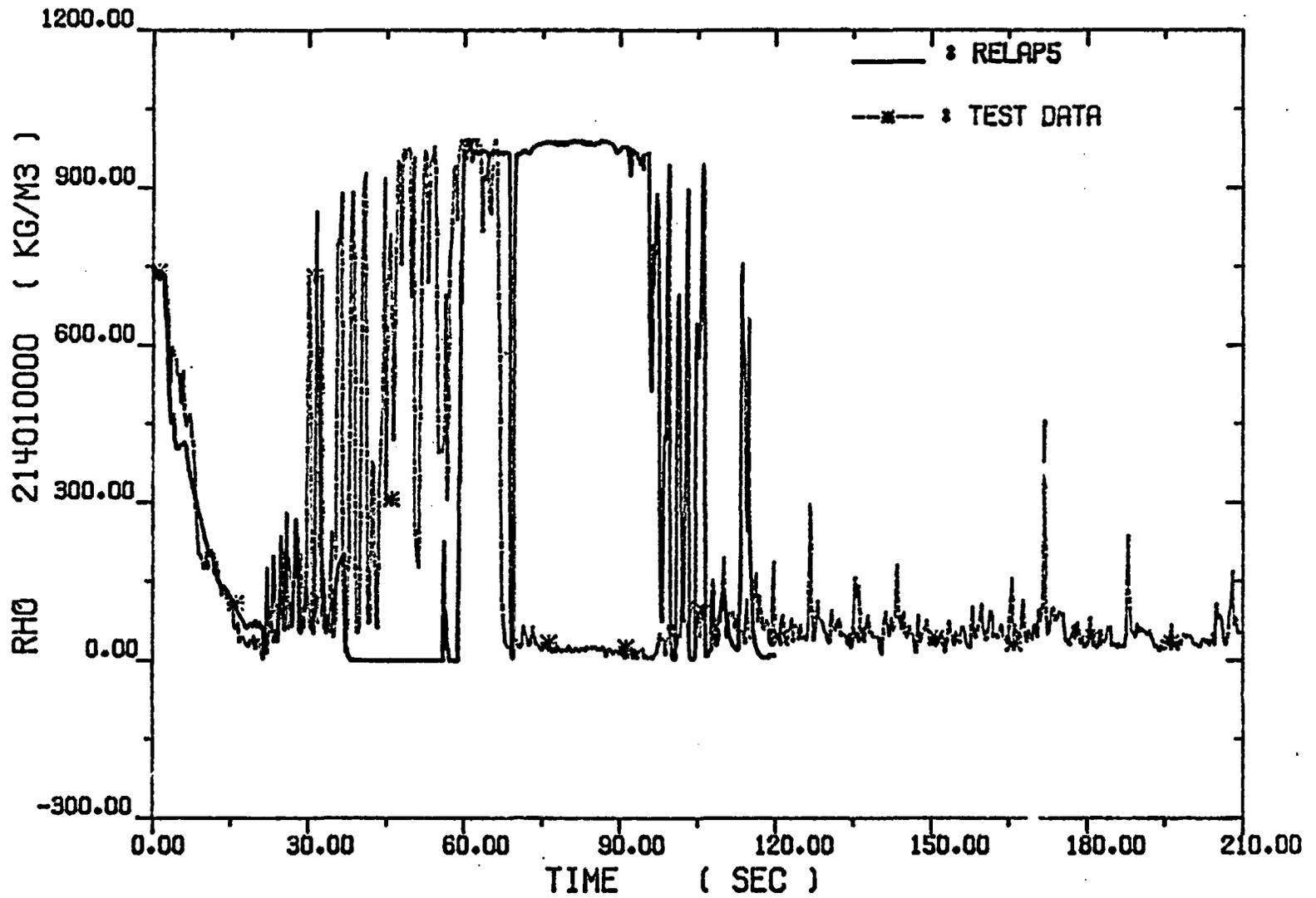
Fig. 4-28. Broken Loop Cold Leg Coolant Densities
