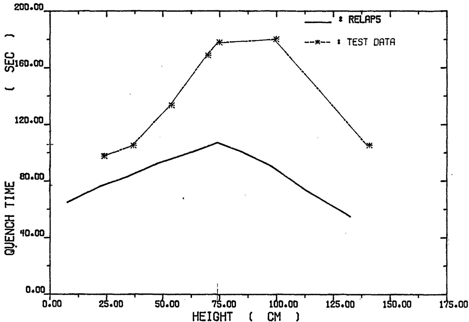
Fig. 4-39. High Power Rod Quench Time versus Elevation
