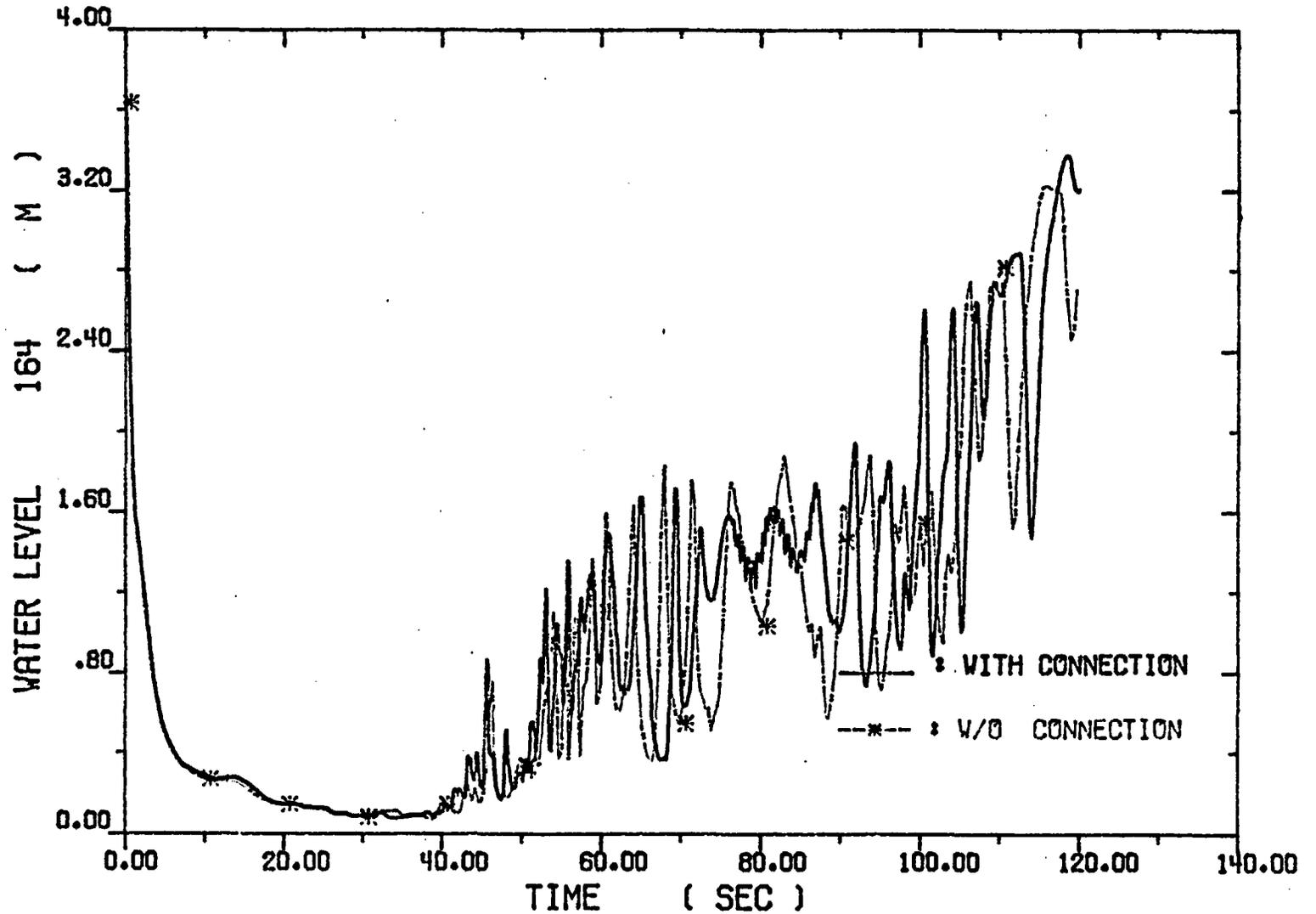
Fig. 4-49. Collapsed Water Levels across the Core
