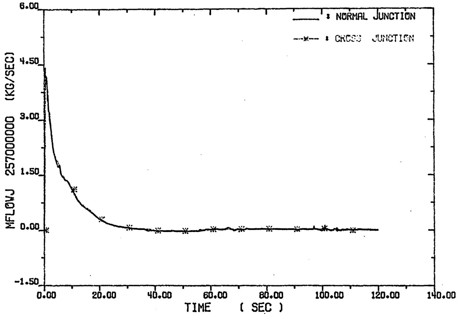
Fig. 4-64. Break Flow Rates near Pump Side
