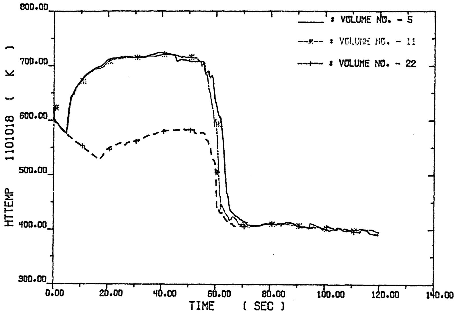
Fig. 4-59. High power Rod Top Section Cladding Temperatures
