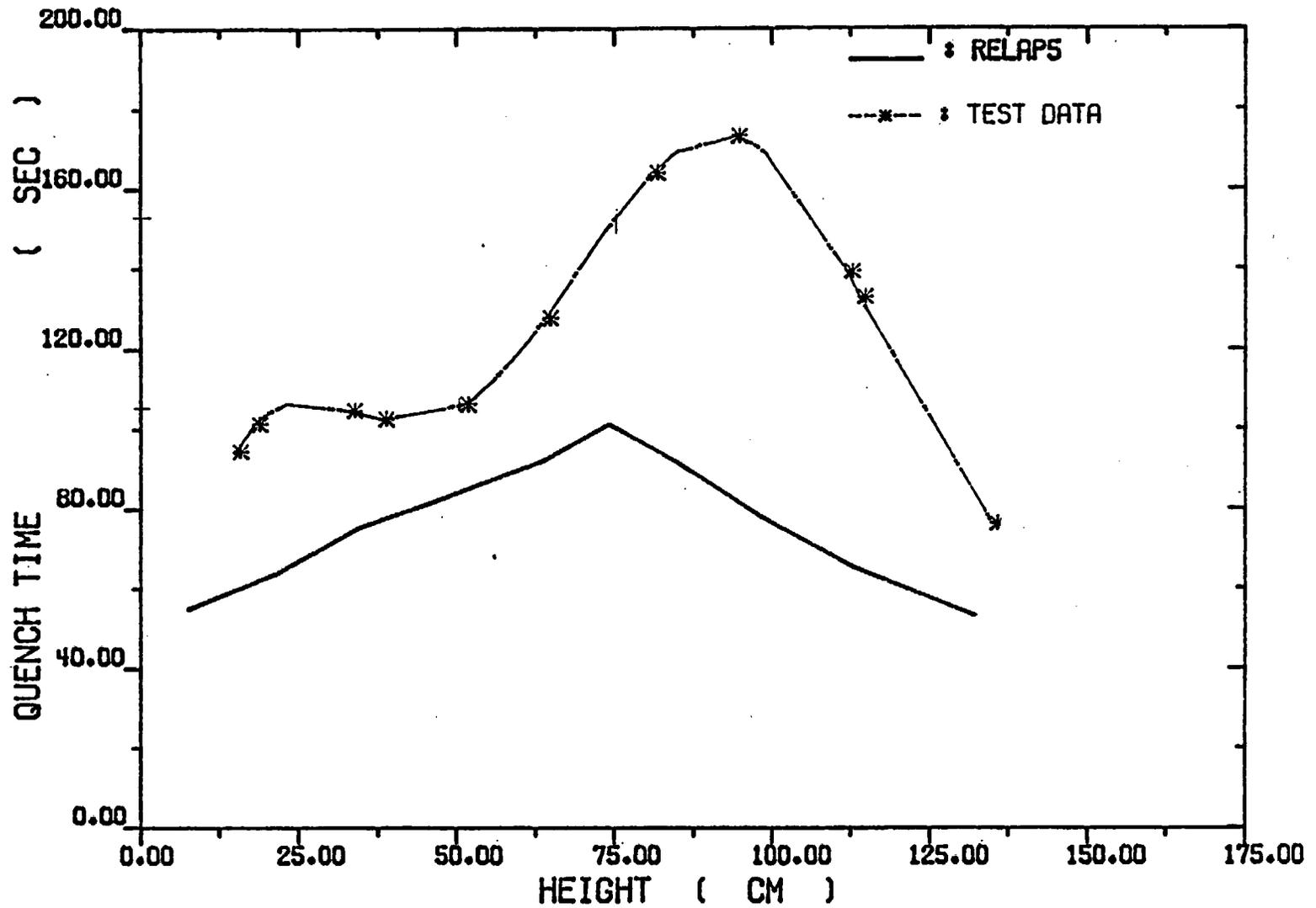
Fig. 4-38. Low Power Rod Quench Time versus Elevation
