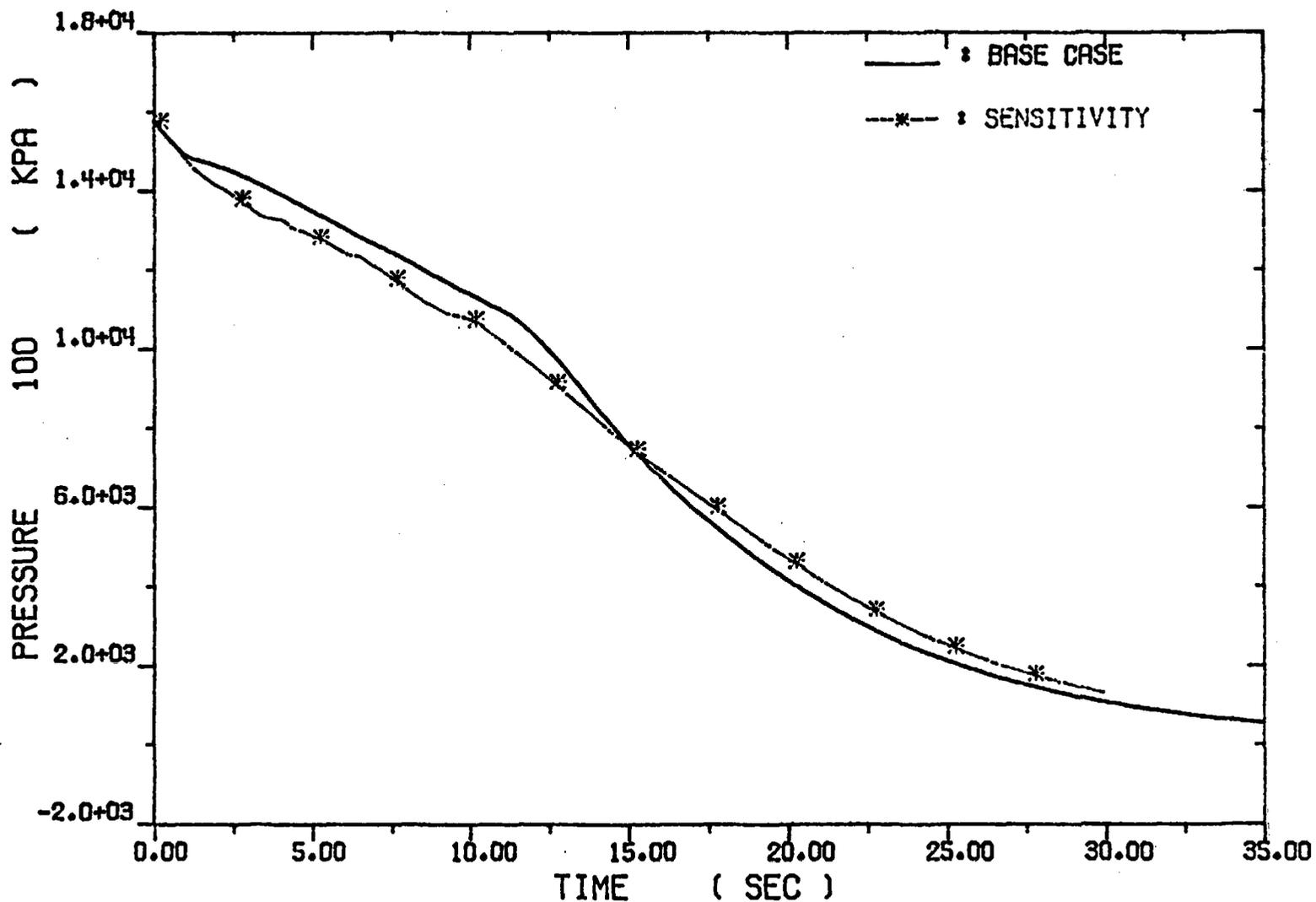
Fig. 4-41. Pressurizer Pressures
