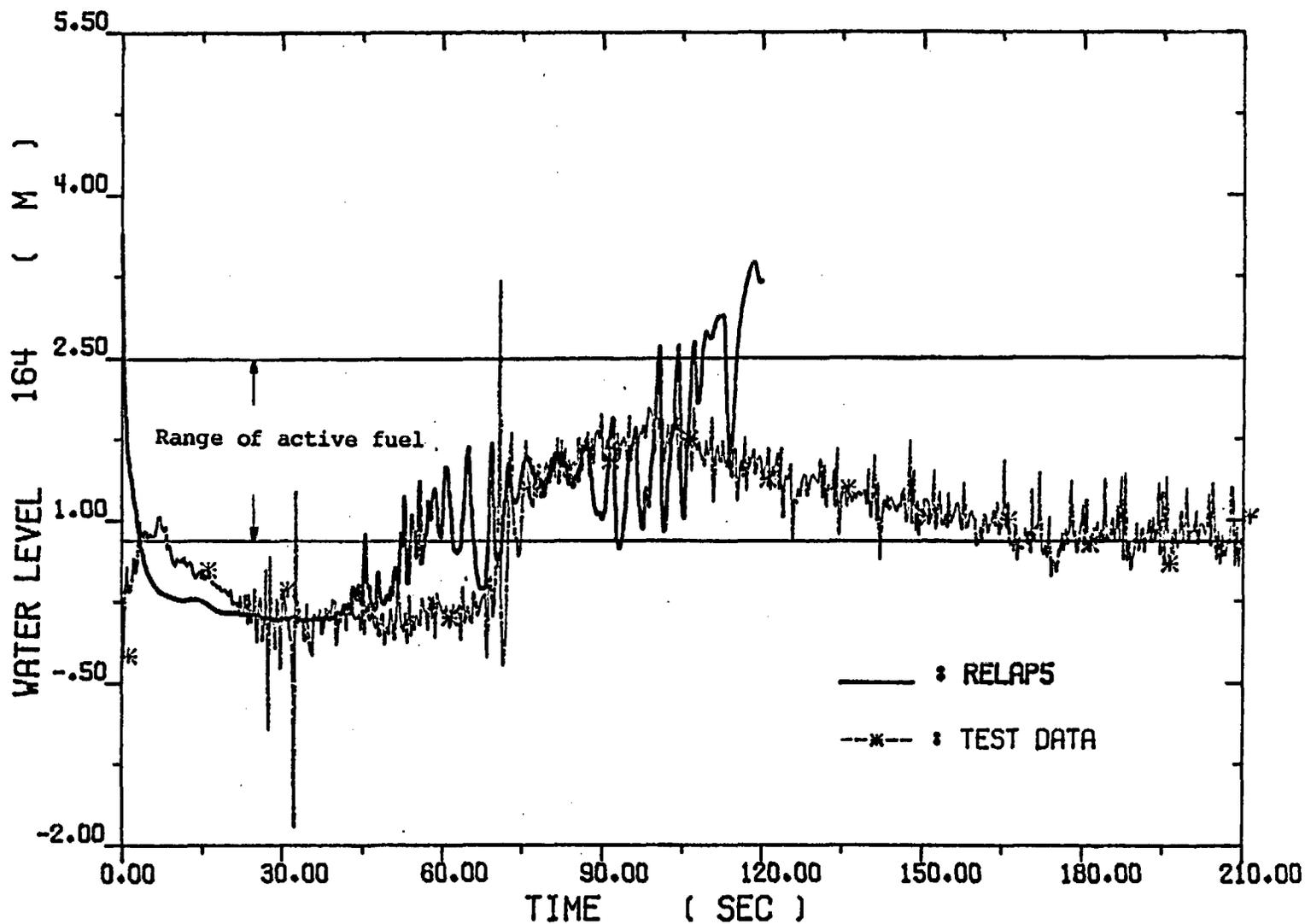
Fig. 4-26. Collapsed Water Levels across The Core
