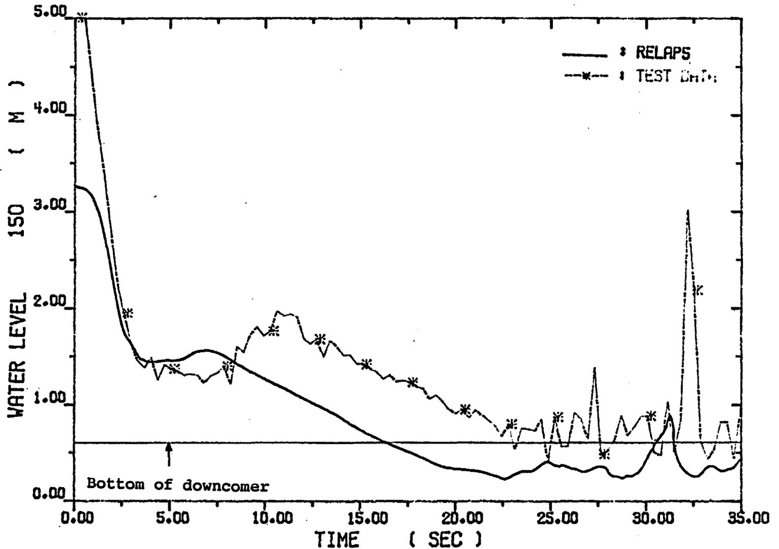
Fig. 4-10. Collapsed Water Levels across The Downcomer
