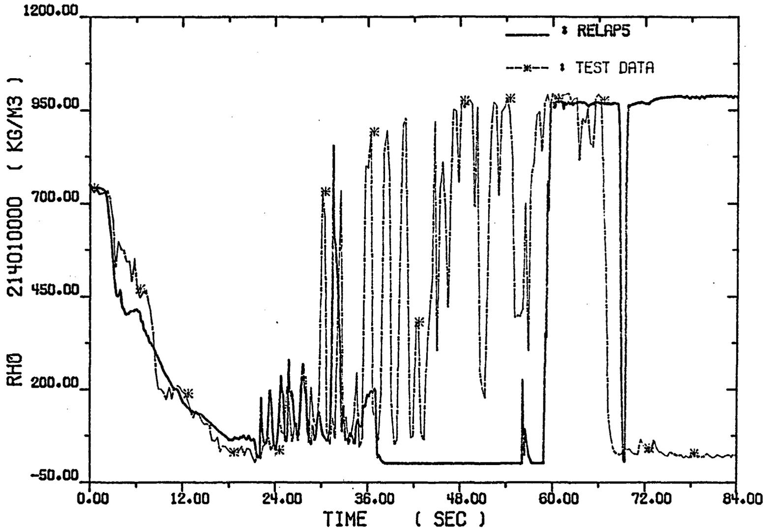
Fig. 4-17. Broken Loop Cold Leg Coolant Densities
