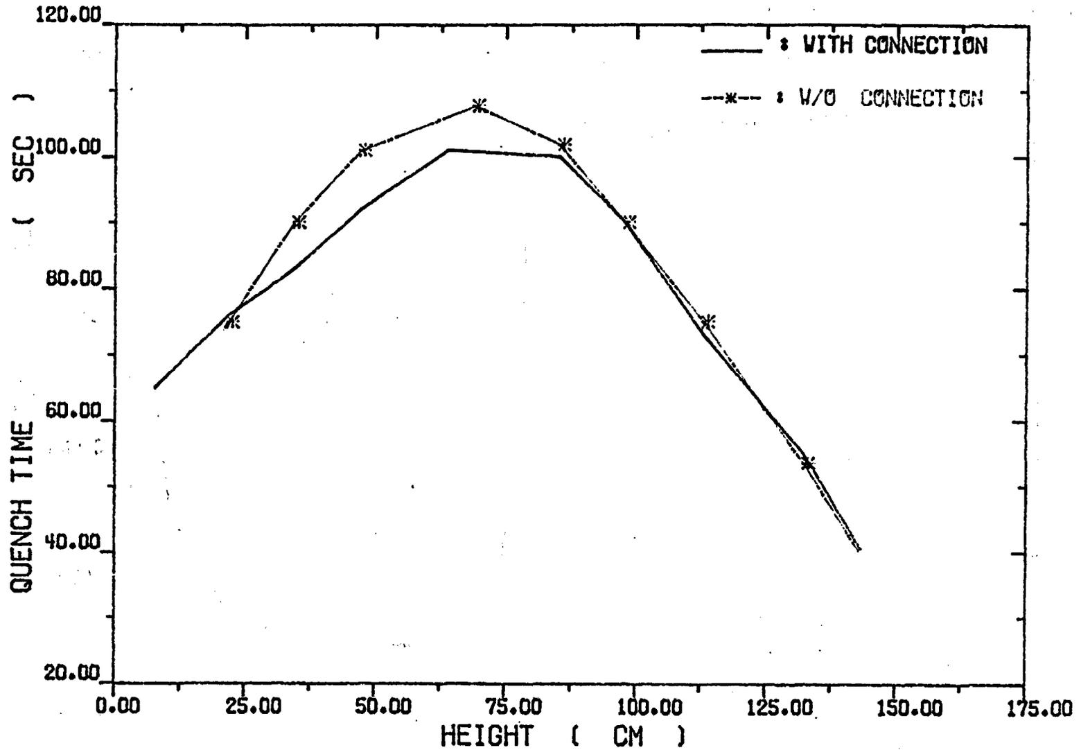
Fig. 4-46. High Power Rod Quench Time versus Elevation
