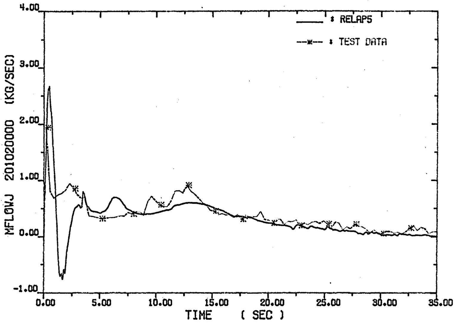
Fig. 4-8. Broken Loop Hot Leg Flow Rates
