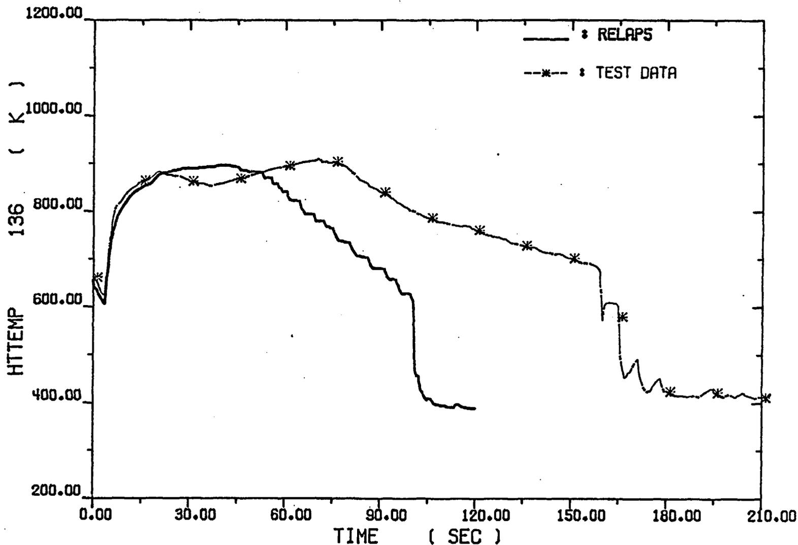
Fig. 4-30. Low Power Rod Hot Spot Cladding Temperatures
