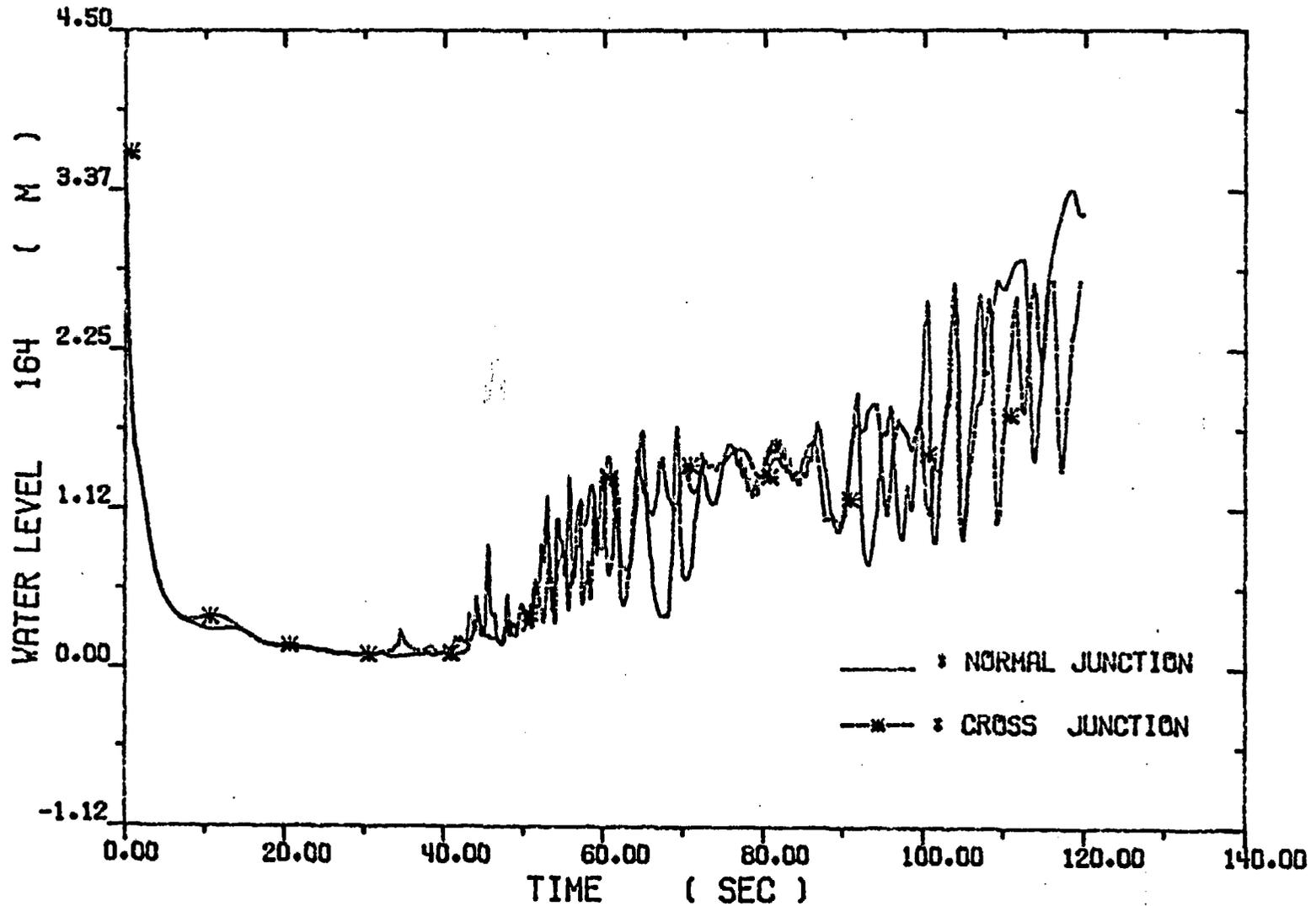
Fig. 4-68. Collapsed Water Levels across The Core
