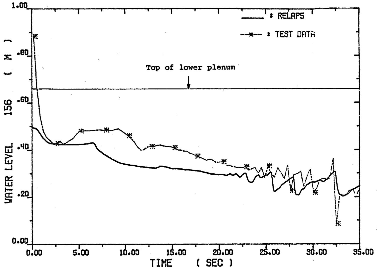
Fig. 4-11. Collapsed Water Levels across The Lower Plenum
