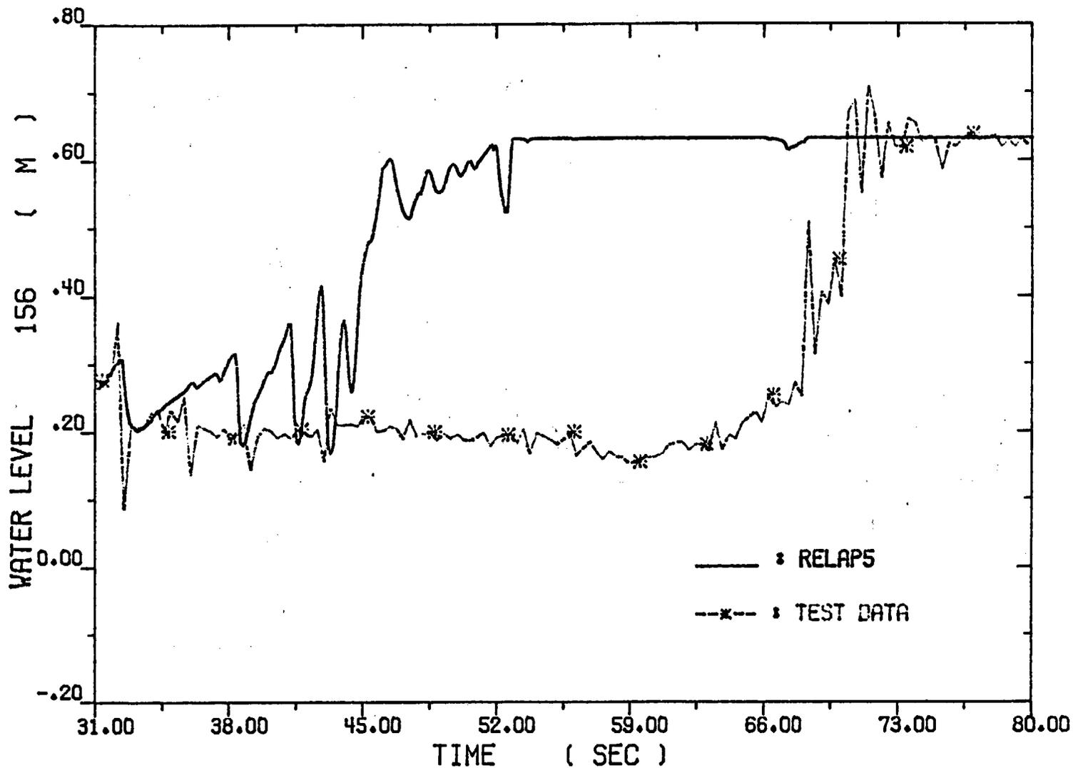
Fig. 4-21. Collapsed Water Levels across The Lower Plenum
