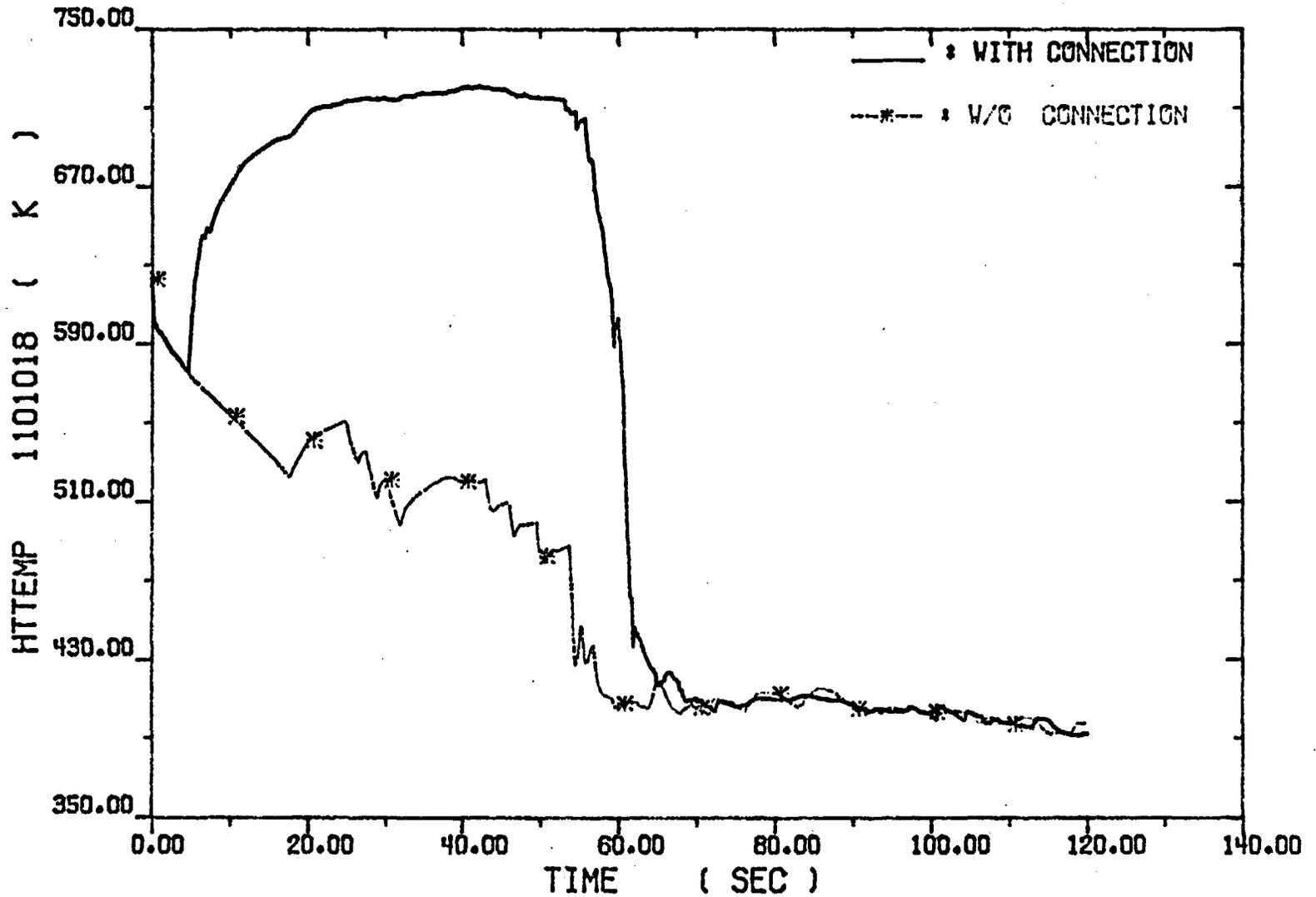
Fig. 4-45. High Power Rod Top Section Cladding Temperatures
