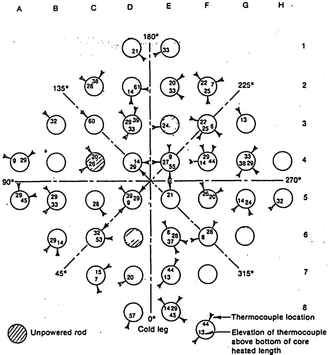
Fig. 2-3. Semiscale Mod-1 Heated Core Plan View
