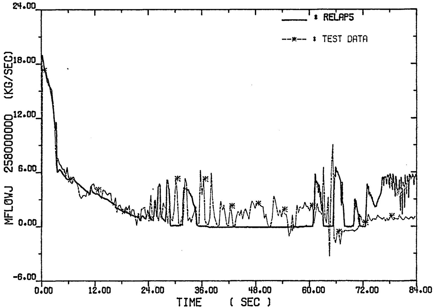
Fig. 4-18. Break Flow Rates near Vessel Side
