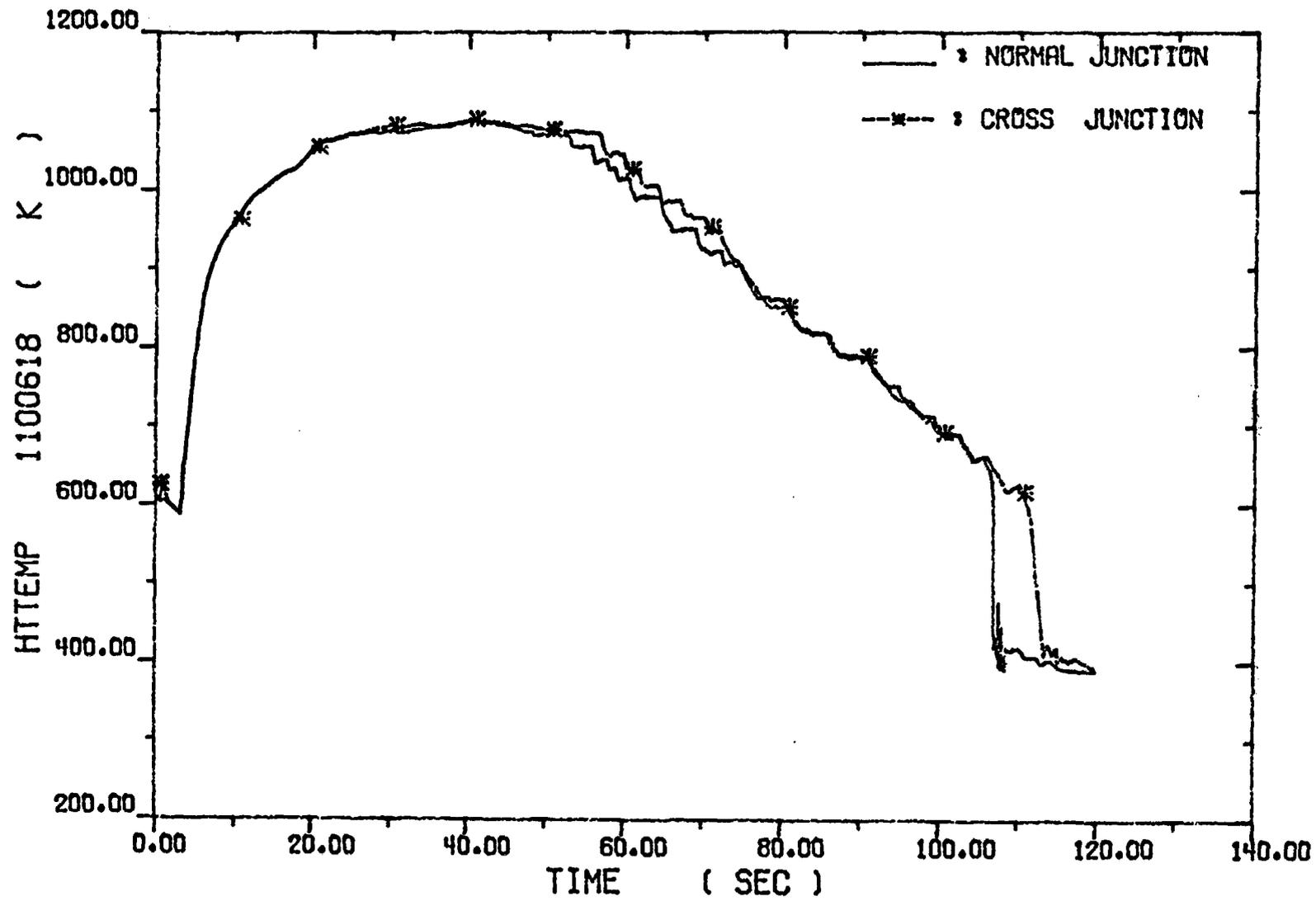
Fig. 4-71. High Power Rod Hot Spot Cladding Temperatures
