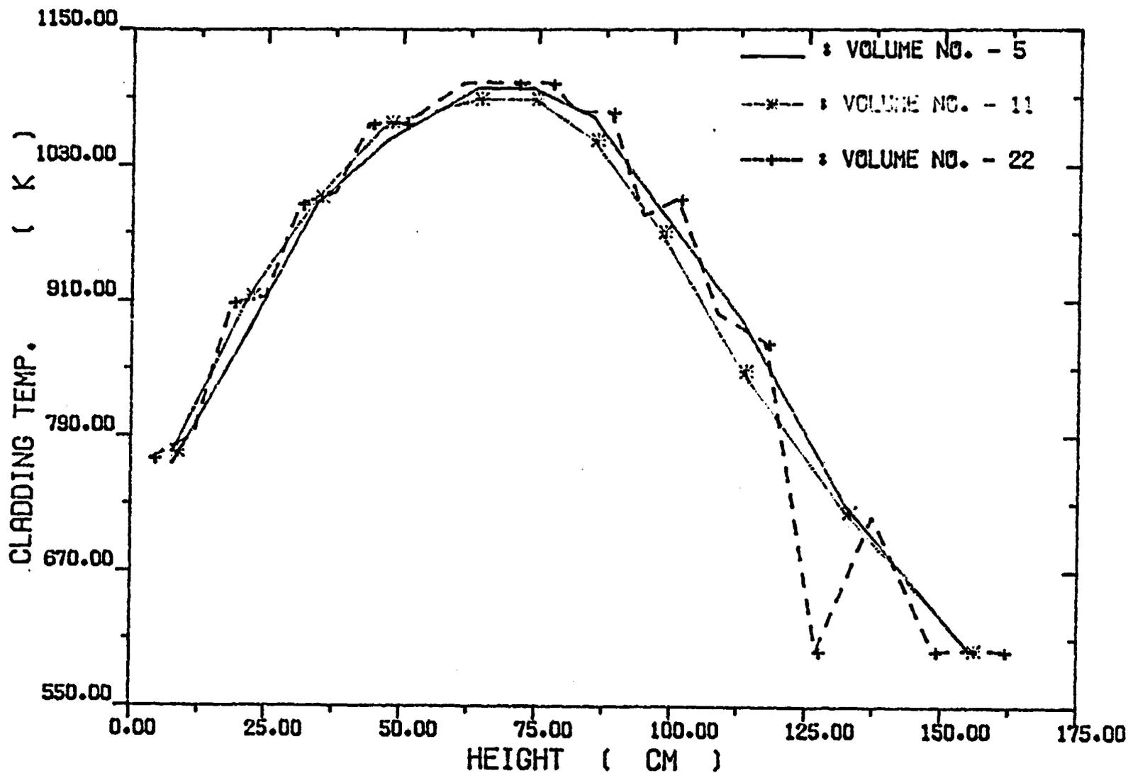
Fig. 4-58. High Power Rod Peak Cladding Temperatures versus Elevation
