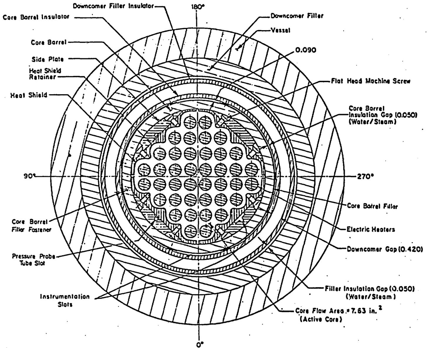
Fig. 2-2. Electric Heater Rod Matrix for Mod-1 Core
