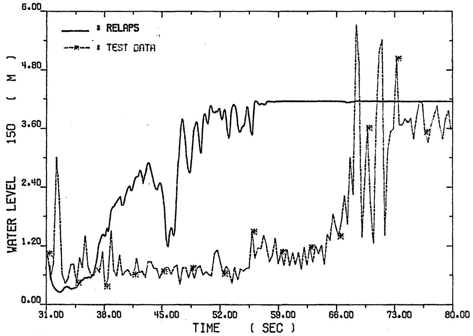
Fig. 4-20. Collapsed Water Levels across The Downcomer
