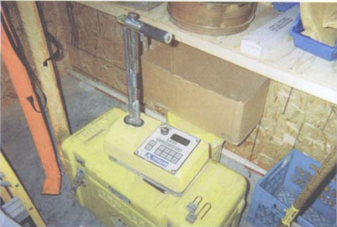
Photos showing secured source rod
