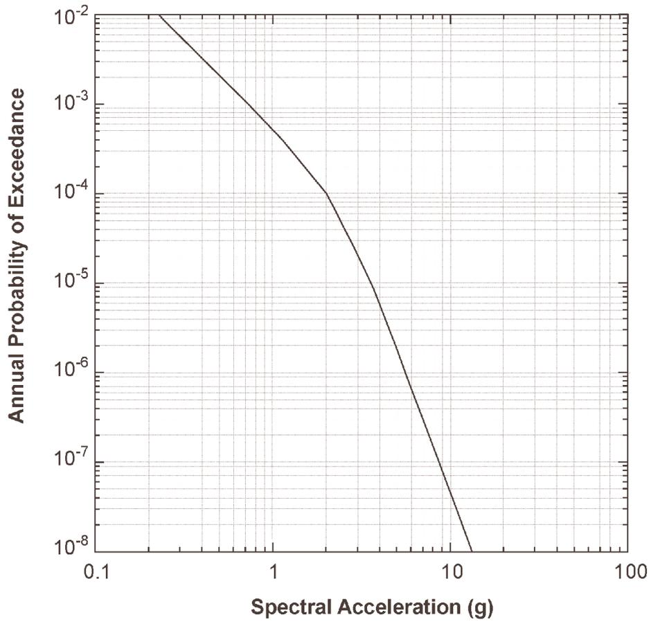
**Figure A-1 Hypothetical Seismic Hazard Curve for Spectral Acceleration at 10-Hz.**
