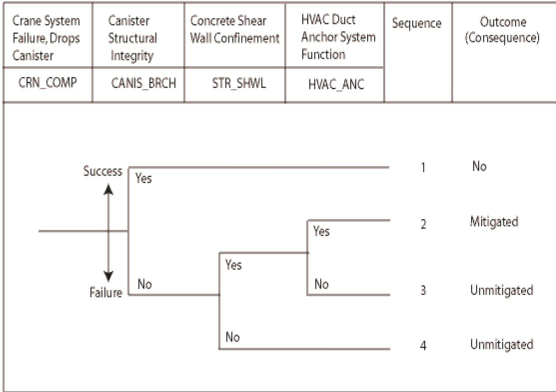
**Figure B-1 Seismically Initiated Event Sequences.**
