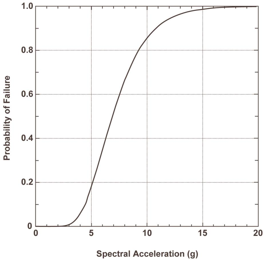
Figure A-2 Hypothetical Seismic Fragility Curve for Spectral Acceleration at 10-Hz.
