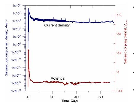
Measured current density and potential using the single crevice assembly for an Alloy 22 cylindrical specimen galvanically coupled to a large Alloy 22 plate in 5 M NaCl solution with the addition of  $2x10^{-4}$  M CuCl<sub>2</sub> at 95 °C [203 °F]
