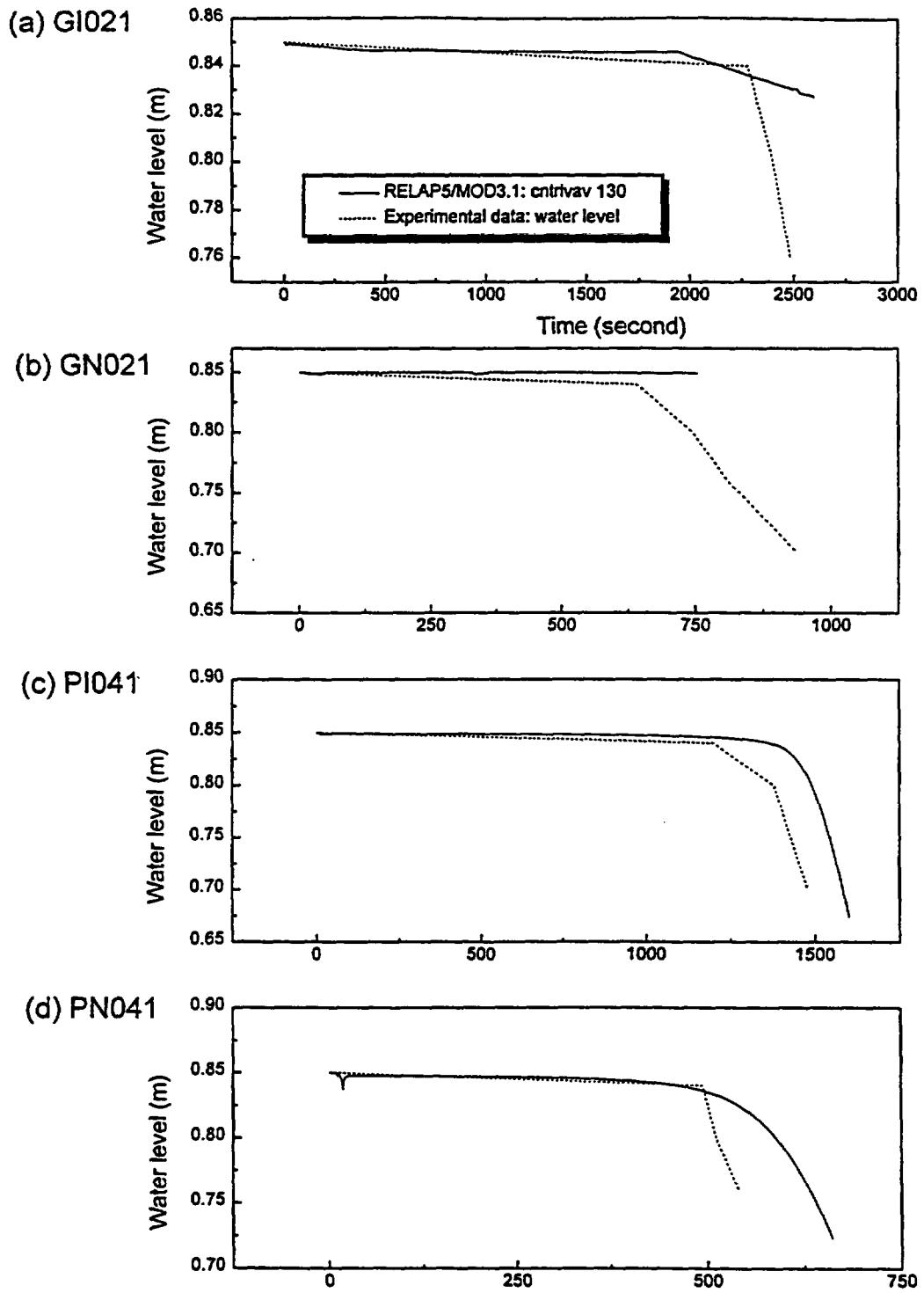
Figure 3.7: Comparison of the water level between experiments and calculation
