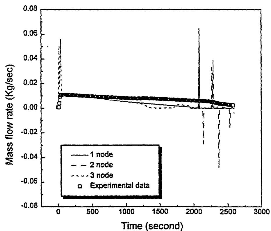
Figure 3.15: Comparison of the steam flow rate between test GI021 and calculation(Nodalization study)
