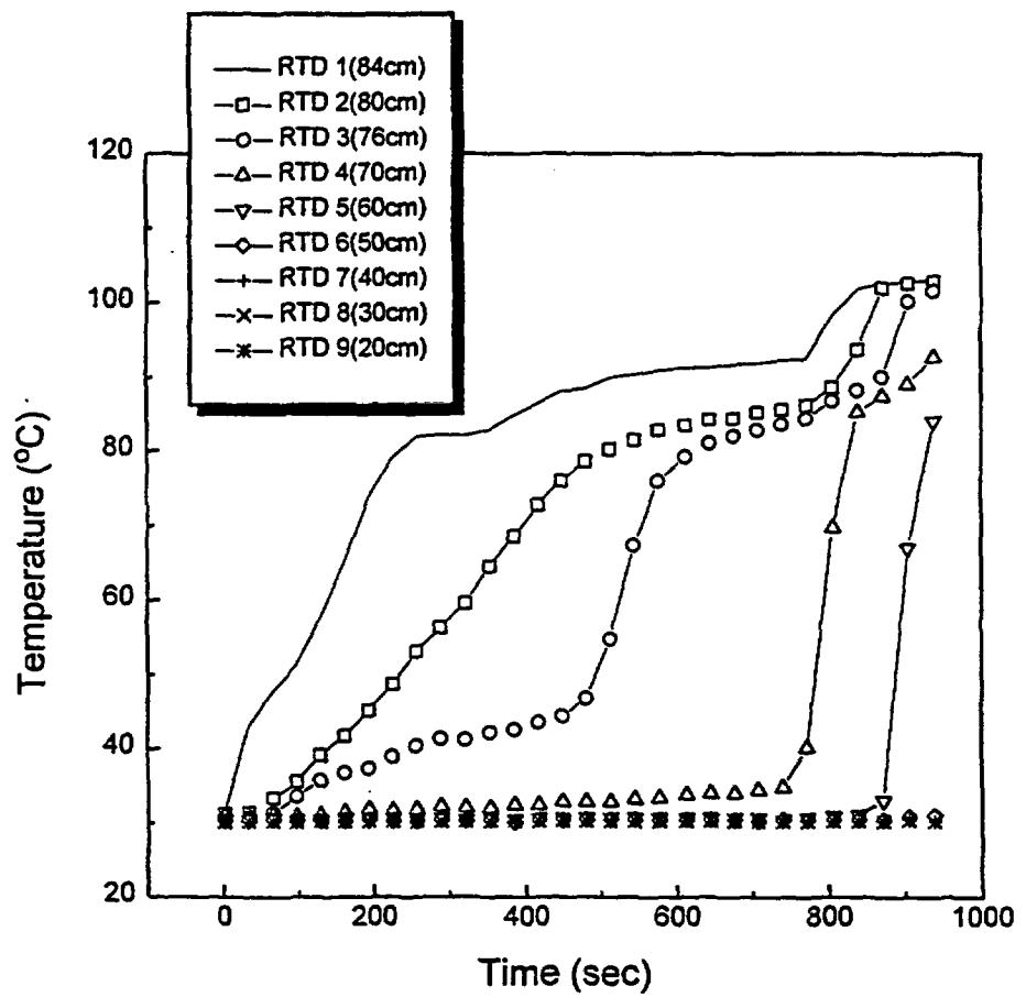
Figure 2.10: The temperature distribution of test section for test GS021
