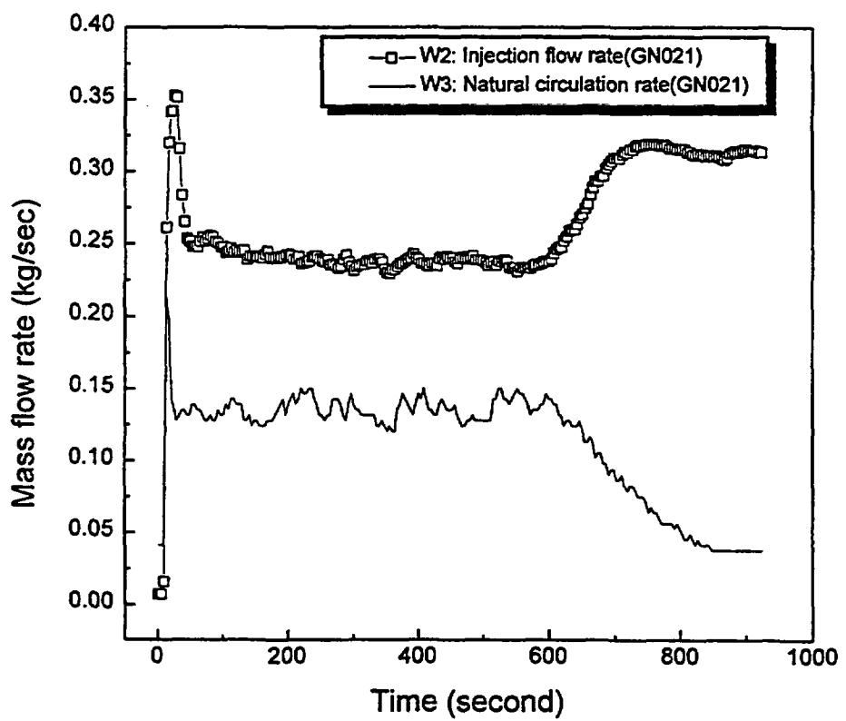
Figure 2.7: The comparison of the natural circulation flow with the injection flow rate for test GN021
