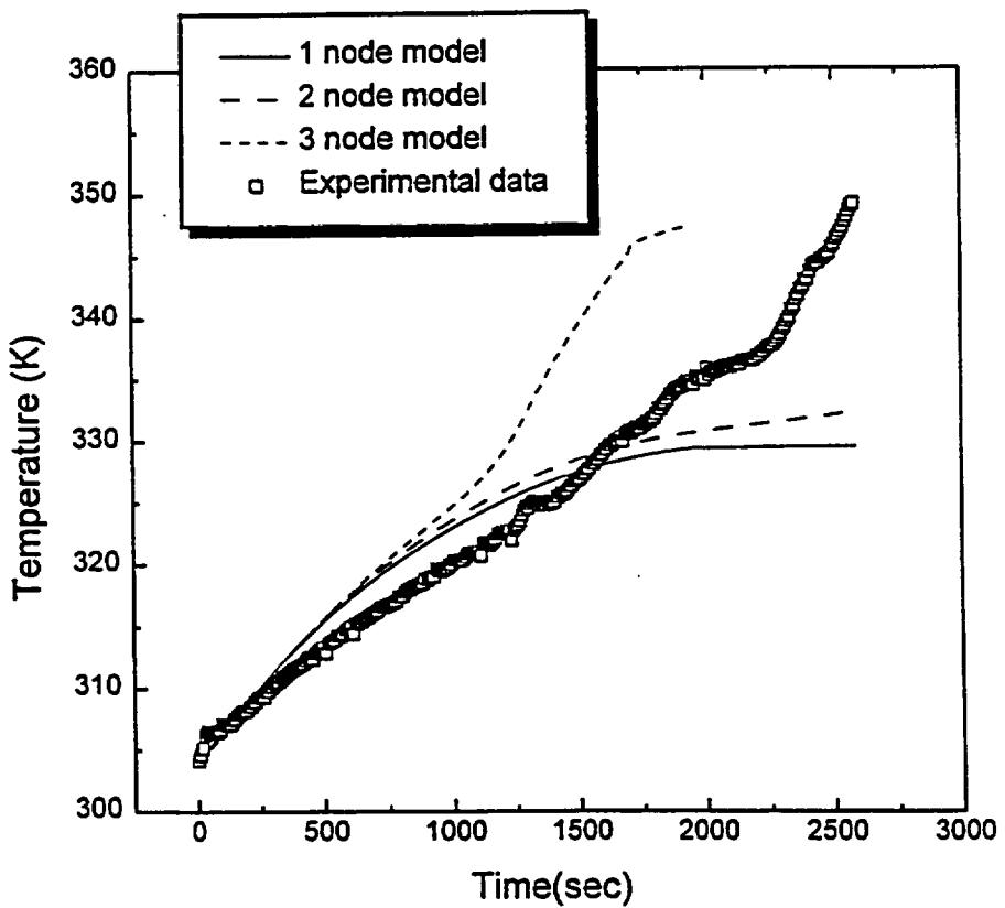
Figure 3.14: Comparison of the pool water temperature between test GI021 and calculation(Nodalization study)
