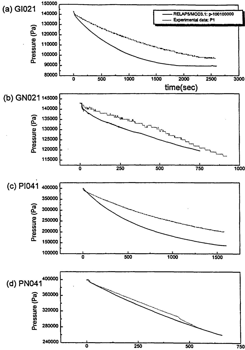
Figure 3.2: Comparison of the steam generator pressure between experiments and calculation
