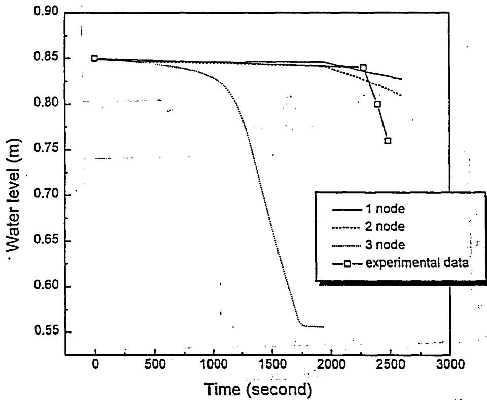
Figure 3.17: Comparison of the water level between test GI021 and calculation(Nodalization study)
