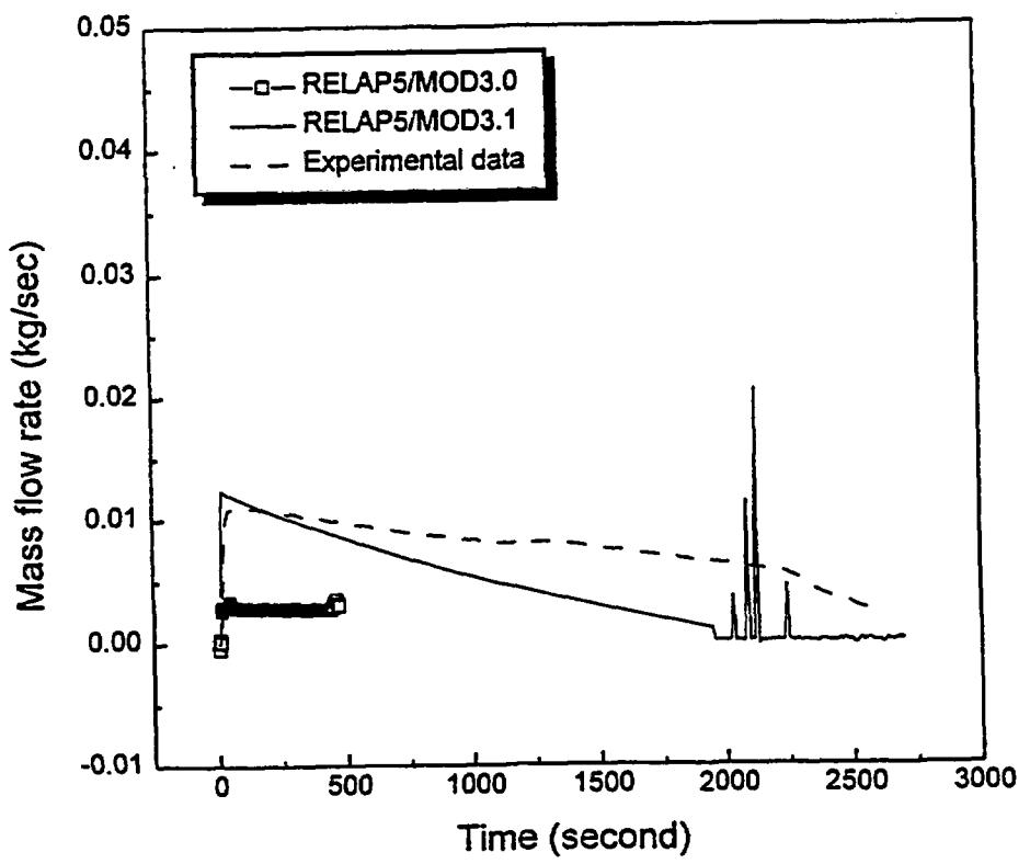
Figure 3.10: Comparison of the steam flow rate between test GI021 and calculation(MOD3.0 vs MOD3.1)
