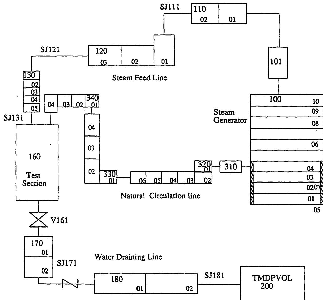
Figure 3.1: A systematic diagram of RELAP5 nodalization
