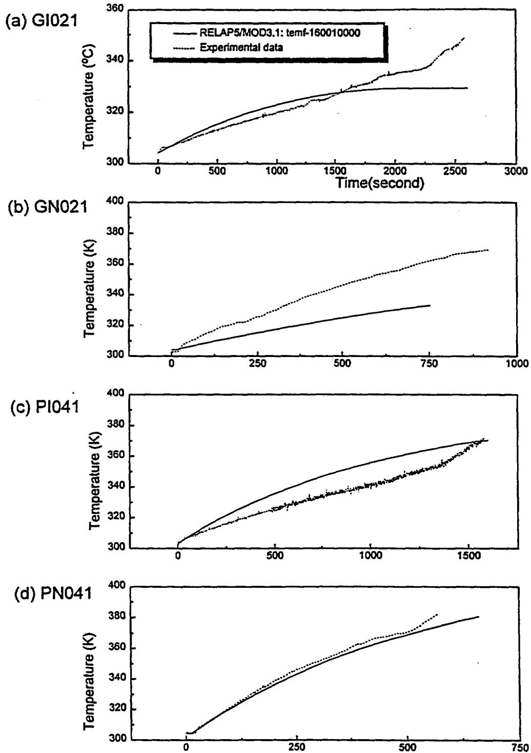
Figure 3.4: Comparison of the pool water temperature between experiments and calculation
