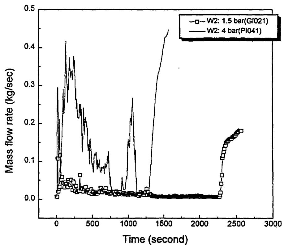
Figure 2.11: The effect of the high pressure on the injection flow rate for test GI021 and PI021
