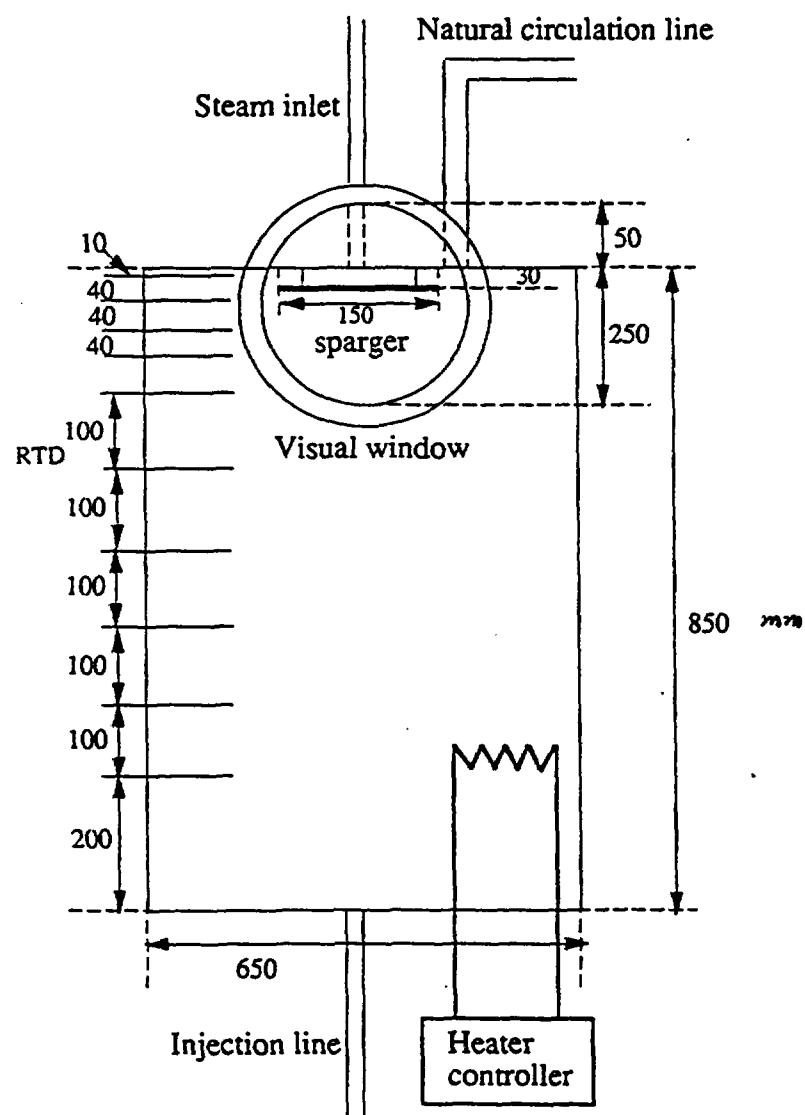
Figure 2.2: A systematic diagram of test section
