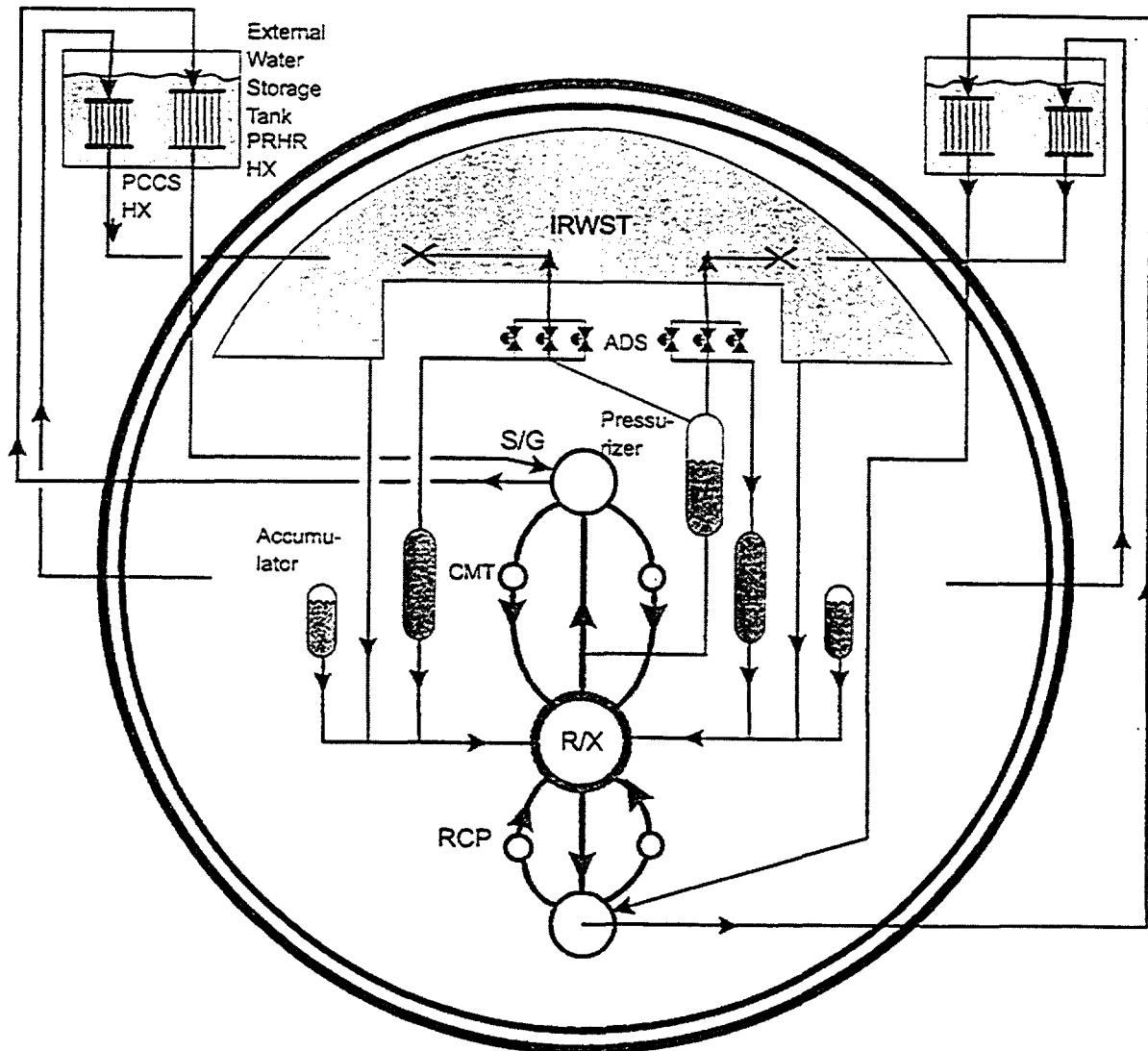
Figure 1.1: A schematic diagram of CARR Next Generation Reactor
