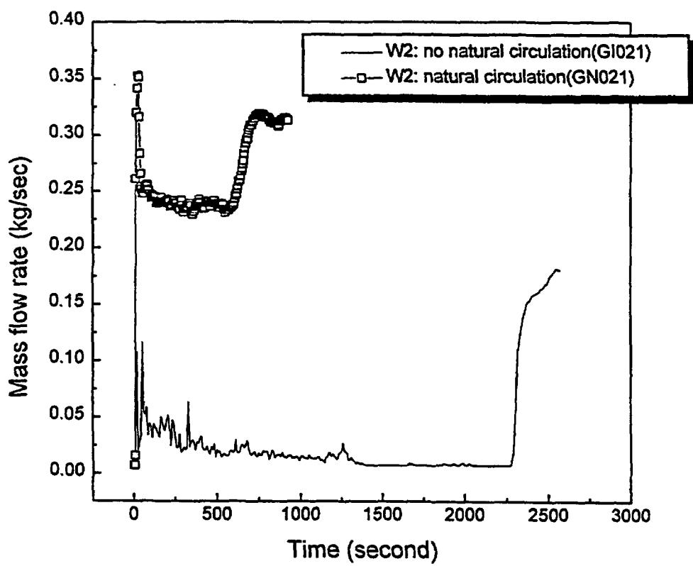
Figure 2.6: The effect of the natural circulation on the injection flow rate for test GI021 and GN021
