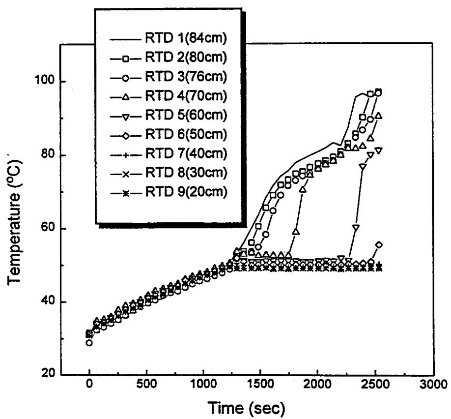
Figure 2.5: The temperature distribution of test section for test GI021
