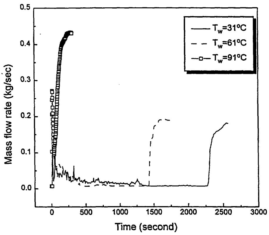
Figure 2.4: The effect of water subcooling on the injection flow rate for test GI021, GI022, and GI023
