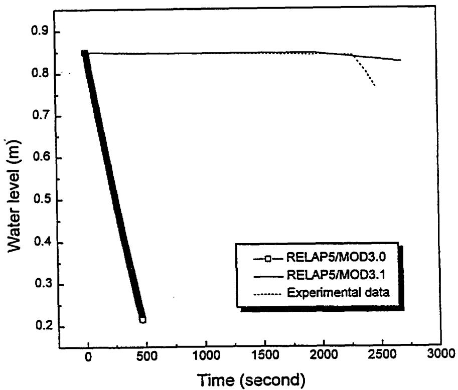
Figure 3.12: Comparison of the water level between test GI021 and calculation(MOD3.0 vs MOD3.1)
