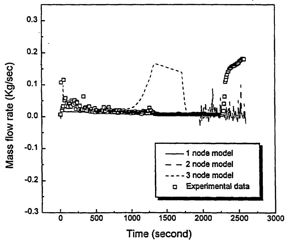
Figure 3.16: Comparison of the injection flow rate between test GI021 and calculation(Nodalization study)
