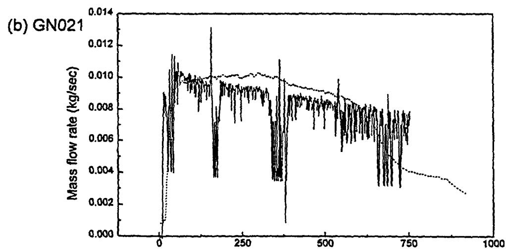
Figure 3.5: Comparison of the steam flow rate between experiments and calculation
