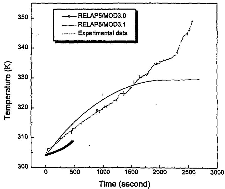
Figure 3.9: Comparison of the pool water temperature between test GI021 and calculation(MOD3.0 vs MOD3.1)
