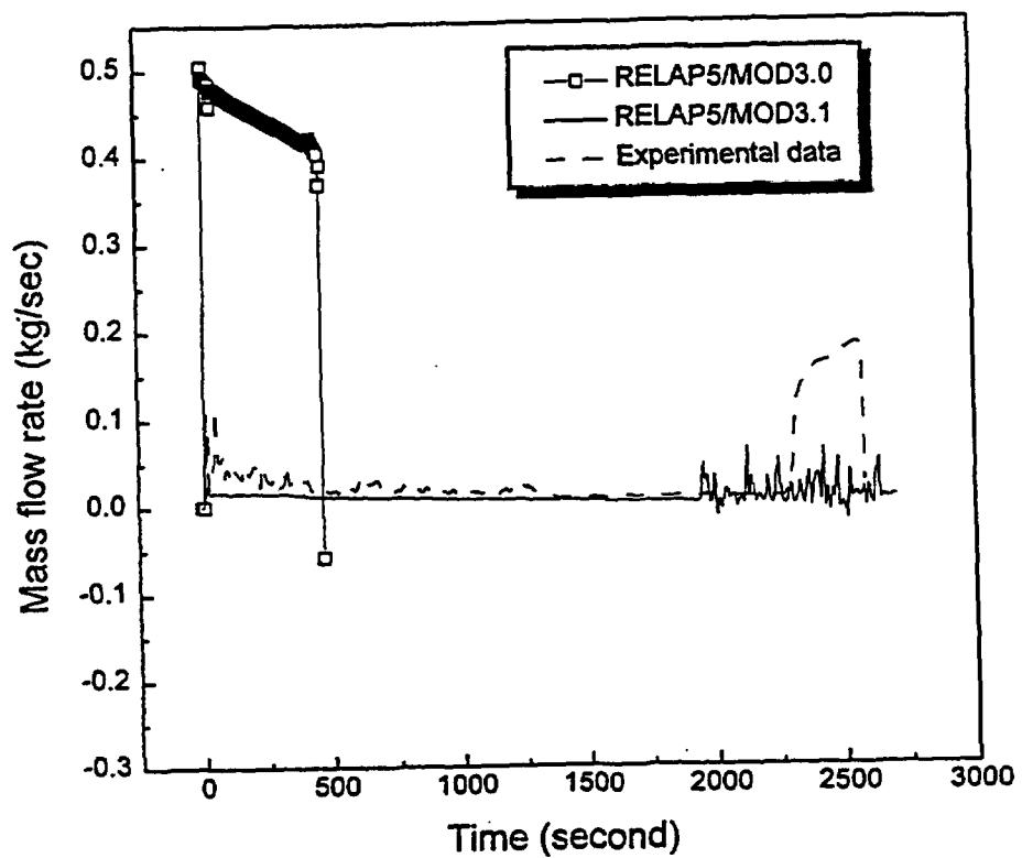
Figure 3.11: Comparison of the injection flow rate between test GI021 and calculation(MOD3.0 vs MOD3.1)
