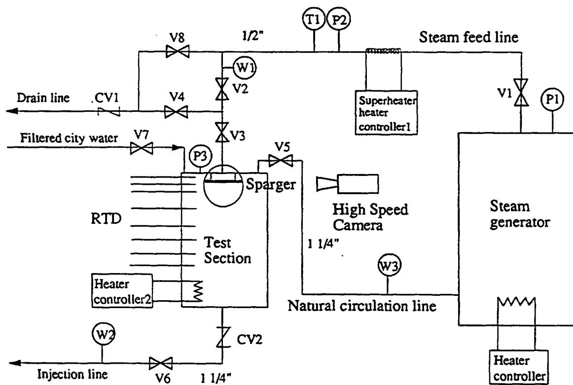
Figure 2.1: A systematic diagram of test facility
