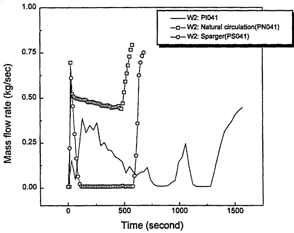
Figure 2.13: The injection flow rate at 4bar for test PI041, PN041, and PS041
