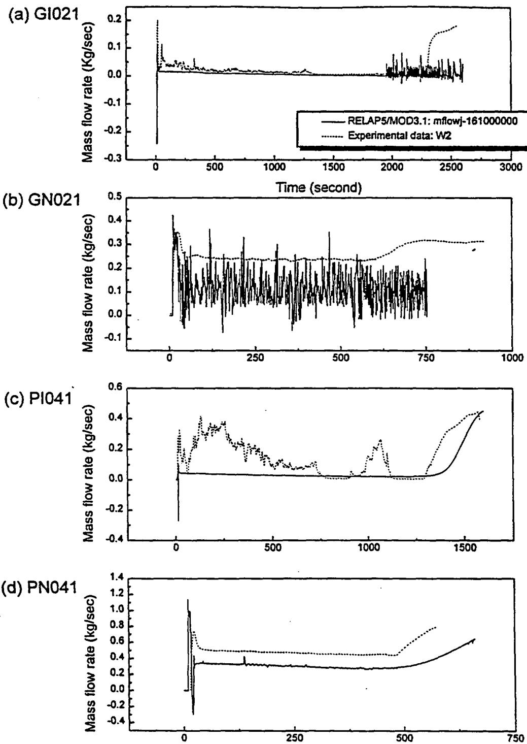
Figure 3.6: Comparison of the injection flow rate between experiments and calculation
