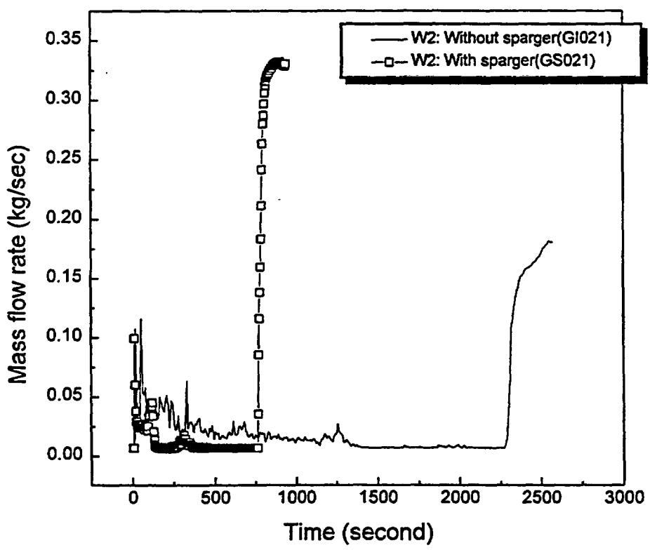
Figure 2.9: The effect of the sparger on the injection flow rate for test GI021 and GS021
