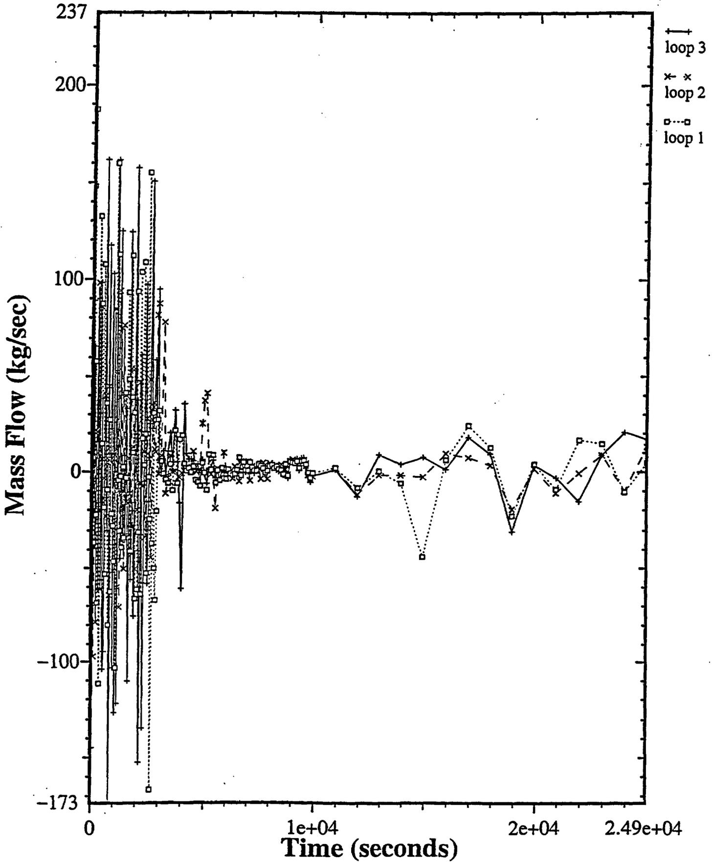
Figure 9: Cold leg mass flow rates.
