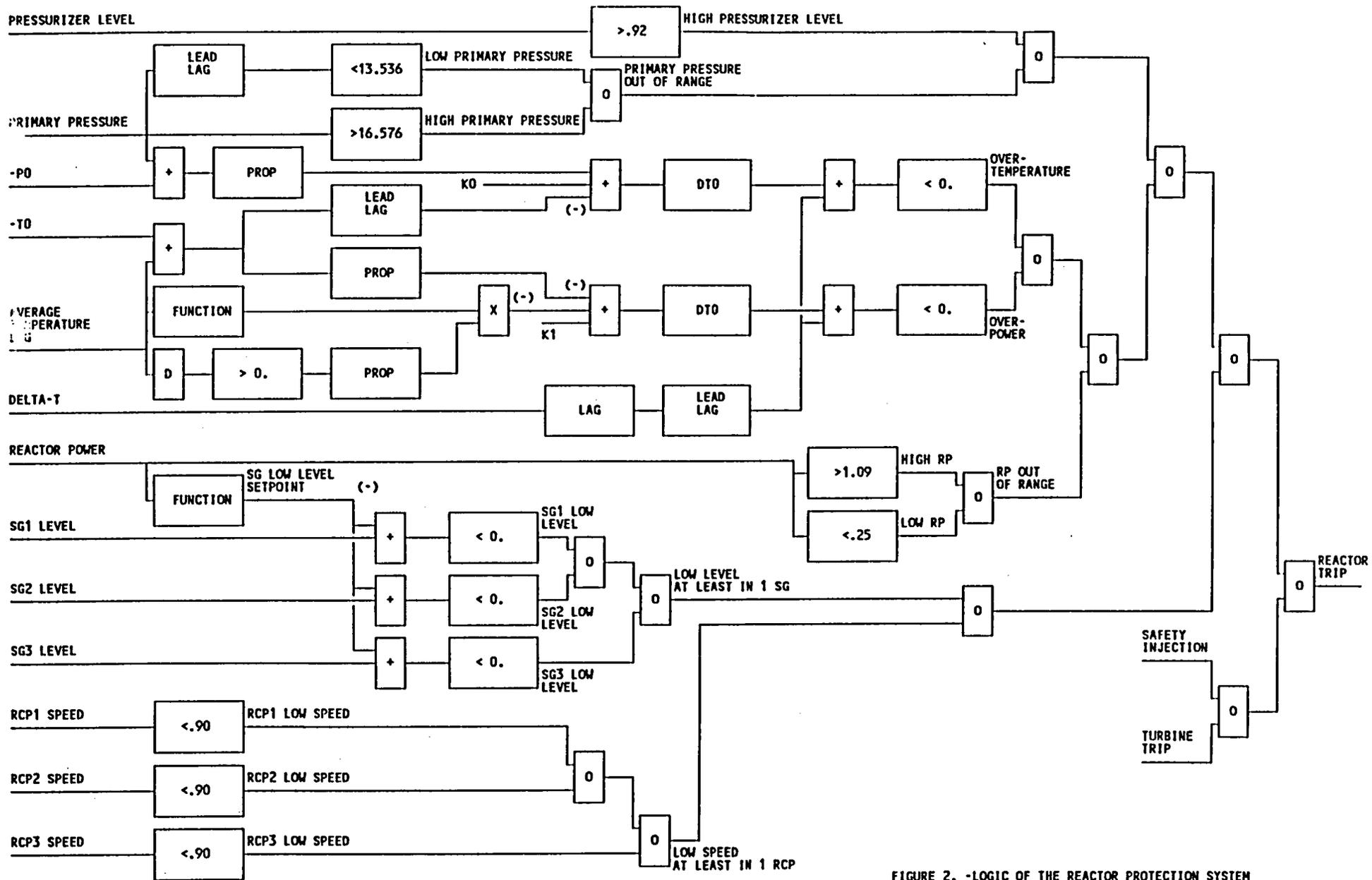
FIGURE 2. -LOGIC OF THE REACTOR PROTECTION SYSTEM
