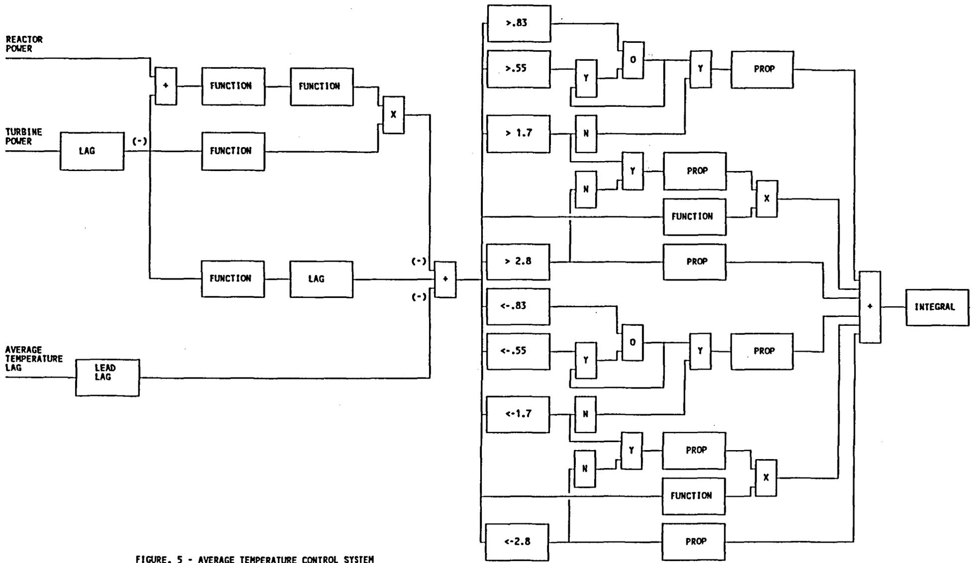
FIGURE. 5 - AVERAGE TEMPERATURE CONTROL SYSTEM
