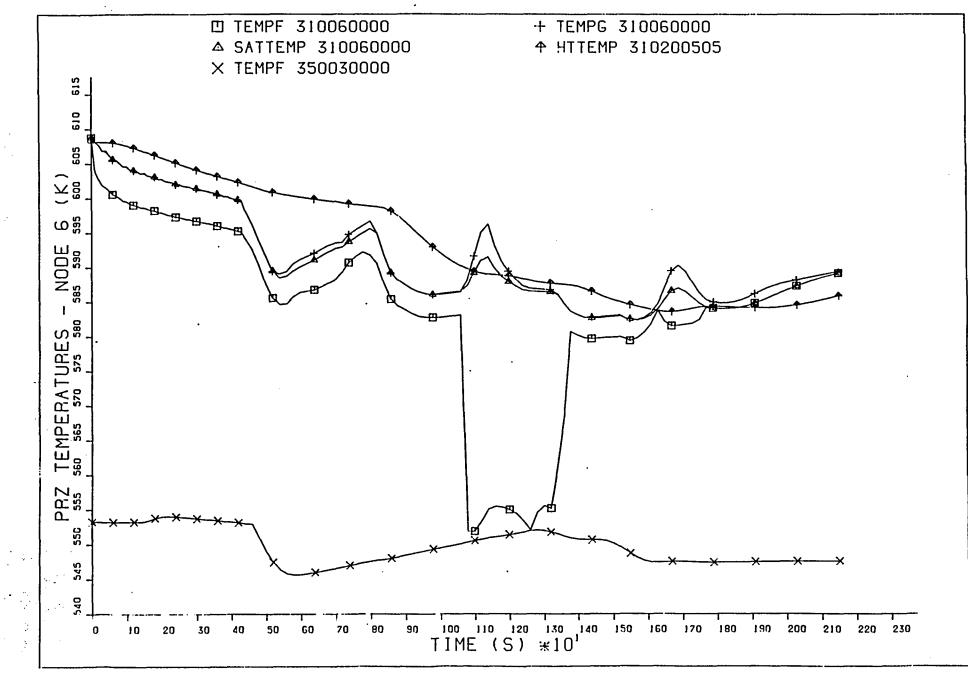
(FIG 6.22) UNION-FENOSA ICAP INADVERTED PRZ SPRAY TOTAL OPENING
