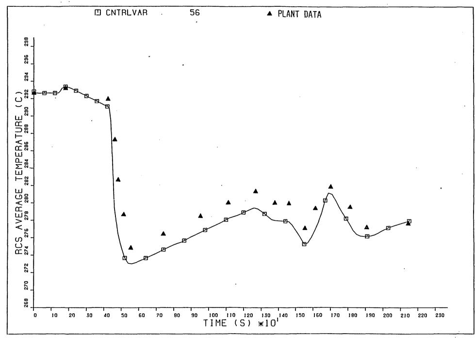
UNION-FENDSA ICAP INADVERTED PRZ SPRAY TOTAL OPENING (FIG 6.2)
