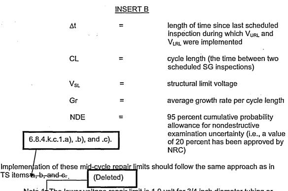
Note 1 The lower voltage repair limit is 1.0 volt for 3/4 inch diameter tubing or 2.0 volts for 7/8 inch diameter tubing.
