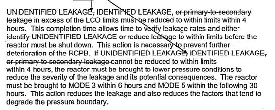
The allowed completion times are reasonable, based on operating experience, to reach the required plant conditions from full power conditions in an orderly manner and without challenging plant systems. In MODE 5, the pressure stresses acting on the RCPB are much lower, and further deterioration is much less likely.
