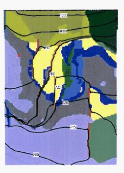
(a) (b) Figure 1. Comparison of Calculated Hydraulic Head Contours for Grid S6b-Run 1 at Layer 7 in (a) GMS Version 6.0 and (b) GMS Version 5.1
