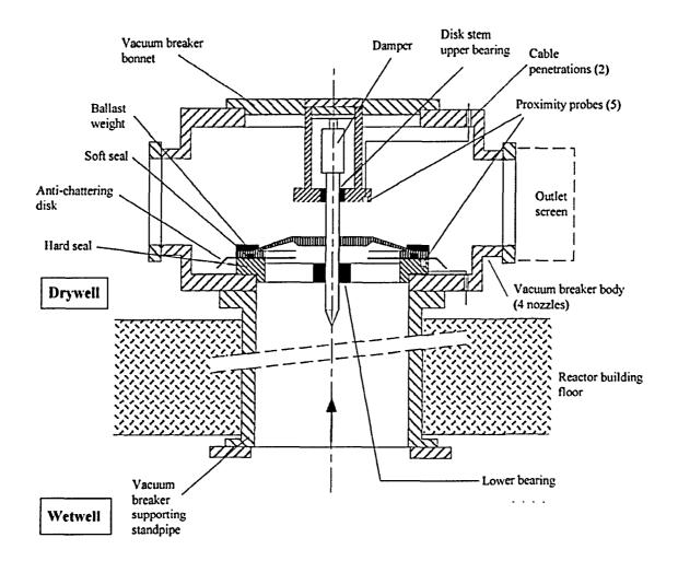
Figure 6.2-28. Vacuum Breaker Design Features
