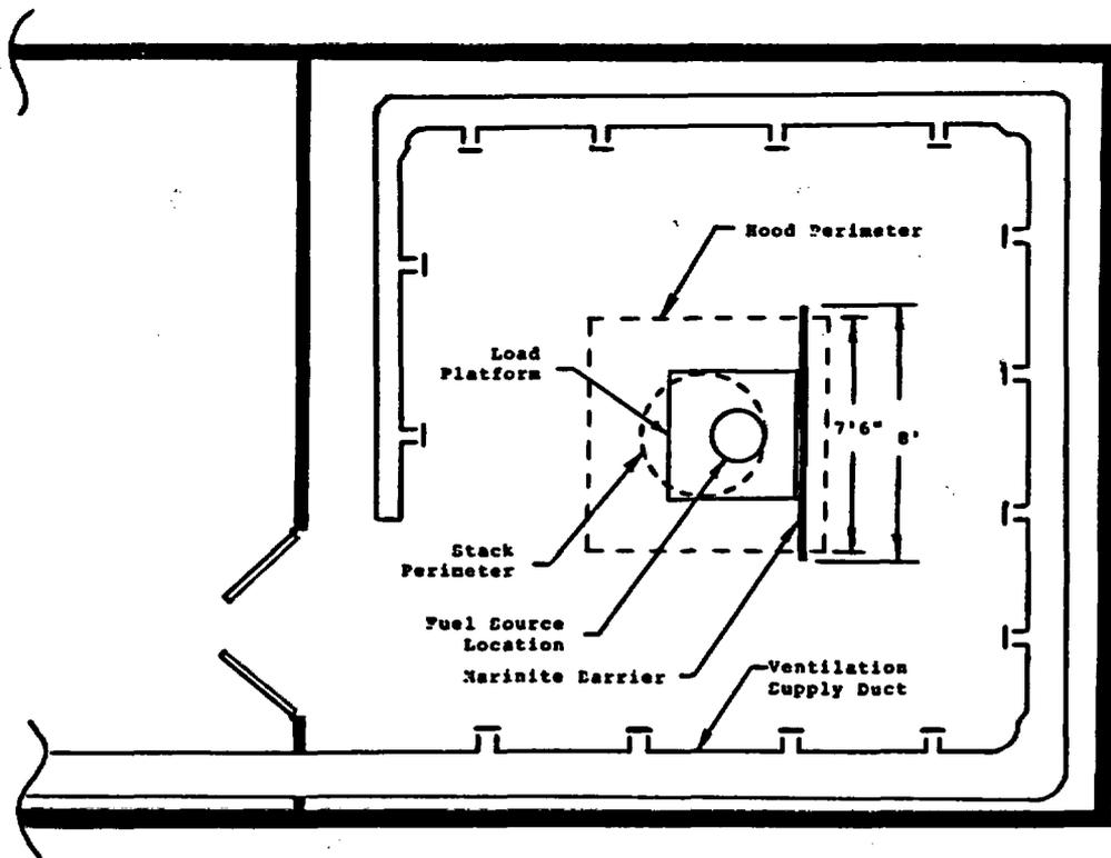
**Figure 2 Exhaust gas collection hood and fuel placement used for trash fire tests**
