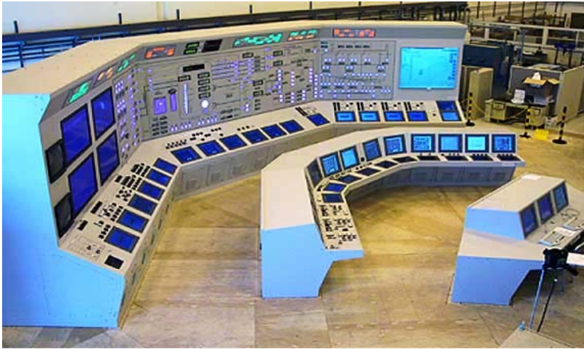
Lungmen Digital Control Room Simulator
